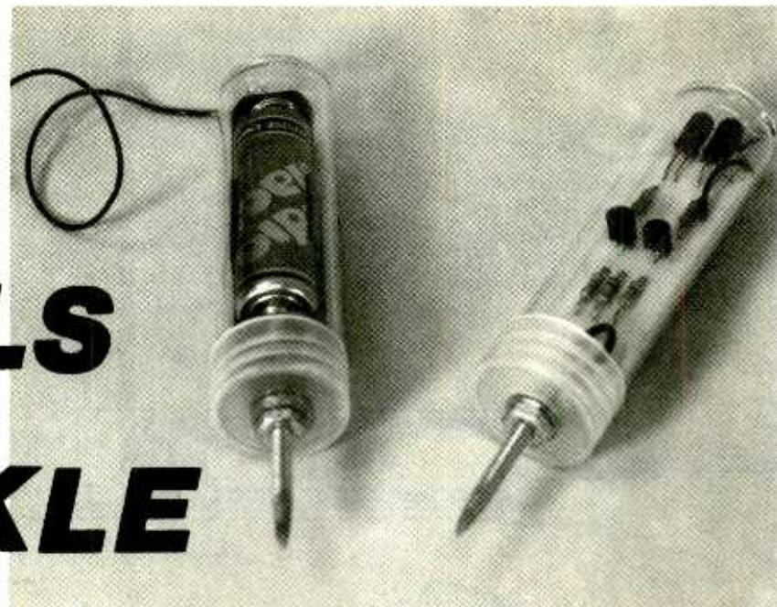
nected in series. An alligator clip is attached to one end of that series-connected pair, and a probe tip connected the other end. When the ends of the Continuity Tester are connected to two points in the circuit under test and there exists a continual path between the two points, the lamp will light, indicating that the points are electrically connected.
