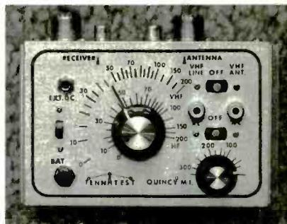
The Tennantest antenna noise bridge offers several useful RF-measurement capabilities, including the determination of resonant frequency of a tuned circuit or antenna, the SWR at resonance, resistive impedance, inductive reactance, and capacitive reactance.
