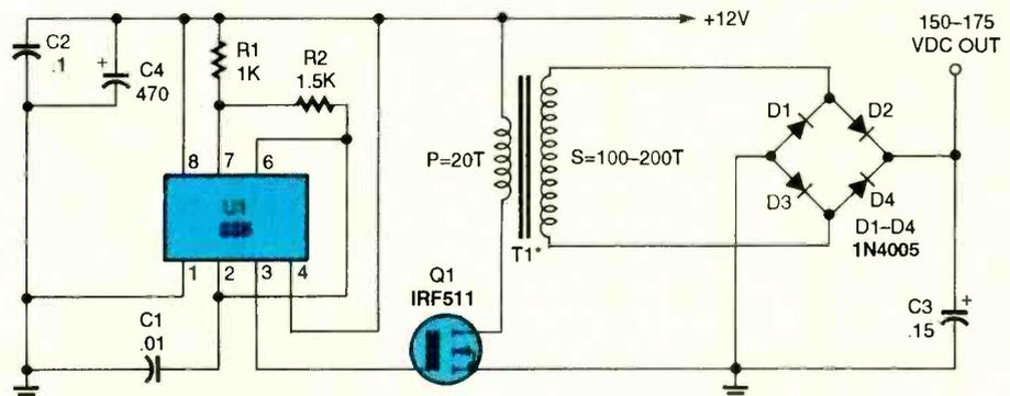
Fig. 6. In this DC-to-DC converter, the 555 is used to produce a rising and collapsing field in T1's primary, generating a higher voltage in T1's secondary winding. That voltage is then fullwave, bridge rectified by D1-D4, and filtered by C3.
