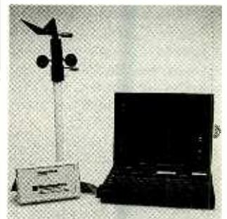
and accessed by other real-time DOS programs. An alarm function sounds the audible annunciator in the computer whenever the peak wind speed exceeds the value set by the user. An optional relay can also activate an external device whenever the wind speed alarm limit is exceeded.
