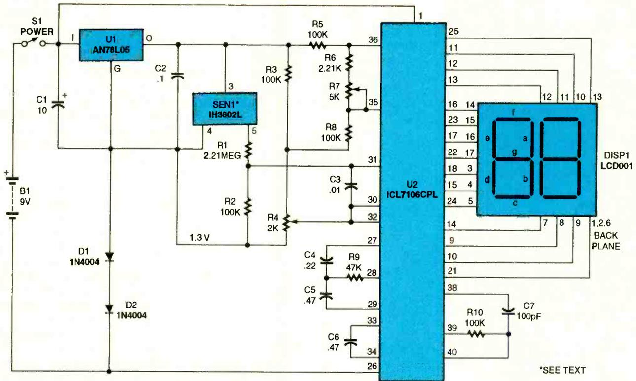
Fig. 1. At the heart of the Digital Relative Humidity Gauge is the Hy-Cal IH3602L, SEN1 (a 6-pin CMOS device with active 3-terminals).
