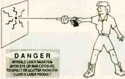
Advanced project produces a burst of light energy capable of burning holes in most materials. Hand-held device uses rechargeable batteries. 500 joules of flash energy excite either a neodymium glass, yag or other suitable 3" laser rod. This is a dangerous CLASS IV project (individual parts/assemblies available).
