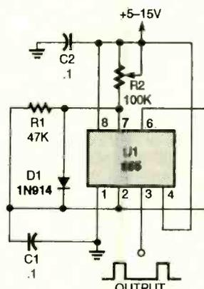
Fig. 2. At the instant that power is applied to the 555 astable, timing capacitor C1 is initially discharged, causing the output of the chip output at pin 3 to be high. Once C1 has charged to about  $\frac{2}{3}$  of the supply voltage, its output goes low, and the discharge transistor turns on, draining the charge on C1.
