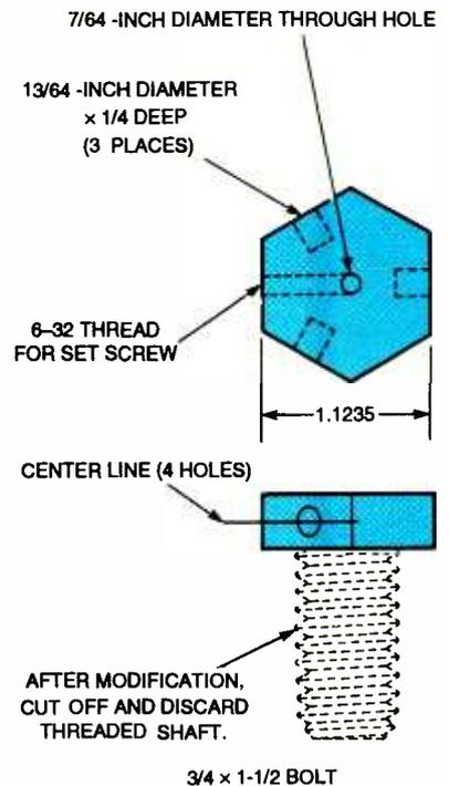
Fig. 3. The rotor hub was fabricated from a  $\frac{3}{4}$ -inch  $\times$   $1\frac{1}{2}$ -inch bolt head. The bolt head was drilled (as shown in this diagram) and shaft of the bolt was cut off. The bolt head was retained as the rotor hub and the shaft was discarded.
