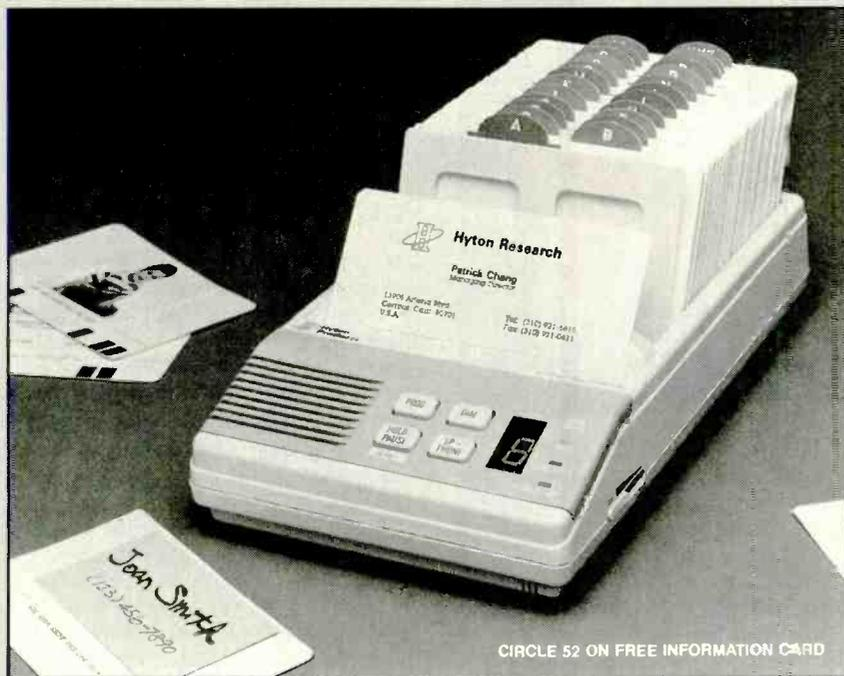
card is pulled from the card file and inserted in the reader slot. Then the DIAL button is pressed. The Phonedex automatically dials the correct number.
