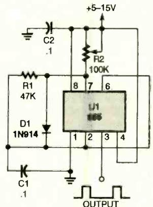
Fig. 2. At the instant that power is applied to the 555 astable, timing capacitor C1 is initially discharged, causing the output of the chip output at pin 3 to be high. Once C1 has charged to about  $\frac{2}{3}$  of the supply voltage, its output goes low, and the discharge transistor turns on, draining the charge on C1.
