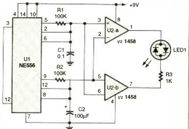
Fig. 3. If you want a really unusual display, check out this LED circuit which slowly shifts between three colors automatically.
