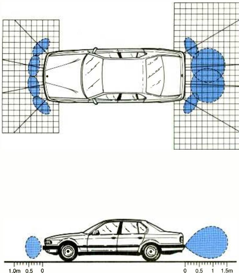
Fig. 3. Detection zones for the PDC system tend to be tight around the front of the vehicle, but less snug toward the rear.
