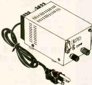
Solid state, fully regulated 13.8 Vdc power supply. 6 AMPS constant, 8 amps surge. Features 100% solid state construction, fuse protection, LED indicator and automatic cutoff short protection.
