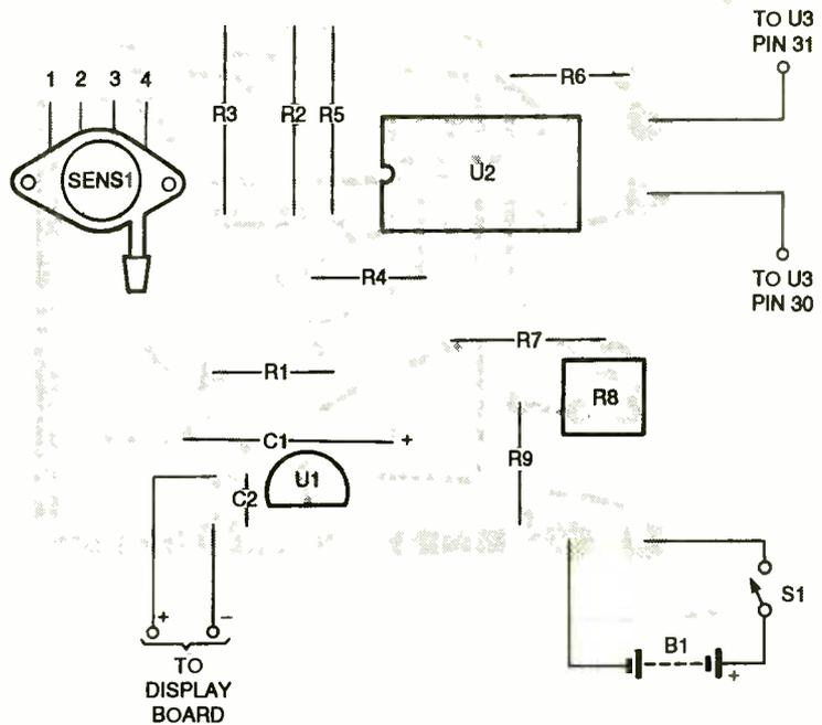
Fig. 5. When assembling the analog board (guided by this parts-placement diagram), it is recommended that sockets be used for the DIP IC's.
