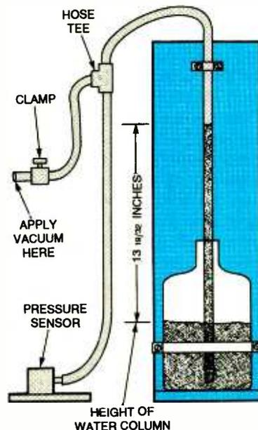
*Fig. 7. For those who wish to obtain the greatest possible accuracy from the circuit, this set up can be used to calibrate the Digital Barometer using a procedure founded in some basic laws of physics.*
