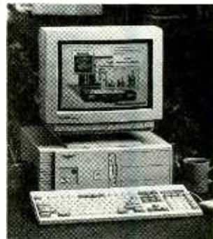
open device bays. The system includes a 101-key enhanced keyboard, a two-button mouse, Super VGA graphics, one game port, one parallel port, and two serial ports.
