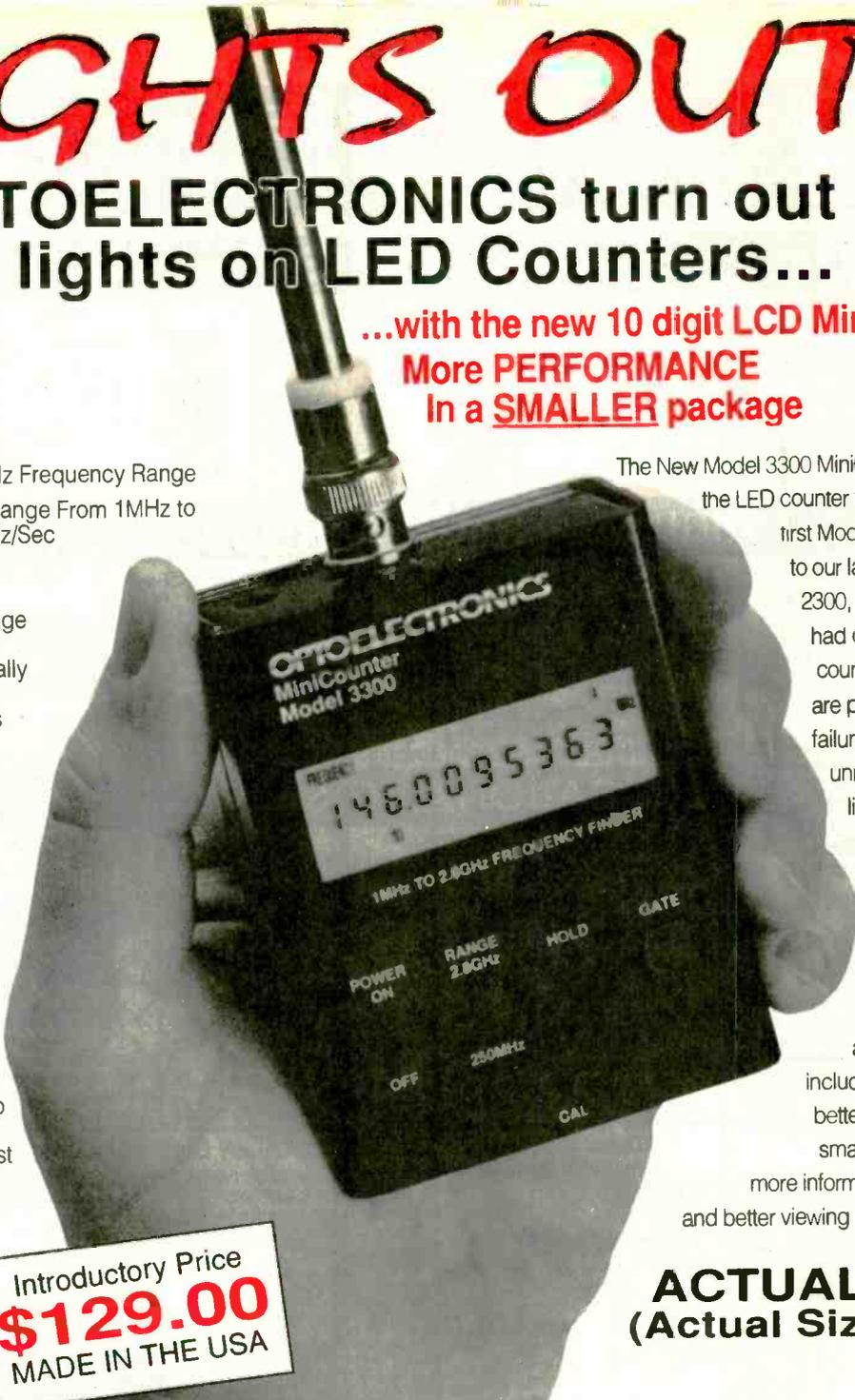
The New Model 3300 MiniCounter breaks the LED counter tradition. From our first Model FC50 (1976) to our latest Model 2300, we have always had quality LED counters. But LEDs are power hungry, failure prone and unreadable in sun light. So the LED counter has now gone the way of the LED wristwatch—replaced by LCD. The LCD advantages include lower power, better reliability, smaller package, more information displayed and better viewing characteristics.
