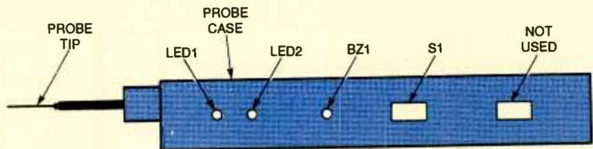
Fig. 5. Here is a graphic representation of enclosure and top-panel layout provided with the kit of parts offered in the Parts List. Even if you choose not to purchase a kit, you might still consider laying out your unit in a similar fashion.
