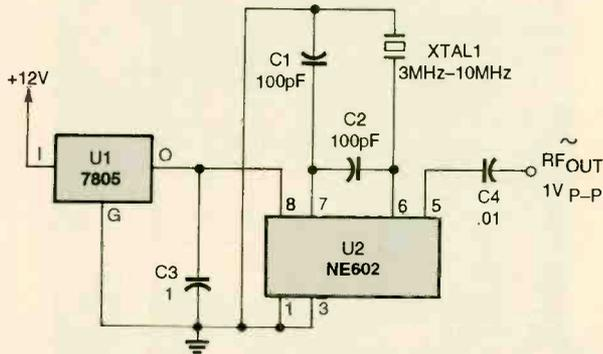
Fig. 5. Built around the oscillator section of an NE602 double-balanced mixer, the operating frequency of this is also crystal controlled.
