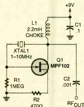
Fig. 2. The unijunction oscillator shown here allows higher frequency operation, and like the previous circuit, uses a quartz crystal (XTAL1) to set its operating frequency.
