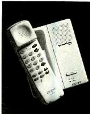
the range of conventional, 46-49-MHz cordless phones and has the added advantages of clarity and security. Conversations are digitized and encoded between the base and the handset; the phone features more than 100,000 digital security codes. In addition, the voice data "hops" over 100 channels. Other features include a concealed handset antenna, 3 ways to mount the handset in the base (upright, horizontal, or wall mount), user-replaceable battery, and handset-speaker volume control.
