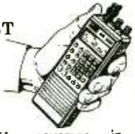
500KHz to 1300MHz coverage in a programmable hand held. Ten scan banks, ten search banks. Lockout on search and scan. AM plus narrow and broadcast FM. Priority, hold, delay and selectable search increment of 5 to 995 KHz. Permanent memory. 4 AA ni-cads and wall plus cig charger included along with belt clip, case, ant. & earphone. Size: 6 7/8 x 1 3/4 x 2 1/2. Wt 12 oz. Fax fact document # 205
