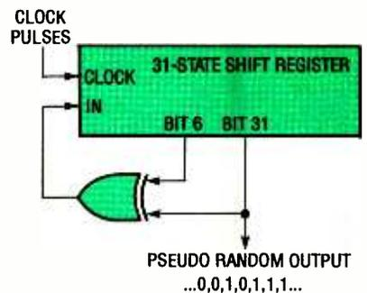
Fig. 2. Shown here is just one of a whole family of shift-register circuits used to produce pseudo-random sequences.
