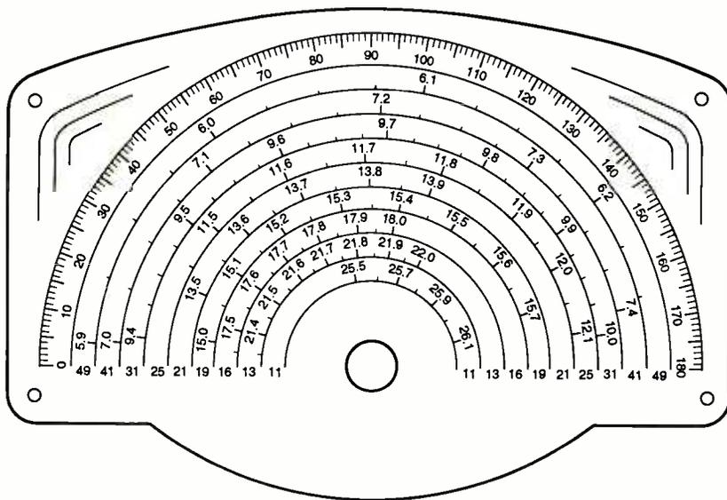
Fig. 7. Using a marker generator, the author first located and marked the 100-kHz points on the tuning dial, then the 50-kHz points, followed by 25-kHz points. This is what his dial looked like when completed. The dial shown here is strictly for reference. Each unit is different and must be calibrated according to the instructions given in the text to compensate for the tolerances of the actual components used in the set.
