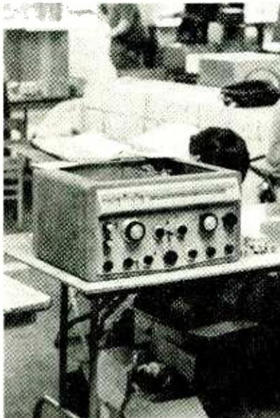
*Looking somewhat forlorn as it waits for a new owner at a radio hamfest, this high-end E. F. Johnson Viking Invader 2000 was an impressive all-mode, high-power amateur transmitter from the 1950's. It covered 3.5–30 MHz in seven bands. It could operate on SSB, AM, and CW, trying to bridge the gap between older and emerging communications modes.*
