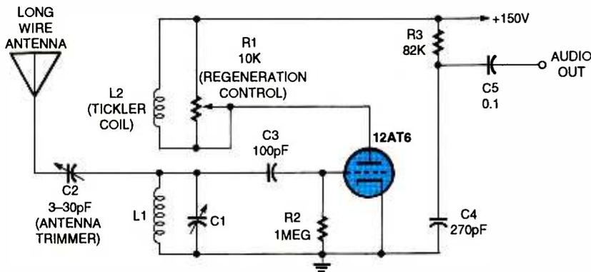
Fig. 1. The traditional tube-based regenerative receiver is essentially an Armstrong RF oscillator with variable feedback that is connected to an antenna and a resonant circuit.
