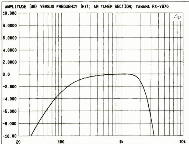
Yamaha made no claims for the frequency response of the AM-tuner section of this receiver, and this plot shows why. Unfortunately, such performance is typical of many otherwise excellent stereo receivers.
