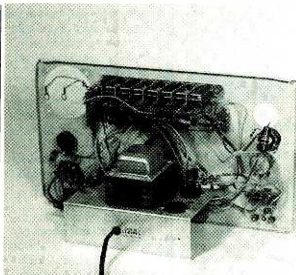
*The rear view of the TO-4 with its case removed. The assembly at the top of the panel is the pushbutton-switch unit.*
