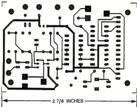
Fig. 3. The author's prototype was assembled on a double-sided printed circuit board, measuring about  $2\frac{7}{8}$  by  $1\frac{15}{16}$  inches. Shown here is a full-size template of the foil side of the board.
