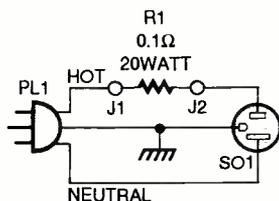
Fig. 2. Testing heavy-load devices with a ten-amp maximum meter can be accomplished with this straight-forward meter add-on. If done right, it could be made from a high-current extension cord.
