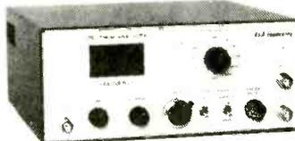
Features: Three digit LED center frequency readout. 12 position calibrated scan width 1 KHz to 50 MHz, switchable bandwidth: wide = 300 KHz, narrow = 15 KHz. Use your low frequency scope for the display. Switchable 10 KHz video filter: Variable IF attenuator. LOG output calibrated in 10 db steps.
