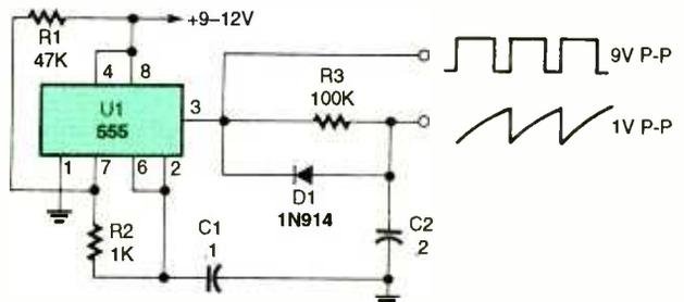
Fig. 2. This sawtooth generator is built around a 555 configured as an astable multivibrator.
