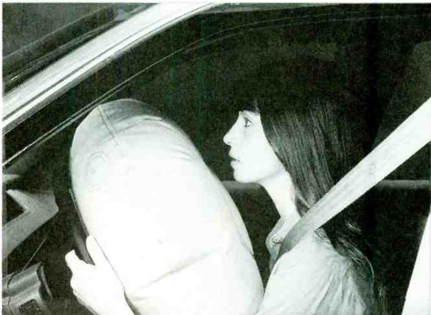
*While not a full-sized air bag like those installed in new cars and trucks, the aftermarket SRS-40 from Breed Technologies can provide air bag protection if seat belts are worn.*
