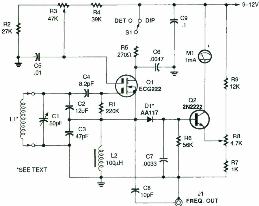
Fig. 2. The Gate-Dip Meter (a variation of its tube predecessor) is built around a dual-gate MOSFET (Q1) which is configured as a Colpitts oscillator.
