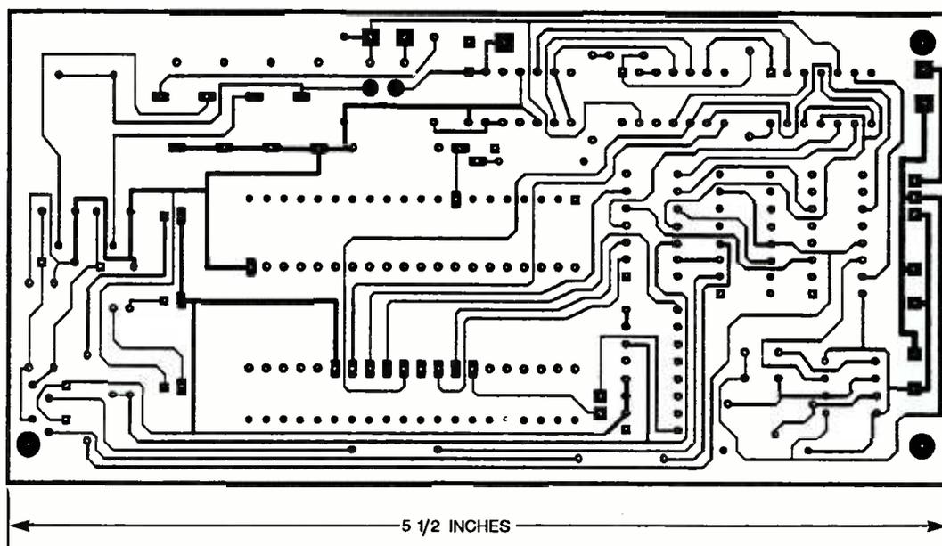
Fig. 2. The Auto-Ranging Digital Capacitance Meter was assembled on a double-sided, printed-circuit board measuring about 5½ by 2⅓ inches. A full-size template of the foil side of the board is shown here.
