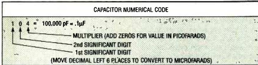
Fig. 3. Unlike resistors, a special numerical code is used on a capacitor's body indicate its value. The illustration shows what each digit in the code represents.
