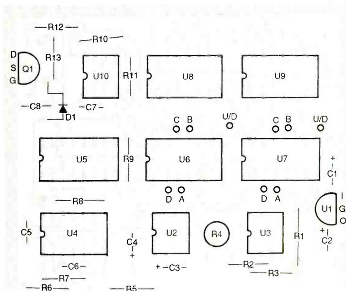
Fig. 4. Use this parts-placement diagram when installing the board-mounted components on the main circuit board.
