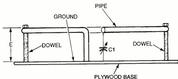
Fig. 3. Here's a side view of the DDDR. The ground plane can be made of sheet metal, metal screening, or even chicken wire.
