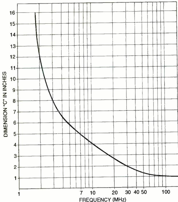
Fig. 2. The length of the air gap will depend on the operating frequency and can be found using this chart.
