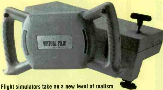
Flight simulators take on a new level of realism with *CH Products' Virtual Pilot*, which works just like a real airplane yoke. Virtual Pilot attaches to a PC through the game port, and features complete aileron and elevator control, throttle, tactile fire buttons located under the thumbs, and trim controls. Although designed for flight simulators such as Microprose's "Fleet Defender F-14 Tom Cat," Virtual Pilot works with every game that uses a standard joystick port. Price: \$109.95.
