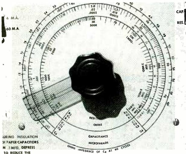
Here's a good look at the instrument's indicator dial. The multipurpose scale can be a bit confusing. Graduations have different values in different places, and must be interpreted with care.
