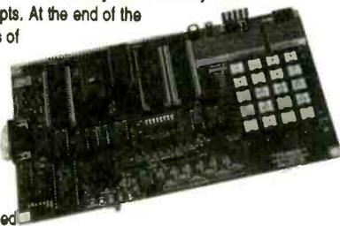
to start programming in machine language. Continue on to program in Assembler, Fort or BASIC with optional upgrade and software. Upgrade includes: RS232 serial port, a serial cable and, 32K of battery backed RAM. Picture shown with upgrade option and optional heavy-duty keypad installed.
