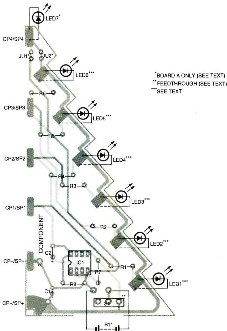
Fig. 4. Use this parts-placement diagram when building your unit. Note that some of the components mount on only one of the boards.
