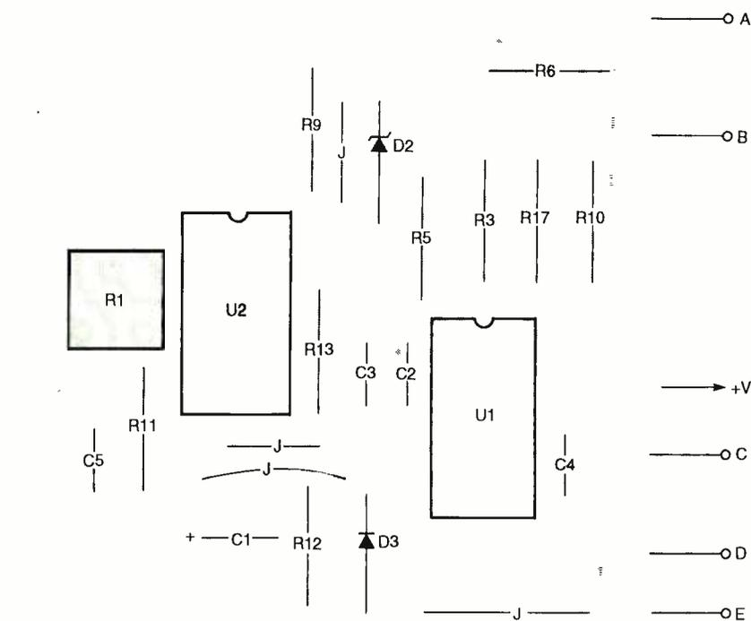
Fig. 3. Potentiometer R1 can be a board-mounted trimmer potentiometer or a panel-mounted unit. If R1 is to be a panel-mounted unit, solder three wires to the appropriate PC pads of the main board and connect their other ends to R1. You'll also need to attach five wires to the appropriate points on the main printed-circuit board to make the inter-board connections.
