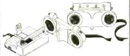
The ED-100 was designed for use as an auto/truck/RV back-up alarm. A digital display and audible beeper inside the vehicle inform the driver of the distance to impact beginning when the vehicle is within 14 feet of another object. Two 40 kHz ultrasonic emitter/detector modules, measuring 5.81" long X 1.9" wide, 2.05" thick, attach to the rear of the vehicle. The device operates on 12 or 24 Vdc.
