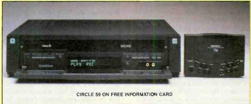
With the door pulled open, the VH8's split personality is revealed. To the left of the unit is the 8mm tape well, with the basic controls (STOP/EJECT, REWIND, PLAY, FAST FORWARD, PAUSE) arrayed in a row beneath it. The right side of the unit features the larger VHS tape well with the same array of controls, as well as the POWER button, audio/video in and microphone jacks, and the RECORD button. Between the two sets of control buttons is found the display.
