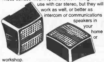
4", 4 ohm, speakers mounted in an unbreakable black plastic, slant-faced enclosure. They are rated 5 watts. Enclosure measures 4.82" X 4.5" X 2.45" h. Each pair is boxed and includes two short pieces of hook-up wire.
