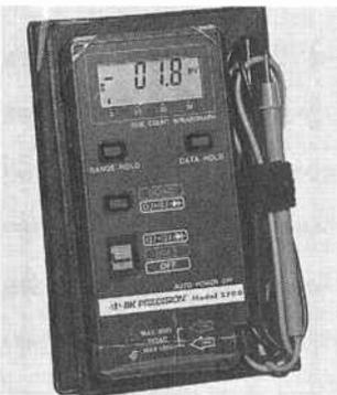
The Model 2700 is aimed at electronic technicians, electricians, home handymen, college students, and hobbyists. The pocket DMM measures up to 450 DC volts in five ranges with 1.3% accuracy (0.7% on the 3-volt range). It measures AC volts to 450 volts in four ranges, and resistance to 30 megohms in six ranges.
