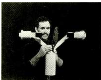
Here is an HSS Visibility Sensor being calibrated prior to its installation on the highway.
