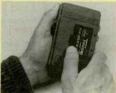
Cartridges slip into a slot on the back of the Bookman unit.
