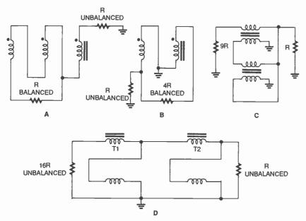
Fig. 3. There are several types of impedance-matching transformers: 1:1 balun (A), 4:1 balun (B), 9:1 un-un (C), and 16:1 un-un (D).
