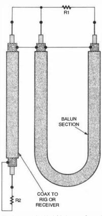
Fig. 1. A coaxial cable 4:1 balun transformer is made from 75-ohm coax cable.
