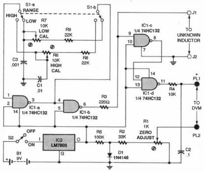
Fig. 1. With this simple Adapter circuit and an ordinary DMM you can measure inductances from 3  $\mu$ H to 5 mH.
