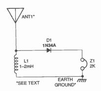
Fig. 3. This broadband RF tester will give you a good idea of the effectiveness of your antennalground setup.
