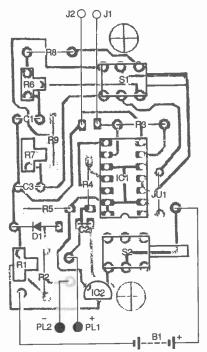
Fig 3. Use this parts-placement diagram as a guide when assembling the Inductance Meter Adapter.
