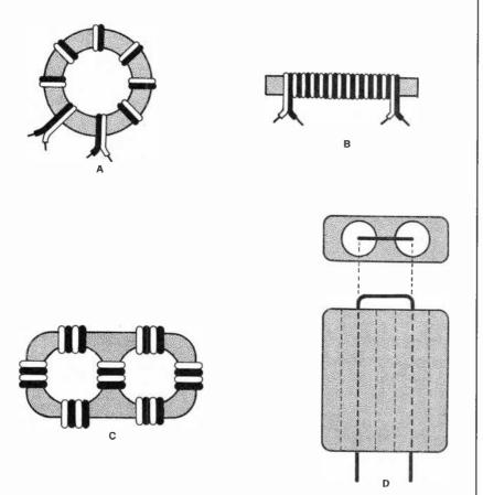
Fig. 4. Shown here are construction details for the most common types of transformers: toroid (A), 76 solenoid (B), bazooka-end view (C), and bazooka-top view (D).
