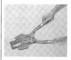
The Ribbon-Cable Assembly Tool can be used with interchangeable dies to accommodate a wide variety of connector styles and sizes. Optional dies are available for 14-, 16-, and 18-pin DIPs; card edge and D-sub connectors; sockets; and delta ribbon.
