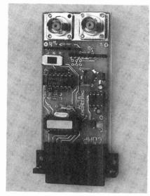
A really compact assembly for the Easyscope is possible when you use a double-sided PC board.
