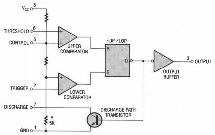
Fig. 4. This internal block diagram of a 555 timer reveals the comparators that operate an R-S flip-flop. They change state when their inputs reach voltage levels programmed by the resistor network.
