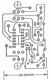
Fig 2. If you'd like to etch your own PC board for the Adapter, use this foil pattern.
