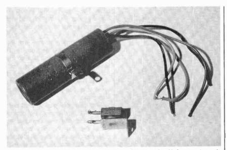
The multi-section electrolytic and the selenium stack rectifier were replaced before powering up the set for the first time.
