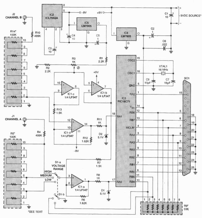
Fig. 1. The schematic for the Easyscope might look complex at a glance, but many of the functions are handled by IC3, a PICI6C71. As a result, this circuit and a PC can replace a complete oscilloscope.
