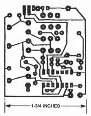
Fig. 2. If you'd like to build the Adapter on a PC board, use this foil pattern to etch your own.
