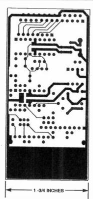
Fig. 3. This is the solder side of the Easyscope board.
