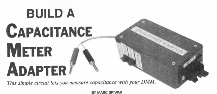
f your budget limits your test gear to a suitable digital multimeter (DMM), then you might want to consider adding a home-brew adapter to Increase its adaptability. One such budget gadget is the Capacitance Meter Adapter described in this article. It's an affordable little circuit that will enable your DMM to measure capacitance at a fraction of the cost of commercial units. As a matter of fact, depending on what parts you have on hand, the circuit could cost you only pennies to build!
