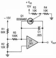
Fig. 8. This ramp generator steadily increases its output voltage until QI suddenly cuts it off.
