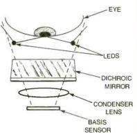
Fig. 2. This overhead view of the Eye Control system shows the twin LEDs illuminating the user's eye with an infrared beam. The position of the beam spots and the image of the user's eye reflect through the dichroic mirror and then pass through the condenser lens and are combined to form an image on the BASIS sensor.
