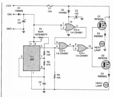
Fig. 1. This is the corrected schematic from the "Daytime Running Lights" article. The MOSFETs are now shown as P-channel types.
