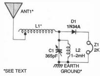
Fig. 6. While an effective crystal receiver, this circuit resembles an antenna-matching device used by amateur-radio operators.
