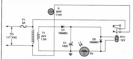
Fig. 1. This circuit uses light-dependent-resistor R1 to sense when a phone with a built-in flasher is ringing. Relay RY1 then closes, lighting lamp [].
