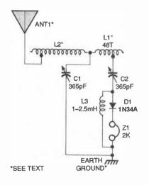
Fig. 7. This three-inductor receiver provides for impedance-matching of the antenna and diode detector.
