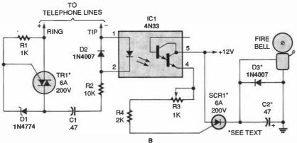
Fig. 4. This circuit (A) senses when a phone rings and activates a loud 10-inch fire bell. Its similar 66 companion (B) features an optocoupler.
