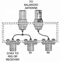
Fig. 2. Here's the connection box for making a 4:1 coaxial balun. It is intended for mounting on the antenna center insulator
