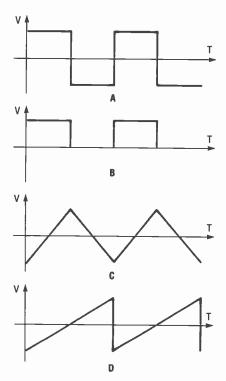
Fig. 1. The basic non-sinusoidal wave family consists of square waves (A), pulsed waves (B), triangle waves (C), and ramps (D).
