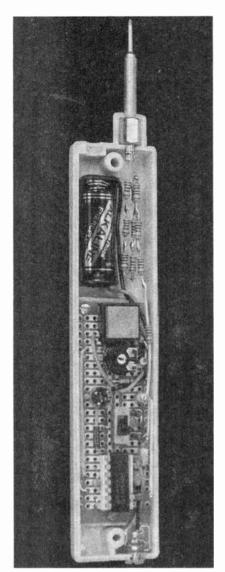
As this internal view of the Probe shows, the project can be assembled quite neatly within a standard logic-probetype case, using perforated board and point-to-point wiring.
