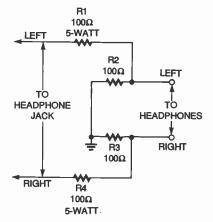
Fig. 2. To use most headphones with the Switchbox you will need an attenuator. Here's a simple add-on you can build in a few minutes.
