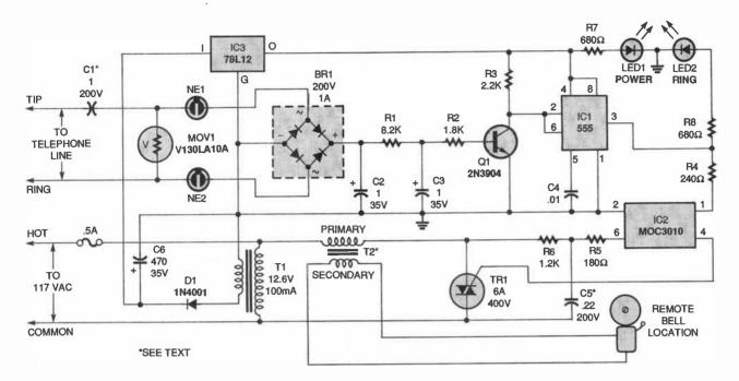
Fig. 5. This low-cost telephone-line extension bell ringer lets you hear your phone ringing in the garage, or in whatever other remote bell location you wish.
