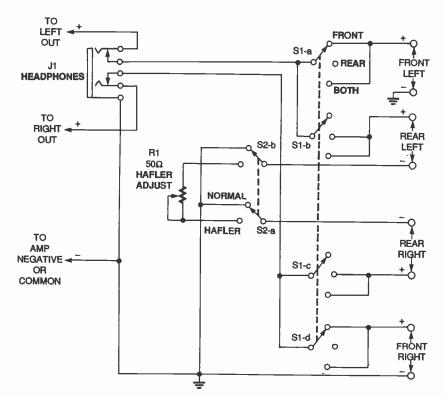
Fig. 1. The circuit for the Surround-Sound Switchbox requires no power source. It passively creates the Hafter effect using existing sum and difference signals.
