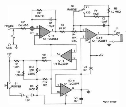
Fig. 1. Here's the schematic for the Active High-Impedance Probe. Note the placement of BP1 near pin 2 of IC1. That Teflon-insulated standoff will greatly help keep the circuit error free.
