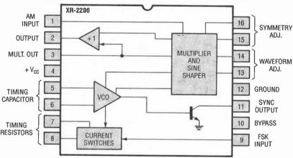
Fig. 9. This is a block diagram of the XR2206 function-generator. Chips like this make building a function generator easy.
