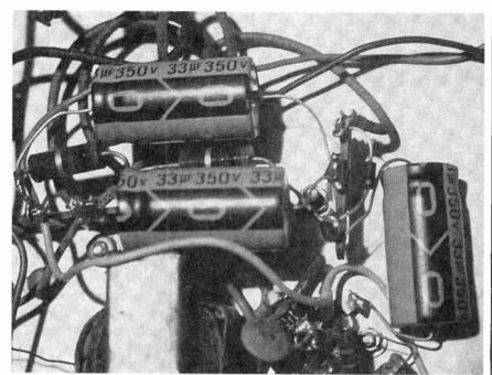
Three individual 33-µF, 350-WVDC electrolytics replace the filter capacitors in the old multisection unit.
