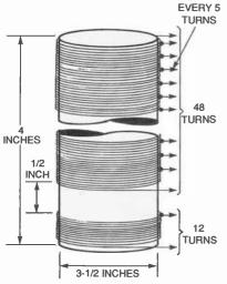
Fig. 1. This small coil is made up of two windings. Note that the 48-turn winding has taps at every five turns. The 12-turn coil will be used for RF coupling.
