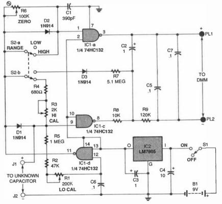
Fig. 1. Here's the schematic for the Capacitance Meter Adapter. The circuit outputs one-millivolt per picofarad in the LOW range setting of S2, and one-volt per microfarad in the HIGH range.
