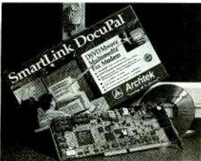
At the heart of the fax/modem is DSVD technology, which multiplexes voice and data for simultaneous transmission over a single phone line. The DocuPal automatically regulates the stream so that data transmitting at 28.8 kbps drops to 14.4 kbps when voice is added. The auto-mode and dynamic rate renegotiation ensure the fastest available speeds, even when connecting with slower modems.
