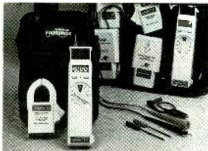
The briefcase-style kit comes equipped with an array of test accessories, including a complete set of test leads, short and long probe tips, an alligator clip, and a full line of accessory heads; a clamp for measuring AC current, and dual-temperature, relative-humidity, and micro-amp heads. The accessory heads slip easily onto the top of the DMM to expand its test capability to meet almost any test condition. For remote access or hard-to-reach
