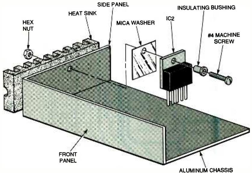
Fig. 5. It is important to electrically insulate IC2 from the chassis and heatsink.
