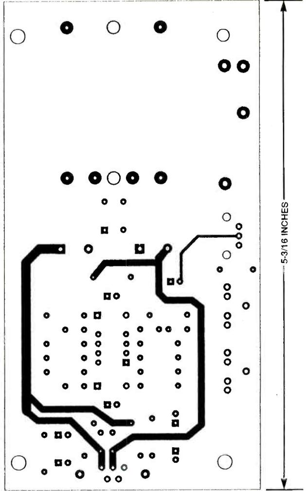
Fig. 2. This is a template of the component side of the Subwoofer PC board, shown full size.
