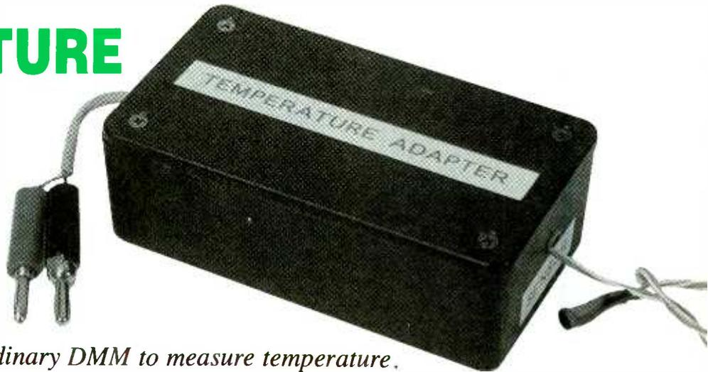
*Use this circuit and an ordinary DMM to measure temperature.*
