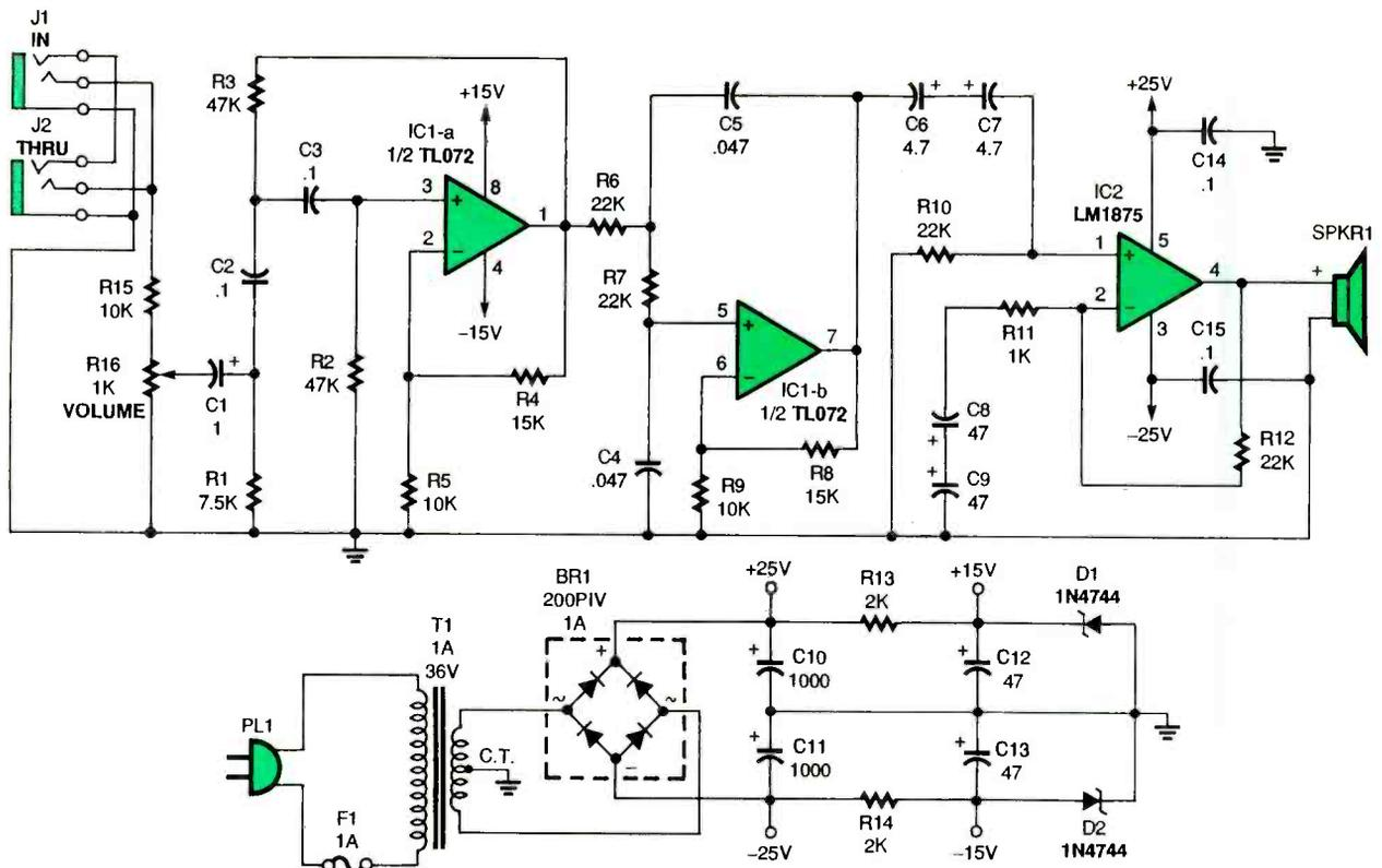
Fig. 1. Here's the schematic for the Multimedia Subwoofer. The circuit is greatly simplified by the use of an integrated 20-watt amplifier, IC2.
