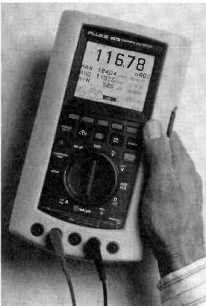
Several innovative technologies were used in the Model 867B's display, including blue LEDs from Nichia of Japan. The color is a broadband, sky blue that is converted to white backlight by means of an amber filter. Coupled with Hitachi's transmissive LCDs, the backlight technology provides higher contrast and a significantly brighter image than other display modes—while using less than half the power of backlights of similar intensity.
