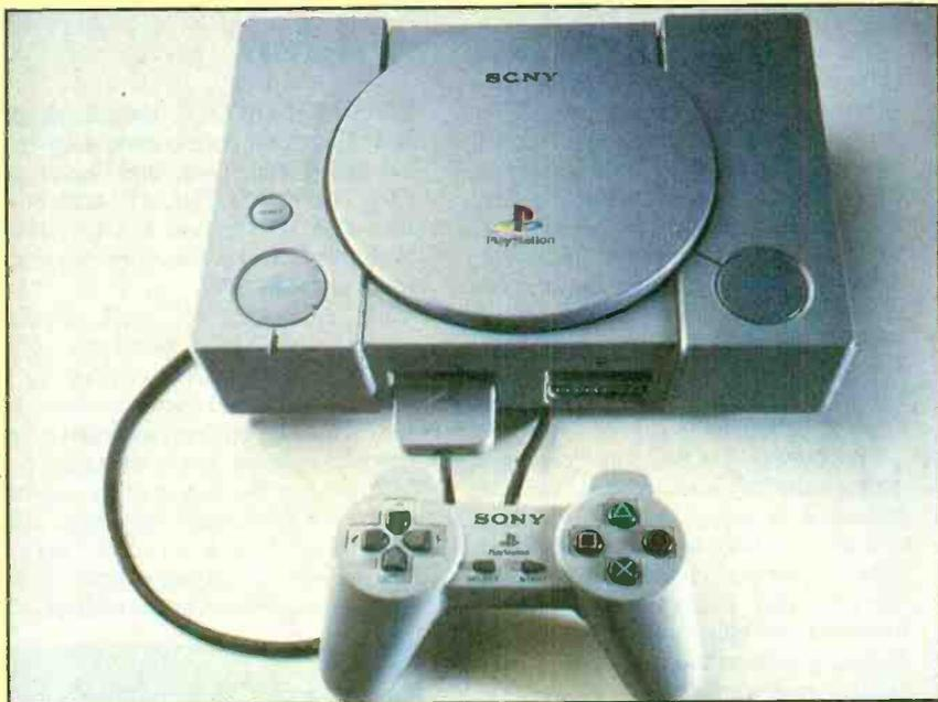
set-top box. At its heart is a 33-MHz, 32-bit RISC CPU that offers a 4-KB instruction cache and a 1-KB data cache. The CPU is backed up by a graphics processor (GPU) that provides a maximum of 16,770,000 colors and 640- × 480-dot resolution. The CPU also handles the texture mapping used in creating 3D games. In terms of audio, the PlayStation delivers CD-quality sound—and can be used to play audio CDs as well as games. The
