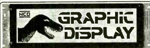
**NEW: RS-232 programmable 240x64 Graphic Display Module.** Upload your BMP/GIF Image Files at 9600/19200/38400/115200 Baud. Complete Support for 30x8 and 40x8 Text. Documentation and QBasic Software Gets You Running FAST!!! Counts as 2 Devices on the NCD RS-232 Network, use up to 8 GDSPs on a Single Serial Line. Many Price Options Available \$99-\$299.
