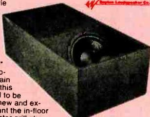
**Specifications:** 10" dual voice coil treated paper cone woofer with poly foam surround ♦ Frequency response: 30-100 Hz ♦ Nominal Impedance: 8 ohms per coil ♦ Power handling: 100 watts RMS channel/140 watts max ♦ SPL: 89 dB 1W/1m ♦ Dimensions: 27" D x 14-5/8" W x 9" H ♦ Net weight: 29 lbs.
