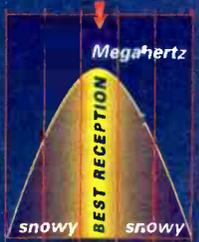
When TV signals are tuned at the TV channel's center frequency, optimum tuning has been achieved.
