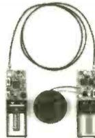
**Model AM/FM-108K Transistor Radio Kit**
