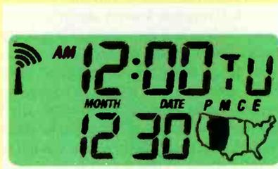
**The Time Machine's LCD displays more than just time, day, and date. The radio tower icon indicates excellent reception, and the map shows that the time zone is Mountain Standard Time.**
