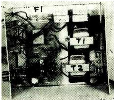
The Fusesaver was mounted in a medium-sized vented metal enclosure.
