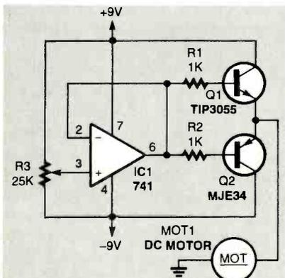
Fig. 7. When you need to provide a driver to a DC motor with reversal capability, this circuit should be utilized. Adjustment of control R3 allows you to control the motor's speed and direction of rotation.
