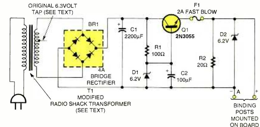
Fig. 1. Schematic of the "A" power unit with parts values noted.
