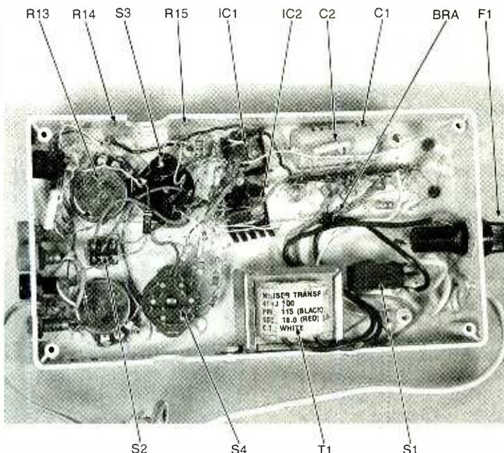
Shown here are the innards of the authors prototype. The unit was hard-wired into its plastic enclosure and the components interconnected with hookup wire. Note that the two trimmer potentiometers (R14 and R15) were glued to the inside wall of the enclosure and connected to the other components using point-to-point wiring techniques.
