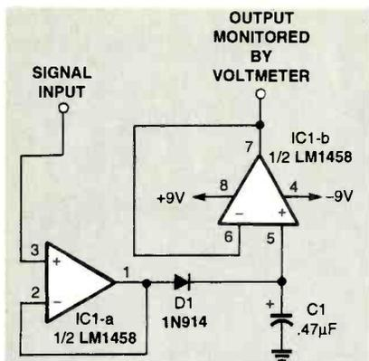
Fig. 6. Here is a simple application of a peak voltage detector and hold circuit using the LM1458 high dual op-amp. As the input changes, the corresponding output voltage at pin 7 is held at its peak value.
