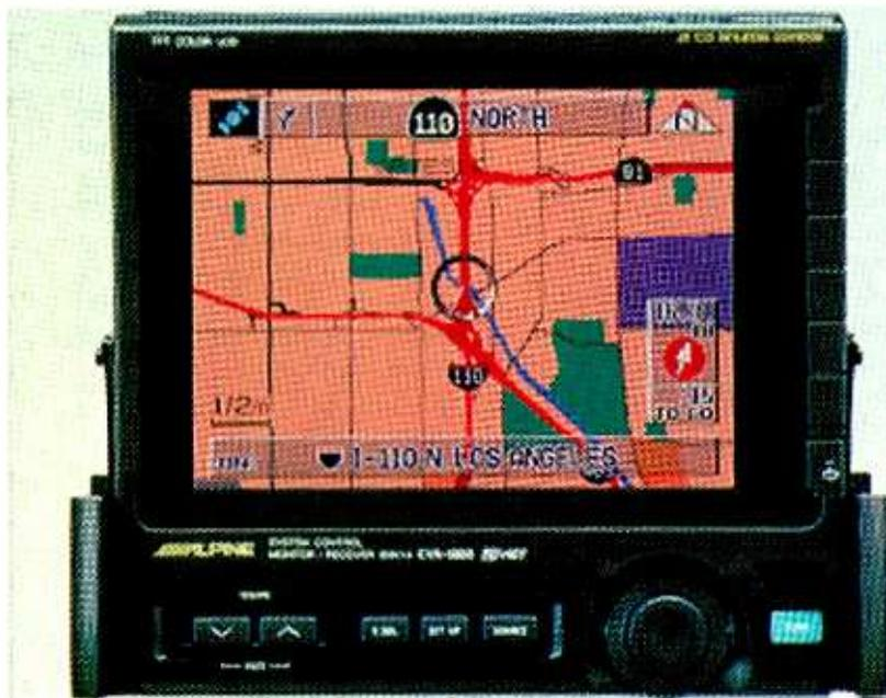
Alpine's CVA-1000 in-dash monitor/receiver combines an Alpine stereo system with an accurate satellite navigation system.
