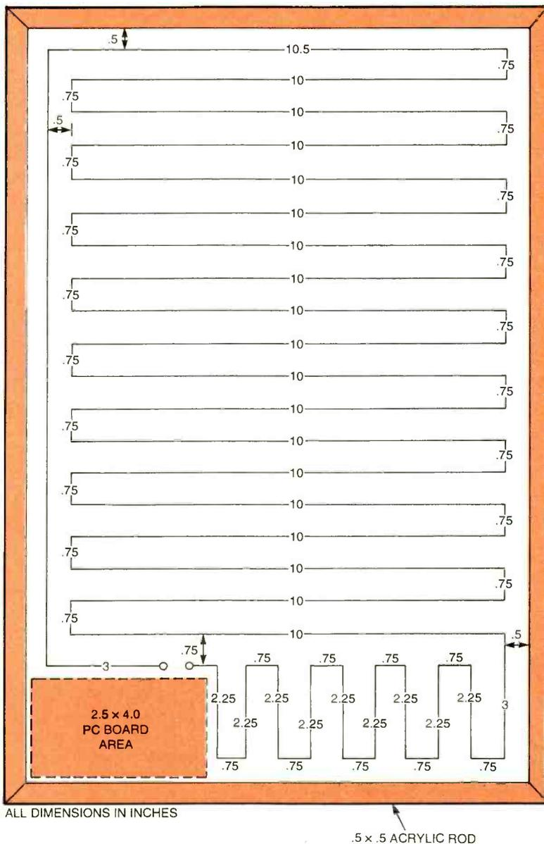
Fig. 3. Glue four lengths of  $\frac{1}{2}$ -inch square acrylic bar stock (mitered to  $45^\circ$  to form good  $90^\circ$  corners, as shown) around the edges, using a thickened clear acrylic cement. Following the pattern shown, lay down the #30 enamel insulated Nichrome wire heating element, and tape it in place with #69 Scotch glass-cloth electrical tape.
