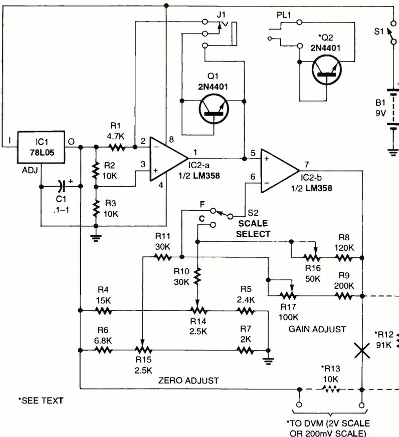
Fig. 10. The Electronic Thermometer can be used to convert any digital voltmeter (DVM) into a reasonably accurate thermometer capable of measuring from about  $-40^{\circ}$  C (or F) to over  $150^{\circ}$  C ( $302^{\circ}$  F). Or, if desired, a dedicated digital voltmeter module can be permanently connected to the circuit.
