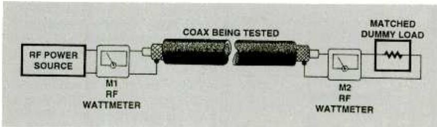
Fig. 4. Loss measurement setup for coaxial cable.
