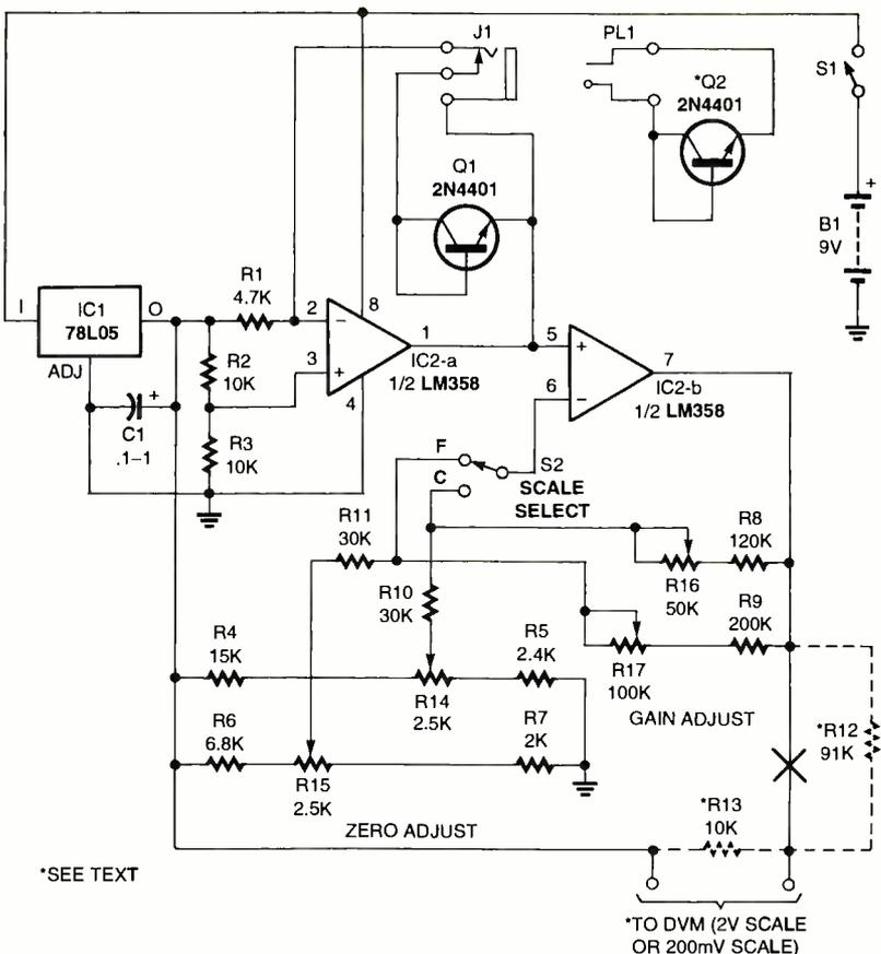
Fig. 10. The Electronic Thermometer can be used to convert any digital voltmeter (DVM) into a reasonably accurate thermometer capable of measuring from about  $-40^{\circ}\text{C}$  (or  $F$ ) to over  $150^{\circ}\text{C}$  ( $302^{\circ}\text{F}$ ). Or, if desired, a dedicated digital voltmeter module can be permanently connected to the circuit.
