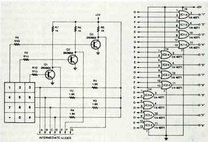
Fig. 5. This circuit is a neat interface for low-cost telephone-like keypads. The switches in the keypad select a specific row and column line when pressed. The 4071 IC provides the proper logic to identify the designated numerical keypad reference.
