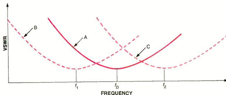
Fig. 2. Family of VSWR-vs.-frequency curves illustrating off-resonance conditions.
