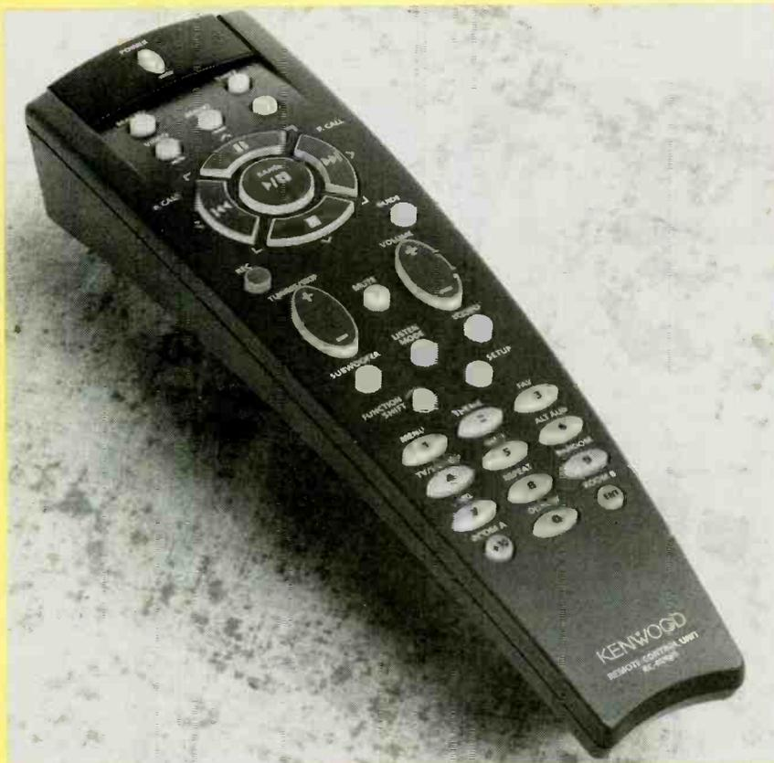
*The FutureSet remote control can be updated via phone to operate components you buy in the future. Macro capability lets you program a series of multi-component operations into one press of a button.*
