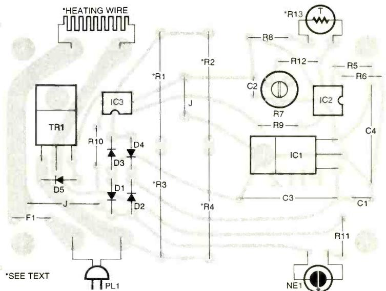
Fig. 5. Assemble the printed-circuit board according to this parts-placement diagram, saving the heating element for last. Connect the thermistor to the board via a pair of 6-8-inch lengths of insulated hookup wire and cover the solder joints at the thermistor with heat-shrink tubing or some glass tape.
