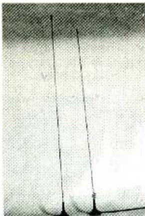
The MFJ-1721 and MFJ-1722 antennas both handle 50 watts on two meters, and their SWR is typically less than 1.5:1. The MFJ-1721 is nominally  $\frac{1}{4}$  wave on two meters and can be adjusted for any frequency to 500 MHz. Only the dual-band antenna, the MFJ-1722, covers the 440 MHz-range as well, with a power rating of 25 watts. It is a full  $\frac{1}{4}$  wave on 144 MHz.
