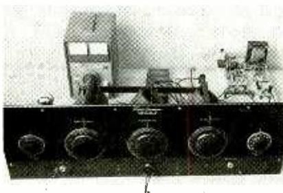
*The NR-5 laid out on my bench for its smoke test. At right rear is the breadboard-mounted "A," "B," and "C" supply. At left is the Eico battery-eliminator/charger temporarily pressed into service to supply bias.*
