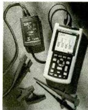
It is designed to be used with Fluke's range of ScopeMeter test tools, Combi-Scope instruments, and with analog oscilloscopes and accessories. When used with a battery-operated test instrument, a single DP120 provides dual-channel measurement on systems with two different ground potentials.
