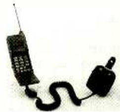
When the caller presses the red button for at least two seconds, the attached cellular phone automatically dials 911, opening a line to the agency that monitors cellular 911 calls. If an emergency occurs during a routine call in progress, pressing the red button immediately terminates that call and initiates a 911 call instead. The red button is well-illuminated for enhanced nighttime visibility.
