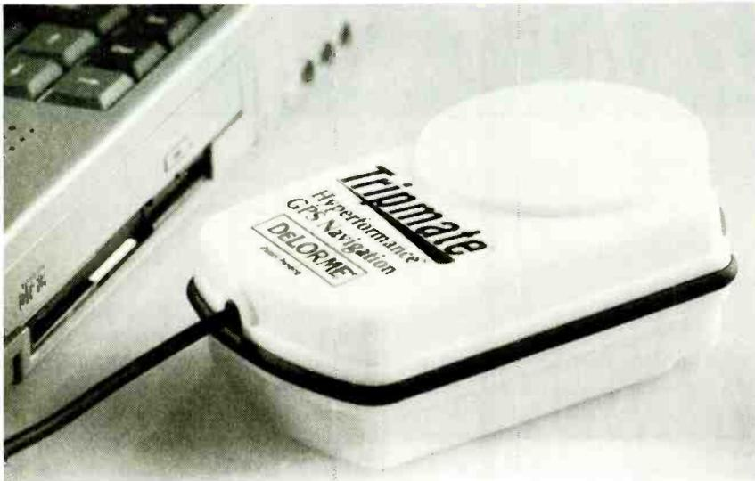
The DeLorme Tripmate Hyperformance GPS Navigation system offers capabilities similar to those of Etak's SkyMap through a 12-channel GPS receiver that plugs into the laptop's serial port via a six-foot cable. Its CD-ROM map database covers the entire North American continent and the Caribbean—and includes about 66,000 restaurants, hotels, and other points of interest.
