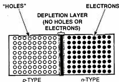
Fig. 1. A PN junction with no voltage applied.
