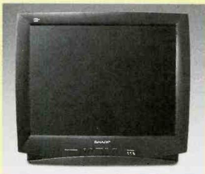
*Sharp's 36-inch DTV-ready analog set has 800 lines of resolution, and component video inputs for use with DVD players and DTV converters.*
