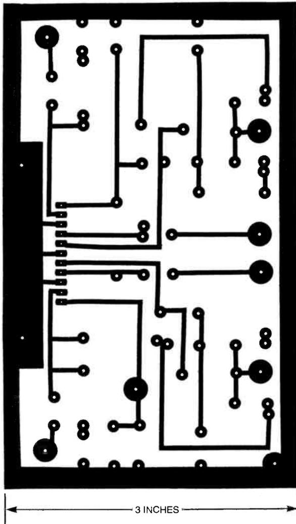
Fig. 3. The Portable CD Amp was assembled on a printed-circuit board, measuring 3 by  $5\frac{1}{16}$  inches. A template of the author's printed-circuit layout is shown here full-size.
