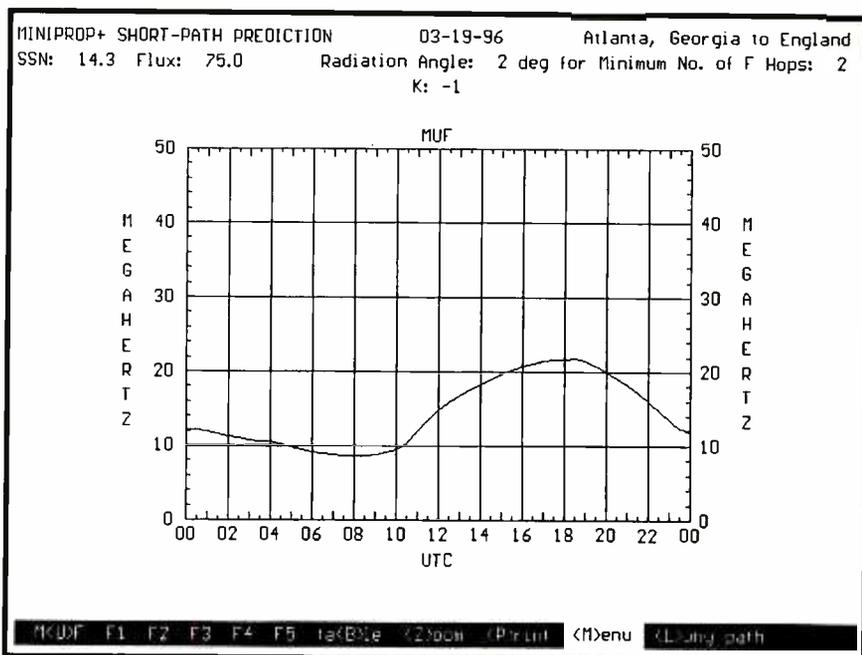
Fig. 6. MINIPROP PLUS 2.5 has significant graphical capabilities. Shown here a display of predicted MUF with a resolution of 30 minutes. The prompt line selections on the graph screen also allow you to view a graph of predicted signal levels or signal-to-noise ratio (SINR) on each prediction frequency.
