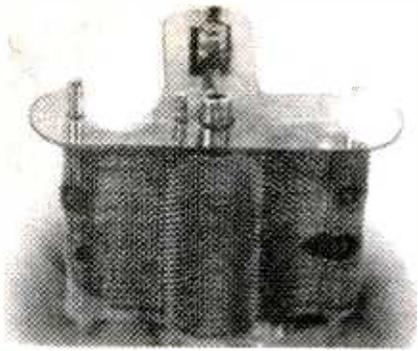
Close-up of type 27's innards. Top of cathode can be seen poking through plate-support structure.
