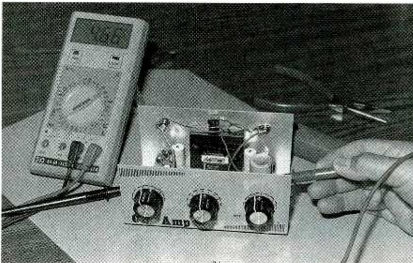
When taking resistance measurements, be sure to turn power to the Portable CD Amp off; failing to do so will damage the resistance measuring circuitry of the meter. When taking voltage measurements be sure that the meter is set to the DC scale and on a range that is higher than the anticipated voltage in the circuit.
