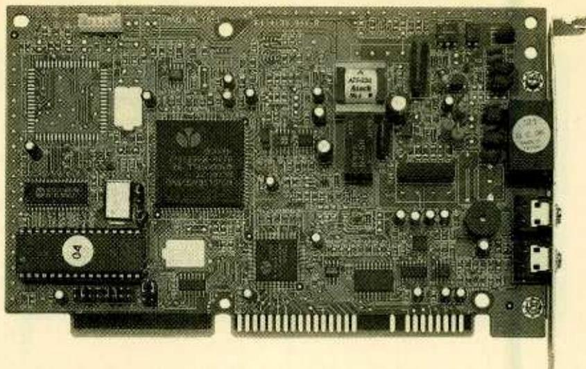
*The Amquest/KDS 56K modem is a fully compatible, hardware-controlled 56K modem, based on the legendary Rockwell Flex 56 technology. The modem features full duplex speakerphone, voice, data, Fax, SVD, Caller ID and V.80 video-conferencing capability.*
