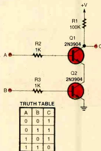
Fig. 4. Shown here is a variation of the circuit in Fig. 3, along with its truth table. By relocating the output (point C) of the circuit and the load resistor to the collector of the upper transistor (Q1), the circuit becomes a NAND gate. The same effect can be achieved by feeding the output of the AND circuit to an inverter.
