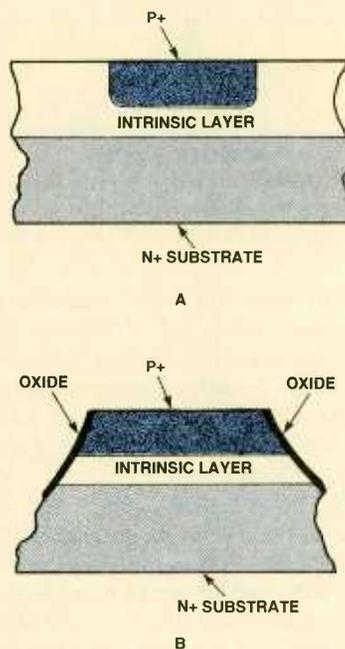
Fig. 1. There are two major structures for PIN diodes: the planar configuration shown in (A) and the mesa fabrication of (B).
