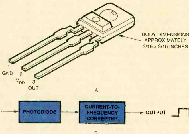
Fig. 1. The unusual TSL245 light-to-frequency integrated circuit is illustrated in A, while B shows a functional block diagram of the converter.
