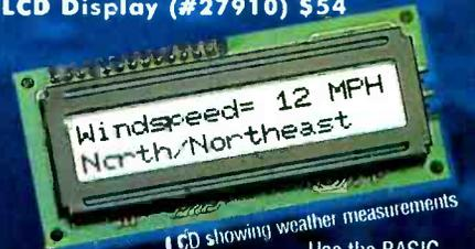
LCD showing weather measurements
