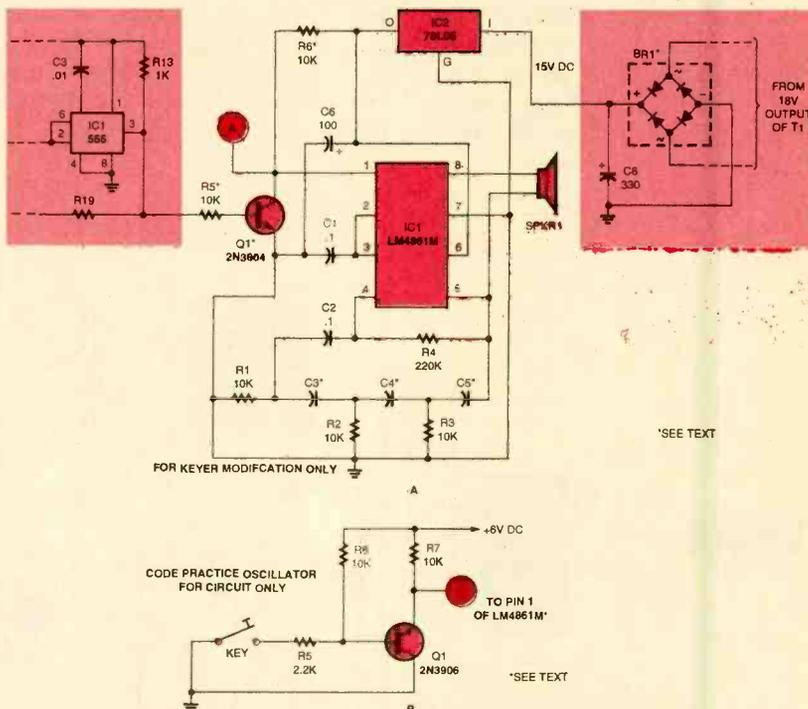
Fig. 5. These interesting circuits use the versatile LM4861M audio power amplifier IC. In (A) the IC is used in a modification to a previous *Popular Electronics* electronic keyer circuit (January 1998, "Think Tank", and shown shaded). This circuit results in better tonal qualities for the generated side-tone. In (B) the oscillator is now used in conjunction with the LM4861M IC and provides an independent code-practice oscillator, which can be used to upgrade your CW skills.
