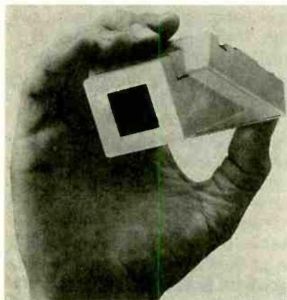
The camera provides over 425 lines of resolution and only .02 lux sensitivity. It comes standard with a built-in electronic shutter and a 4mm wide-angle lens. Other lenses are available as well: 2.5-, 6.5-, 8-, and 12-mm. There is also an optional audio capability.
