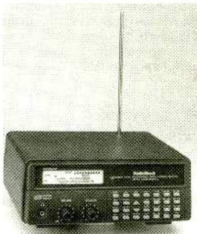
The triple-conversion circuitry of *RadioShack's PRO-2041* desktop (and mobile) scanner fights interference—a feature normally reserved for high-priced units.
