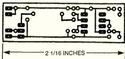
Fig. 2. The bulk of the Flight Timer's circuitry was assembled on a printed-circuit board, measuring  $2 \frac{1}{16} \times 7 \frac{7}{16}$  inches. A full-size template of the author's printed-circuit foil pattern is shown here.
