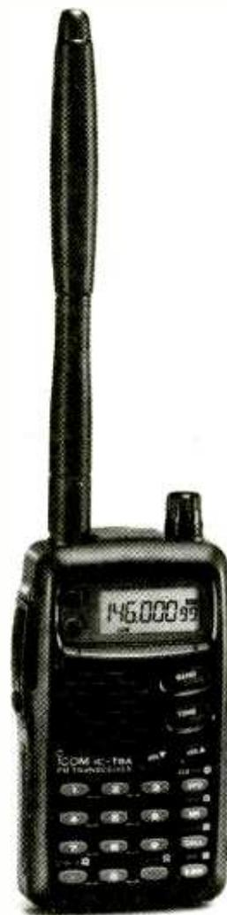
The T8A has a memory capacity of 123 channels, including 10 scan edges and 1 call channel per band. Simply pressing the BAND switch selects the active band. Arranged in 10 groups of 20 channels, the channels are easy to scan using a variety of scanning methods. Output power is 5 watts on all bands.
