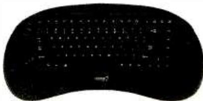
The *BeamerPlus* features an enhanced key layout including full-size cursor keys and large shift, enter, backspace, and spacebar keys. Full-size typing keys, embedded numeric key pad, inverted-T cursor arrows, separate insert and delete keys, and 12 function keys provide the full 104 key functions with only eighty-six keys, saving valuable space. The keyboard also provides a contaminant-resistant trackball and associated mouse-click buttons.
