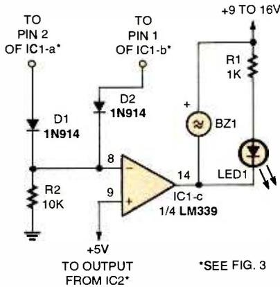
Fig. 4. Here's the same dual voltage monitoring circuit with a light and buzzer alarm added.
