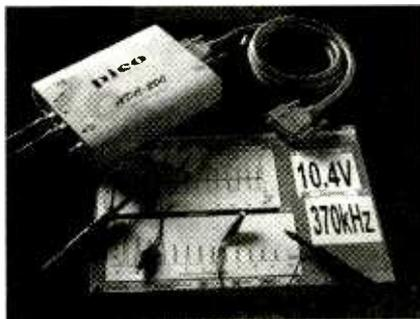
A feature of the ADC200-100 is simultaneous display of the oscilloscope, spectrum analyzer, and digital multimeter functions provided by the *PicoScope* software supplied with the instrument. In addition, the autoranging multimeter features simultaneous display of multiple parameters, such as true rms or DC voltage, dB gain, and frequency measurements.
