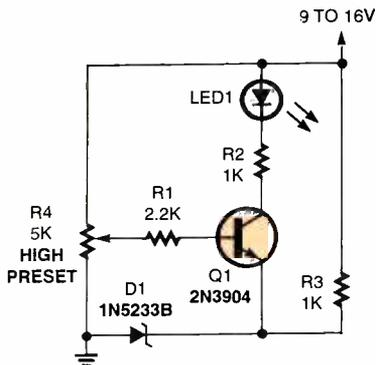
Fig. 6. Here's a simple over-voltage monitoring circuit, but designed with discrete components.
