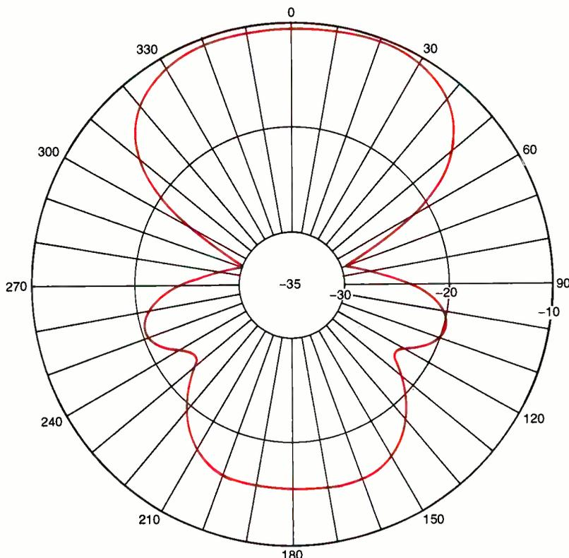
Fig. 5. Azimuthal antenna pattern at 25 MHz. Pattern appears in the shape of a "rag doll," with major and minor peaks and nulls.
