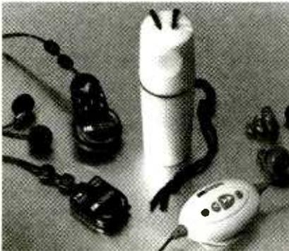
Smallest of the three is the Model 110, which weighs less than one ounce and measures just  $1\frac{3}{4} \times 1 \times \frac{3}{8}$  inches. Model 120 is slightly larger, with a built-in key ring, plus high-low volume control. It also weighs less than one ounce and is  $2\frac{3}{8} \times 1 \times \frac{1}{2}$  inches. Two 1.5 V batteries are included. Both models, which come in black or silver, are available with a waterproof carrying case.
