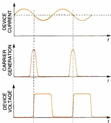
Fig. 3. Examples of IMPATT voltage and current waveforms.
