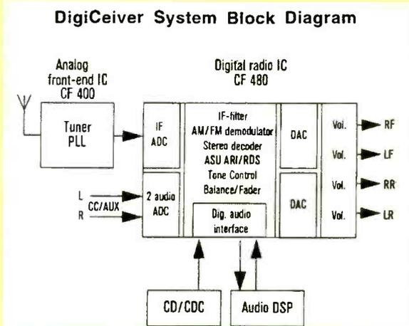
As a result of high-integration strategies, the complete functionality of a top-level car radio has been reduced to a two-chip set. The digital radio IC contains additional inputs for both analog and digital sources plus a communications interface for digital signal processing.
