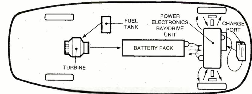
Fig. 1. The typical HEV has a small internal-combustion engine, motor/generator, and some form of energy-storage device—usually a battery, although a flywheel or ultra capacitor might be used. Only one power source, usually an electric motor, is used for propulsion in a series HEV system. The other source, typically an ICE, is used for battery charging and an additional source of power when needed such as for acceleration or high climbing. (General Motors)
