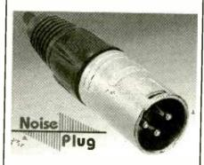
Inside is an ultra wideband, avalanche-junction white-noise source. The output of the source is frequency limited, amplified, and passed through a precision —3dB per-octave low-pass filter. The result is a full audio spectrum noise source with equal energy distribution in all octaves.
