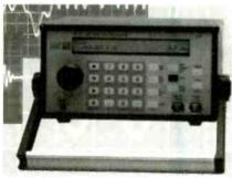
skipped points. It provides function, arbitrary waveform, and pulse-generation capabilities.
