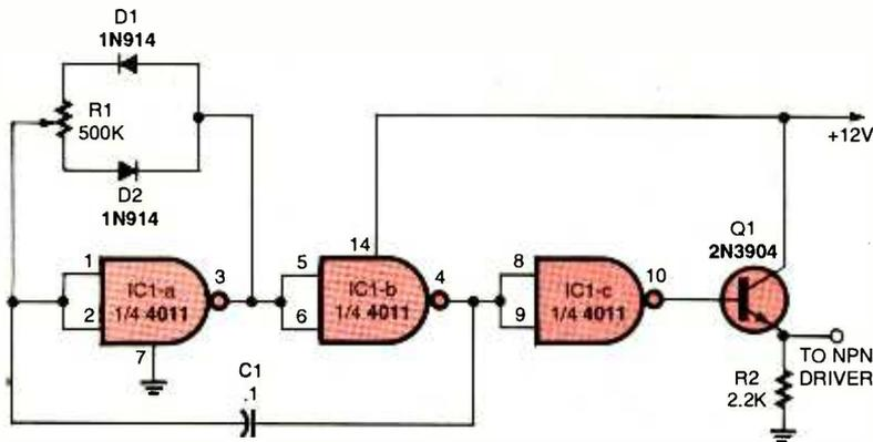
Fig. 2. The basic circuit illustrated in Fig. 1A can be modified—as illustrated here—so as to function with any of last month's NPN-input circuits. Note that this circuit and the previous one are identical except that a third gate has been added to the circuit and R2 has been switched from the collector lead of Q1 to its emitter terminal.
