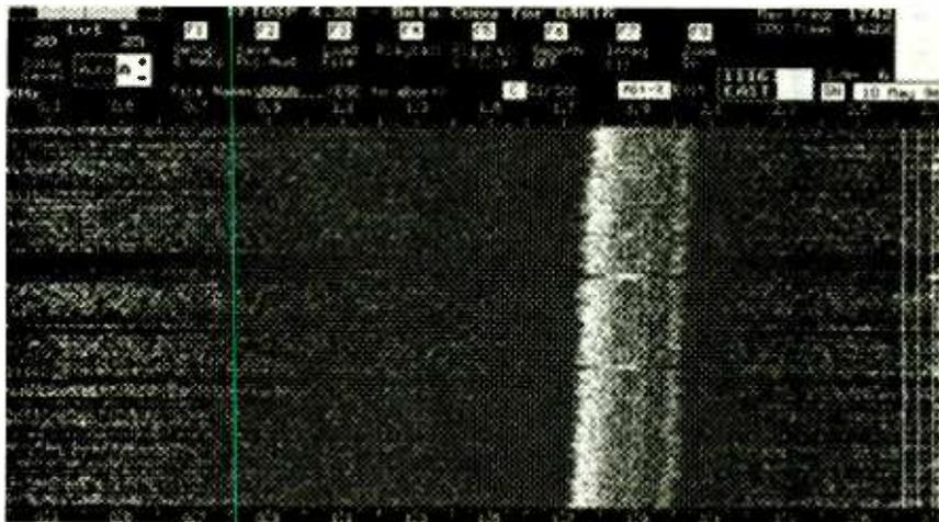
*To accomplish their objective—to reach farther and farther out into space in the hopes of contacting intelligent life forms—SETI stations use digital signal processing. Shown here is an example of the first candidate signal received by The SETI League in May of 1996, which turned out to be interference from a classified military satellite.*
