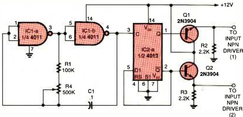
Fig. 3. The complementary outputs of this AC-driver circuit can be connected to the two inputs of any of the NPN-input voltage-reversal circuits.
