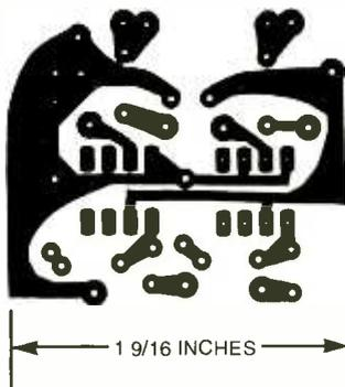
Fig. 4. The author's prototype of the circuit was assembled on a printed-circuit board, measuring 1 7/16 by 1 7/16 inches. A full-size template of the author's board is shown here.
