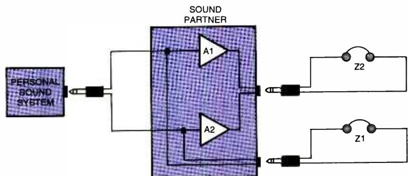
Fig. 2. The *Sound Partner* is configured such that audio from a personal sound system is fed to the headphones connected to J1 without modification, while the same two-channel audio is fed to a pair of amplifiers, which provide two-channel audio to a second set of headphones.
