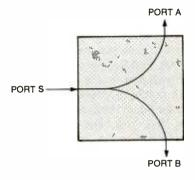
Fig. 1. Splitter/combiners are typically passive electronic networks that provide one common port and two or more independent ports. Shown here is a 3-port splitter/combiner.
