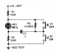
Fig. 4. Here a single neon lamp is pressed into 82 service to help form an on/off latching circuit.
