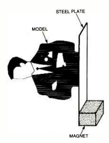
Fig. 12. Mounting the model for side illumination can be accomplished by glueing the model to a small steel plate and then placing it on its side using magnets.
