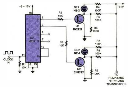
Fig. 9. The circuit in Fig. 7 can be expanded to drive a total of ten lamps by adding duplicate circuits to the remaining outputs of the 4017 and connecting the RESET terminal (pix 15) of IC1 to ground
