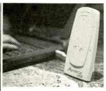
WebGear's Aviator lets your computer data take to the airwaves, allowing for wireless networking within a maximum 125-foot range. It comes in both USB and parallel-port versions.
