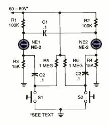
Fig. 5. This circuit configuration carries the concept outlined in Fig. 4 a step further by adding a second neon lamp along with additional support components to the circuit.
