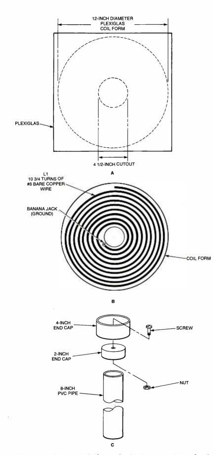
Fig. 5. The pancake coil—comprised of 10<sup>4</sup>/<sub>4</sub> turns of number 6 bare copper wire—was formed on 36 a '4-inch thick piece of Plexiglas material that was cut into a 12-inch diameter circle.
