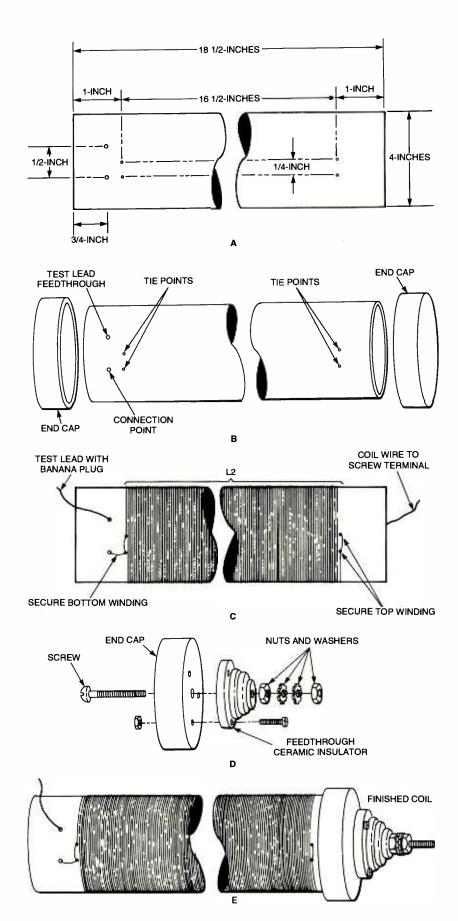
Fig. 6. The tower (or secondary) coil was wound on an 18<sup>1</sup>/2-inch length of PVC pipe. Shown here are fabrication details of the tower-coil assembly.
