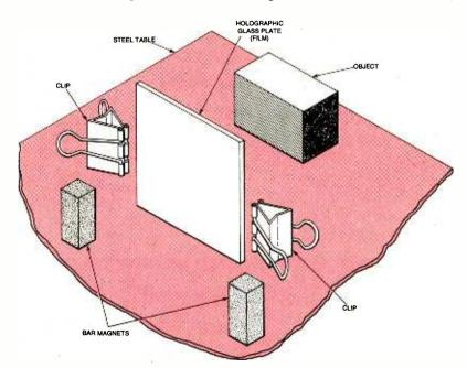
Fig. 7. A 2<sup>1</sup>/2-inch square glass plate, mounted directly on to the steel table with medium-size binding clips and bar magnets, serves as holographic film.
