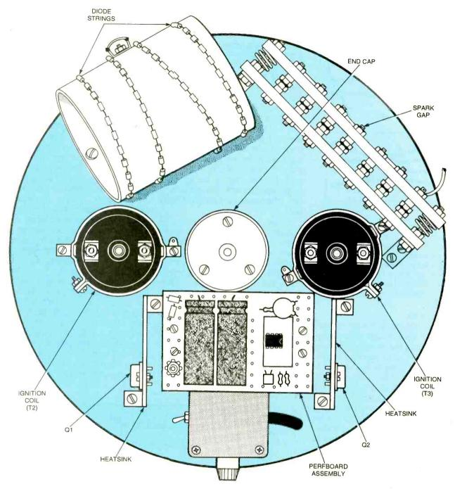
Fig. 4. The perfboard assembly was mounted suspended above T1 and supported by a pair of 23/4-× 1½-inch wood blocks that were on a 12-inch circular baseboard, as illustrated here.
