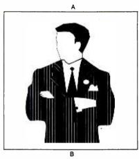
Fig. 11. To correct the problem outlined in Fig. 10, place the model on its side, with the top portion of the model pointed toward the "A" side of the plate, as shown here, to orientate the holographic image right-side up when viewing with a vertical light source.
