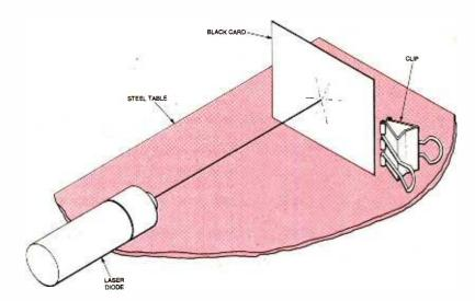
Fig. 8. A shutter card was made from a piece of black, non-glossy cardboard, measuring approximately  $2^{1}/2 \times 2$  inches, and a medium binding clip was attached to make the card freestanding. No magnets were used on the shutter-card binding clip, because doing so would make it more difficult to lift the shutter card without creating unnecessary vibrations.
