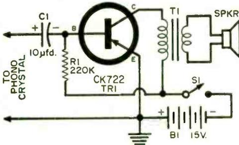
**Note** the simplicity of the phonograph amplifier circuit. The tap on the secondary of the output transformer should be selected for highest volume.
