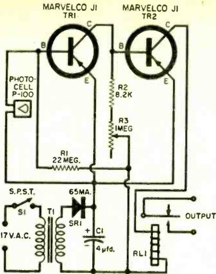
**Schematic** and parts list for the photo-relay.
