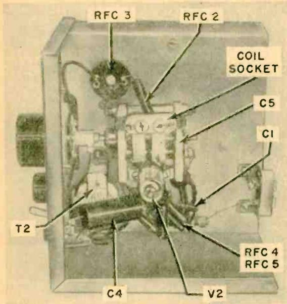
Exterior view of the receiver (at right) shows cutout in the right side through which the various coils are inserted into the coil socket to obtain the desired frequency band. In this photo, the coil for the 28-50 mc. band has been inserted; coils for the other two bands are also shown.
