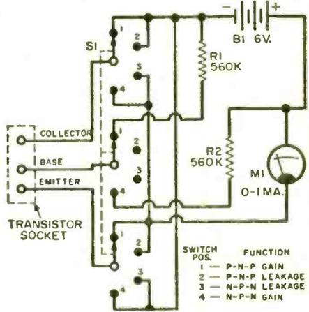
To check the common-emitter current gain, merely set the switch to the gain position. An upward swing indicates a current gain. If the leakage reading was very low, the meter reading, multiplied by 100, can be called the approximate beta ( $\beta$ ) for the transistor. At any rate, the meter reading can be checked against Table 1.
