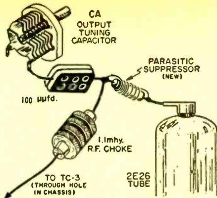
Fixed capacitor and r.f. choke formerly connected to pin #3 (plate) of the 6L6-G tube socket are moved above the chassis for connection to plate cap of the 2E26. Pictorial is shown at left.
