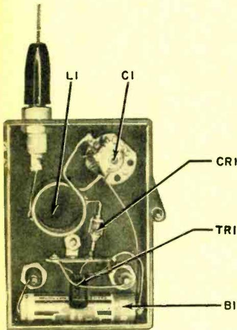
tinned wire and mount it across the terminals of C1. The coil is tapped one-half turn up from the end attached to the rotor of C1. Connect this tap to the antenna jack by a short length of wire. The rotor of C1 is connected to the emitter of TR1 by another length of short wire.
