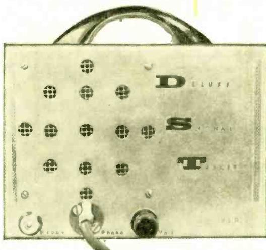
**W**ith the possible exception of a volt-ohm-milliammeter, signal tracers are perhaps the most useful test instruments in the home workshop. However, a.c.-operated signal tracers have always been handicapped by their sensitivity to 60-cycle pick-up. And battery-powered models, using vacuum tubes, have the disadvantages of high-battery drain, tube fragility and low audio output.
