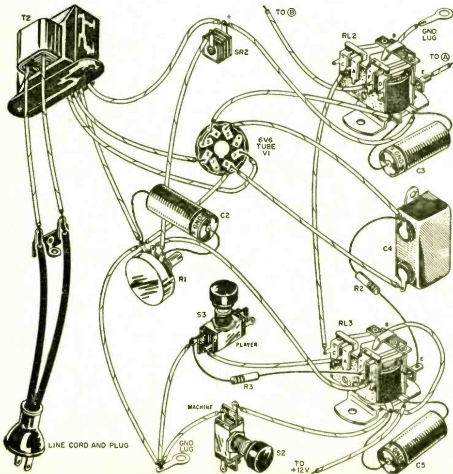
Pictorial wiring diagram for auto-response panel.
