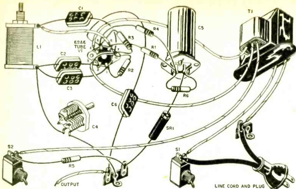
Follow the pictorial and schematic diagrams in building the dial setter. Note that C5 is grounded through its metal mounting plate.
