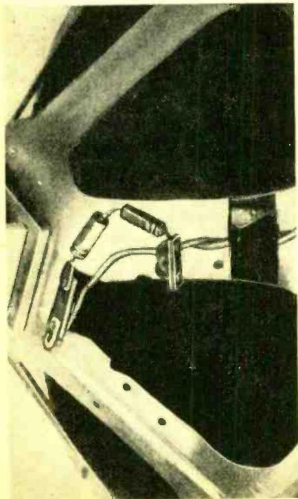
. . . using a series capacitor on woofer frame.
