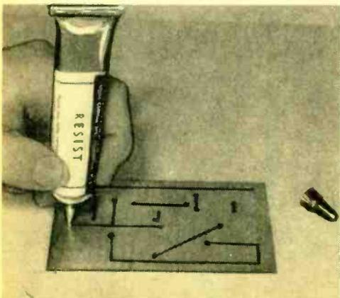
Using a ball-point ink tube to draw the circuit.
