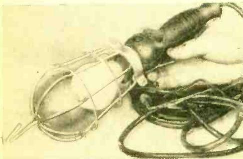
Drop lights with extension cords should be well insulated with a shade and heavy wire screen protecting the bulb (left). Some of these drop lamps will have a built-in switch, a handy item if the light is to be used regularly.
