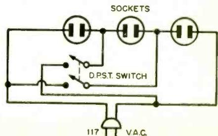
Schematic of dimmer control for photofloods.
