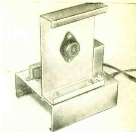
**Above** are two views showing the mounting details for the heat sink for the 2N255, the power transistor. Four flat fiber washers should insulate the chassis for the heat sink from the amplifier chassis.
