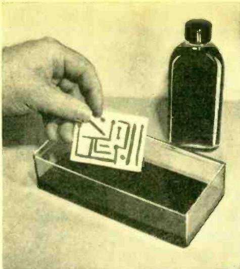
Placing prepared circuit board in the etchant.
