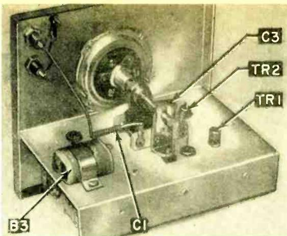
Top and bottom views of the "two-lunger." *C1* is a "gimmick" capacitor which allows a wide range of frequencies to be received. Aluminum brackets hold *T1* and *B3* in place.
