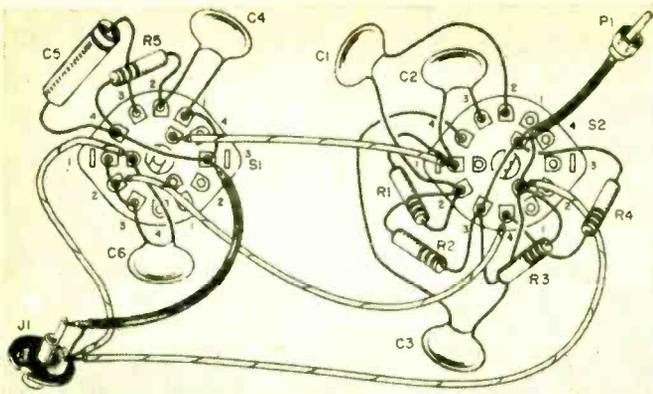
**Wiring layout** for the equalizer should closely follow the pictorial diagram at left. Switches S1 and S2 are viewed from rear. The schematic diagram below shows how S1 controls the bass turnover frequency while S2 regulates treble roll-off.
