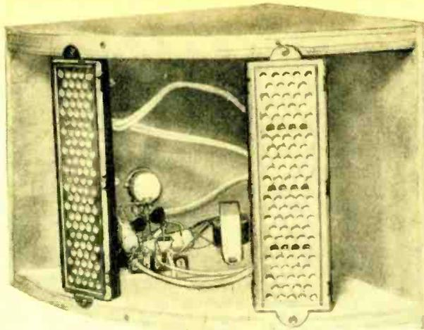
Completed electrostatic tweeter system. Tweeter elements should be positioned for best high frequency dispersion.
