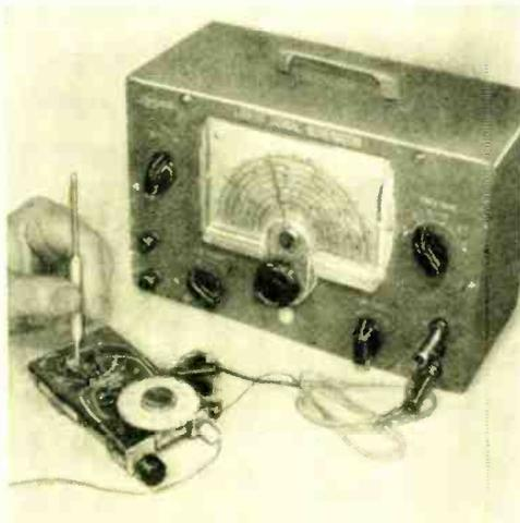
To align the superhet, you'll need a signal generator and an insulated alignment tool.
