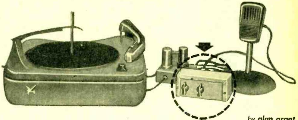
*tubeless circuit permits mixing and equalizing signals from phono pickups and microphones*
