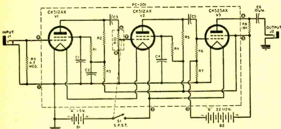
Fig. 1. Schematic diagram of complete amplifier assembly. Portion of circuit within dashed line (except *R10*) is part of printed circuit plate PC-201. See parts list.
