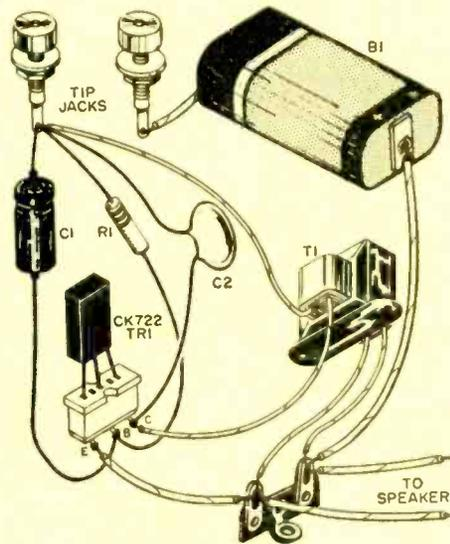
**Layout** of parts is not critical, but if you want to color the plastic case, don't mount the parts until after the paint has dried. Check all wiring before connecting the hand key or trying the unit.
