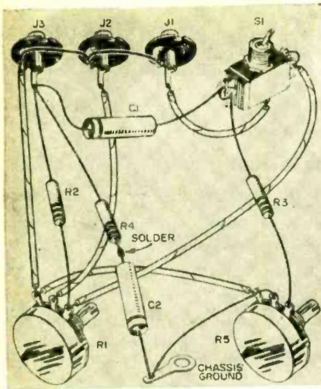
**Schematic and pictorial for building the mixer-equalizer.** Parts list is given below. If bass is too prominent for good voice intelligibility on microphone input, a small capacitor (on the order of 0.001  $\mu\text{fd}$ .) should be inserted at point ②.
