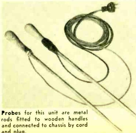
Probes for this unit are metal rods fitted to wooden handles and connected to chassis by cord and plug.
