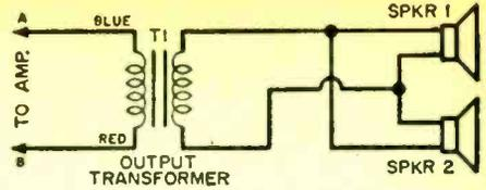
Hookup of 4" or 5" PM speakers may be made either in parallel as shown or in series (see text). Check for proper phasing by reversing the voice coil connections to one of the speakers; then note effect upon bass reproduction and connect for best results. T1 is a 50L6 output transformer. Complete phono amplifier circuit is on page 148.
