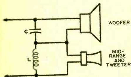
Fig. 2. Elementary crossover circuit for a system using a single woofer and a single tweeter. The inductive component, or coil, may be made at home (see text) from inexpensive materials that you will find at your local hardware store.
