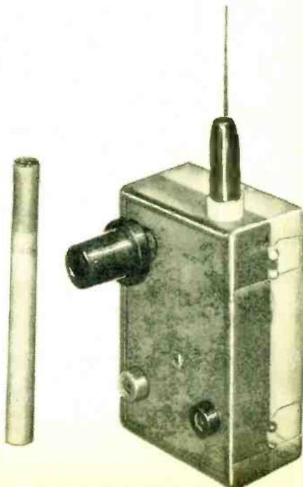
**Simplicity of construction** is shown in photo and schematic diagram of receiver. Headphones can be plugged directly into output of single transistor, but greater volume results if transistor TR2 is added and J2/J3 repositioned in circuit.
