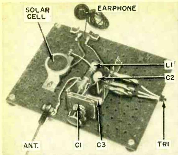
The broadcast receiver is shown above, made up in breadboard fashion to simplify construction and experimental changes in parts value or circuit arrangement. Perforated Masonite makes an excellent breadboard chassis, and you don't have to worry about layout and machine work as you would on metal.
