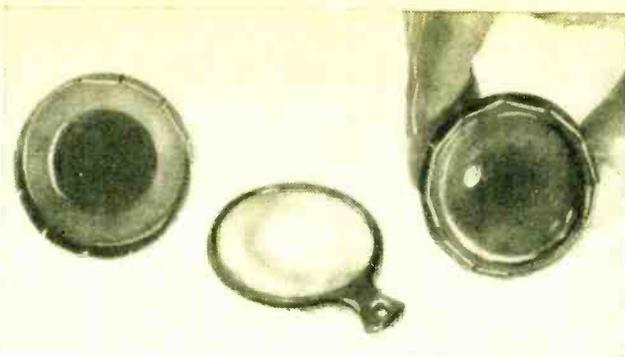
**Assembly of the infrared optical system.** The frame of the lens (center) is snipped off with diagonal pliers, and the lens set into the flange of the infrared filter holder (left). A piece of spaghetti tubing, about  $\frac{1}{8}$ " in diameter, is fitted around the edge of the lens, and the serrations of the flange are then bent inward to hold the lens in place (right).
