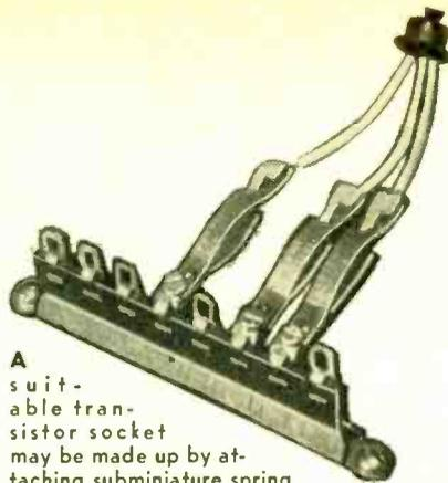
A suitable transistor socket may be made up by attaching subminiature spring clips to a tie-point strip. Use a 7- or 8-terminal strip; you'll find the extra terminals handy for other components.
