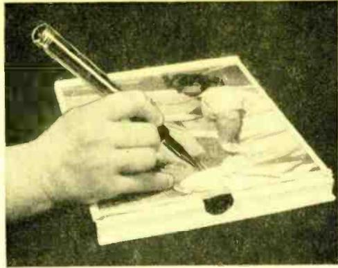
With an inexpensive electric pencil you can make your signature a part of your photographs. You can also use it for simple retouching jobs. Approximate assembly details are shown in the cross-sectional sketch. The model in the photograph was made up from a "radiator inspection light" picked up at a local auto supply store: this is essentially a standard penlight equipped with a curved Lucite rod to conduct light "around corners."
