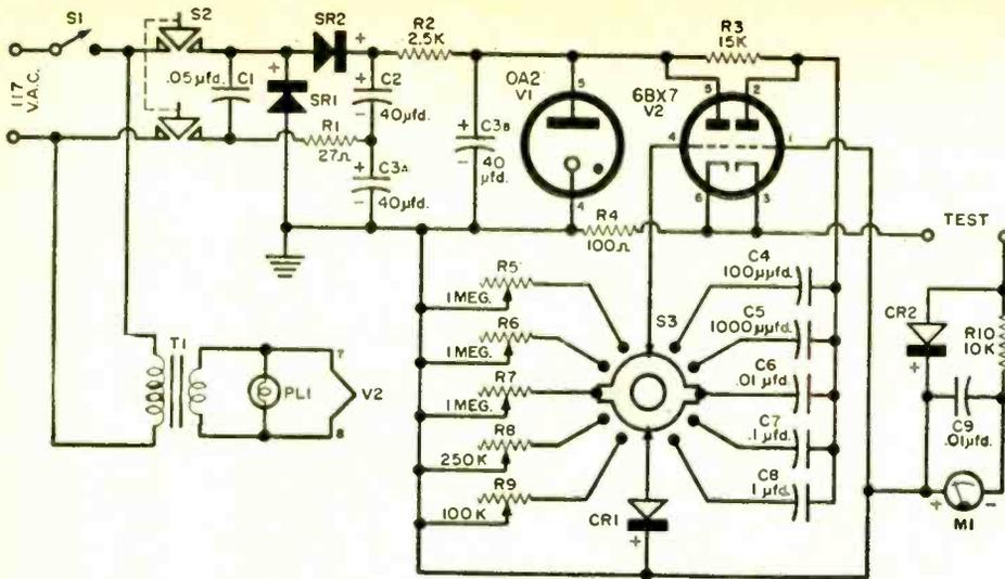
Schematic and parts list for the "Capaci-Meter".
