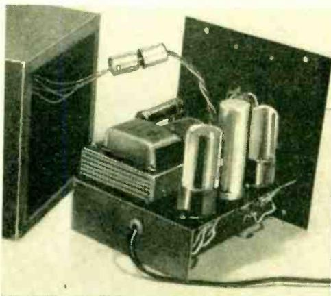
Components are mounted as shown here. Miniature cable connectors which join the four leads that go to strobotron socket on top of case make it simple to remove chassis for inspection or repairs.
