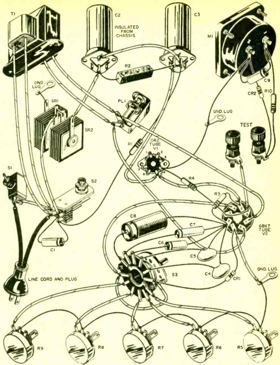
Pictorial of the "Capaci-Meter." Schematic and parts list are on page 52.
