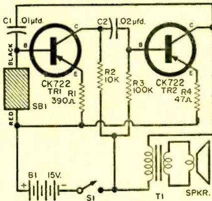
You can use a similar scheme, or provide separate transistor sockets. Make the connections to the battery by soldering leads directly to its terminals. Avoid overheating the battery.
