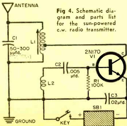
Fig 4. Schematic diagram and parts list for the sun-powered c.w. radio transmitter.
