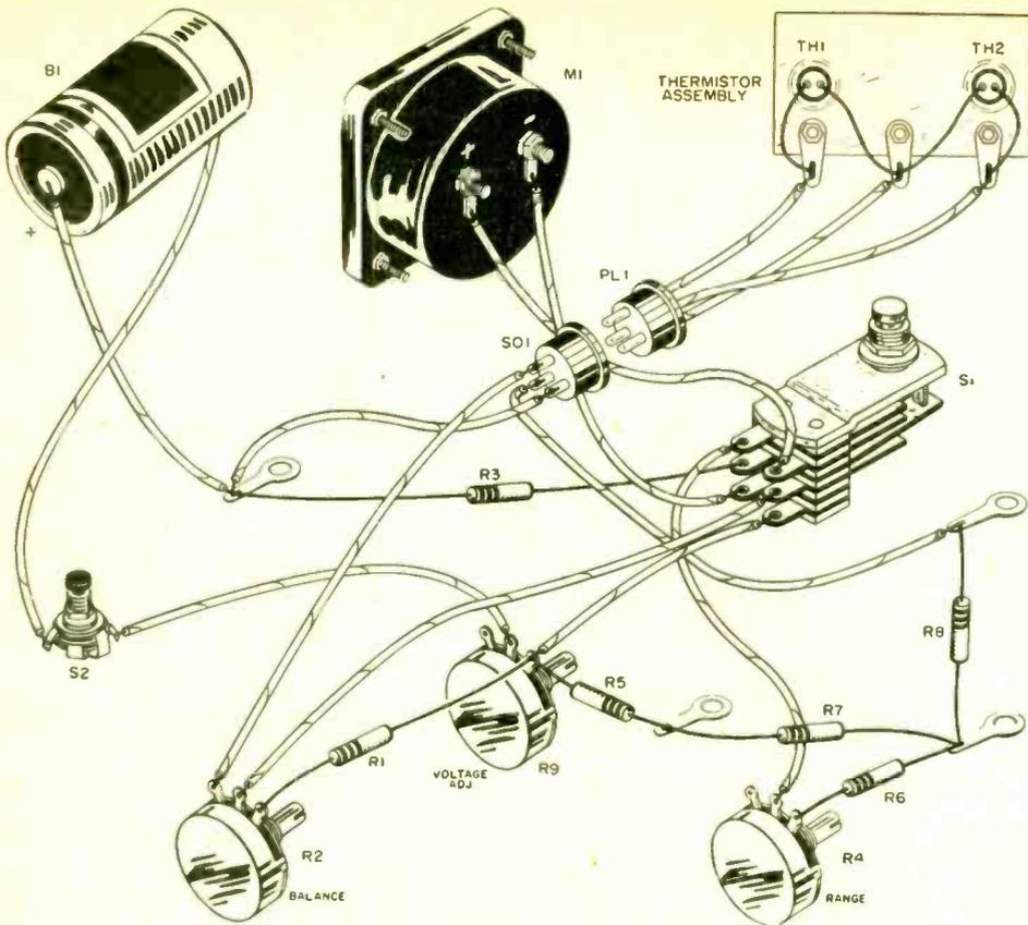
Pictorial wiring diagram of the anemometer.
