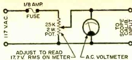
Setup for calibrating the calibrator.
