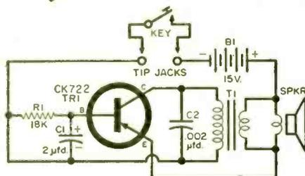
Simple single transistor circuit provides enough output to drive loudspeaker. Entire circuit can be mounted in small plastic box.
