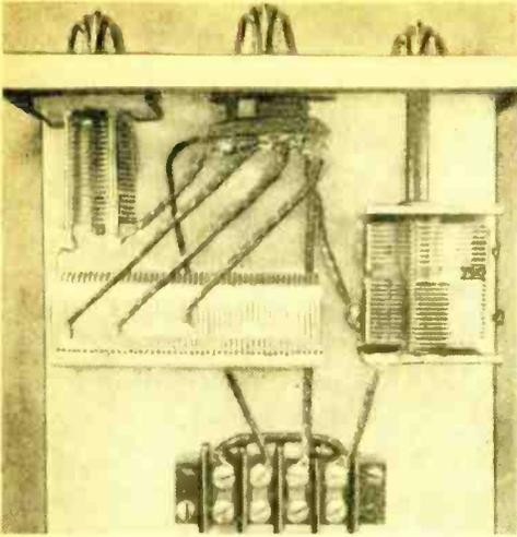
**Top** of unit shows placement of capacitors. Follow the schematic shown below for proper wiring.
