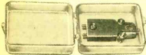
**Vibration pickup** or "transducer" assembly consists of phono cartridge mounted in plastic case.
