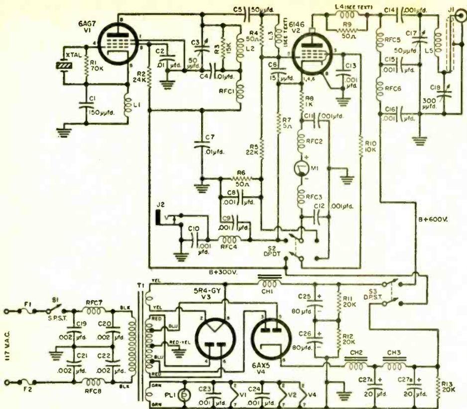
the 6146 beam tetrode (V2) using components  $R_4$ ,  $L_3$  and  $R_9$ ,  $L_4$ .
