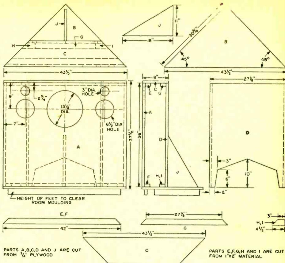
**Construction** plans for building the "Hi-Five." The entire cabinet can be built from a single 4' x 8' sheet of plywood. The home builder will find this project is economical and requires no power tools.
