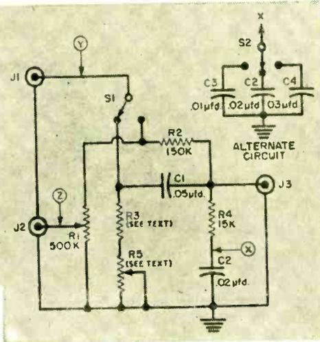
boost. A 0.03- $\mu\text{fd}$ . capacitor will provide essentially flat response, while an 0.01- $\mu\text{fd}$ . unit will increase the bass. If you don't want to bother with the switch, simply experiment with different values until you find one that is pleasing to your ear.
