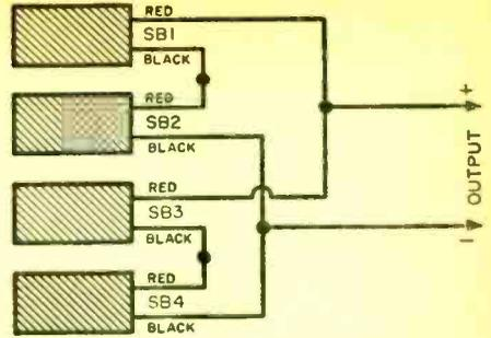
**Fig. 1.** Four-cell battery with series-parallel connection. The upper pair and lower pair are each connected in series and then in parallel. Color coding shown applies to B2M selenium cells.
