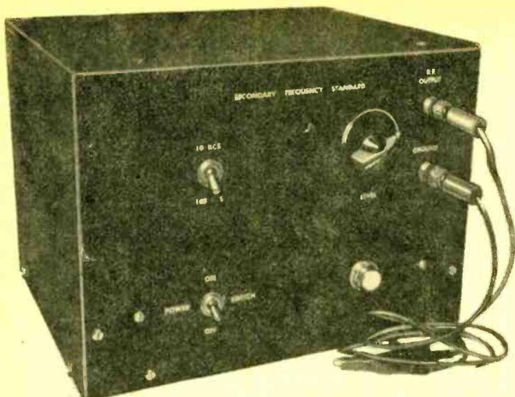
Front panel view of the spot frequency injector (left) which is designed around two printed-circuit kits. Below are the printed-circuit boards shown with all small parts mounted.
