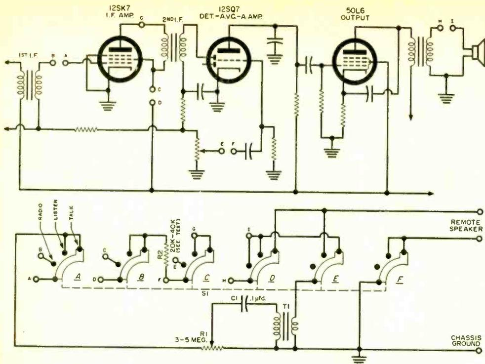
The partial schematic above is of a common type of a.c./d.c. home receiver. The lettered terminals on switch shown beneath it should be connected to similarly lettered points in receiver.
