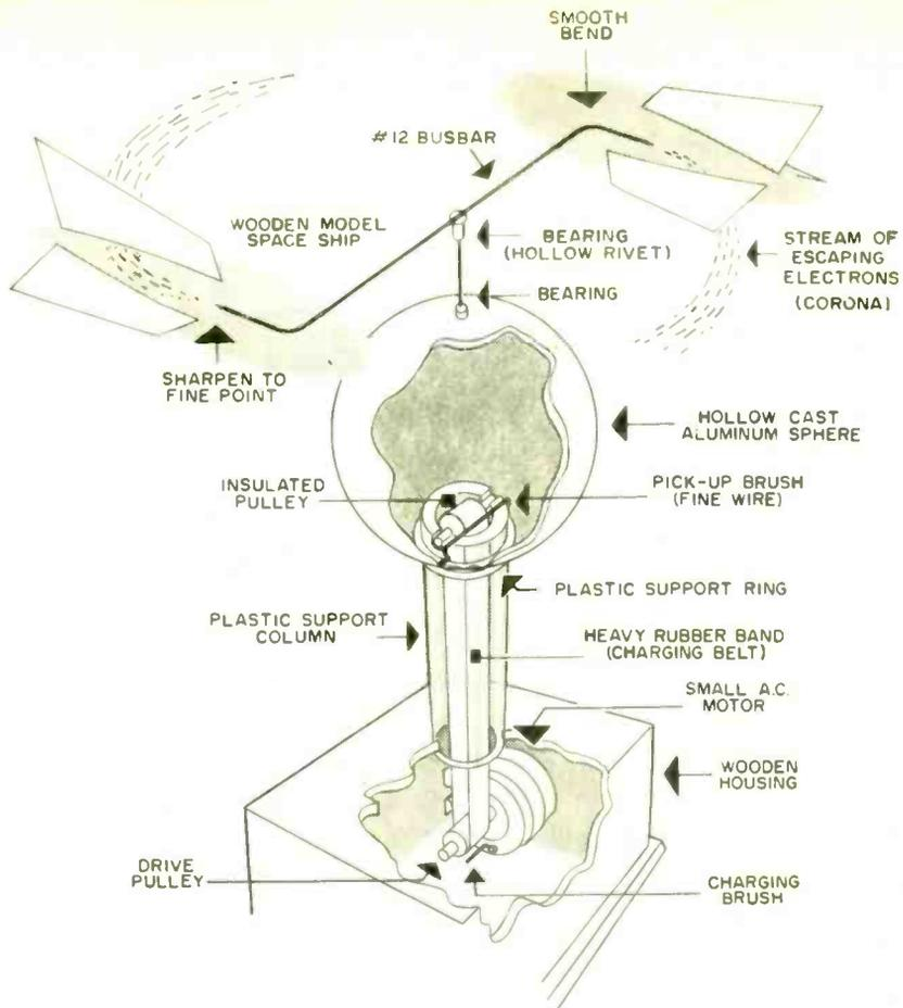
**Exploded view** of model spaceship showing construction details.
