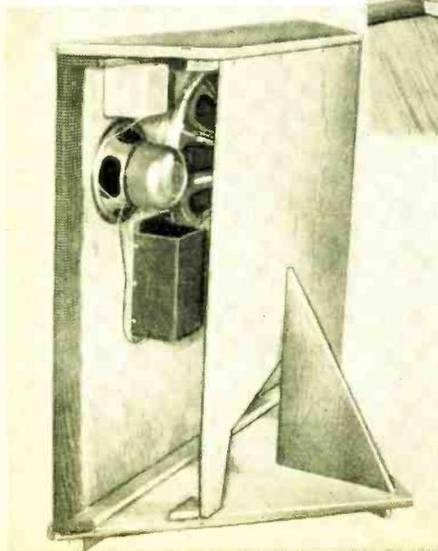
The baffle is shown above without grille to illustrate location of the five speakers. Side view shows construction details; note that the crossover network is mounted where it interferes least with the cross-sectional area of the labyrinth. See the illustration on the opposite page for details on providing acoustical isolation for the tweeter.
