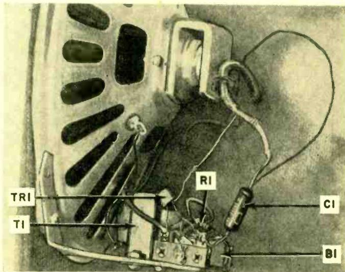
No volume control is included or necessary in the amplifier shown here. The transistor used may be a CK722, 2N107 or equivalent. The shielded phono lead connected to CI has its shield grounded to the speaker frame.
