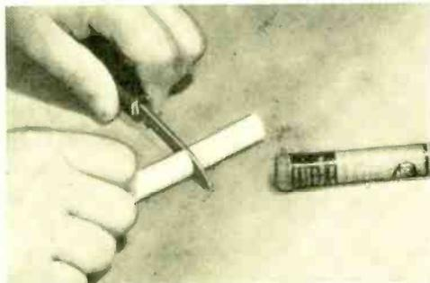
**Operating power** for the simple receiver is supplied by an 11.2-volt battery, made up by cutting an eight-cell section from an RCA Type VSO87 "separable cell" battery. You can easily cut out the desired section with an ordinary pocket knife.
