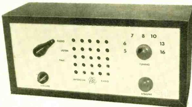
Photo at right shows a.c.-d.c. radio set converted for use as radio-intercom unit.
