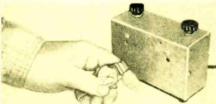
Above illustration shows the dark-room timer being calibrated with a watch. A clock with a sweep second hand may also be used for calibration. At the right, the timer is being used with a contact printer.
