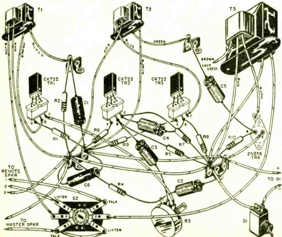
Pictorial and schematic diagrams of the transistorized intercom.
