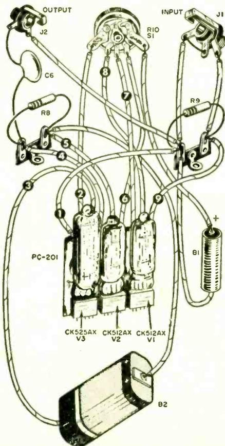
**Pictorial** diagram shows how printed-circuit is hooked up to other components.
