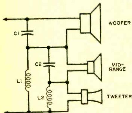
Fig. 3. Three-way system involves the use of a more complex crossover network. Twice the number of components required for a two-way network are necessary when designing three-way network.
