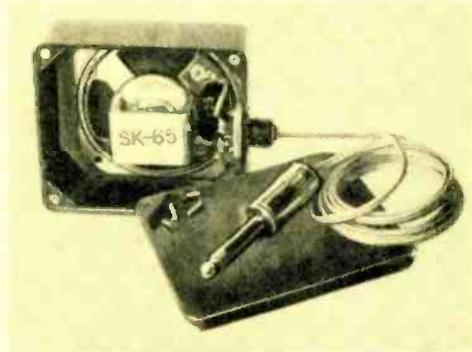
mits the speaker to be plugged into a closed-circuit jack installed on the radio. (Mount the jack on the radio cabinet or back panel, making sure that it is insulated from the radio's chassis.) The jack is wired into the voice-coil circuit in a manner that mutes the radio's speaker when you plug in the pillow speaker.
