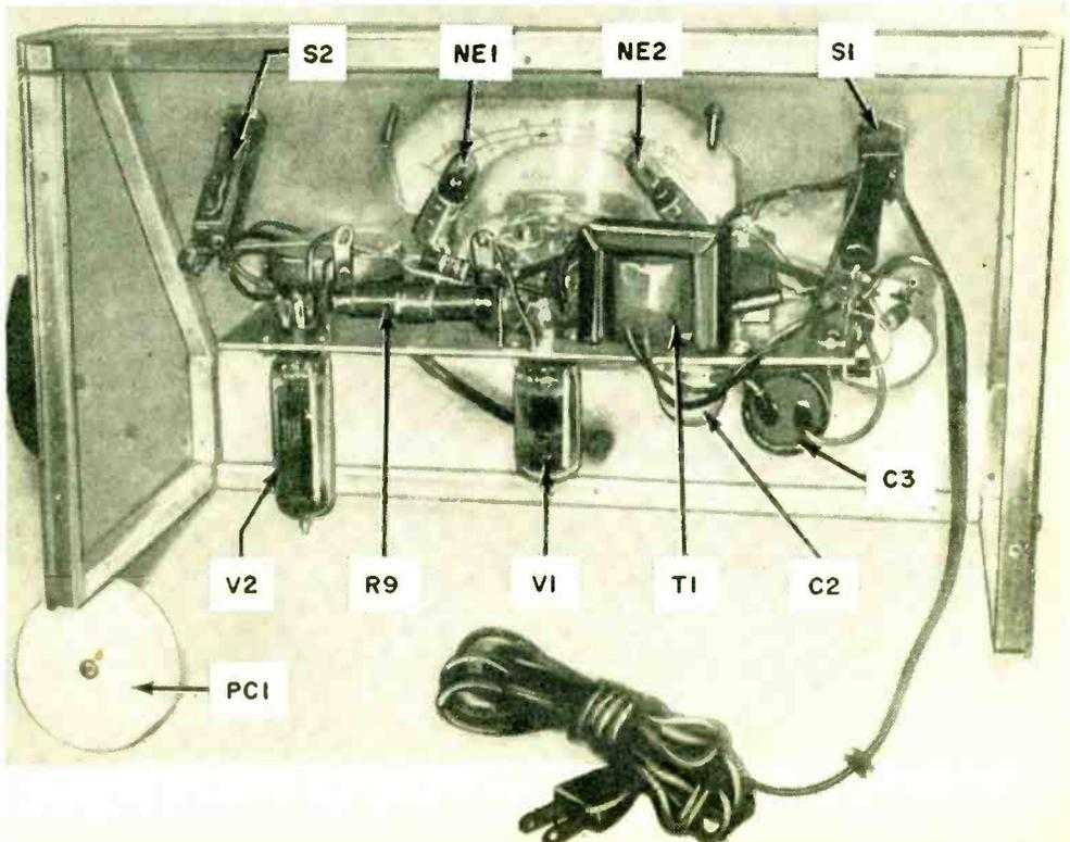
enlarger. Also, the resistance of the cell varies significantly and proportionately with light intensity at the low levels with which we are concerned.
