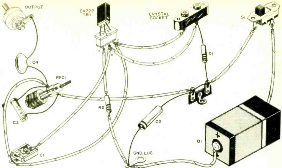
Follow these diagrams when you build the crystal calibrator. Parts list is given below.
