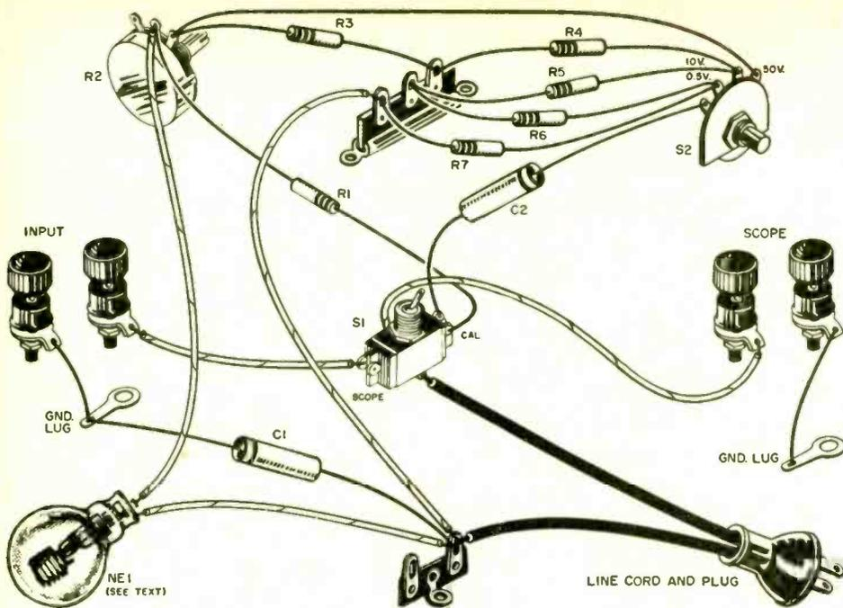
Follow the pictorial and schematic diagrams in putting the oscilloscope calibrator together. The parts list and a description of how the unit operates are given below.
