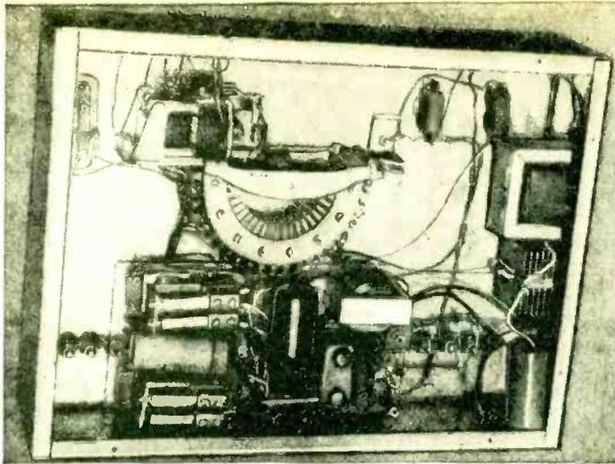
Underside of "Challenger" game with auto-response circuit in place. All wiring on subchassis is completed before unit is installed in cabinet.
