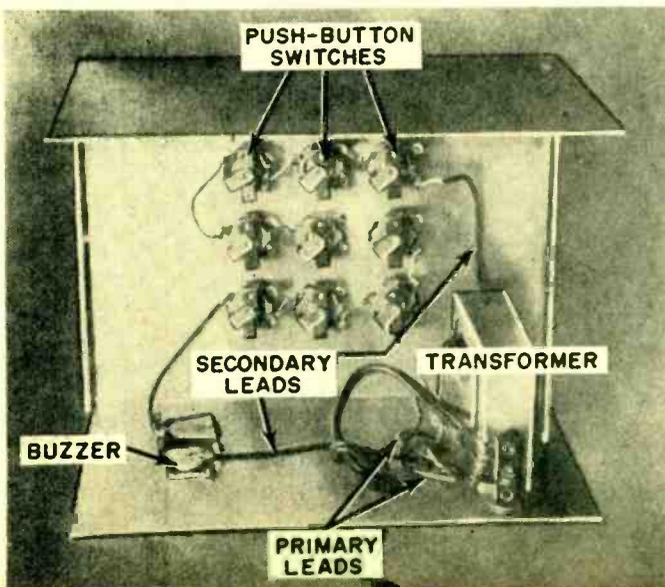
Metal cabinet, doorbell transformer and buzzer, a two-terminal tie-point strip, nine push-button switches, power cord and hookup wire make up the simple parts list for the intelligence tester. Push buttons with s.p.d.t. contacts are employed, and connection is made to normally closed contacts of all switches except the three that will be used to ring the buzzer.
