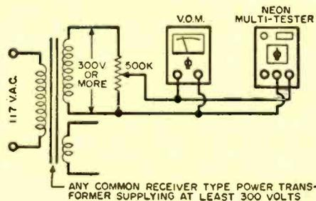
Voltage calibrating setup for the multitester.
