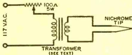
Schematic above shows how easy it is to build the burning tool. In the photo at top of page, you will note how the Nichrome tip is attached to the ends of the test prods. If you wish, you can remove the prod points, since they may tend to obstruct your work. Cement holds the prods in place.
