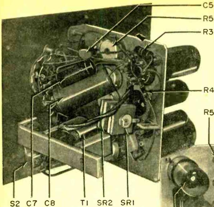
Suggested layout of the "Capaci-Meter" components is shown below and at left. Physical modifications may be made without altering its accuracy.
