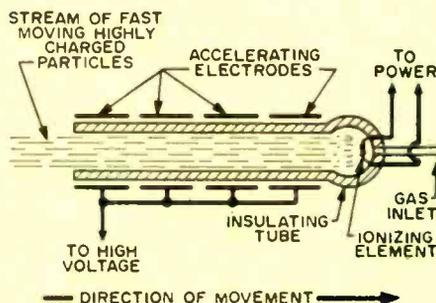
ment. These particles then are accelerated in a steady stream by a series of electrodes carrying high voltages—much in the same manner that the electron beam in a TV cathode-ray tube is accelerated forward to strike the fluorescent screen.
