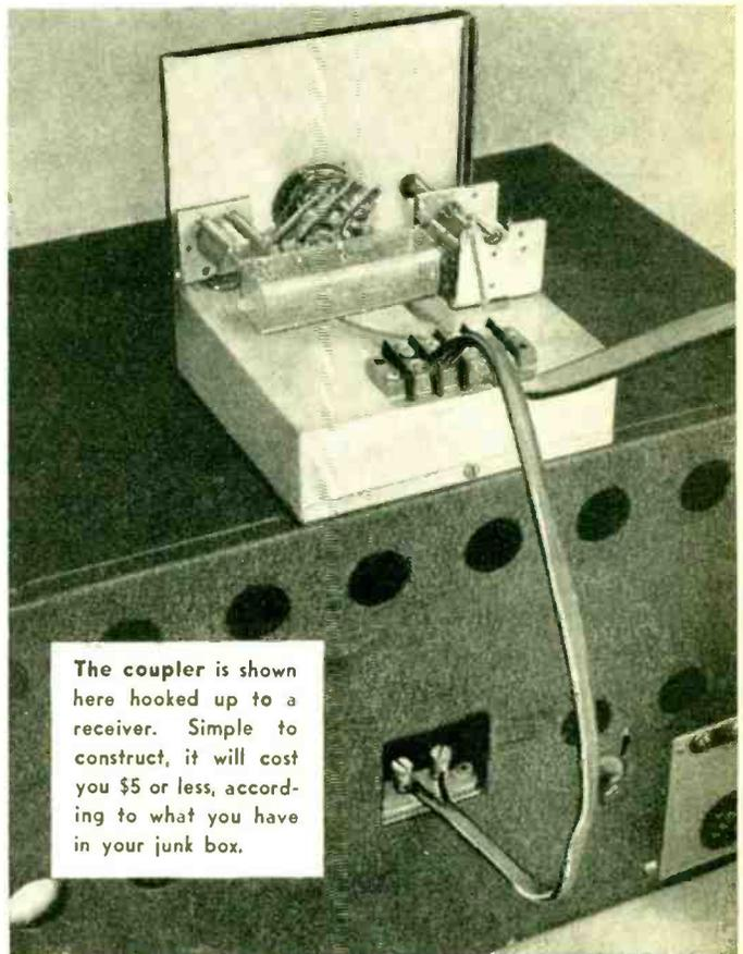
The coupler is shown here hooked up to a receiver. Simple to construct, it will cost you \$5 or less, according to what you have in your junk box.
