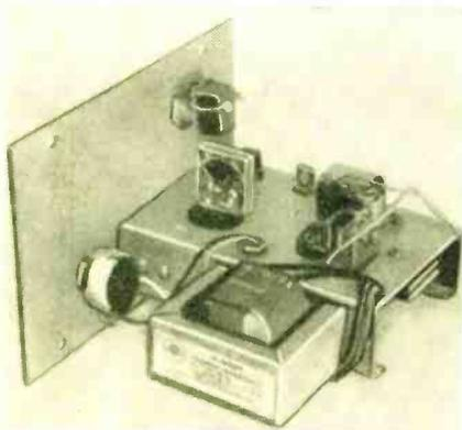
The above view of the photo-relay shows the transformer mounting clearly and the relative positions of *R3*, s.p.s.t. switch *S1*, and the Sigma relay, *RL1*. You can also see the front of the solar cell (P-100) which is plugged into holes #4 and #6 of the octal socket.
