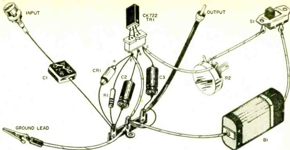
Hook up the "bargain basement" signal tracer's components as shown in the pictorial diagram above; schematic and complete parts list for this simple test unit are given below and at right.
