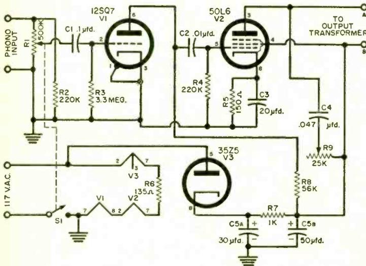
**Phono amplifier circuit, above and at left, may be modified to suit constructor. R2 can be varied from 68,000 ohms up to the figure shown here. Changing the value may improve the tone of some cartridges.**
