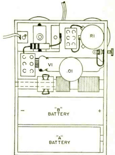
Parts layout above shows how components can fit into very small case. Compare this diagram with the pictorial at bottom of page.
