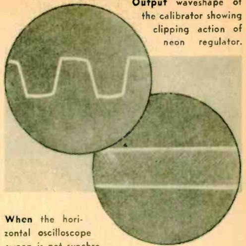
**When the horizontal oscilloscope sweep is not synchronized with the calibrator, a waveform like the one at the right is obtained. This is easier to use in calibrating the calibrator.**
