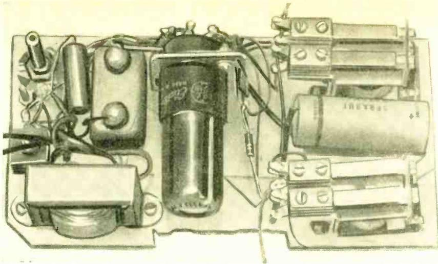
Recommended placement of parts in auto-response panel.
