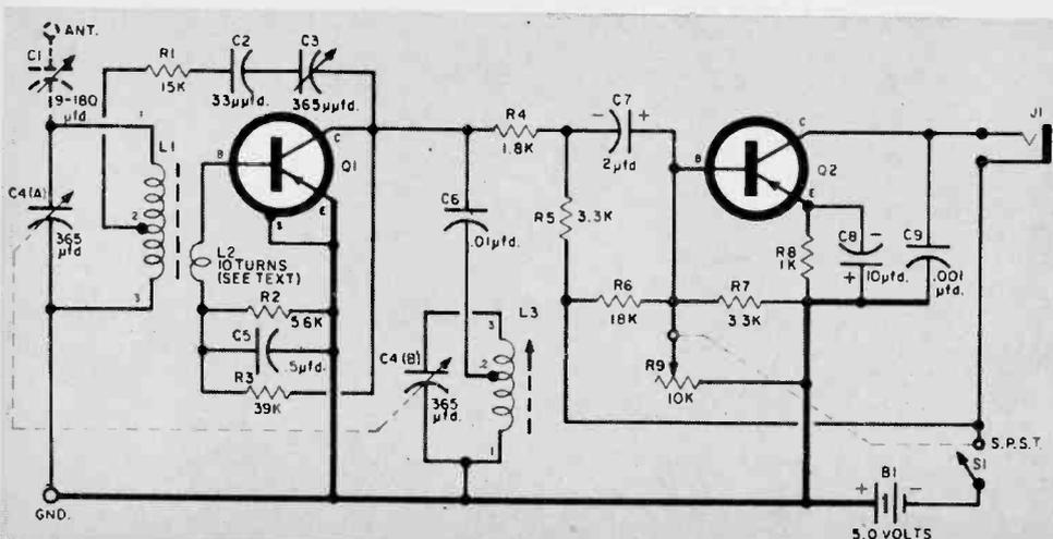
**Major parts placement** is shown in bottom and rear views of chassis. Phone jack J1 should be insulated if metal chassis is used. Note use of two-gang tuning capacitor (C4) and one-gang regeneration control (C3).
