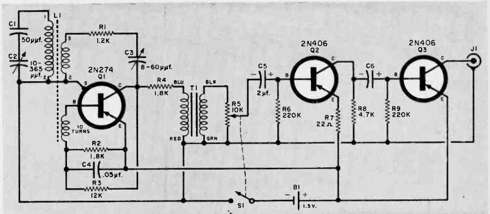
type phono jack, but it could be one of the miniature phone jacks. A thin strip of plastic is mounted on the solder lug of *J1* for use as a tie strip for the audio amplifier section.
