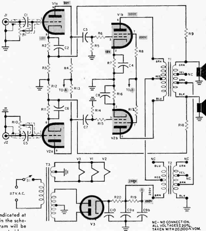
Voltages indicated at V1's socket in the schematic diagram will be close but not identical to those of V2.
