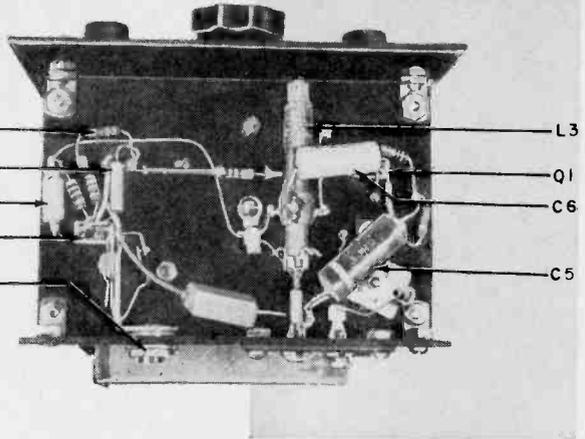
use the largest antenna that your chassis will accommodate (4" or more) and mount it as far away from any metal as possible. An external antenna and ground can be hooked up for peak performance.
