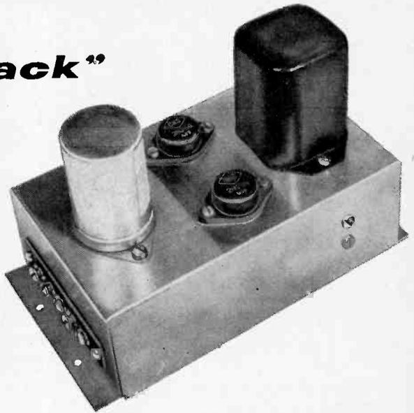
Here is an easy-to-build two-transistor power supply that will deliver a whopping 250 volts d.c. at 125 ma. from any 12-volt automobile battery. Although this project was specifically designed to provide power for a modulator six-meter station, it can be used wherever high voltage d.c. is required and where there is only a storage battery available.
