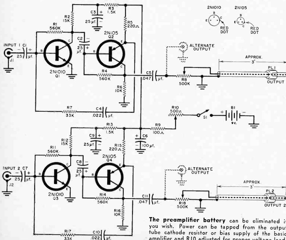
The preamplifier battery can be eliminated if you wish. Power can be tapped from the output tube cathode resistor or bias supply of the basic amplifier and R10 adjusted for proper voltage load.
