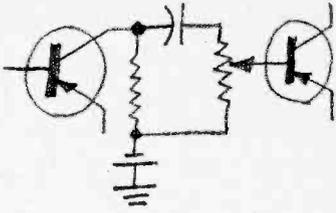
“A vacuum-tube circuit volume control transferred to a transistor circuit would look like this. Whereas a tube draws almost no grid current, the base input of the transistor does—and right through the control. You can see how moving the “pot” arm up and down is not only going to tap off a part of the signal current, which is what we want it to do, but unfortunately it’s also going to change the value of the base bias resistor. A volume control with no problems looks like this.
