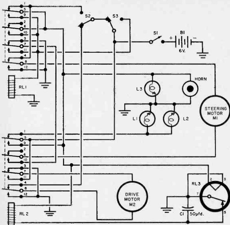
The coding of brain relays RL1 and RL2 correspond to the relay contact pictorial shown on next page. Note that RL3 may not operate unless batteries are at full charge.
