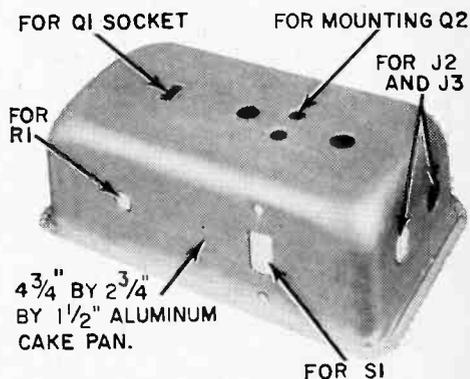
1 A small toy aluminum pan is used as the chassis. The holes can be cut to size with a pen knife and a few small files. Schematic and parts list are on next page.
