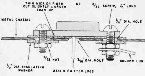
**2** Prior to mounting power transistor Q2, cement two 1/2" fiber washers to the chassis as shown. If done correctly, the mounting screws and lugs of Q2 will be insulated from chassis ground.
