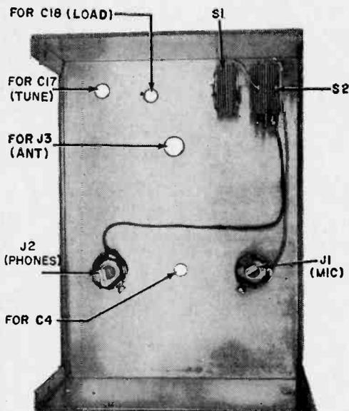
can install the transmitter next. Visually check the chassis alignment and drill the holes to fit the shafts. Mount the transmitter using extra nuts on the *Tune* and *Load* capacitors. Now connect a 2" piece of insulated hookup wire to pin 2 of *V2* and a 6" piece of wire to the antenna jack. Run the longer wire through a convenient hole in the transmitter chassis and twist tightly around the shorter wire soldered to *V2*. This forms a "gimmick" capacitor a little
