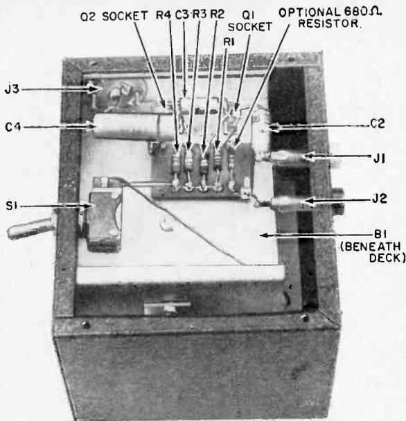
**Bottom view** of black box with cover removed. The two transistors and the battery are on the other side of the deck. A 680-ohm resistor can be wired across J1 and J2 to widen bandwidth, but sensitivity will be lost.
