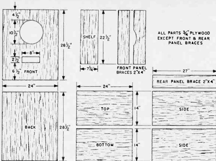
**Construction** of the Reflex 12 is simple since all joints are butted. At left, wooden parts are shown cut to required dimensions. Below is an exploded view of the enclosure's construction.
