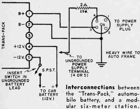
mounting plate. The 5-screw terminal strip is mounted on the *outside* of the chassis lip to minimize the possibility of shorts.
