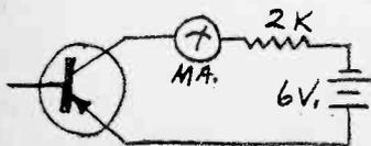
plification factor (*beta*) in the collector circuit.”
