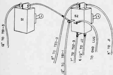
Fig. 6. Wiring details of toggle switches *S1* (on-off) and *S2* (transmit-receive). Leads to *J1* and *J2* should connect to the normally grounded lugs (*J1* and *J2* are insulated from the metal chassis by 1/2" rubber grommets).
