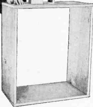
**1** Sides, top and bottom of enclosure are assembled using a good wood glue and 8d (penny) finishing nails. All joints are butted with five or six nails per joint. Design of cabinet makes use of cleats unnecessary.
