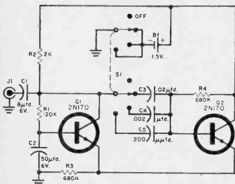
**Frequency-determining** capacitors C3, C4 and C5 will provide 100-, 1000-, and 10,000-kc square waves. Other frequencies can be obtained by using other capacitor values.
