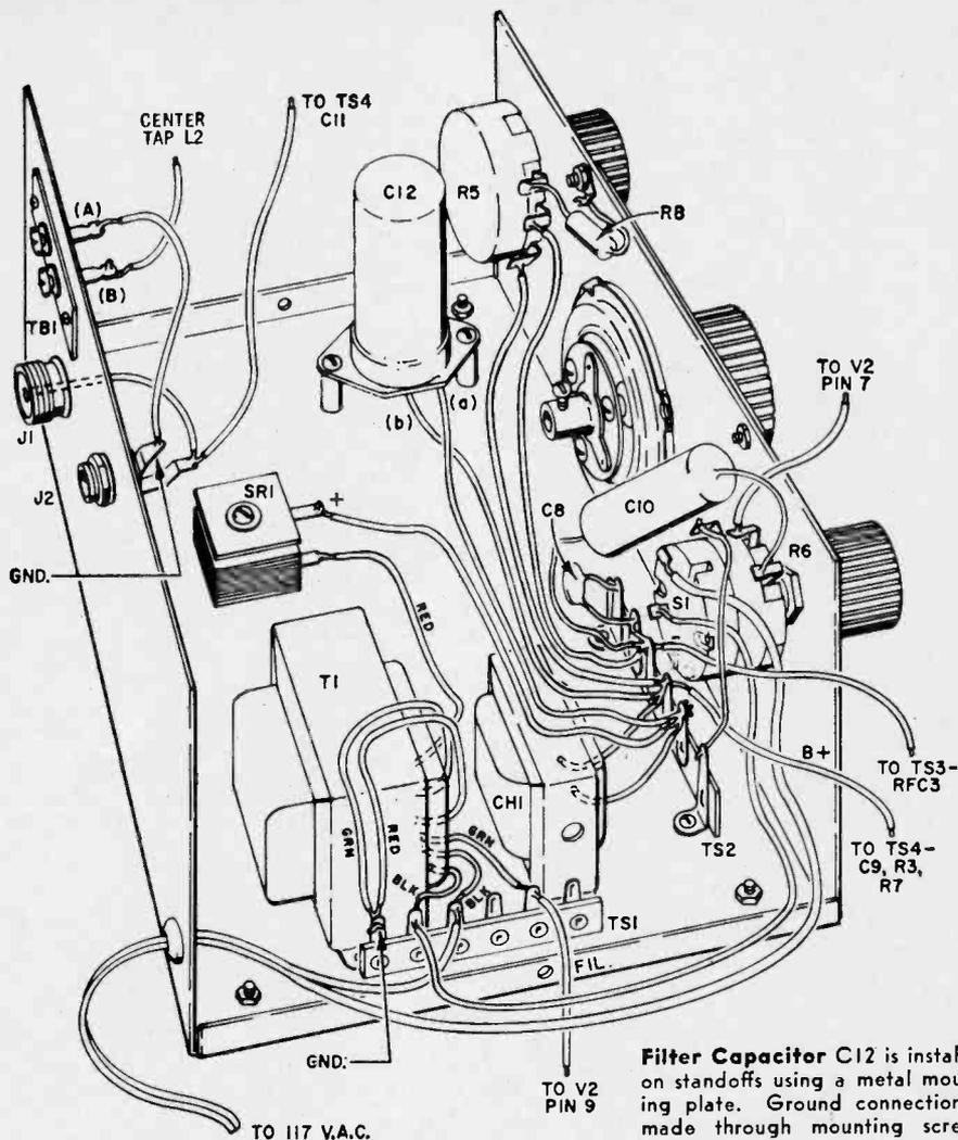
**Filter Capacitor C12** is installed on standoffs using a metal mounting plate. Ground connection is made through mounting screws.
