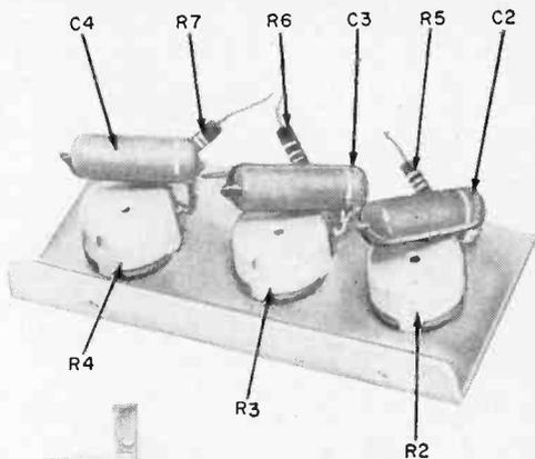
**Subchassis** holds the calibrating potentiometers. Three holes in the back panel provide access for screwdriver calibration.
