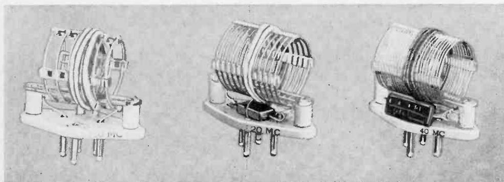
tickler winding starts with unused pin 1. Solder one end of a piece of hookup wire in this pin. Then make three turns around the center of the coil and solder the remaining free end of the wire into unused pin 5. It is important that this winding, like the winding already on the coil, be in a clockwise direction.
