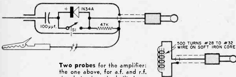
Two probes for the amplifier: the one above, for a.f. and r.f. signal tracing, is built in a small shielded container; the induction probe at right has an unshielded winding.
