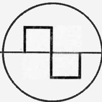
We have all read of the advantages of using square waves to test our hi-fi equipment, only to be scared off by the cost and complexity of the generator. The rise-time requirements are strict, or interpretation of the results is very difficult. However, low-cost transistors are available which make possible a simple unit with rise-times as good as 2.5 *microseconds*.
