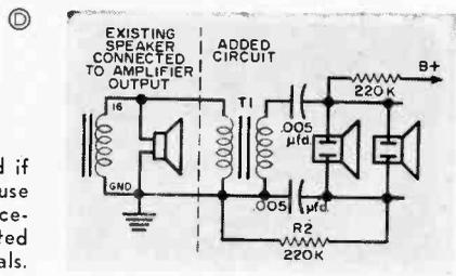
Alternate circuit to be used if the circuits of B and C cause the amplifier to oscillate. Voice-coil leads of T1 are connected to amplifier output terminals.
