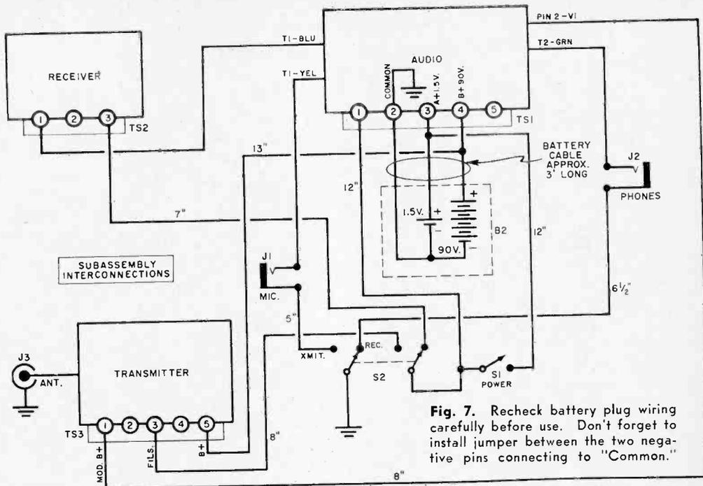
Fig. 7. Recheck battery plug wiring carefully before use. Don't forget to install jumper between the two negative pins connecting to "Common."
