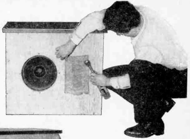
8 Plastic hi-fi grille cloth made by Mellotone is wrapped around cabinet and stapled into place. This material is recommended for speaker enclosures because it is strong, good-looking, and acoustically transparent. After the grille cloth is stapled, legs or a base can also be installed.
