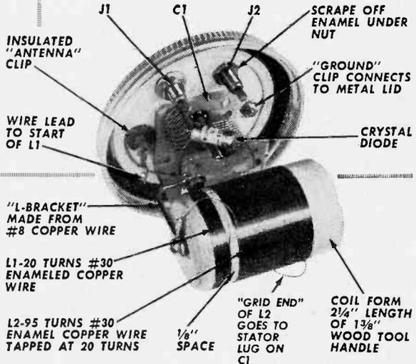
The next time you finish a jar of peanut butter, don't throw away the empty jar. Put a crystal receiver in it! A few inexpensive parts will transform that old dispenser of sandwich filling into a dispenser of local radio broadcasts.
