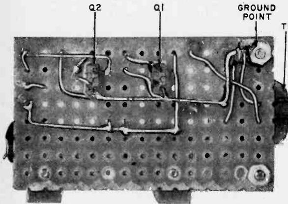
but they are not necessary. The leads of the transistors may be run through the holes in the board and connections soldered directly to them. Be sure to use a heat sink and solder as quickly as possible, since transistors are very easily damaged by excessive heat.
