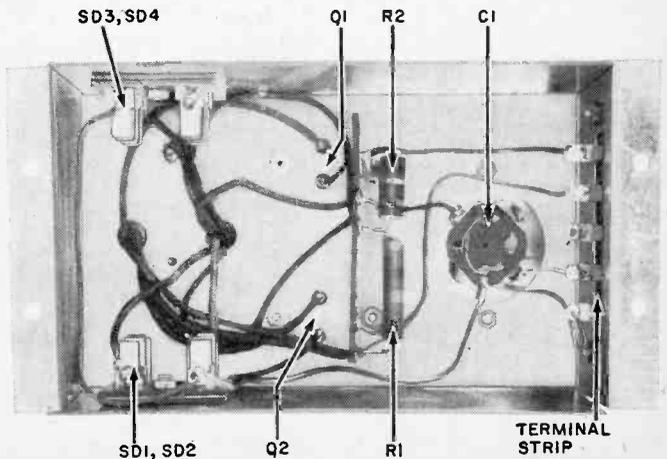
**Parts arrangement** beneath the chassis is non-critical. Holders for the silicon rectifiers may be fuse clips or special diode clips. Make sure that all components are properly insulated and polarized.
