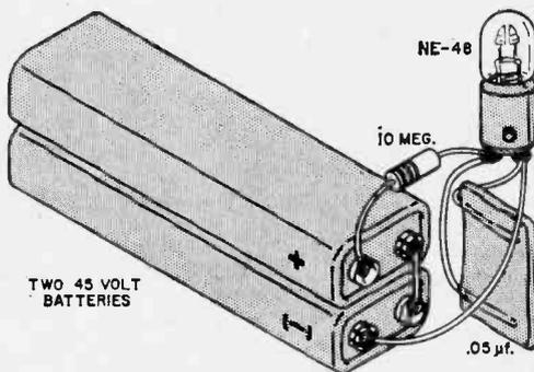
The "bug's" battery terminals should be insulated carefully to prevent the kiddies from getting a 90-volt "tickle" from the battery.
