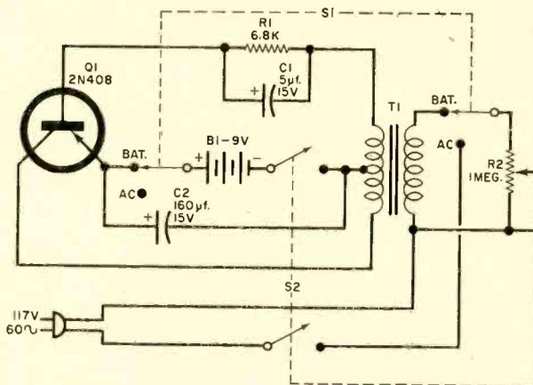
Center-tapped secondary of reverse-connected transformer T1 is coil for Hartley oscillator circuit. About 125 volts appear across primary.
