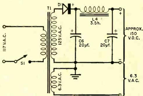
supply. If you are powering the booster from an a.c. (only) communications receiver, connect the booster's three-wire power cable to a plug that matches the set's accessory socket, if it has one. The exact "B" supply voltage for the booster should be about 150 volts d.c., but no more than 170 volts d.c. If your receiver has a 12-volt a.c. heater supply, connect a 36-ohm, 2-watt, 5% composition resistor in series with the booster's ungrounded 6.3-volt a.c. heater lead.
