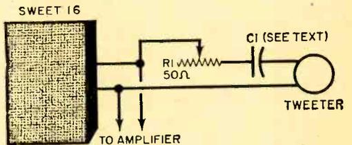
**Schematic** diagram of a recommended hi-pass filter for use with super-tweeter.
