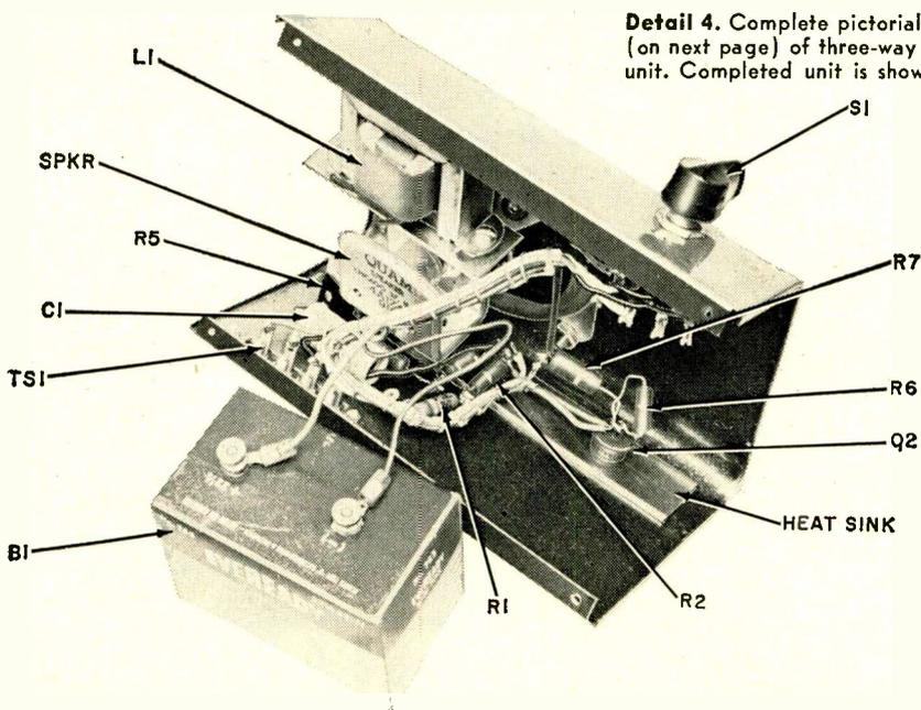
**Detail 4.** Complete pictorial diagram (on next page) of three-way intercom unit. Completed unit is shown below.
