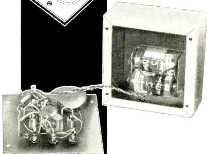
position, the "bad" lamp shouldn't light; if it does, the transistor has excessive leakage. If both lamps light when *R1* is at a maximum, it indicates that the transistor is operative but may not work in critical circuits.
