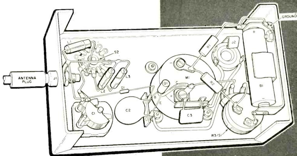
**Small metal utility box** houses and shields FSM parts. The leads of coils L1, L2 and L3 should be as short and direct as possible. Notice that the polarity of mercury battery B1 is unusual; the casing is positive and the insulated center disc is negative.
