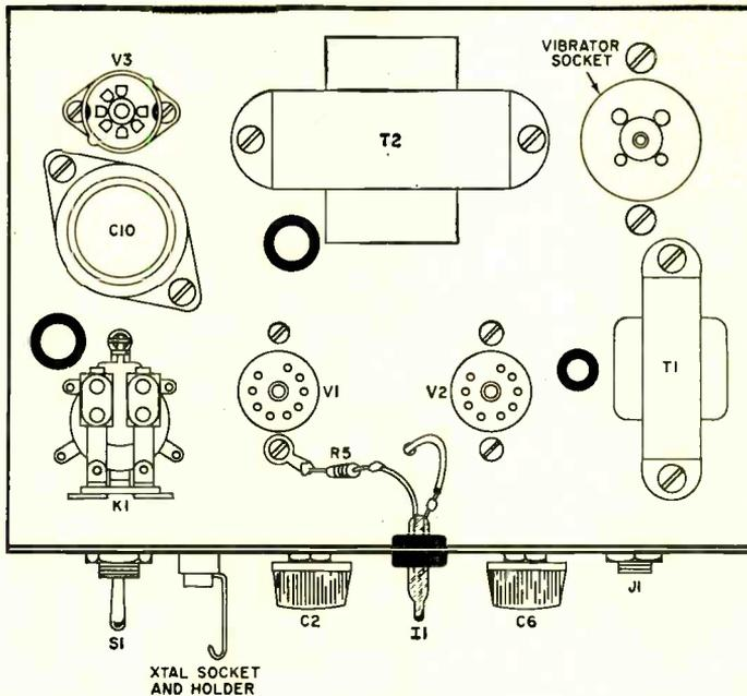
Drawing of top of chassis, with case removed. Neonbulb *V3* serves as a tuning indicator and is held in place by a rubber grommet; *R5* is soldered directly to one lead and attached to a solder lug under a screw at *V1*'s socket.
