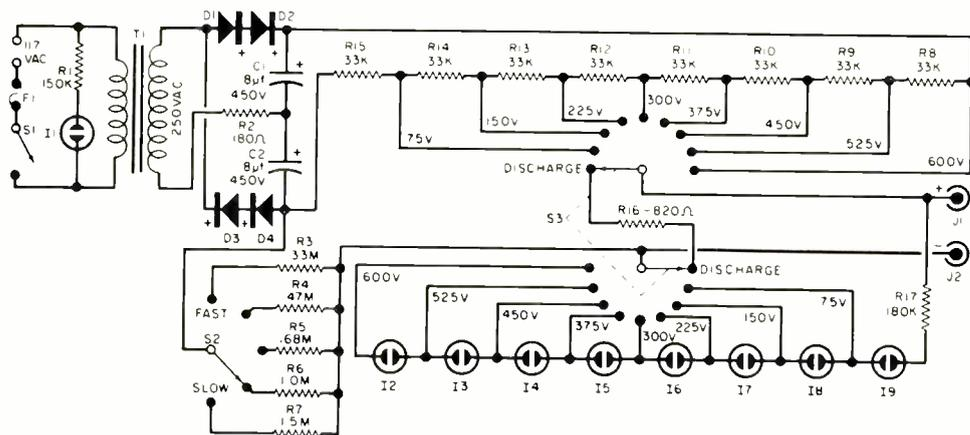
**Schematic diagram** of the "Restorer." Switch *S3* taps the power supply's voltage divider, selecting the "forming" voltage, and also controls the indicating lamp circuit. Switch *S2* inserts the proper current-limiting resistor.
