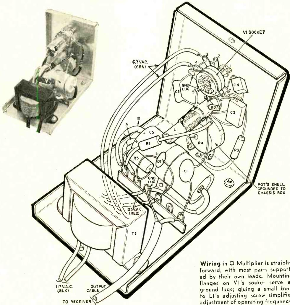
Wiring in Q-Multiplier is straightforward, with most parts supported by their own leads. Mounting flanges on V1's socket serve as ground lugs; gluing a small knob to L1's adjusting screw simplifies adjustment of operating frequency.
