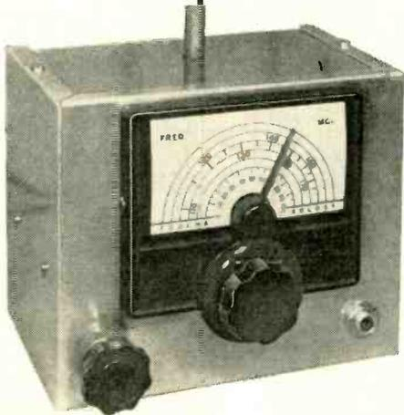
**T**HE BAND OF FREQUENCIES (108 to 174 mc.) lying between the FM band and television Channel 7 offers the experimenter a variety of exciting and informative listening—aircraft communications and navigation signals, messages from ships at sea, and so on. Here, too, are “on the spot” reports from police and fire department emergency crews, and even the two-meter ham band.
