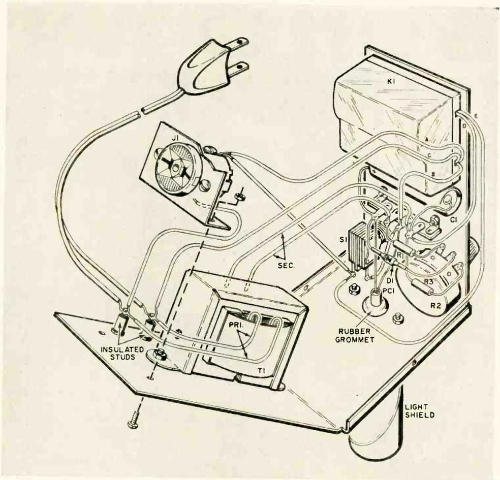
**Infrared detector wiring** is simple and straightforward, although photocell PCI requires special consideration. See text for details.
