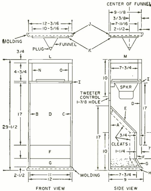
Diagram showing placement of all parts in enclosure. Resistive panel (E) will overlap the duct panel and must be trimmed to fit.
