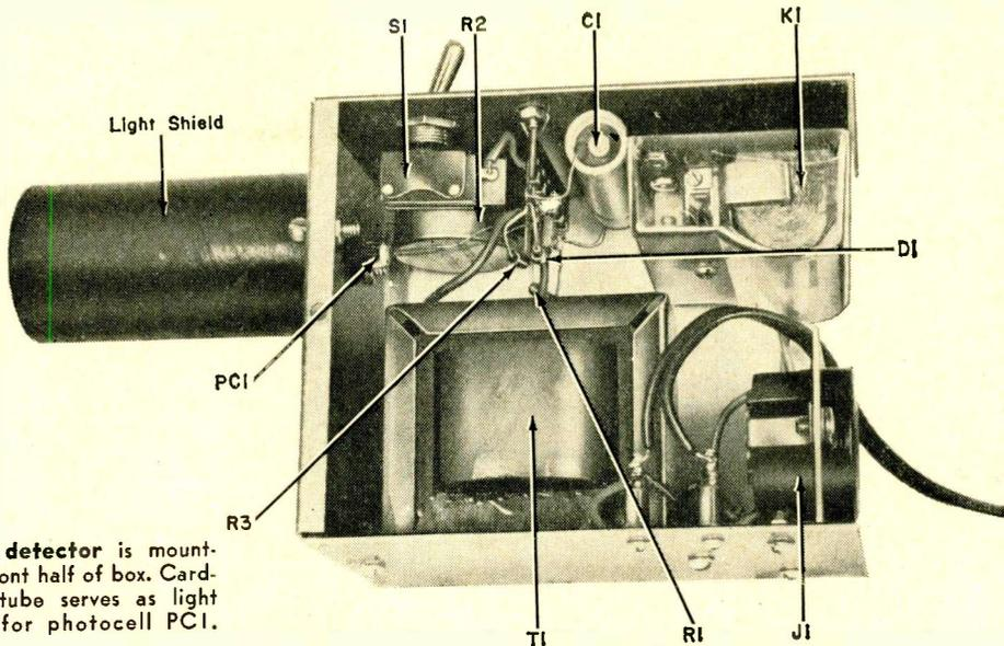
Entire detector is mounted in front half of box. Card-board tube serves as light shield for photocell PC1.
