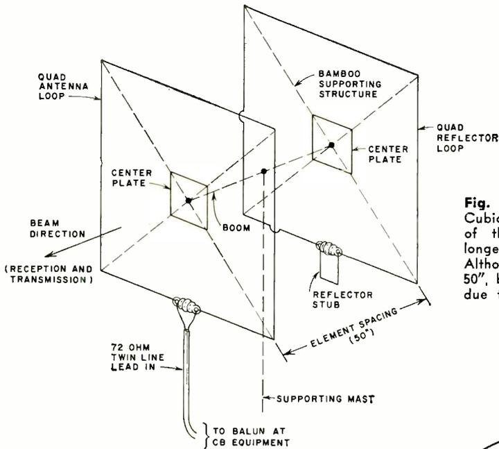
**Fig. 1.** Designer's "eye view" of Cubical Quad antenna. Each side of the square loops is slightly longer than one-quarter wavelength. Although spacing between loops is 50", boom will be about 1" shorter due to thickness of center plates.
