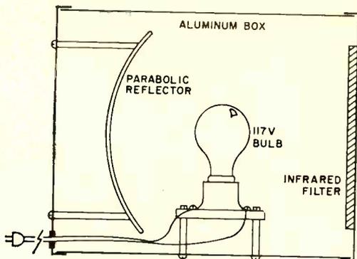
Infrared spotlight's box should have lightproof air vents. Use high-wattage lamp for long beam lengths.
