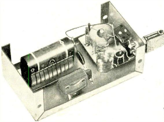
Follow the parts layout shown here as closely as possible to minimize changes in stray capacitances.
