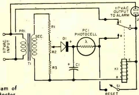
Schematic diagram of the infrared detector.
