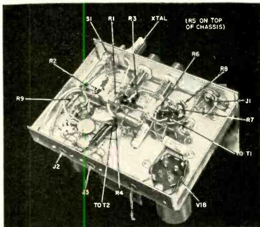
Two views of underside of chassis, showing location of principal parts. Leads should be as short as possible.
