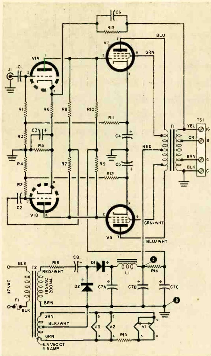
**In normal operation**, voltage from point A to point B is 390 volts d.c. Heater current to tube V1 is "starved" by use of dropping resistor R15.
