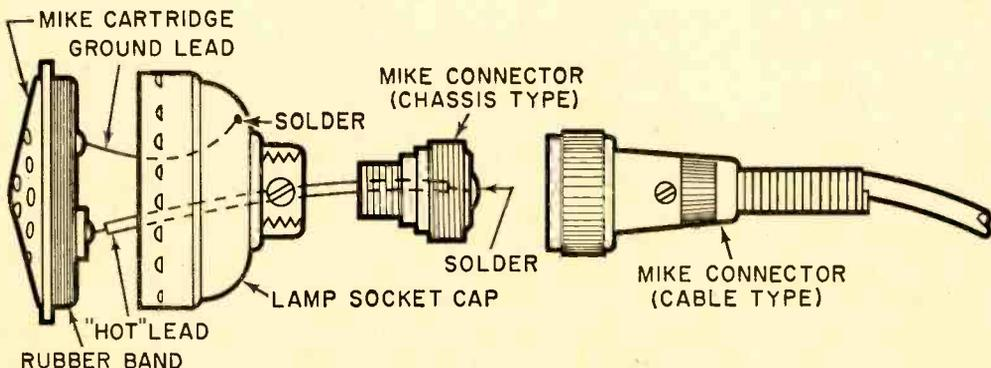
out to a mike connector (Amphenol 75-PC1M) screwed into the cap's mounting collar.
