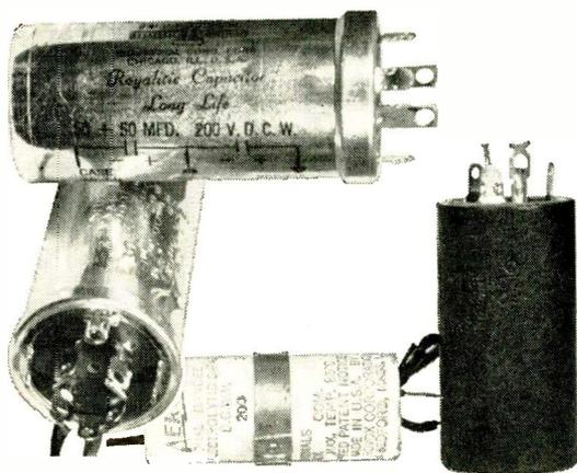
the film to deteriorate. Full voltage placed on an electrolytic that has been idle for some time will almost invariably puncture the weakened dielectric, ruining the unit.
