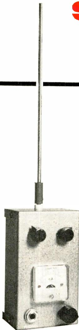
The FSM has headphone output jack for checking transmitter's audio quality. Plugging in headphones does not change sensitivity of instrument.
