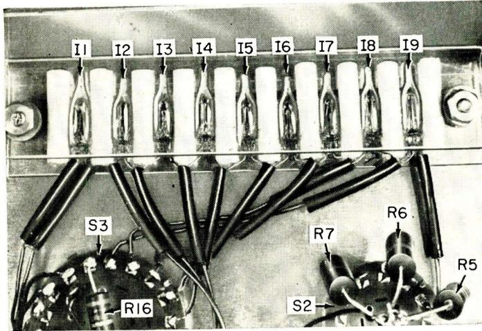
**Details of the Restorer's lamp holder can be seen clearly in this photo; the author made his holder from a single strip of plexiglass. Quick-drying cement keeps lamps and rolled-paper separators in place.**
