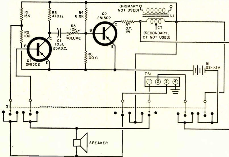
**Two-stage transistorized amplifier** above is heart of each of the three-way intercom units. External cable connections are made to terminal strip TSI.
