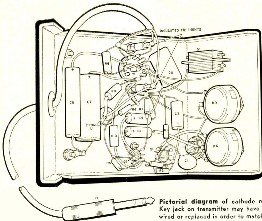
**Pictorial diagram** of cathode modulator. Key jack on transmitter may have to be re-wired or replaced in order to match plug P1.
