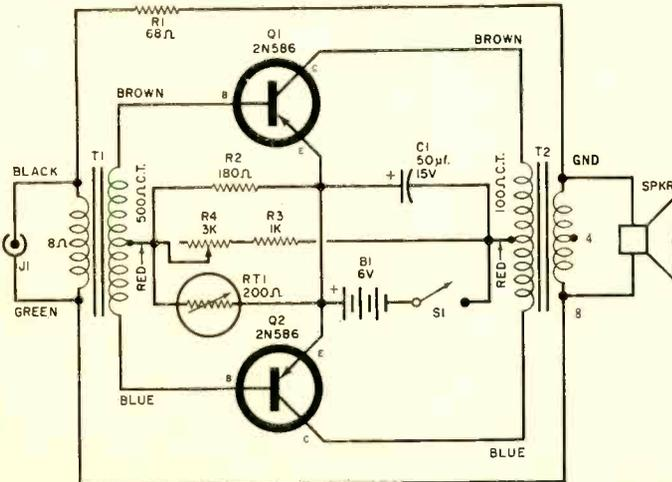
**Pictorial diagram** (above, top) and schematic diagram (left) show simplicity of Transi-Booster circuitry; proper setting of *R4* and effect of *R1* are discussed in text. Small schematic (above) gives details for adding a phone jack to a transistor portable.
