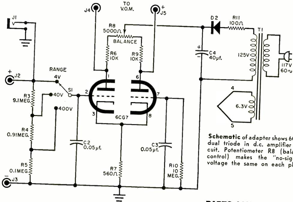
Schematic of adapter shows 6CG7 dual triode in d.c. amplifier circuit. Potentiometer R8 (balance control) makes the "no-signal" voltage the same on each plate.
