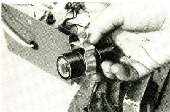
**Socket assembly** for tube V2 in workshop tester includes mounting bracket and escutcheon plate.
