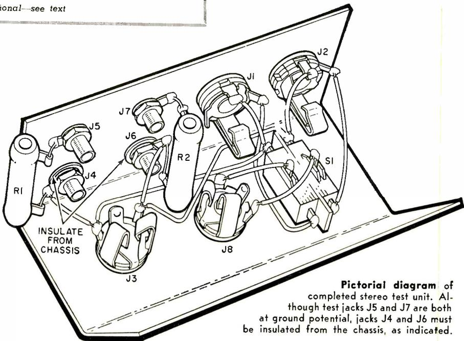
**Pictorial diagram** of completed stereo test unit. Although test jacks J5 and J7 are both at ground potential, jacks J4 and J6 must be insulated from the chassis, as indicated.
