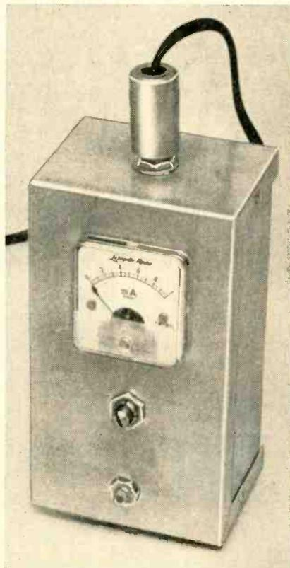
mounted in a holder made of 1" sheet-metal or aluminum strip.
