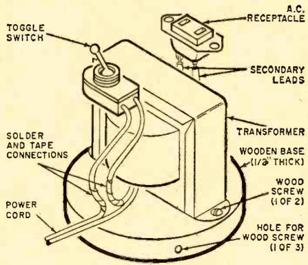
**Isolation transformer assembly** makes it safe to operate any a.c./d.c. receiver with a hi-fi set.
