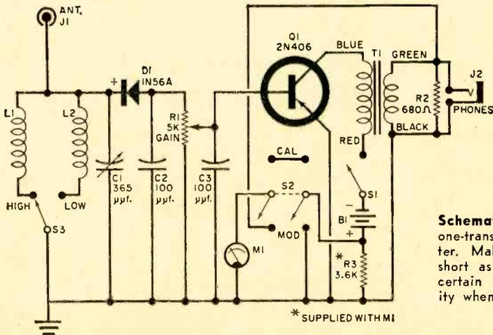
**Schematic diagram** of one-transistor Monitor Meter. Make all r.f. leads as short as possible, and be certain to observe polarity when wiring diode D1.
