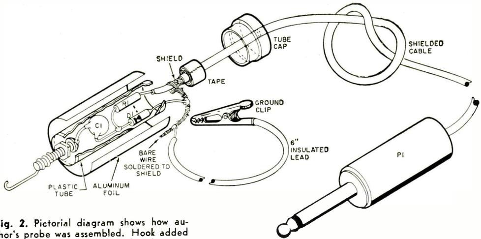
**Fig. 2.** Pictorial diagram shows how author's probe was assembled. Hook added to probe screw simplifies trouble-shooting.
