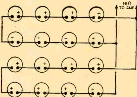
**Wiring diagram** for use with a 16-ohm amplifier output. See text for instructions on how to phase speakers properly.
