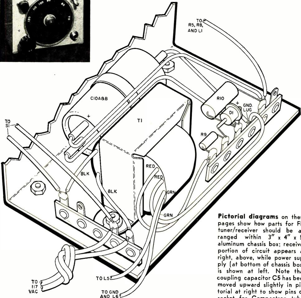
**Pictorial diagrams** on these pages show how parts for FM tuner/receiver should be arranged within 3" x 4" x 5" aluminum chassis box; receiver portion of circuit appears at right, above, while power supply (at bottom of chassis box) is shown at left. Note that coupling capacitor C5 has been moved upward slightly in pictorial at right to show pins on socket for Compactron tube.
