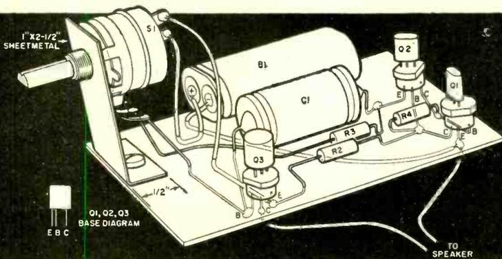
Lightweight lines in pictorial diagram indicate leads running under board. Mounting nut for potentiometer R1 also secures chassis to side of baffle.
