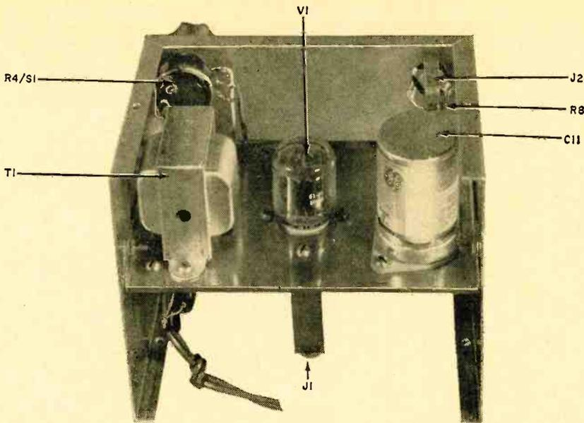
**Inverted view** of receiver with cover removed shows placement of major components. All parts are mounted on subchassis except regeneration control  $R4$  and phone jack  $J2$ .
