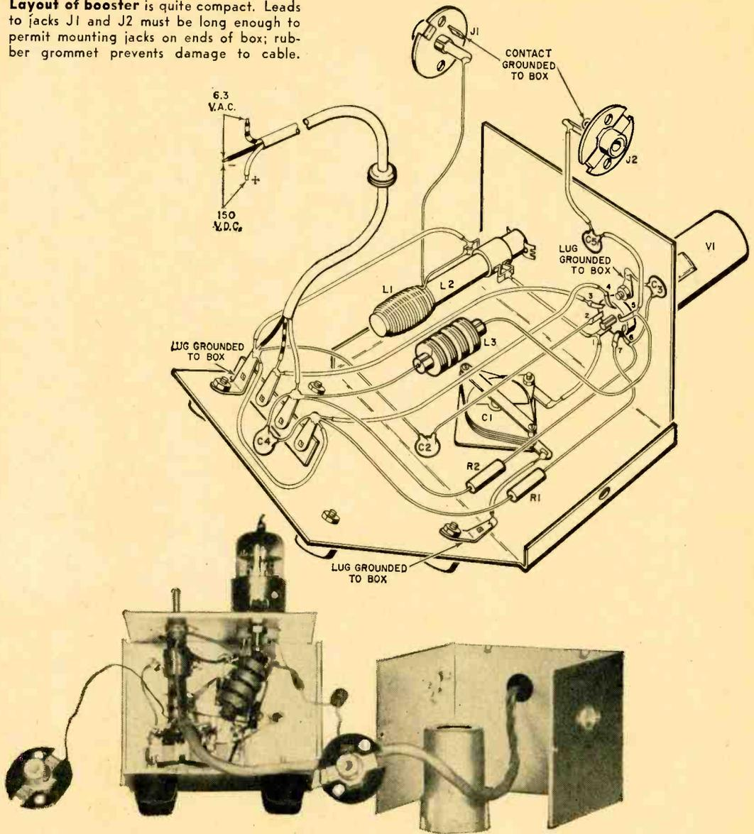
jack *J1* and connect the receiver's antenna terminals to jack *J2*. For operation with a long-wire antenna, connect only the center (hot) terminal of *J1* to the antenna with a good ground connected to *J1*'s ground.
