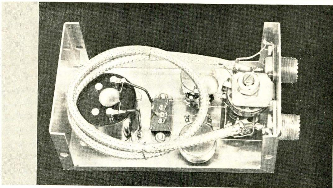
**Parts layout of power meter** is highly symmetrical and reflects arrangement of schematic diagram on page 157 very closely. See text for details of pickup loop.
