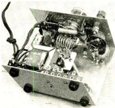
rate as the frequency of the incoming signal; the frequency of this oscillation is determined principally by the values of coil *L2* and variable capacitor *C3*. The lower-frequency oscillation or "quench" frequency is determined chiefly by the values of capacitor *C4* and resistor *R2*, as well as the position of the tap on *L2*. Amplitude of the quench oscillation, in turn, depends on the plate voltage and can be controlled by the setting of potentiometer *R7*.
