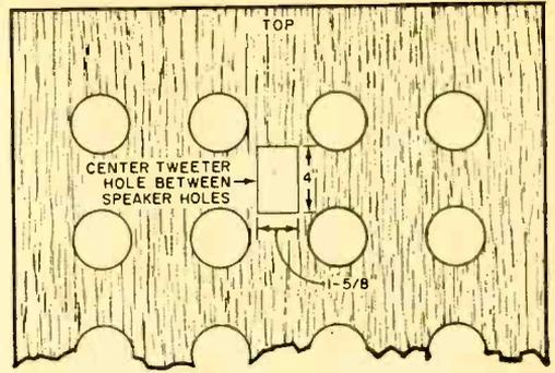
**Cutout** for tweeter should measure  $4 \times 1\frac{5}{8}$ " as shown if a Calrad Type CT-3 is used; other tweeters may require a different size hole.
