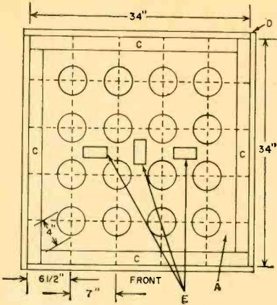
**Front panel (A)** is drilled following layout at left before side rails (C) are attached. Spacers (E) can be cut to fit from pieces sawed off from side rails.
