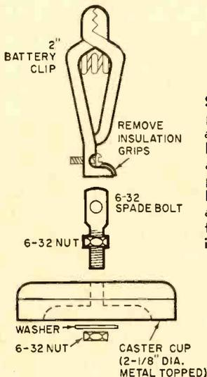
**Swivel desk mike** pictured above is assembled from a lamp socket cap plus a few other common pieces of hardware. Diagram of stand is at left; construction of microphone is shown below.
