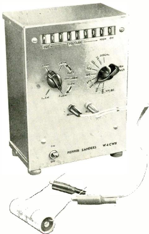
**I**F YOU'RE one of the many experimenters who have large stocks of used electrolytic capacitors in storage, you know that such units often break down as soon as they are again placed in service. These capacitors aren't cheap, and you can avoid wasting them by using this efficient automatic restorer. Costing less than \$16.00 to build, the device will give the most senile electrolytic in your spare parts box a new lease on life.
