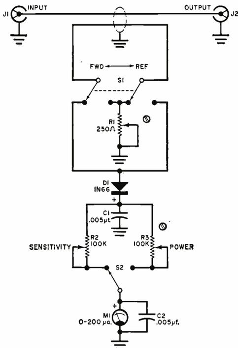
**Schematic diagram** of CB meter. Potentiometers R1 and R3 should have screwdriver adjustment. in the *Ref* position. The SWR can then be calculated using the lowest *Ref* value.
