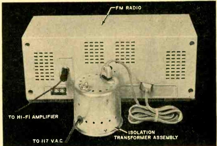
hi-fi amplifier and speaker system. The jack is wired across the radio's de-emphasis capacitor, as shown in the schematic diagram. Although the exact mounting details will vary from set to set, the jack can usually be placed at some convenient spot at the rear of the radio.
