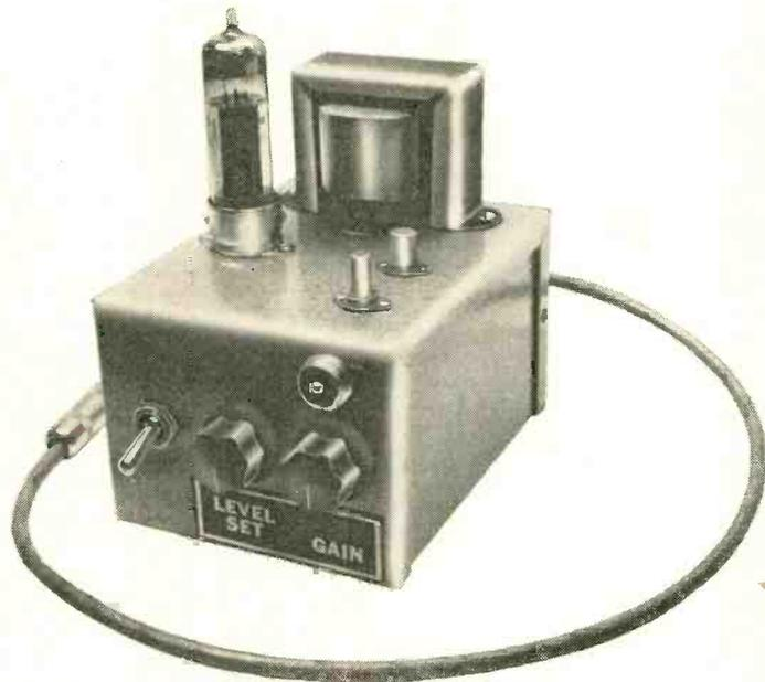
**H**ERE'S a simple modulator specifically designed for amateur transmitters whose plate current during c.w. operation is 120 ma. or less. Compact in size as well as easy to install and remove, it can be used with almost any small transmitter having a keyed final amplifier. Powering the modulator is no problem, since the entire unit—with the exception of the 6BQ5 heater—
