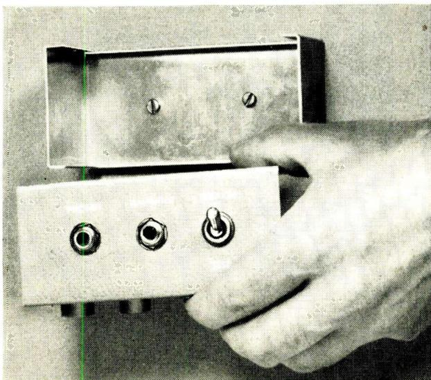
**Aluminum utility box** with snap-on cover simplifies mounting of stereo test unit. With cover attached to equipment cabinet, the test unit can easily be removed. If "easy remove" feature is not needed, however, the unit can be mounted in an aluminum box and permanently attached to the hi-fi cabinet.
