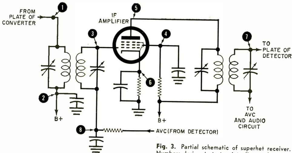
Fig. 3. Partial schematic of superhet receiver. Numbers designate test points discussed in text.
