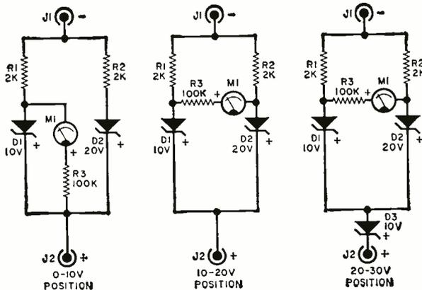
**Equivalent circuits** for each of the three positions of the range switch. "Offsetting" diode *D3* is placed in the circuit only when *S1* is in the 20-30 volt position.
