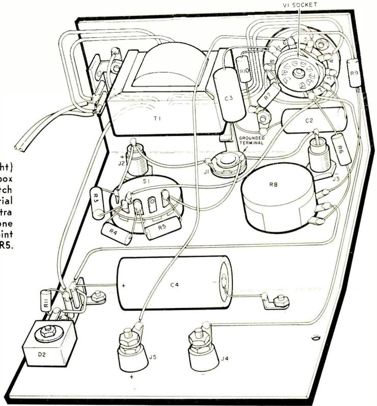
tive lead to *J5*. The adapter is plugged in and, after it has warmed up, balance control *R8* is set for a zero reading on the multimeter. Connect the adapter's d.c. test leads across a 1.5-volt flashlight cell, then several cells in series, and finally a variable voltage power supply—checking several points on the three ranges.
