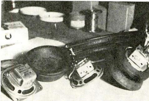
Speaker mounting flanges should be clipped off, as shown. Enlarge holes in cushions for best response.
