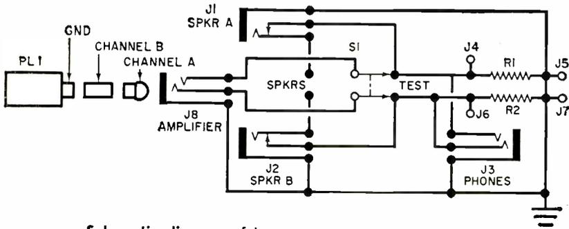
**Schematic diagram** of inexpensive stereo test unit. As explained in text, output from stereo amplifier can be fed to speakers A and B, stereo headphones, or test jacks J4 to J7.
