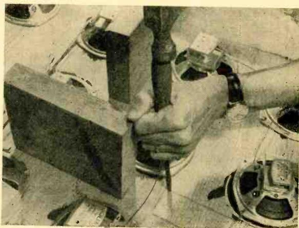
**Chisel and hammer** combination is best for making required cutout, tweeter placement is not critical.
