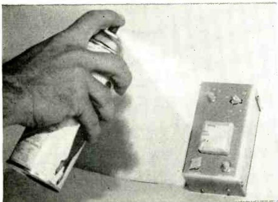
A clear plastic spray such as Krylon is used to protect the panel decals. Front panel parts are covered with tape and cardboard while spraying.
