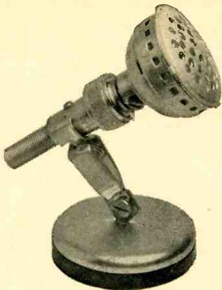
THE VARIETY OF inexpensive microphone cartridges now on the market is a challenge to the experimenter's ingenuity. Many of them are sensitive units with good frequency response. Mount one in an appropriate housing and you'll have a useful microphone at little cost.
