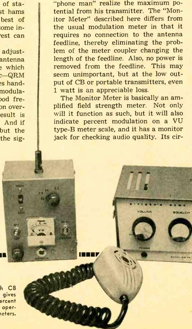
Particularly useful with CB rigs, the Monitor Meter gives continuous indication of percent modulation for transmitters operating between 80 and 10 meters.
