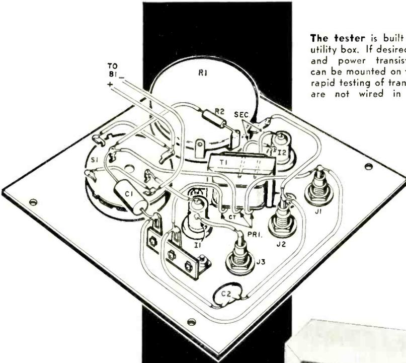
The tester is built in a small utility box. If desired, an audio and power transistor socket can be mounted on the box for rapid testing of transistors that are not wired in a circuit.
