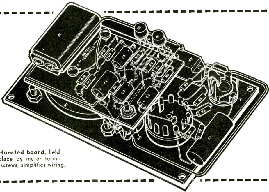
**Perforated board, held in place by meter terminal screws, simplifies wiring.**
