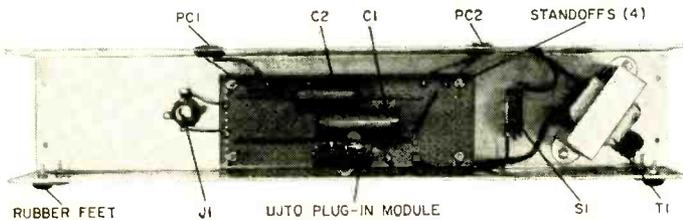
Fig. 5. Electrical components are first mounted on the perforated phenolic board which is then mounted on the chassis with four standoff spacers. Orientation must be as shown in diagram.
