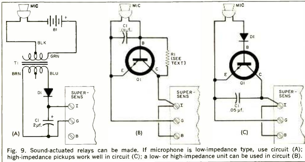
Fig. 9. Sound-actuated relays can be made. If microphone is low-impedance type, use circuit (A); high-impedance pickups work well in circuit (C); a low- or high-impedance unit can be used in circuit (B).
