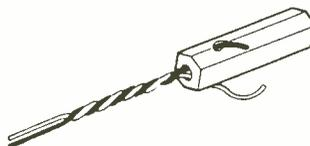
ameter and drill three holes in it as shown in the diagram. Hole size depends on the gauge of the wire you intend to twist; side holes should be drilled at angles of less than 45° for best results. To use, simply insert the two wires in the side holes and pull them from the center hole. Connect one end of the wires to be twisted in a vise and place the die in a hand drill. Then simply rotate the drill and work the die along wires until the lengths of wire are properly twisted.
