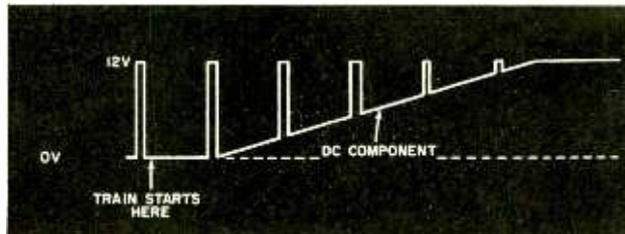
Fig. 1. The ordinary power pack is nothing more than a full-wave rectifier whose output is a pulsating d.c. voltage with peaks that look like the waveform above. For most locos, the average power required for starting is much too high for a smooth start, and the trains pull out with a sudden jerk, and at a speed not akin to real railroading.
