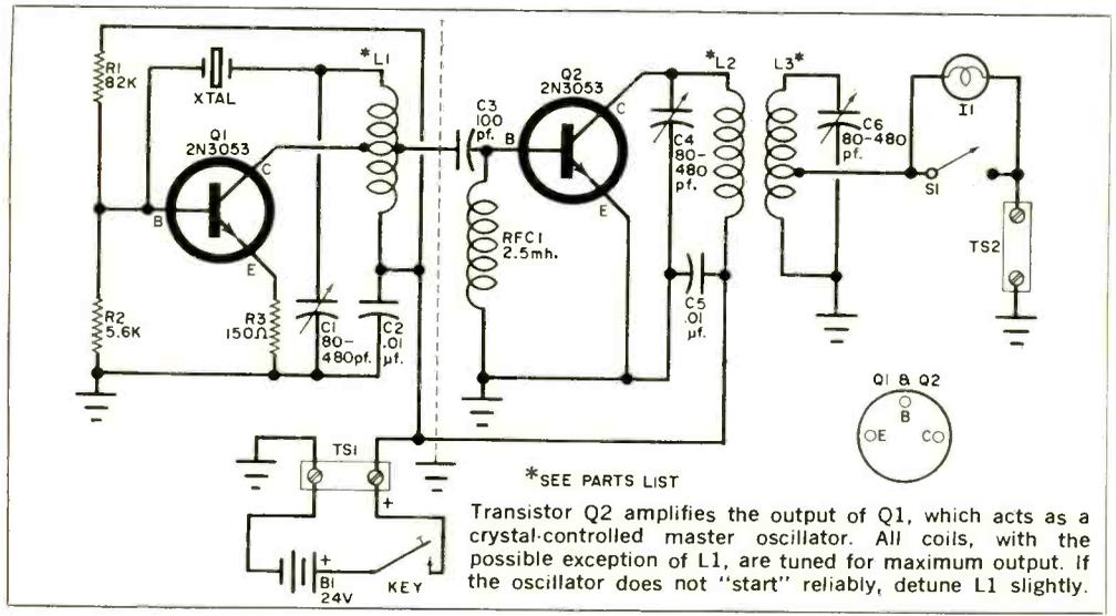
Transistor Q2 amplifies the output of Q1, which acts as a crystal-controlled master oscillator. All coils, with the possible exception of L1, are tuned for maximum output. If the oscillator does not "start" reliably, detune L1 slightly.
