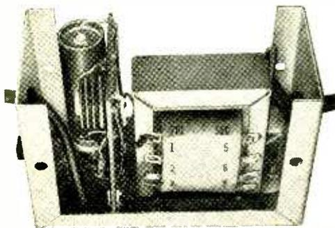
Preassemble the circuit board and install after *S1*, *I1*, and *T1* (in that order) are mounted. Connect all leads and check the circuit before closing box.
