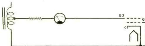
Fig. 2. Meter reads relative emission. Tests made at 1-minute intervals show warm-up characteristics.
