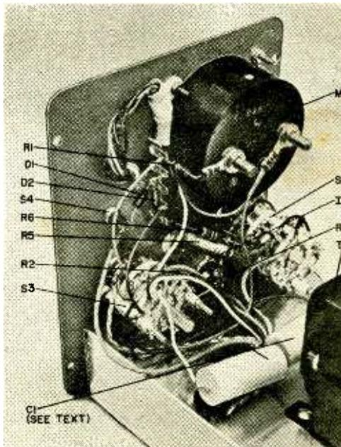
Fig. 6. Nothing is critical here, except for meter polarity. Most of the components are panel-mounted.
