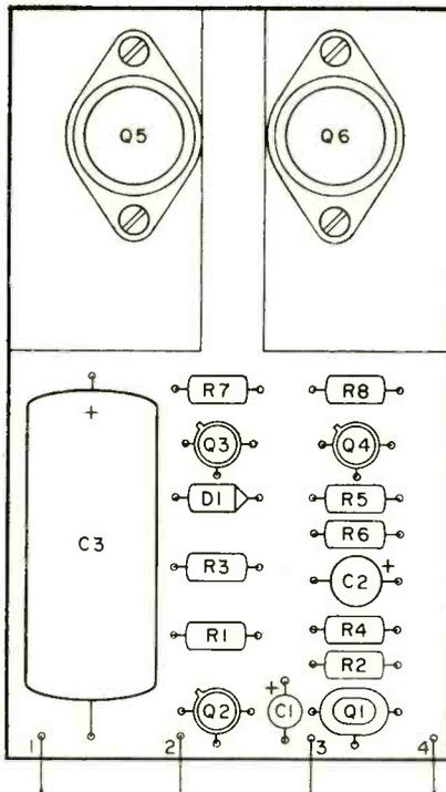
Fig. 2. Carefully locate and solder all of the components onto the printed circuit board as shown.
