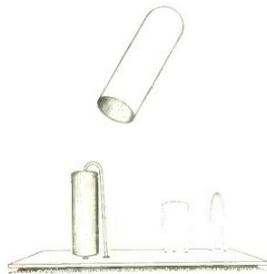
the component and the lead with a plastic "Fit-Cap," such as manufactured by the Alpha Wire Co., and apply a bit of heat. The shrinkable plastic reduces in size, grips and insulates the component.
