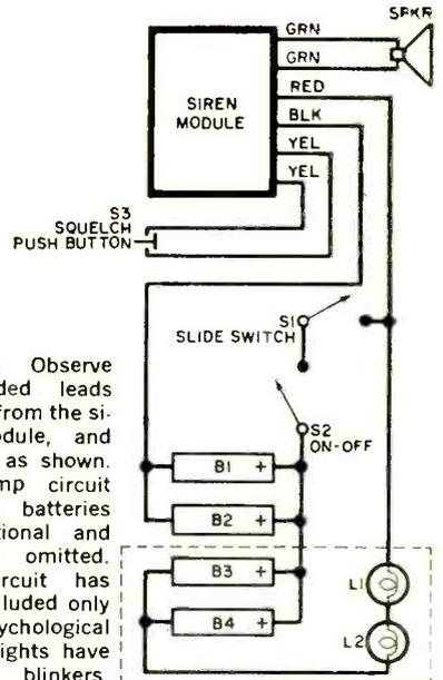
Fig. 2. Observe color-coded leads coming from the siren module, and connect as shown. The lamp circuit and its batteries are optional and can be omitted. This circuit has been included only for psychological effect. Lights have built-in blinkers.
