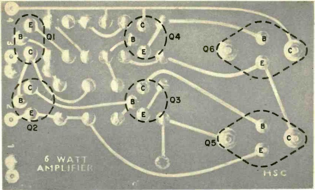
Fig. 3. Use this full-size guide in making your printed circuit board. Space the transistors about  $\frac{1}{2}$ " above the board and hold transistor leads on top side of board with a pair of long-nose pliers when soldering.
