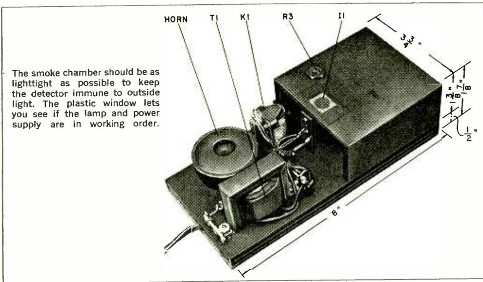
or other wall hanger for holding the finished smoke alarm. Complete all wiring and mounting of parts before you screw down the back cover.
