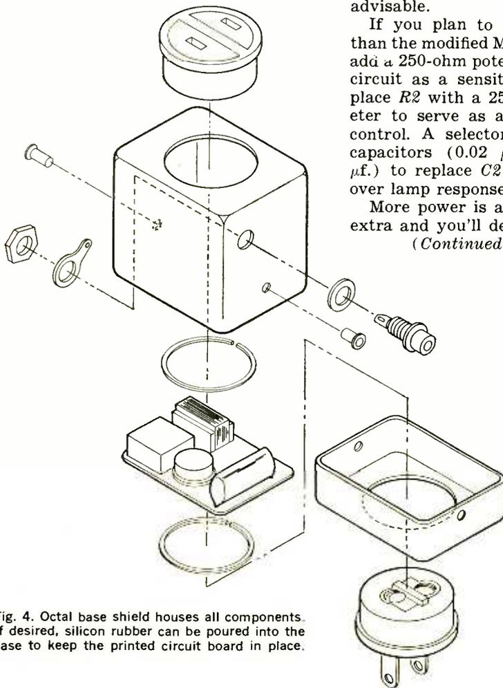
Fig. 4. Octal base shield houses all components. If desired, silicon rubber can be poured into the case to keep the printed circuit board in place.
