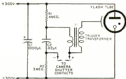
Flash shutter contacts are polarized. Check with a voltmeter, and connect positive side to V2's plate.
