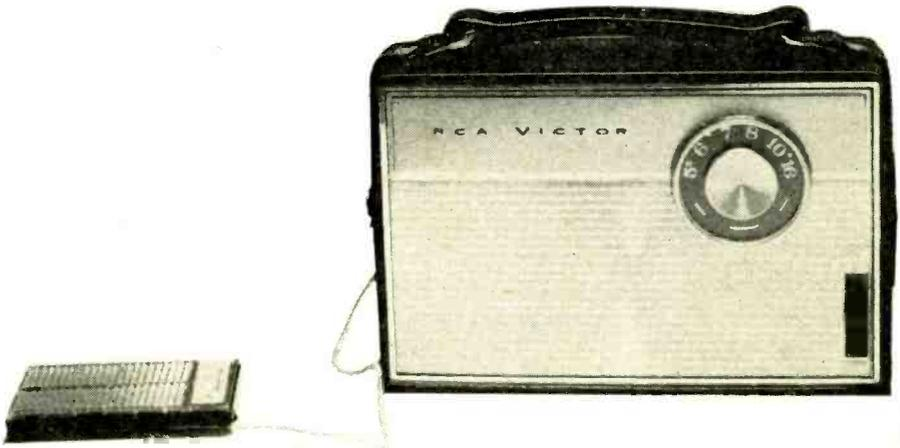
want to add a switch (see schematic) to provide a choice of either solar or battery power. Or you can simply connect the pack's 6" leads to the battery connections inside the radio. You can even use the solar pack as a plug-in supply by connecting an earphone jack and cord to the pack, removing the existing wires from the radio's earphone plug, and running a pair of wires from the plug to the battery connections.
