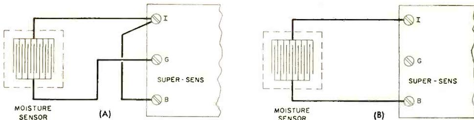
Fig. 8. These circuits can be used to control humidifiers and lawn sprinklers. Just a drop of rain on the sensor will release the relay in circuit (A). Circuit (B) can detect slightest trace of moisture.
