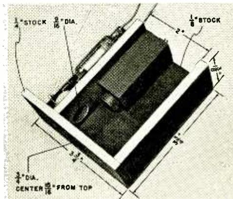
Photocell is mounted at right angles to the sharply focused light. Paint inside of the wooden smoke chamber flat black to minimize light reflections.
