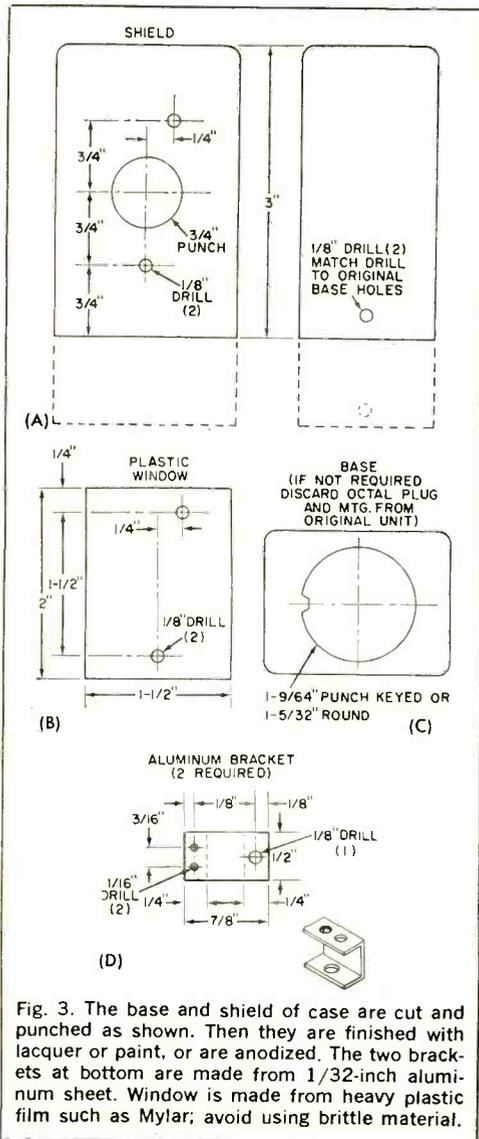
Fig. 3. The base and shield of case are cut and punched as shown. Then they are finished with lacquer or paint, or are anodized. The two brackets at bottom are made from 1/32-inch aluminum sheet. Window is made from heavy plastic film such as Mylar; avoid using brittle material.
