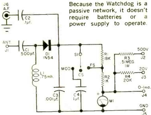
Because the Watchdog is a passive network, it doesn't require batteries or a power supply to operate.
