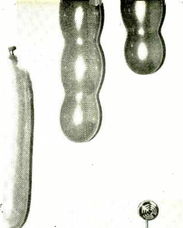
Sound-actuated unit (lower right) flashes strobe as first balloon, hit with dart, bursts. Insert shows drop of milk hitting black background; mike was 10" away, sensitivity of trip unit reduced to just half.
