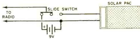
Your portable can be switched to either battery or sun operation by adding a slide s.p.d.t. switch.
