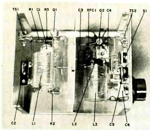
Bend fins on Q2's heat sink to avoid contact with cabinet and leads. For best results, locate components as shown. Lead dress is not too critical,
