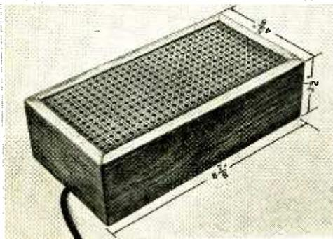
Completed unit is mounted vertically, as close to the ceiling as possible. Rising smoke enters smoke chamber through metal grille to set off the alarm.
