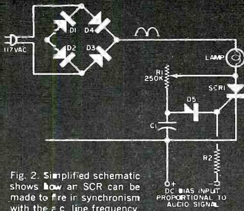
Fig. 2. Simplified schematic shows how an SCR can be made to fire in synchronism with the a.c. line frequency.
