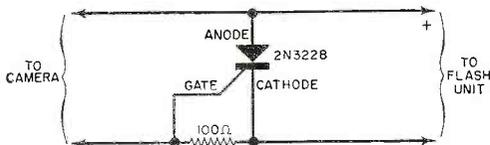
“felt” across the camera’s contacts and extends their life. You can assemble the 2N3228 silicon control rectifier (SCR) and 100-ohm resistor in any small plastic container; a coin holder will do nicely. If you insert the assem-
