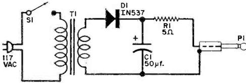
Optional power supply can be installed next to the motor if you use a large enough pie plate as a base, or you can mount it in a box. Construction and parts are not critical.
