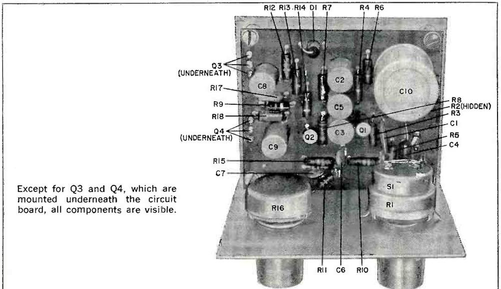
Except for Q3 and Q4, which are mounted underneath the circuit board, all components are visible.
