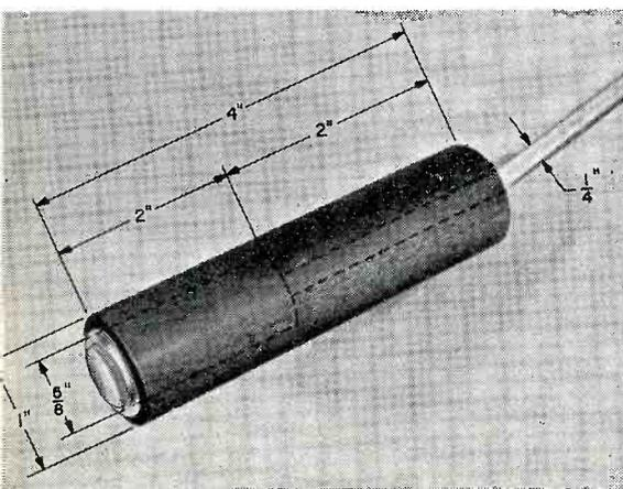
Fig. 3. Switches mounted on one end of wooden dowels make suitable hand-held responders. Any normally open push-to-close type of switch can be used.
