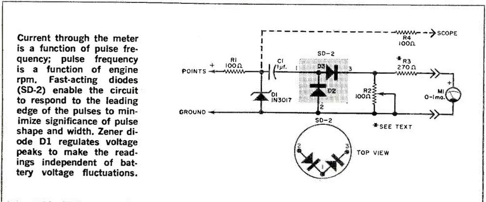
3.5 ma. would indicate 3500 rpm.) When other commercial rpm meters are used, R3 may have to be jumped, as some of them incorporate 0-2 ma. movements. Regardless of scale markings or meter movements used, you should calibrate the tach before you install it in your car.
