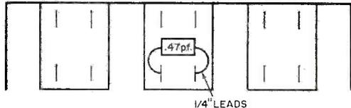
ham band and other services. Solder a 0.47-pF capacitor or “gimmick” across the output resonant tank, and cut the capacitor leads as short as possible—they should be no longer than ¼ inch. Now connect the capacitor across the two tabs sticking out from the center wafer on the bottom of the chassis.
