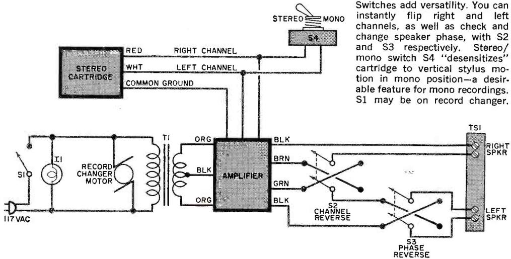
Switches add versatility. You can instantly flip right and left channels, as well as check and change speaker phase, with S2 and S3 respectively. Stereo/mono switch S4 "desensitizes" cartridge to vertical stylus motion in mono position—a desirable feature for mono recordings. S1 may be on record changer.
