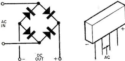
Hardly bigger than a thumbnail, the new prepackaged bridge rectifiers offer numerous advantages to the circuit designer as well as to the experimenter.
