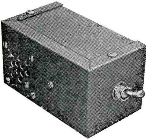
Completed unit should be located within easy reach of the driver. Only two wires connect the alarm to the lights and ignition system. Ground the case.
