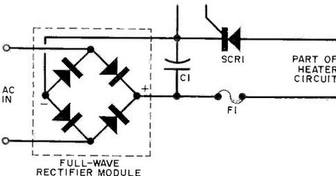
Fig. 5. A full-wave bridge rectifier in the line circuit causes the SCR to conduct on both half cycles, resulting in a doubling of the heater power.
