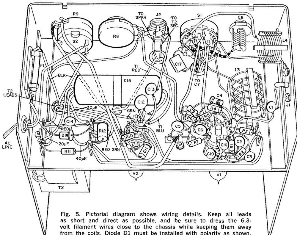
Fig. 5. Pictorial diagram shows wiring details. Keep all leads as short and direct as possible, and be sure to dress the 6.3-volt filament wires close to the chassis while keeping them away from the coils. Diode D1 must be installed with polarity as shown.
