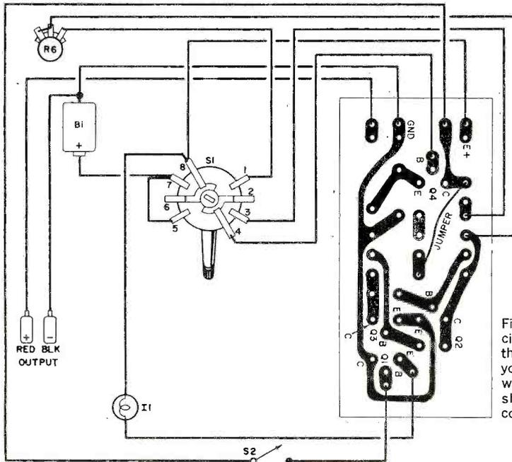
Fig. 4. If you use a printed circuit board, these will be the only wiring connections you will have to run. Jumper wire shown on the circuit board should be mounted on the component side of the board.
