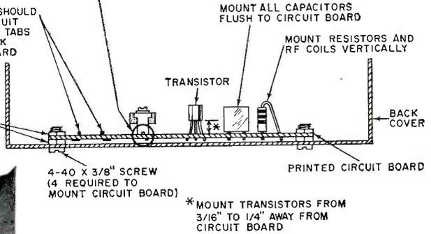
This i.f. amplifier contains two transistors, three i.f. transformers, and crystal diode detector. Be sure to get the J. W. Miller Model 8902-B specified and not the older-style Model 8902 with outboard i.f. transformer.
