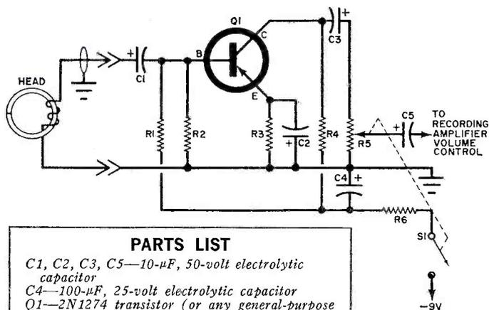
Fig. 2. The echo preamplifier employs a single common emitter stage to provide the necessary gain for the echo effects. Shielded cable connects new pickup head to preamplifier. Capacitor C4 and resistor R6 eliminate hash in tape recorders with brush-type d.c. motors.
