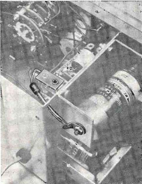
Looking inside a typical VTVM (Heathkit IM-13), note how Eveready N54 nickel-cadmium cell slips into battery holder. Only two additional parts are needed. Tie point is added to support wiring connections between R1 and diode rectifier D1. Filament connection is made at pin 9, V2, in this case.
