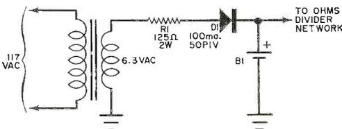
EVERY seasoned experimenter/hobbyist will agree that the VTVM is a basic tool for circuit testing and electronics repair work. But it has one shortcoming—hidden inside that metal case is an ordinary flashlight battery. Too often this battery is forgotten until the experimenter realizes that the ohmmeter readings are way off and a corrosive fluid is seeping out the bottom of the VTVM case.
