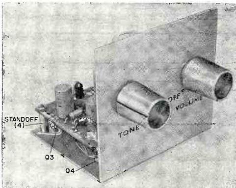
Transistors *Q3* and *Q4* can be inserted in small metal cable clamps and installed underneath the standoffs used to support the printed circuit board.
