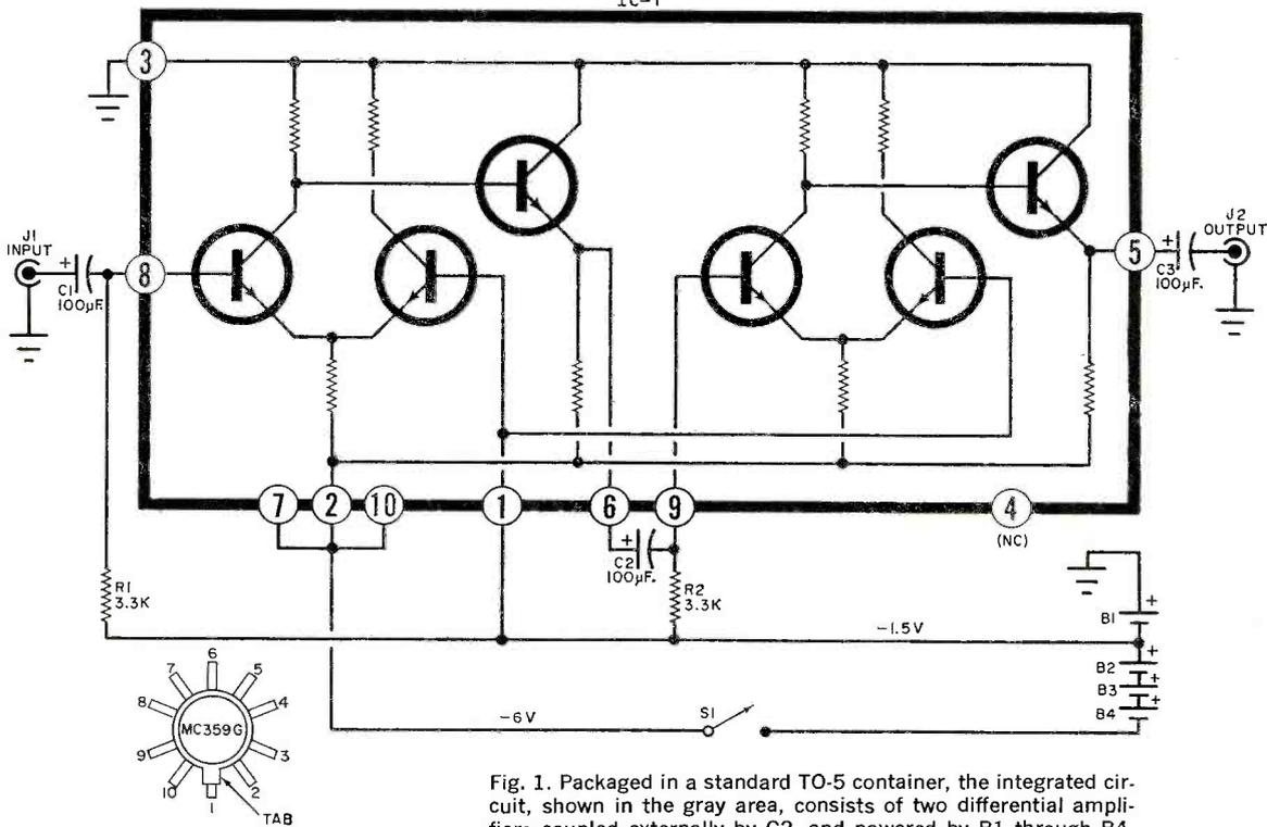
Fig. 1. Packaged in a standard TO-5 container, the integrated circuit, shown in the gray area, consists of two differential amplifiers coupled externally by C2, and powered by B1 through B4.
