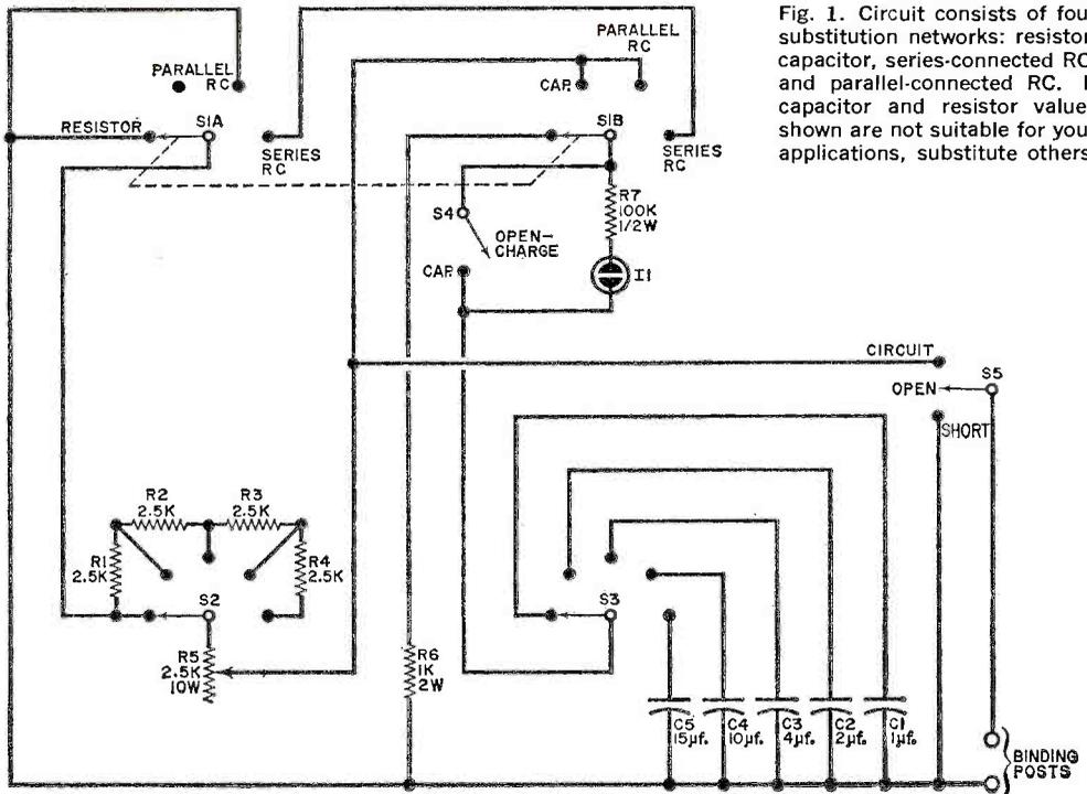
Fig. 1. Circuit consists of four substitution networks: resistor, capacitor, series-connected RC, and parallel-connected RC. If capacitor and resistor values shown are not suitable for your applications, substitute others.
