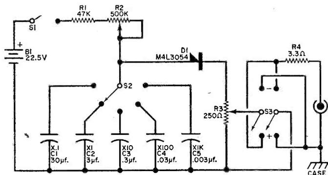
Fig. 3. Frequency depends upon battery voltage and amount of resistance and capacitance in the circuit. Combination of R1 and R2 provides an 11 to 1 spread within each of five decade ranges. Pulse repetition rate can be varied from 1 every 10 seconds to 11,000 each second.
