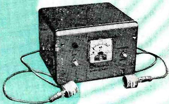
same chassis that detects this "sound." The "sound" is a 25-kc. note, which is about 10 kc. above most people's hearing range. In many respects the system is similar to the common light source and photocell alarm system, but with several
