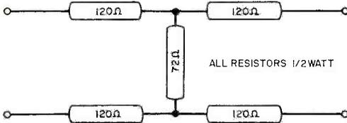
pad shown, the values given are for a 300-ohm line feeding into a TV set with a 300-ohm input. If the especially strong signals appear on one or two channels only, you can add a d.p.d.t. switching arrangement in the circuit to switch the pad in and out of the line as desired.
