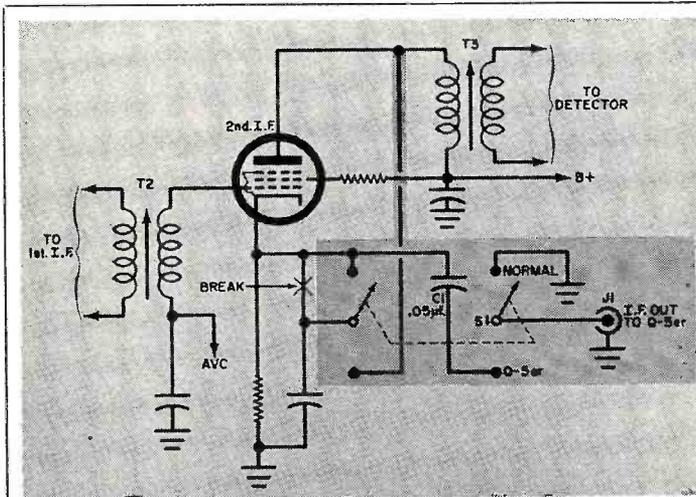
In the "Normal" position, the receiver operates as originally designed. In the "Q5-er" position, the output of the i.f. stage is bypassed to ground and the 455-kHz i.f. signal fed into the connection to the Q5-er.
