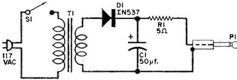
Optional power supply can be installed next to the motor if you use a large enough pie plate as a base, or you can mount it in a box. Construction and parts are not critical.
