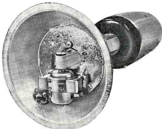
The small d.c. motor can run on flashlight batteries, but you may find it more convenient to assemble a small power supply.
