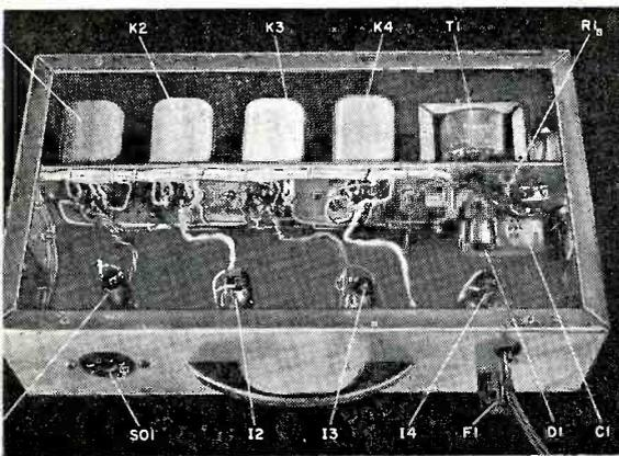
Fig. 2. Construction is simple. Another way to assemble the Reflexometer is to do away with the sub-chassis and mount the relays on top side of case.
