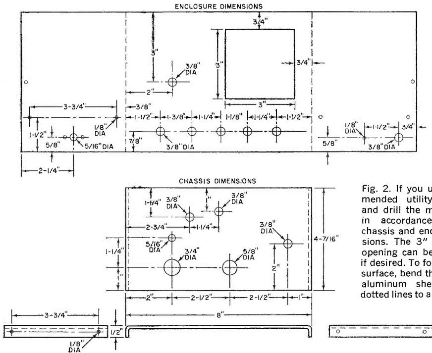
Fig. 2. If you use the recommended utility box, punch and drill the mounting holes in accordance with these chassis and enclosure dimensions. The 3" x 3" speaker opening can be made round, if desired. To form the chassis surface, bend the edges of the aluminum sheet along the dotted lines to an angle of 90°.
