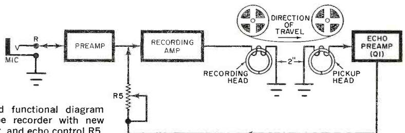
Fig. 1. This simplified functional diagram shows a modified tape recorder with new head, echo preamplifier, and echo control  $R5$ .
