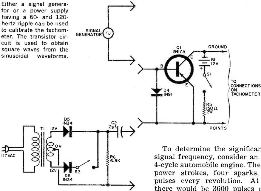
larity of the diodes and the external connection to the distributor.
