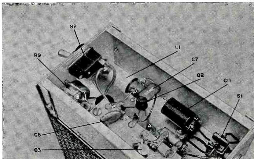
action can be controlled by changing the value of  $R5$ —reducing the value of this resistor should reduce the tendency toward regenerative oscillation. The receiver should show signs of regeneration with the antenna connected and the gain control turned “full-on.”
