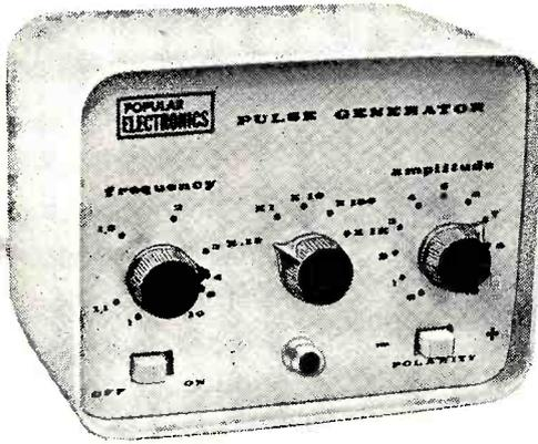
*Variable amplitude and frequency trigger for counting, testing, and experimenting*
