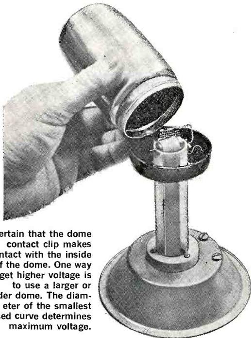
Be certain that the dome contact clip makes contact with the inside of the dome. One way to get higher voltage is to use a larger or rounder dome. The diameter of the smallest exposed curve determines maximum voltage.
