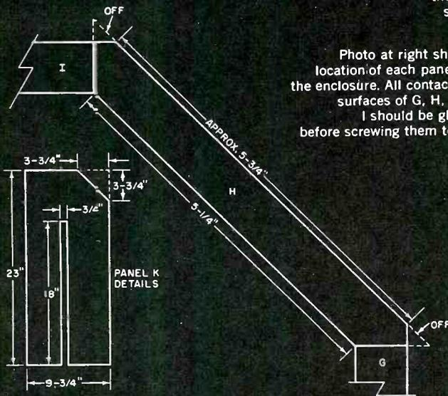
Photo at right shows location of each panel in the enclosure. All contacting surfaces of G, H, and I should be glued before screwing them to K.
