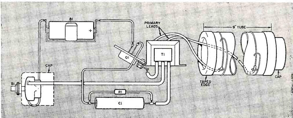
All components, including battery, fit into cardboard tube. Primary leads from *T1* pass through inside of tube to the outside, and are covered with foil. About 1" of space separates the 4"-wide electrodes.
