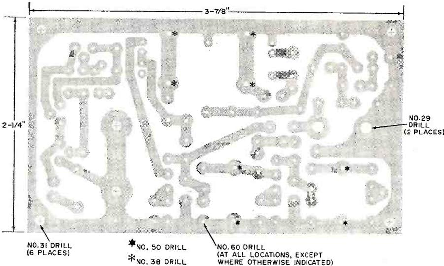
Copper foil side of homemade printed circuit board should have the outline shown in the 1:1 drawing above. Holes to pass wire leads are drilled with a #60 drill. All other holes are drilled to the sizes indicated.
