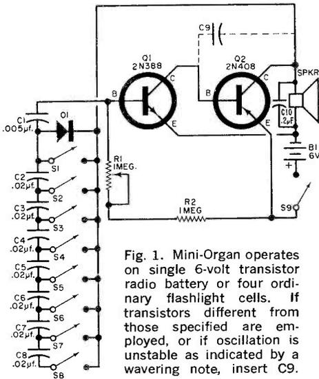
Fig. 1. Mini-Organ operates on single 6-volt transistor radio battery or four ordinary flashlight cells. If transistors different from those specified are employed, or if oscillation is unstable as indicated by a wavering note, insert *C9*.
