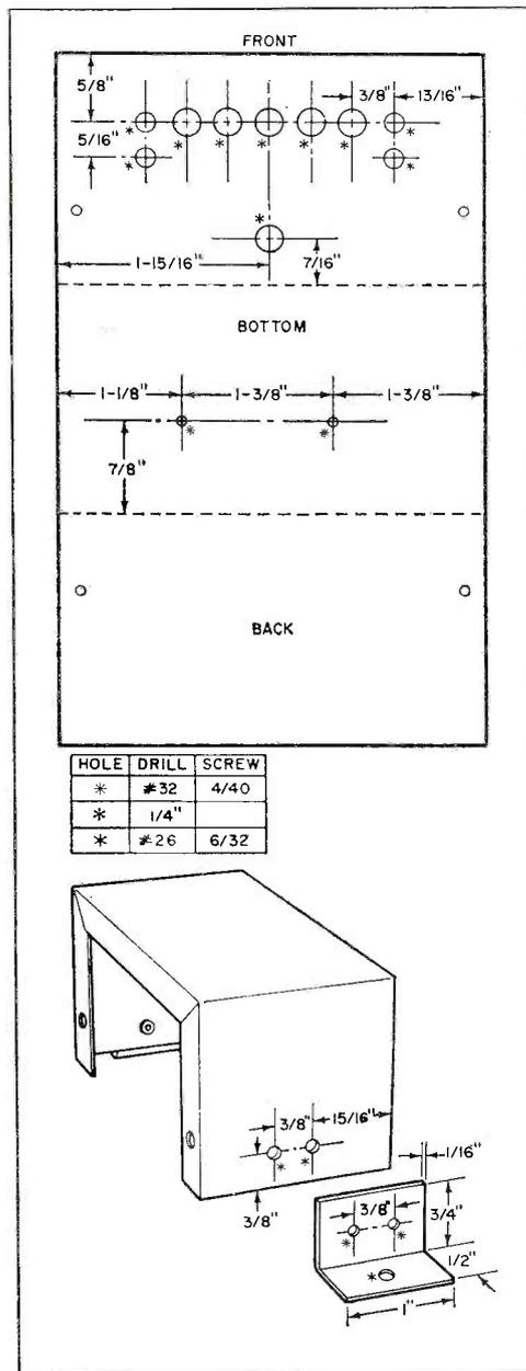
Location and size of holes may vary for different style of terminal strip. It's a good idea to lay out all parts before drilling any holes in the box.
