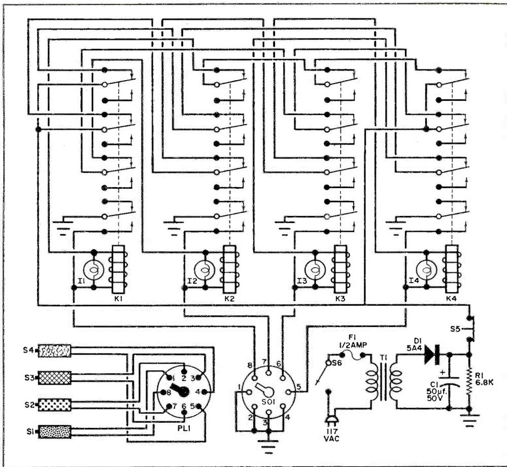
Fig. 1. Responders S1 to S4 can complete only one relay circuit at a time. The first switch closed latches its respective relay, lights its lamp, and disables the other relays until the circuit is reset.
