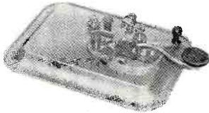
tions on the tray until you find a place where the clicks sound the loudest. You can also make louder sounds by increasing spring tension and contact gap, and by pressing harder.
