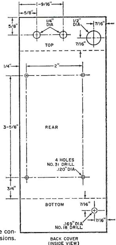
If you purchase an LMB aluminum box No. 139, you can duplicate construction of the receiver shown on the cover using these dimensions.
