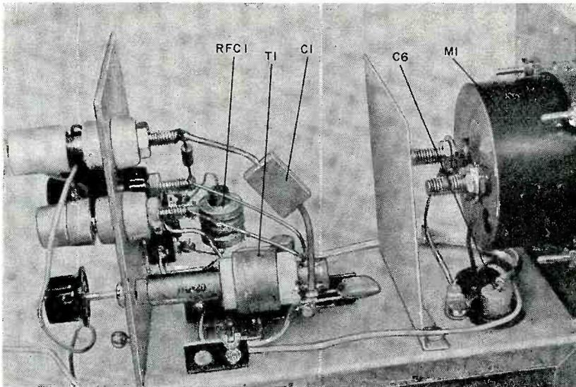
Note the aluminum shield that the author found necessary to add above the chassis to prevent feedback from the meter to the input circuitry surrounding *C1*. Coupling capacitor *C6* is mounted in a rubber or plastic grommet so that one lead is above the chassis, the other lead below it. Leads to the meter pass through another grommet.
