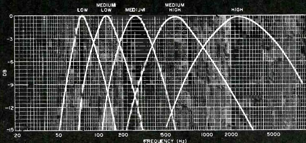
Fig. 1. These frequency response curves show the relative attenuation of each band of frequencies in the audio spectrum.
