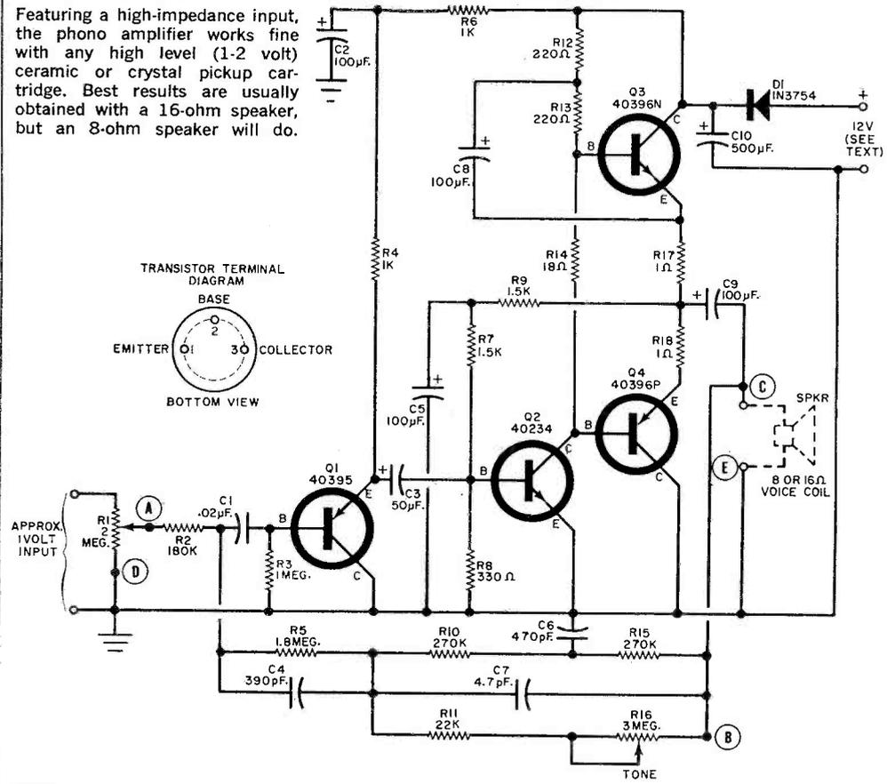
**How It Works.** The amplifier input from a phono cartridge is applied to the base of emitter follower *Q1* (as shown in the schematic diagram, above) through volume control *R1*, limiter resistor *R2*, and coupling capacitor *C1*. With *Q1* serving as an impedance-matching device, this transistor provides a high input impedance to the source and a low output impedance to driver *Q2*.
