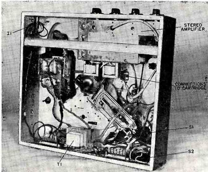
Solid-state stereo amplifier runs cool and is compact enough to fit into record changer base. Parts location is not critical, but adequate clearance for the changer mechanism must be provided. It's a good idea to run the changer through a cycle by hand in order to check clearance requirements.
