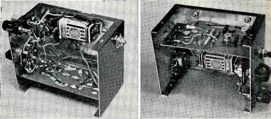
Fig. 3. The bottom cover has been removed to show how printed circuit board is mounted in the cabinet. In view at left, the unit is on its left side. In view at right, the unit is turned on its right side.
