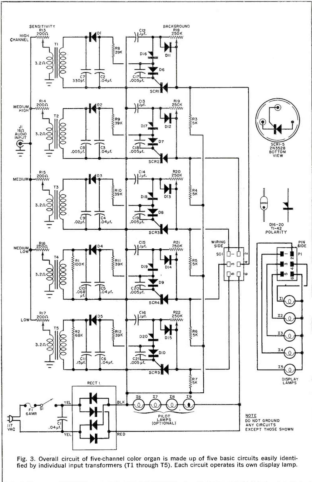
Fig. 3. Overall circuit of five-channel color organ is made up of five basic circuits easily identified by individual input transformers (T1 through T5). Each circuit operates its own display lamp.
