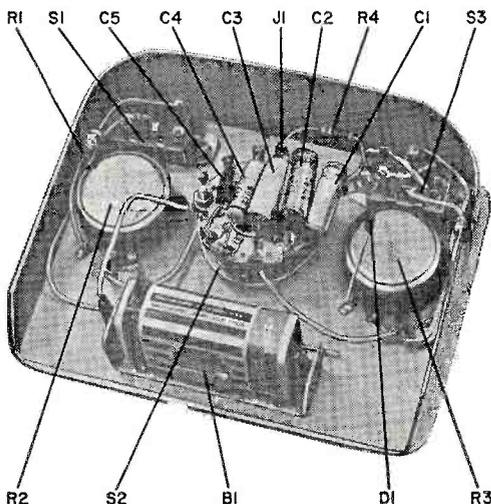
Only electrical connection to the chassis is at J1. The unused side of S2 conveniently serves as a terminal strip for the common capacitor leads.
