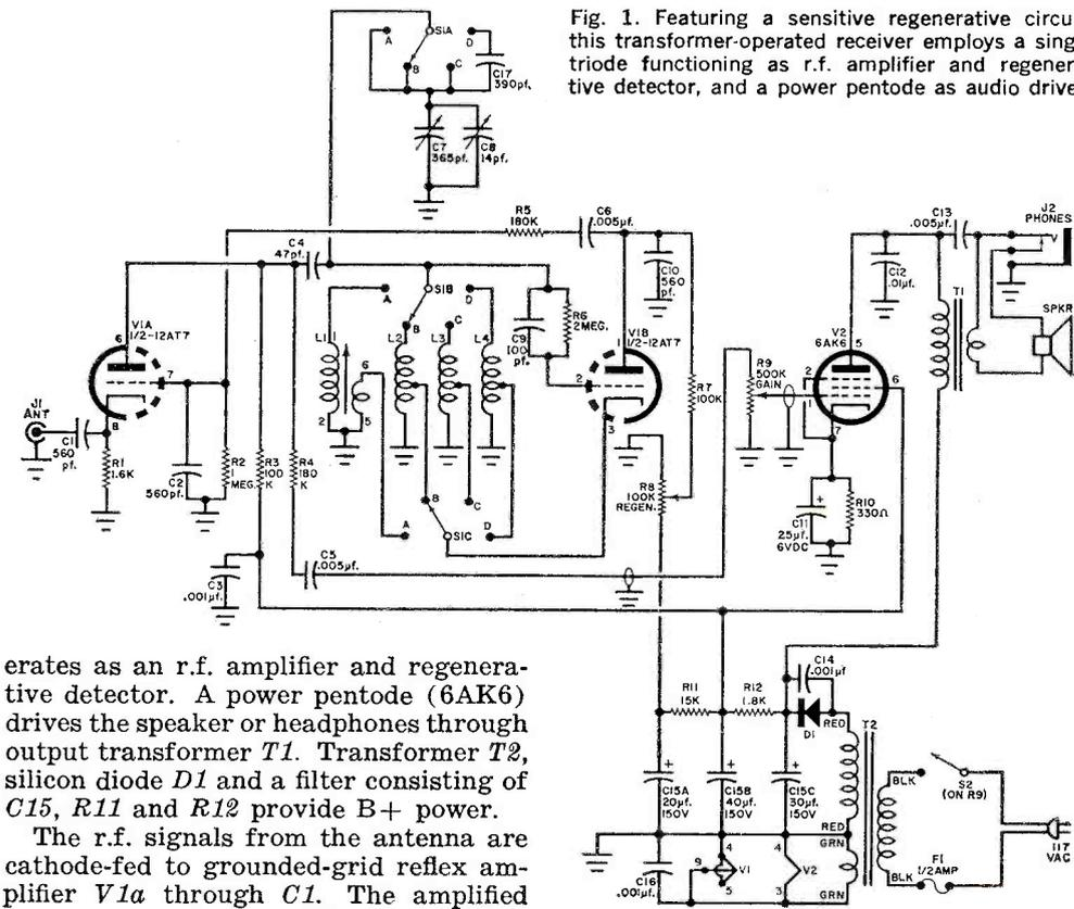
erates as an r.f. amplifier and regenerative detector. A power pentode (6AK6) drives the speaker or headphones through output transformer *T1*. Transformer *T2*, silicon diode *D1* and a filter consisting of *C15*, *R11* and *R12* provide B+ power.
