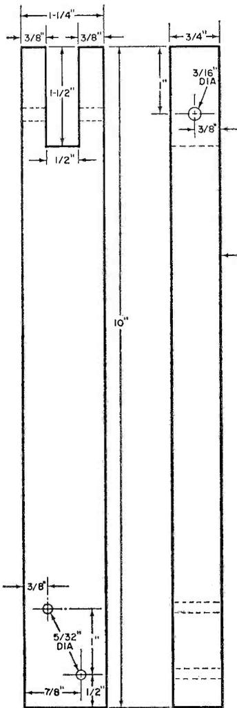
Fig. 3. These are the dimensions of the wooden support and crossarm that were used in the author's model. If desired,  $\frac{1}{4}$ " hardwood can be substituted for the aluminum photocell bracket.
