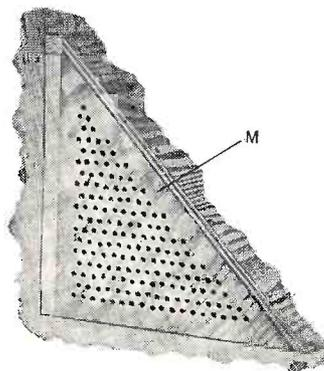
Cage side cover is held in place by 2 1/2"-long screws fed into front and bottom of cabinet from outside, and by 1 1/4" screws through piece L.
