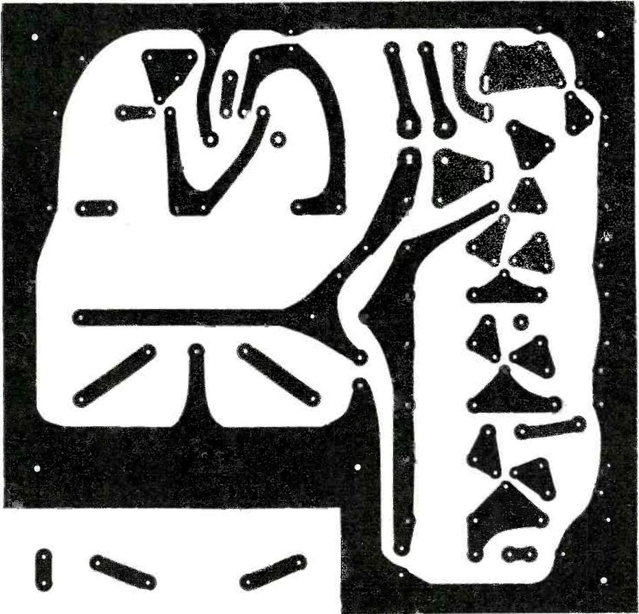
Fig. 2. Actual size photo of conductor side of printed circuit board. Components can be mounted on any type of chassis, but care should be exercised to prevent stray leakage, or coupling.
