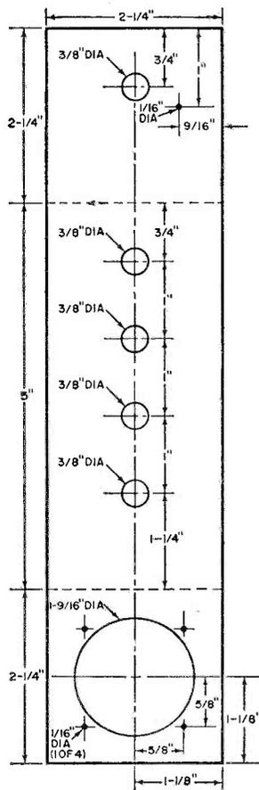
Fig. 3. Type of box used and layout are not critical, but make the four bolt holes for the meter a bit oversized to permit rotating the meter if necessary to keep it straight. If you have enough room on your transmitter, you can mount all the parts directly on it, and thus do away with the cable and the box.
