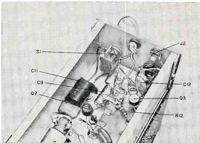
This view is toward the rear of the chassis. Jack J1 is under J2—one jack being regular phone size, the other a miniature. Switch S1 controls the time constant of the output circuit so that a chart recorder can read a rough average of the background noise—not individual noise bursts. Circuit values given are suitable for use with a Rustrak low-cost chart recorder such as the one shown on the cover.
