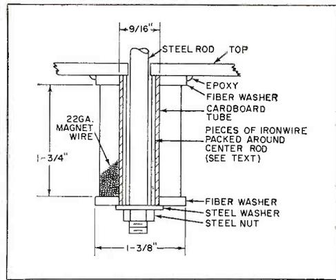
Fig. 4. Construct coil forms as shown. Each coil takes about 80 feet of No. 22 enamel-coated wire. A 1/2-pound spool should be enough for both coils.
