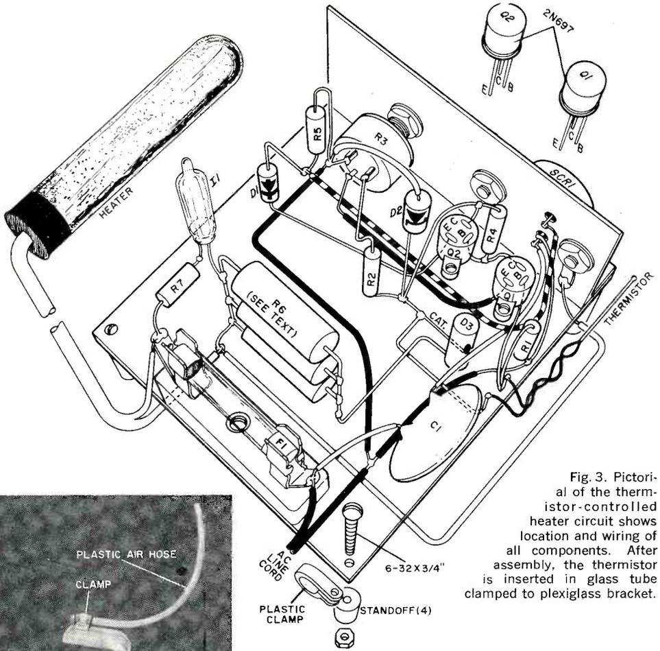
Fig. 3. Pictorial of the thermistor-controlled heater circuit shows location and wiring of all components. After assembly, the thermistor is inserted in glass tube clamped to plexiglass bracket.
