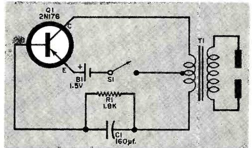
Unusual application of filament transformer steps up Q1's pulse output to excite the electrodes—and any one who happens to be holding on to them.
