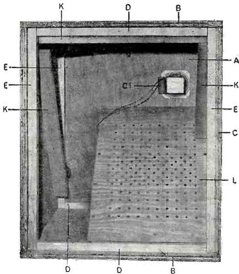
Location of tweeter is not critical. If you want to dispense with testing procedure, drill 80 1/4"-diameter holes (8 rows of 10) in woofer compartment.
