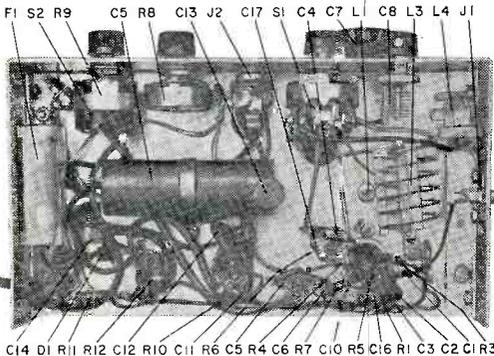
Fig. 7. Layout is simple and uncramped. Plastic fuse cover prevents accidental contact with a.c. line if you're working on the receiver with power on.
