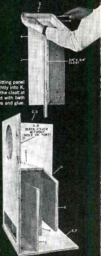
After fitting panel J tightly into K, secure the cleat at the joint with both screws and glue.
