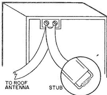
length of lead-in wire across the set's antenna terminals, letting the free end hang loosely toward the floor. Check to see if there's an
