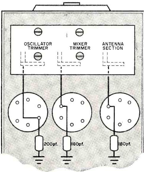
This combination wiring/pictorial diagram shows the exact wiring position of the three silver mica fixed capacitors. Placing these capacitors in the circuit bandspreads the receiver's tuning range.
