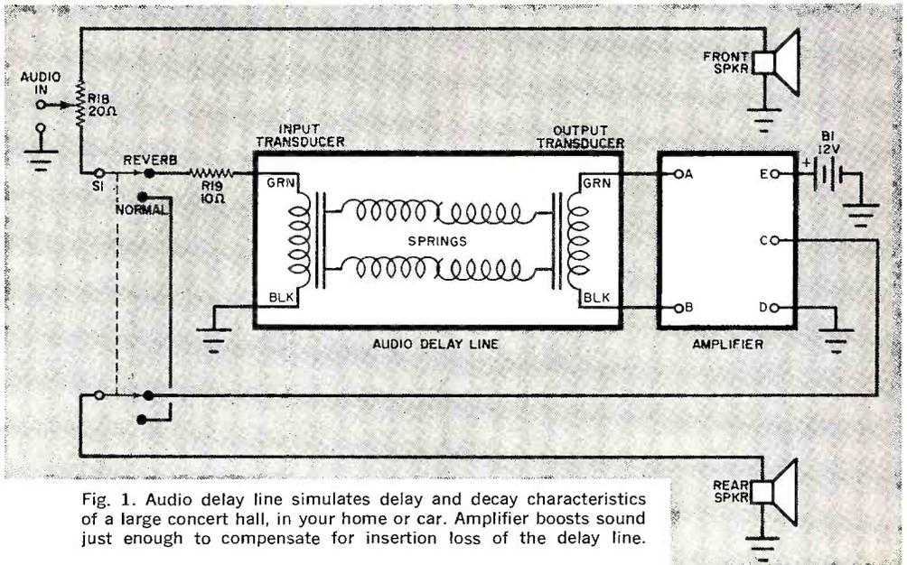
Fig. 1. Audio delay line simulates delay and decay characteristics of a large concert hall, in your home or car. Amplifier boosts sound just enough to compensate for insertion loss of the delay line.
