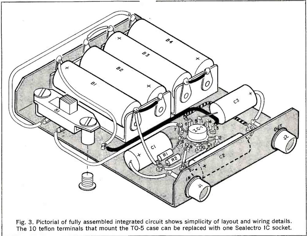
Fig. 3. Pictorial of fully assembled integrated circuit shows simplicity of layout and wiring details. The 10 teflon terminals that mount the TO-5 case can be replaced with one Seaelectro IC socket.
