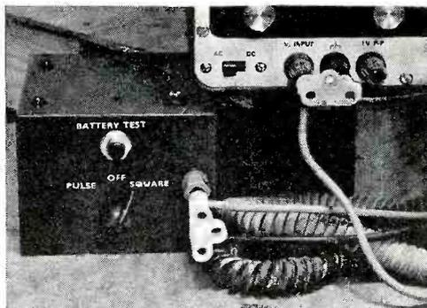
(1) Set selector switch to *SQUARE* and connect a jumper between Q3's base and ground to disable the multivibrator.
