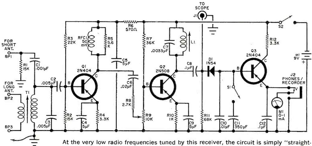
At the very low radio frequencies tuned by this receiver, the circuit is simply "straight-thru." Regeneration is not desired, and when T1 and L1 are resonated to the same frequency, R9 must be turned down to curb feedback. Output jack J1 is optional if the user wants to "look" at some of the strange VLF signals between 25 and 35 kHz.
