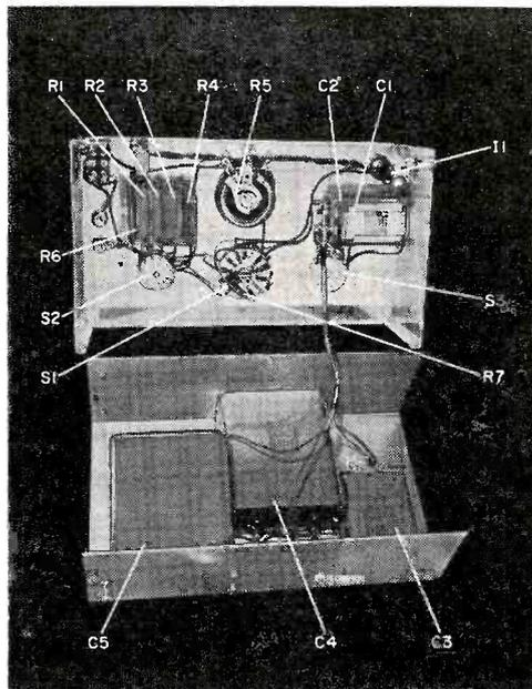
Fig. 2. Use of heavy-duty components puts this substitution box in a class all by itself. You need have no fear of burning out the 10-watt resistors.
