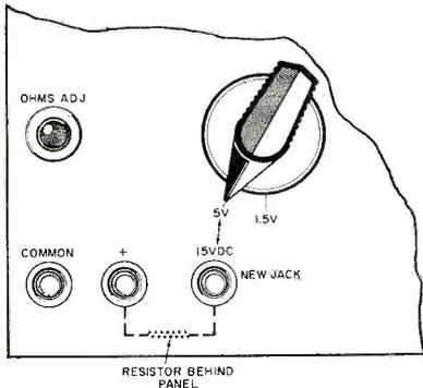
to "5 V," and the d.c. test lead in the new jack, a full-scale deflection will indicate 15 volts. With the d.c. scale essentially linear, a mid-scale reading will indicate 7.5 volts. Inscribe "15 VDC" on the front panel directly
