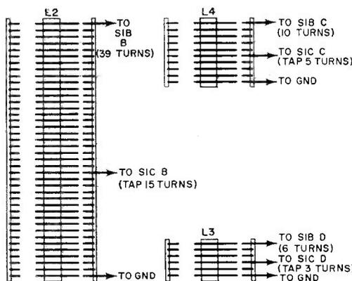
ponents and circuit wiring. Be sure to dress the 6.3-volt filament wires close to the chassis while keeping them away from the coils. Keep all wiring as direct and as short as possible.
