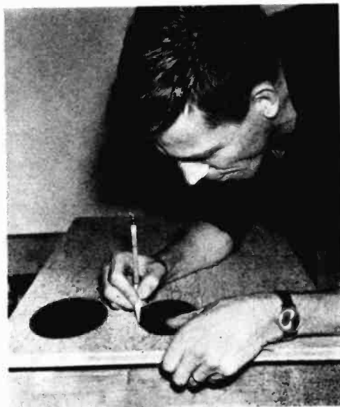
Fig. 4. Templates that are cut from heavy paper or cardboard greatly facilitate the laying out of speaker cutout lines on the front board. A different template is needed for each size of speaker used.
