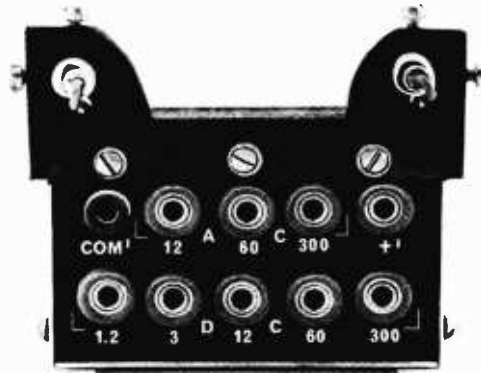
Fig. 3. Mount the jacks for d.c. voltage in lower portion of a piece of Bakelite; jacks for COM', +', and a.c. voltage can be mounted in upper portion.
