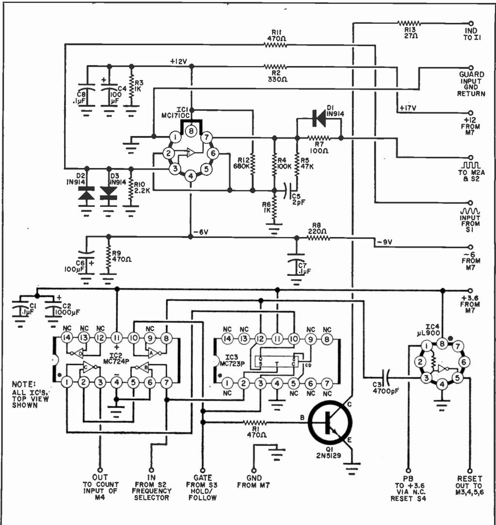
Fig. 1. The comparator module actually contains three separate circuits: input signal comparator (IC1), signal-time base synchronizing circuit (IC2 and IC3), and automatic reset generator IC4.
