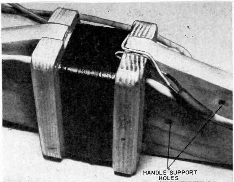
evenly and firmly as possible and avoid kinking the wire. When the winding is finished, protect it with a couple of layers of plastic electrical tape. Be sure that you can identify each end of the coil.
