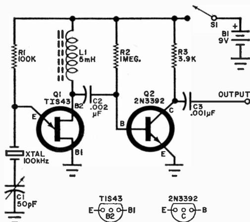
Although simple, this oscillator is very stable and will remain on the frequency for a long time.
