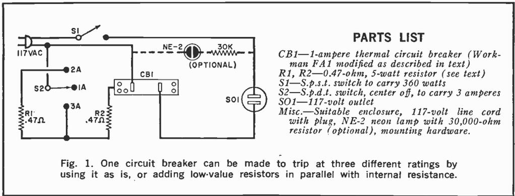
tance of the thermal portion of the breaker is 0.96 ohm. To increase its current carrying capability, a one-ohm resistor can be connected across the resistor part of the breaker. To increase the current rating even farther, a  $\frac{1}{2}$ -ohm resistor can be connected across this portion.
