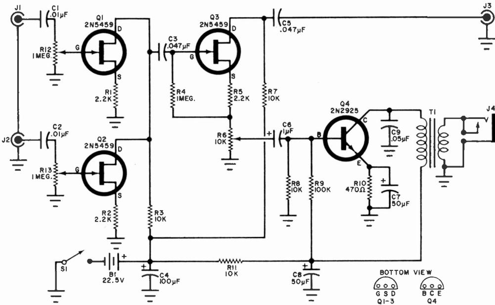
After preamplification and mixing take place in Q1 and Q2, signal is fed to output through Q3; Q4 is monitor amp.
