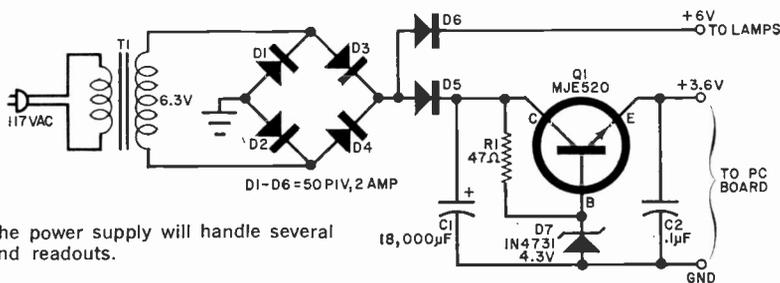
Fig. 8. The power supply will handle several DCU's and readouts.
