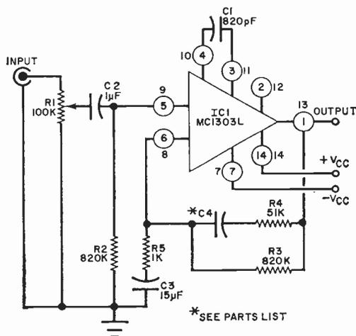
Fig. 2. This NAB tape-head equalized preamp can be preset for either 3¾ in./s or 7½ in./s depending on value selected for C4 (can be switch selected).
