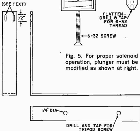
Fig. 6. Lengths of L bracket legs must be calculated for your particular camera; do not omit slots.
