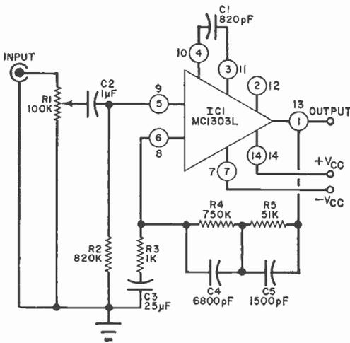
Fig. 3. This circuit is used for RIAA equalization for magnetic phono playback. A slight change in R4 value can be made (see text) without doing harm.
