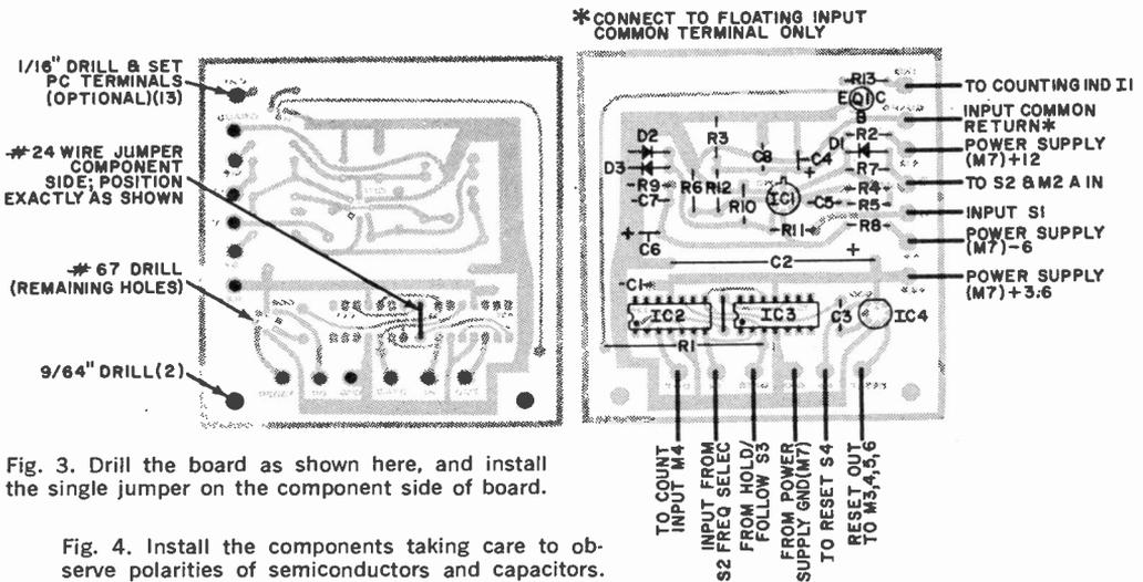
Fig. 3. Drill the board as shown here, and install the single jumper on the component side of board.
