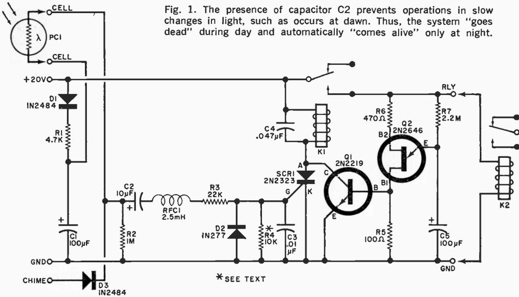
Fig. 1. The presence of capacitor C2 prevents operations in slow changes in light, such as occurs at dawn. Thus, the system "goes dead" during day and automatically "comes alive" only at night.
