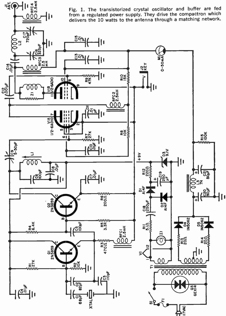
Fig. 1. The transistorized crystal oscillator and buffer are fed from a regulated power supply. They drive the compactron which delivers the 10 watts to the antenna through a matching network.
