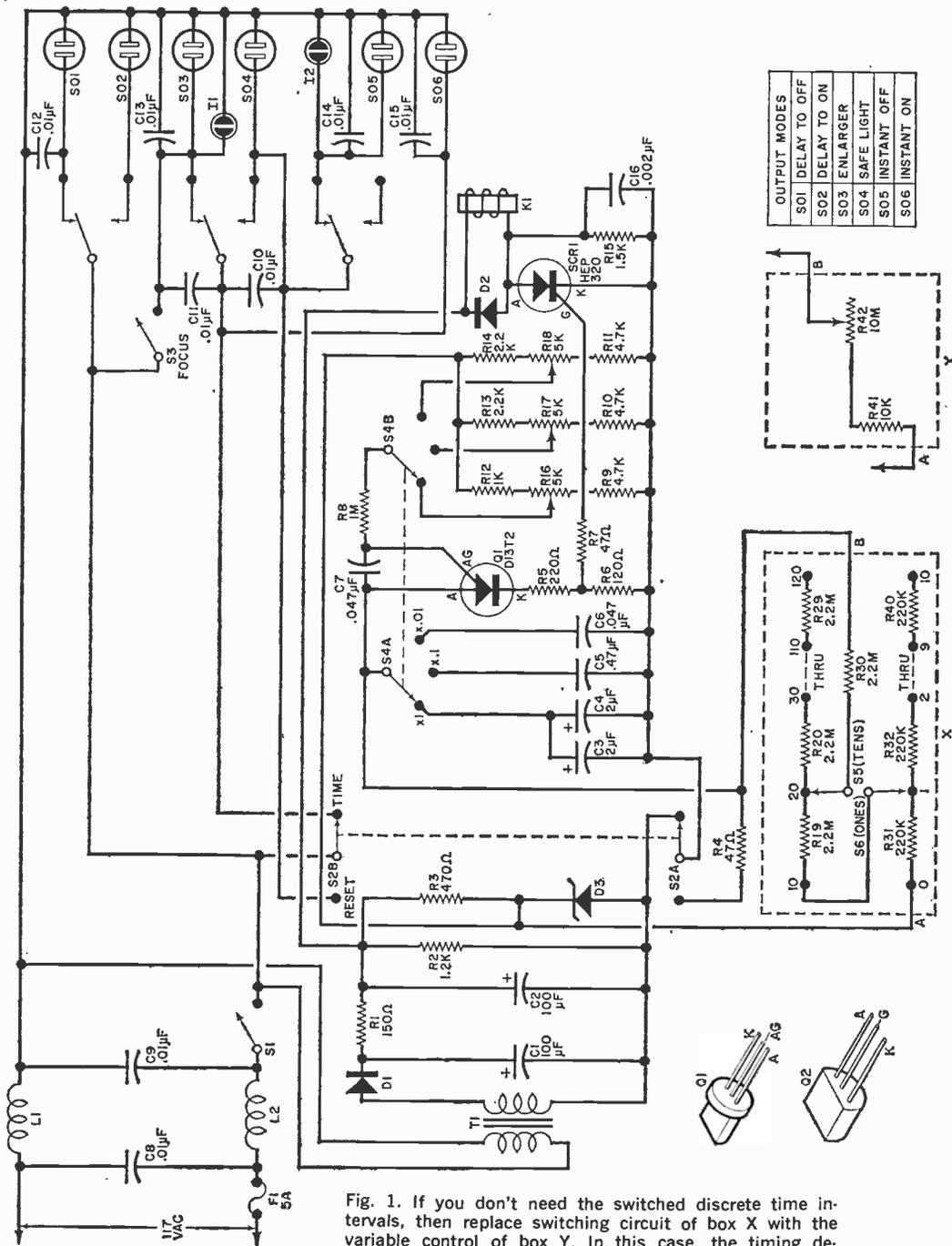
Fig. 1. If you don't need the switched discrete time intervals, then replace switching circuit of box X with the variable control of box Y. In this case, the timing depends on the accurate calibration of potentiometer R42.
