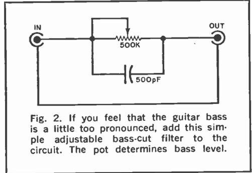
Fig. 2. If you feel that the guitar bass is a little too pronounced, add this simple adjustable bass-cut filter to the circuit. The pot determines bass level.
