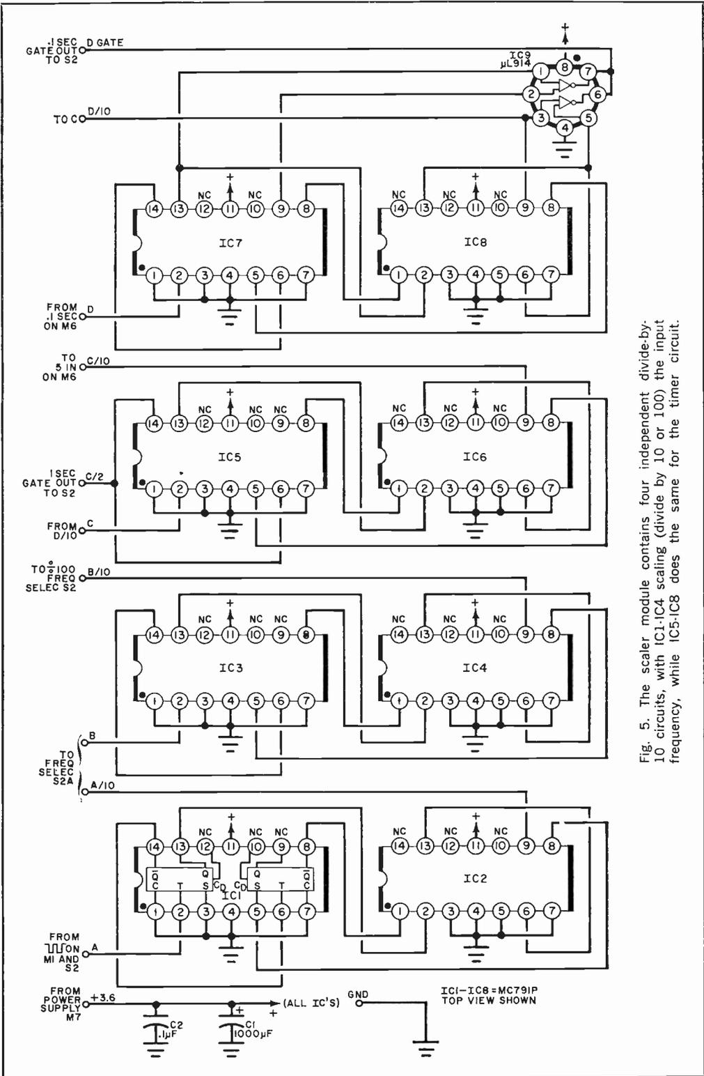
Fig. 5. The scaler module contains four independent divide-by-10 circuits, with IC1-IC4 scaling (divide by 10 or 100) the input frequency, while IC5-IC8 does the same for the timer circuit.
