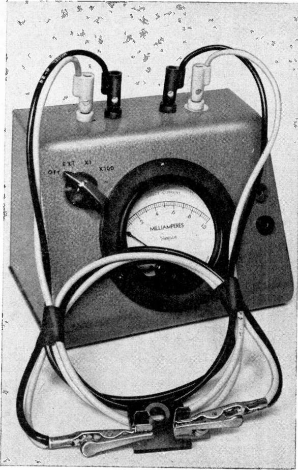
**T**HE UBIQUITOUS VOM is one of the handiest pieces of test equipment available to the electronics experimenter. Although useful in a thousand different ways, there are times when a VOM can be the cause of damage to the equipment being tested—by applying excessive current to low-resistance devices, for instance. This means that you can't use a conventional VOM to test D'Arsonval meter movements, meter fuses, or transistors, to name a few items that are current sensitive.
