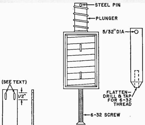
Fig. 5. For proper solenoid operation, plunger must be modified as shown at right.
