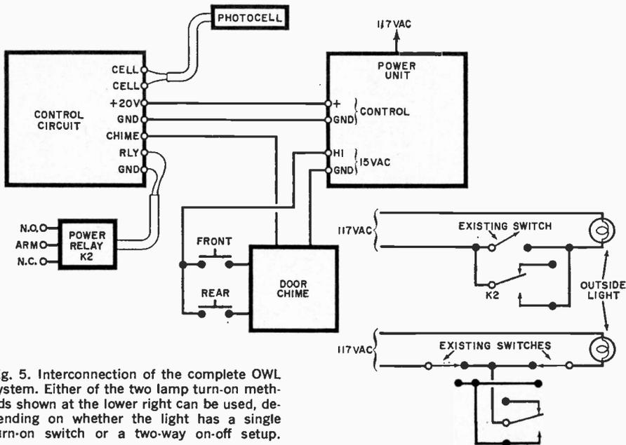
Fig. 5. Interconnection of the complete OWL system. Either of the two lamp turn-on methods shown at the lower right can be used, depending on whether the light has a single turn-on switch or a two-way on-off setup.
