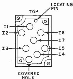
Fig. 6. Rear view of the commercial display unit showing the location of the seven segment-illuminator bulbs.
