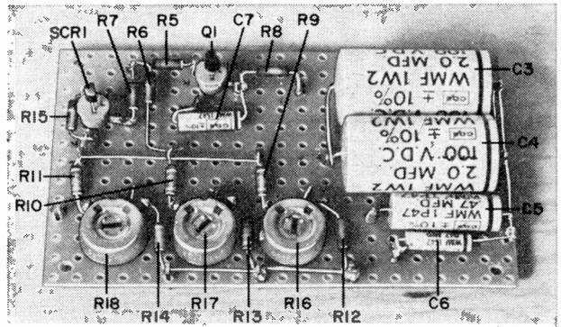
If you have built the single-range 2-to-60-second timer, a special scale for  $R42$  must be prepared. Using a pointer knob, set  $R42$  at about 85 to 90% of full resistance and adjust  $R16$  for 60 seconds. Mark the position for  $R42$ . Then by trial and error, locate and mark the settings of  $R42$  for 50, 40, 30, 20 and 10 seconds. These major divisions can then be subdivided into discrete second steps and marked on the front panel.
