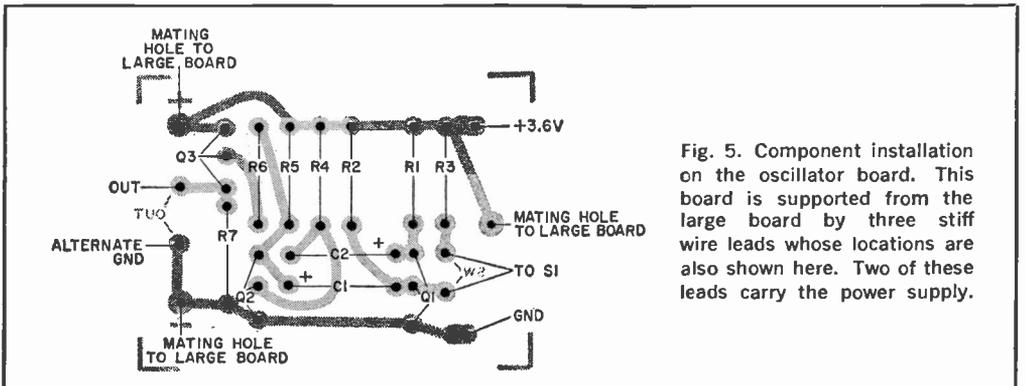
Fig. 5. Component installation on the oscillator board. This board is supported from the large board by three stiff wire leads whose locations are also shown here. Two of these leads carry the power supply.
