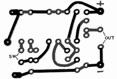
Fig. 4. Actual-size foil pattern for the oscillator.
