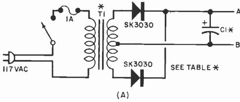
**M**ANY READERS have asked us to print a circuit design for a power supply that would be simple yet would provide the unusual d.c. voltages that may be required in experiments and project constructions involving semi-conductors. In answer to these requests, we suggest a circuit given in the *RCA Solid-State Hobby Circuits Manual*. (The handbook is available at most electronics parts distributors for \$1.75.)
