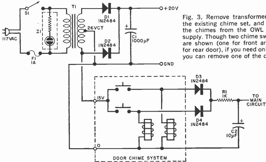
Fig. 3. Remove transformer from the existing chime set, and power the chimes from the OWL power supply. Though two chime switches are shown (one for front and one for rear door), if you need only one, you can remove one of the diodes.
