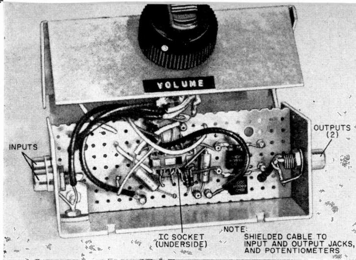
The IC preamplifier can be fabricated on perf board. A 14-lead in-line socket may be used to save possible damage to IC while soldering it into the circuit. Use shielded leads for the input and output, and to (coaxial) potentiometers.
