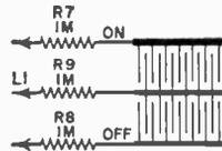
Prepare an etched board similar to above for use as a moisture detector or touch panel wall plate. For moisture detection, *L1* gives a positive source.
