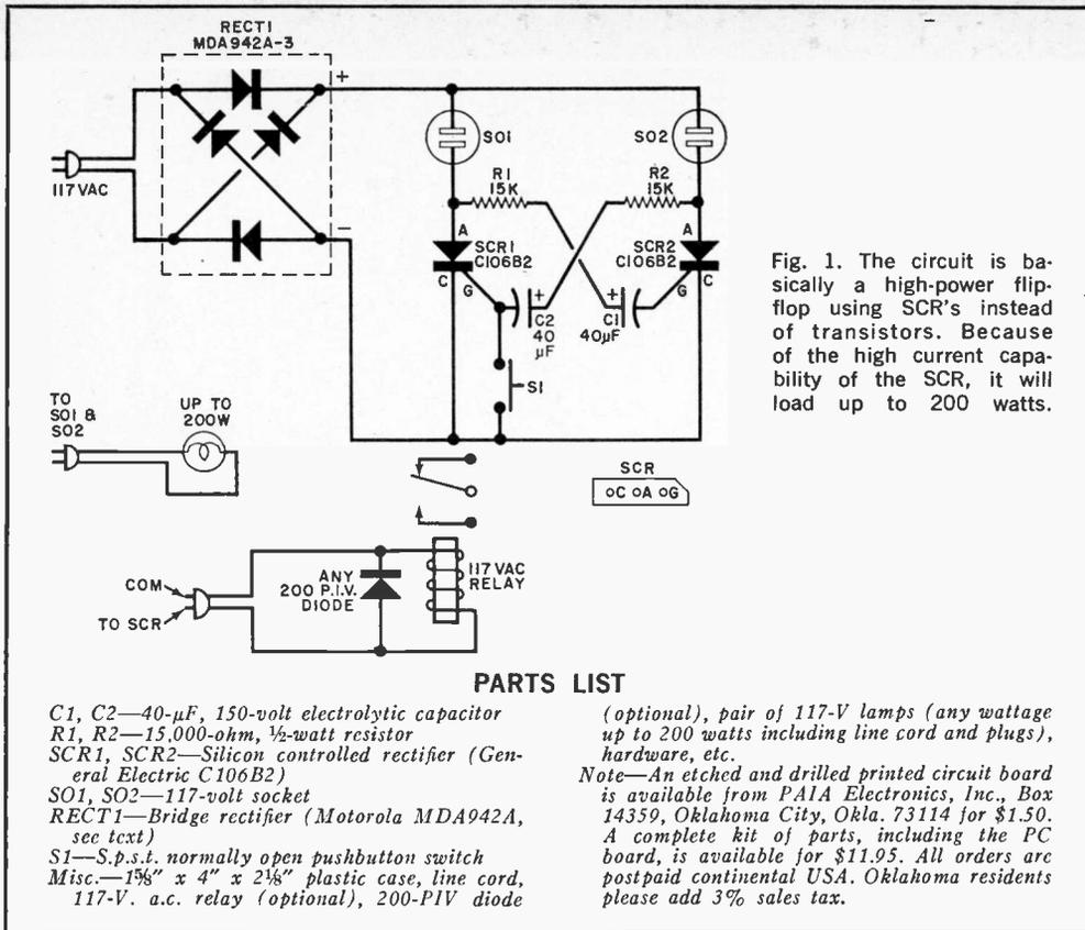
a.c. line power is used in this device, be very careful of component polarities and short circuits, as a wrong connection can easily destroy components or vaporize the conducting path on the circuit board.
