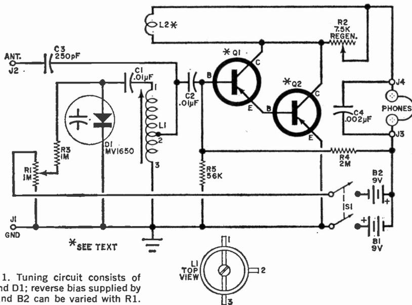
Fig. 1. Tuning circuit consists of L1 and D1; reverse bias supplied by B1 and B2 can be varied with R1.
