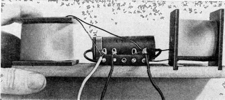
wire out through the remaining holes in the coil forms. Scrape away about  $\frac{1}{2}$ " of the insulating enamel from the free ends of the coil windings.
