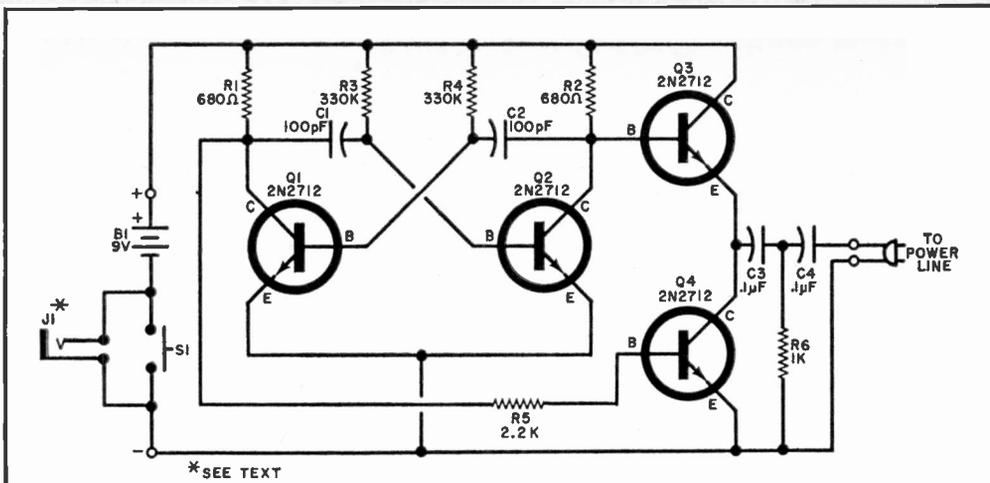
Fig. 1. Power is applied only when S1 (or J1) is closed. The multivibrator then generates a high-frequency audio signal which is passed down the power line to the receiver.
