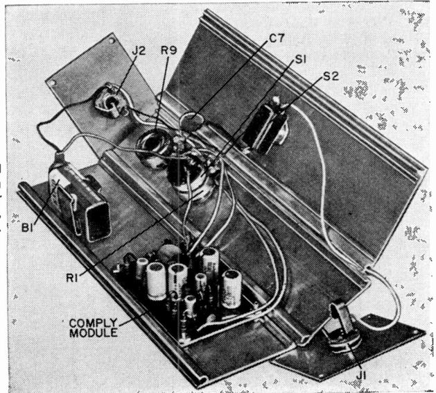
**Construction.** Packaging the compressor can be accomplished in one of two ways. The first is to mount the entire subsystem in a very strong metal box with the footswitch (S2) on the top and the other controls and input-output jacks on either the sides or ends. Since this scheme requires an exceptionally strong metal box, you may prefer the second
