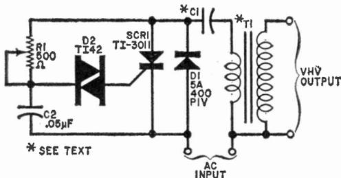
By driving the very-high-voltage power supply with a variable-voltage transformer, output voltage can be made to vary above and below 10,000 volts.
