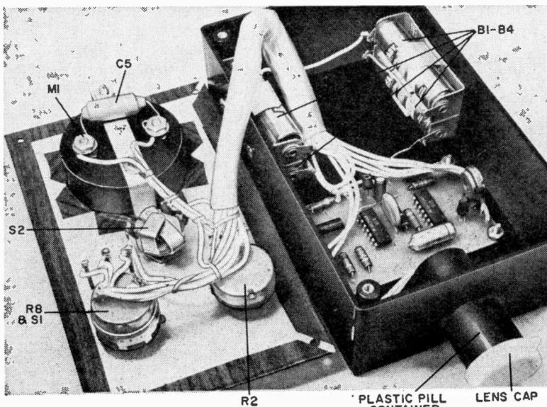
The wiring between the PC board and the front panel can be made neat by passing it through a piece of plastic tubing.
