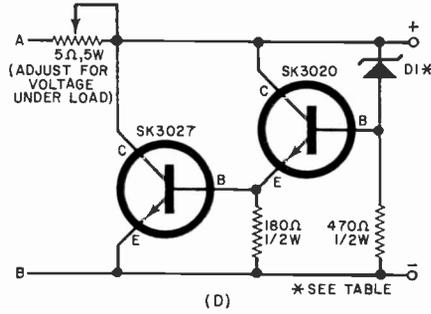
plies delivering 15 volts or less, while that at B is for 3- to 35-volt outputs. Below 15 volts, take your pick—two less rectifier diodes are required for circuit A.
