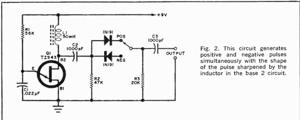
Fig. 2. This circuit generates positive and negative pulses simultaneously with the shape of the pulse sharpened by the inductor in the base 2 circuit.
