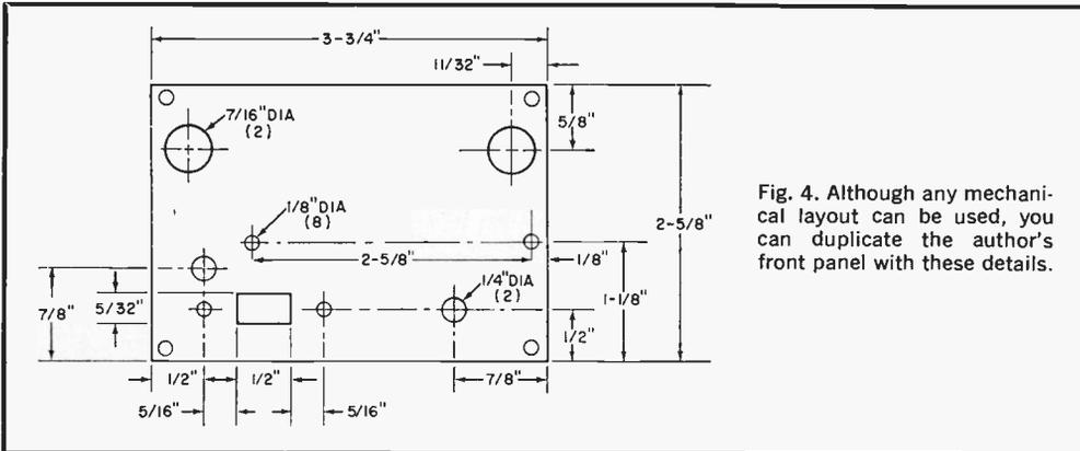
Fig. 4. Although any mechanical layout can be used, you can duplicate the author's front panel with these details.
