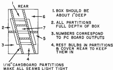
Fig. 7. You can make your own readout by following construction information shown here.
