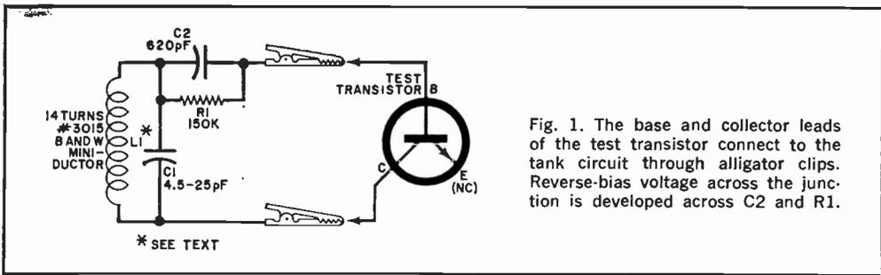
Fig. 1. The base and collector leads of the test transistor connect to the tank circuit through alligator clips. Reverse-bias voltage across the junction is developed across C2 and R1.
