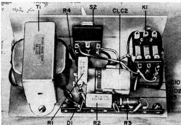
Fig. 3. Component mounting of the power supply and relay panel. Insulate metal case of dual capacitor C1-C2 by wrapping it in plastic tape before inserting the capacitor in its mounting clip. A terminal strip supports small components.
