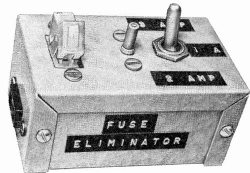
ing, it has one definite current rating. In working with instruments and equipment of different wattage ratings, you may be too far over or under the breaker rating. By adding a couple of low-cost resistors and a switch, you can now make a multi-current circuit breaker that can be preset for several ratings.
