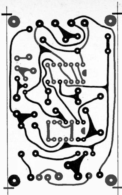
Fig. 2. Actual size printed-board foil pattern for the Op-Tach. Note the semi-circular end identifiers for the IC's.
