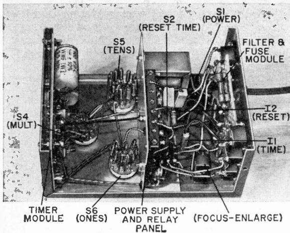
Fig. 2. A metal chassis is suggested for the timer to avoid picking up stray electrical noise which may cause erratic timing. The power supply and relay panel is secured to the main chassis by mounting hardware for switch S2. Other two boards are mounted on four stand-off terminals.
