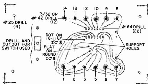
Fig. 7. Parts layout for the socket-contact board. Note the three support holes for oscillator board.
