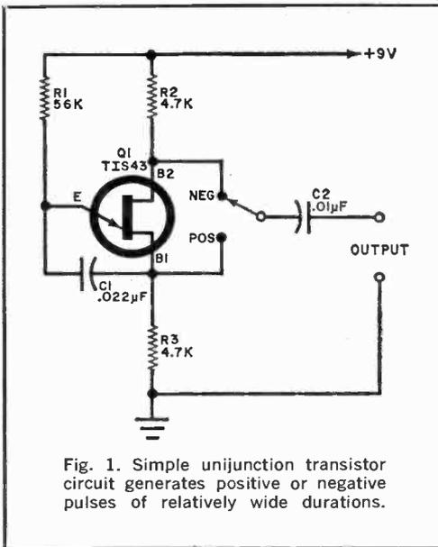
Fig. 1. Simple unijunction transistor circuit generates positive or negative pulses of relatively wide durations.
