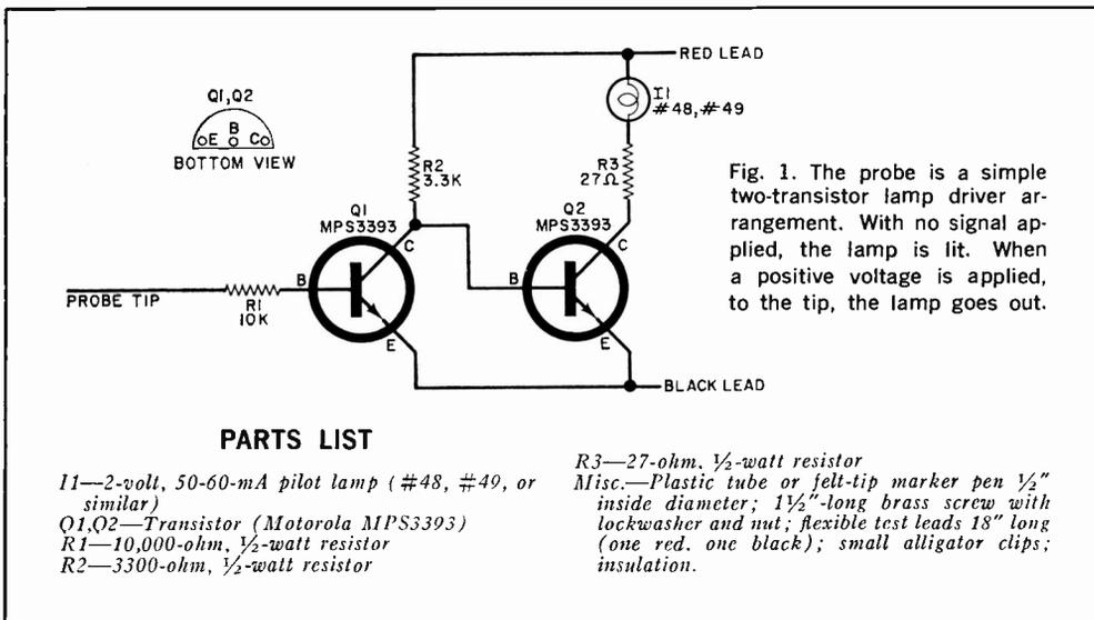
Fig. 1. The probe is a simple two-transistor lamp driver arrangement. With no signal applied, the lamp is lit. When a positive voltage is applied, to the tip, the lamp goes out.
