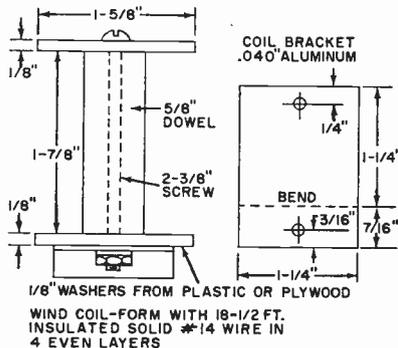
Fig. 4. Construction data for LI. Plastic tape can be wound over coil to keep it from unravelling during mounting.
