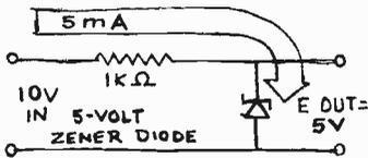
Thus, the same current-voltage relationship as in the voltage divider network exists when the zener diode is substituted and a 10-volt potential is applied to the input.
