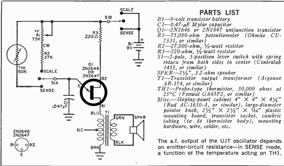
bottom of the chassis. The output transformer *T1* and the loudspeaker are on the other half of the cabinet. The remainder of the components are assembled on a small piece of plastic mounted on L brackets within the cabinet. The dial knob used for *R1* should be large, with a distinct pointer, and the calibration marks can be either numerical (in degrees F) or in Braille.
