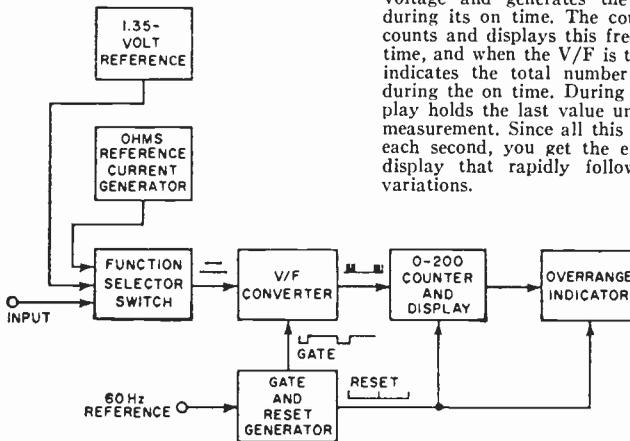
converter. This is a current-driven unijunction oscillator whose output frequency is proportional to the input voltage. Unlike industrial V/F converters, this one runs "open loop" and relies on calibration and inherent linearity rather than on complex and expensive feedback schemes for accuracy. Linearity, range, and resolution are more than adequate for the one-part-in-200 digital display used.
