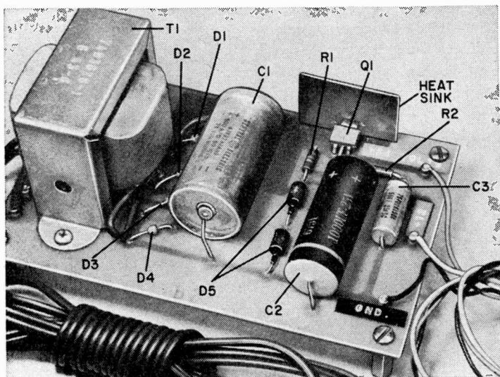
If you do not have a 24-volt zener, use a pair of 12-volt units in series as shown here. You must break the foil that shorts one diode connection.
