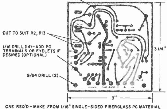
than #67 for the IC mounting holes. Optional eyelets or PC terminals can be added where indicated.
