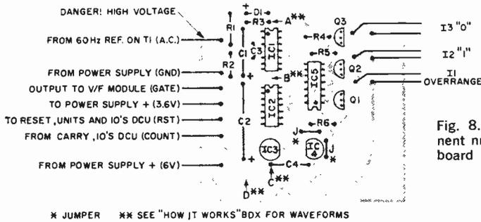
Fig. 8. Double and triple check component numbers, values, and orientation on board both before and after soldering.
