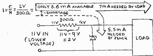
This leaves only 2 volts, dropped across the source resistor, to drive the current through the resistor. As a result, current drops to about 6.67 mA.
