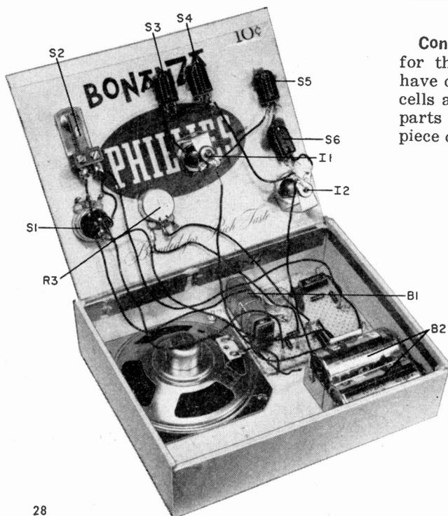
**Construction.** Many of the parts needed for the Gadget Box you will probably have on hand. Except for the speaker, D cells and holder, lamps, and controls, all parts can be mounted on a 3"-square piece of perforated board, using flea clips (Continued on page 93)
