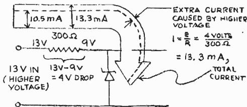
As you can see, the current through the diode jumps to 13.3 mA. Back to the
