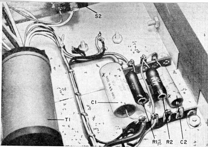
Resistors and capacitors are mounted between two terminal strips. Note how a wire harness makes for a clean, neat internal arrangement. This photo also shows the two isolated metal chassis and the method of wiring the power transistors. Both the emitter and base connections are soldered direct to the transistor leads; the collector connection is made to a solder lug under the collector (and case) mounting hardware.
