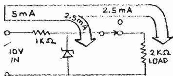
The reduction in current through the zener diode has little or no effect on it (up to a certain point), and the diode maintains a constant 5-volt output. As a result, the 2000-ohm load has 5 volts across it. Because the load is a resistor (it can be any other type of load for that matter), it cannot ignore Ohm's law, so it draws current:  $I_{load} = E/R = 5/2000 = 2.5$  mA.
