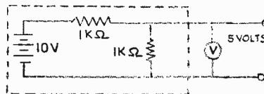
With the switch open and the load disconnected, the output is 5 volts with 5 mA in the output resistor. Closing the switch puts the 2000-ohm load in parallel with the output resistor so that the 6 mA now drawn from the source divides: 4 mA through the output resistor and 2 mA through the load resistor.
