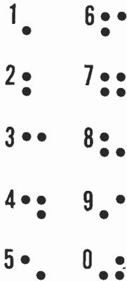
Braille numbers, in various combinations, can be embossed on front panel for use by a blind person.
