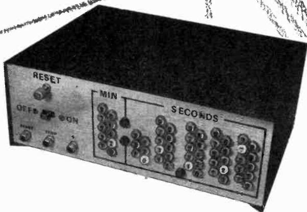
**T**HE AVAILABILITY OF LOW-COST decimal-readout counting units has created an entirely new "ball park" of experimentation for the advanced electronics hobbyist. This new area is digital-readout instruments and we will be publishing several articles on such projects in the issues to come. The first is the "Sports Timer," a real-time clock, described here.
