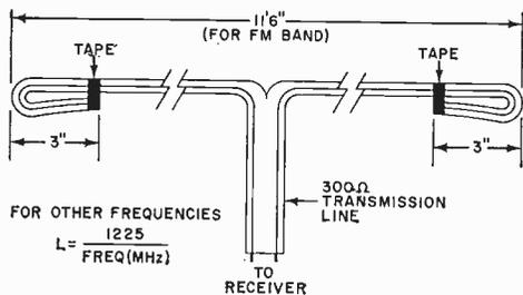
For 88-108-MHz FM band, the extended double Zepp is made of 11 feet 6 inches of split 300-ohm line.
