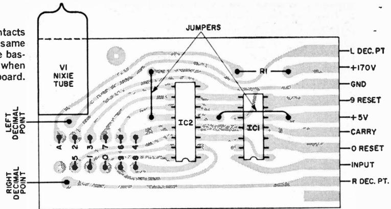
or used with a PC-board edge connector. After mounting and soldering *IC1* in place, install the second jumper.
