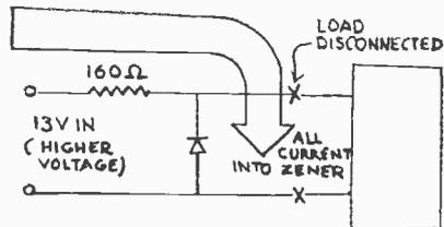
Fortunately, Ohm's law shows that a 1/4-watt resistor will adequately handle the current, and multiplying 9 volts by 13.8 mA tells us that our 250-milliwatt zener is dissipating only 124.2 milliwatts. Now we have a regulator circuit we can build with confidence.
