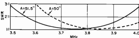
Length of side A depends on coverage desired and determines the standing wave ratio for the dipole.
