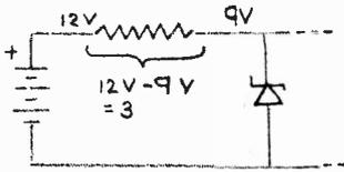
The result is that 3 volts is dropped across the resistor. Ohm's law now tells us the value of the resistor:  $R = E/I = \text{voltage drop}/\text{current} = 3/0.0105 = 286$  ohms. Because 286 is not a standard ohmic value, we would use a 300-ohm resistor. Next, we use the power formula to determine the power rating required:  $P = 0.0105 \times 3 = 31.5$  mW. Almost any commercially-made 300-ohm resistor can be used; it just has to dissipate more than 31.5 mW.
