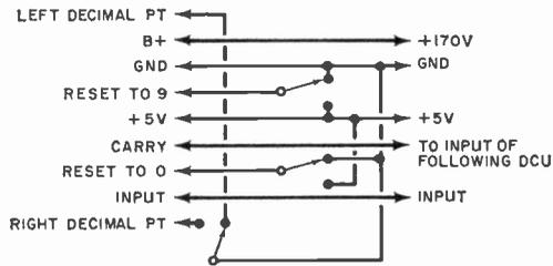
Fig. 6. Prior to wiring them into chassis, test individual DCU's using this circuit.
