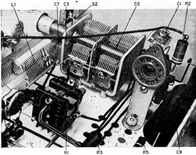
Fig. 4. Details of vacuum tube L-bracket (top) and rectifier and bypass capacitor mounting (bottom). The bracket is a narrow piece of scrap aluminum bent into an L-shape as shown with the vertical section about 1½" long; mount the socket so that pin 4 faces the chassis. Also clearly shown in lower photo are the 4-36 screw and nut that prevents the rotor of C5 from opening fully to avoid accidental operation on 20 meters. Note method of "countersinking" L1's turns on both sides of tapped turn.
