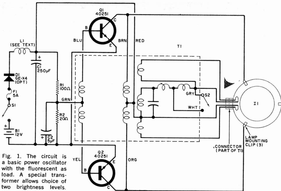
Fig. 1. The circuit is a basic power oscillator with the fluorescent as load. A special transformer allows choice of two brightness levels.
