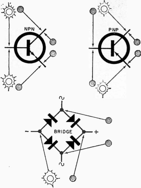
To check a transistor for type, connect probes as in two diagrams at top. If unit is npn, the lamp connected to the base will glow; if it is pnp, the lamp connected to either emitter or collector will glow. In a bridge rectifier, the lamp connected to the low side of d.c. glows.
