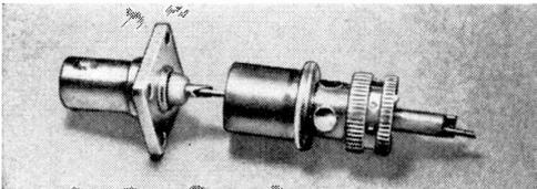
way out of this problem is to make an adapter. A type UG 261/U single-hole mounting BNC connector makes a good slip fit into the stem of a PL259 plug for the adapter assembly. First, solder a length of bare, solid hookup wire into the BNC connector, and slide the wire through the stem of the PL259 plug as shown in the photo. Now, bend the end of the wire over the center contact of the PL259, bringing the flange of the BNC into contact with the PL259 plug. Solder the
