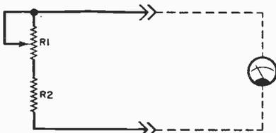
Values of potentiometer  $R1$  and resistor  $R2$  depend on the internal resistance of the meter movement.
