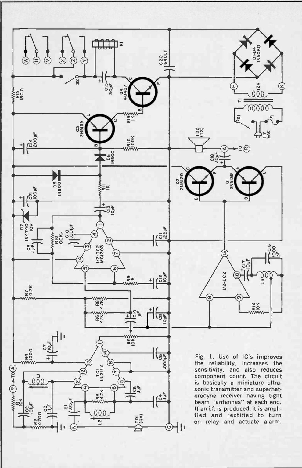
Fig. 1. Use of IC's improves the reliability, increases the sensitivity, and also reduces component count. The circuit is basically a miniature ultrasonic transmitter and superheterodyne receiver having tight beam "antennas" at each end. If an i.f. is produced, it is amplified and rectified to turn on relay and actuate alarm.
