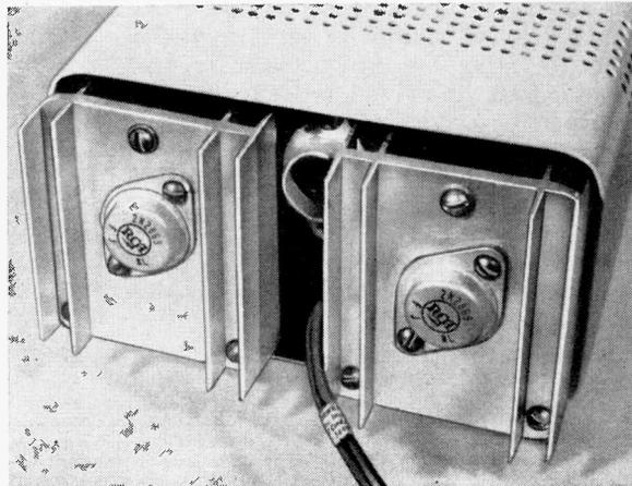
carefully select the location for SO1. Drill the hole for and mount this five-contact socket. Then solder 6" lengths of heavy-duty stranded hookup wire to the contacts of each transistor socket, and mount the transistor/heat-sink assemblies on the rear of the case. Use
