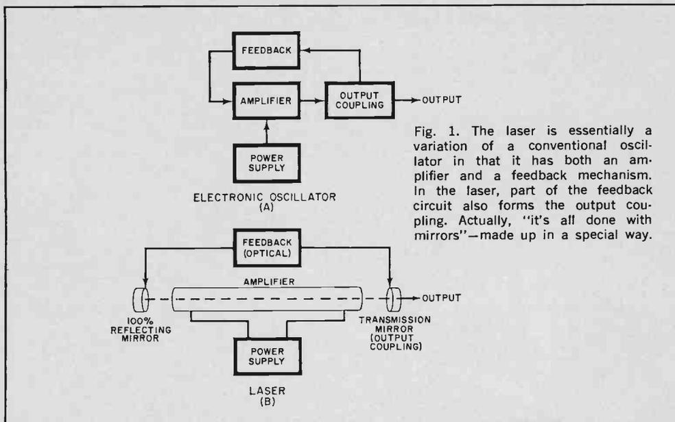
Fig. 1. The laser is essentially a variation of a conventional oscillator in that it has both an amplifier and a feedback mechanism. In the laser, part of the feedback circuit also forms the output coupling. Actually, "it's all done with mirrors"—made up in a special way.
