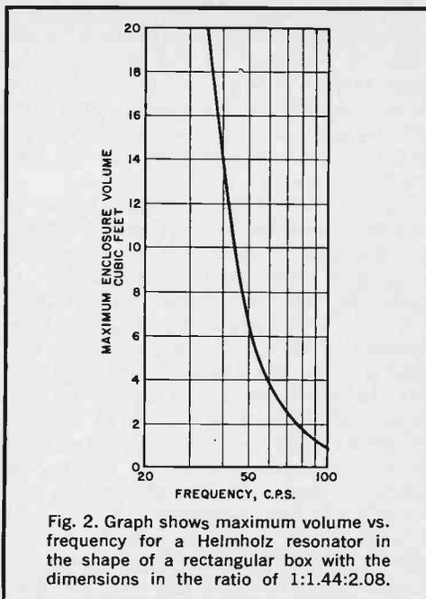
Fig. 2. Graph shows maximum volume vs. frequency for a Helmholtz resonator in the shape of a rectangular box with the dimensions in the ratio of 1:1.44:2.08.
