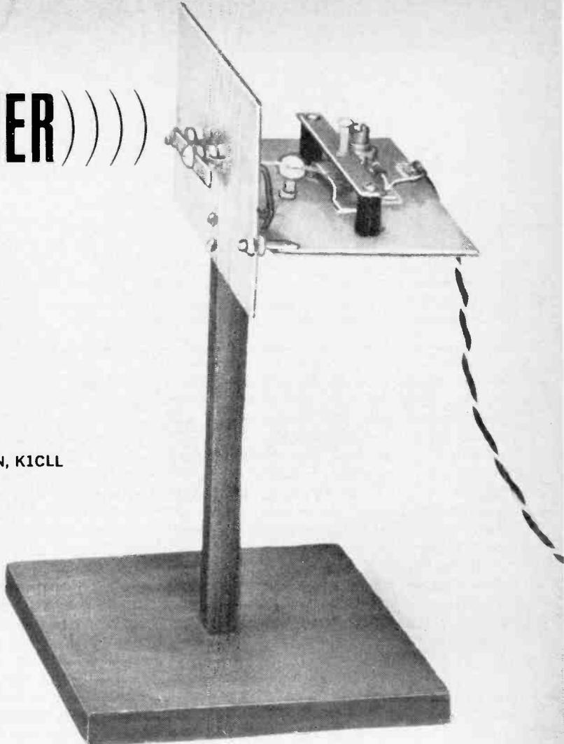
not easy to tune. The construction technique used in this project results in a tuned circuit that is electrically the same as stripline but it is easier to build and tune. In this case, we use a ground plane, air and nylon for insulation, and ordinary thin copper strips for the r.f. conductors.
