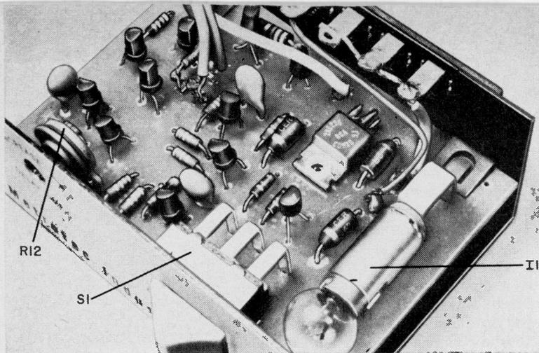
When mounting the PC board in the chassis make sure you can gain screwdriver access to R12 so that delay time can be adjusted as desired. If you have no need to vary this time, eliminate the hole.
