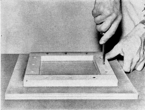
Fig. 4. Prior to mounting top plate on column, attach  $1\frac{5}{8}$ " x  $\frac{3}{4}$ " pine cleats as shown in photo.
