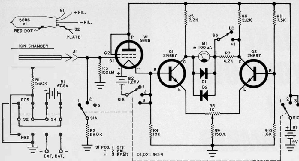
Ions detected by the ion chamber develop a small voltage drop across the very high resistance of R3. This voltage is amplified and operates a transistorized bridge. Sensitivity depends on the value of R3 which must be extremely high to make the circuit effective.
