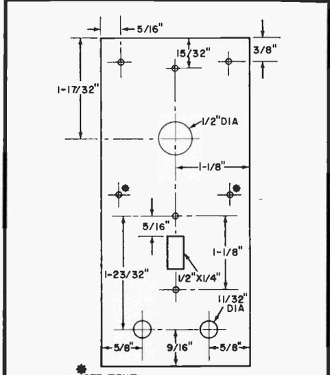
Fig. 2. Dimension details shown in drawing are for machining front of the utility box.
