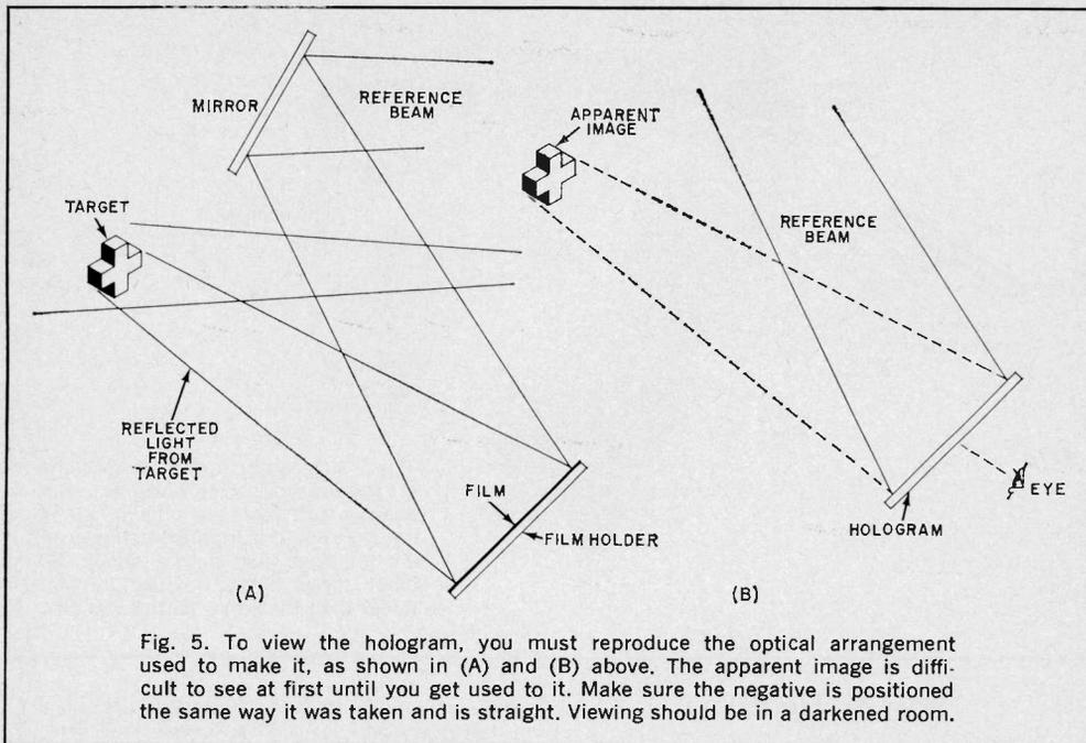
Fig. 5. To view the hologram, you must reproduce the optical arrangement used to make it, as shown in (A) and (B) above. The apparent image is difficult to see at first until you get used to it. Make sure the negative is positioned the same way it was taken and is straight. Viewing should be in a darkened room.
