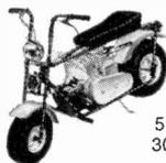
Giant 18 x 8.50 rear tire gives positive traction in mud, sand, gravel, snow... goes where other bikes can't. 2-speed. 5-HP 4-cycle engine. Up to 30 mph. **Kit GT-18**, 140 lbs.
