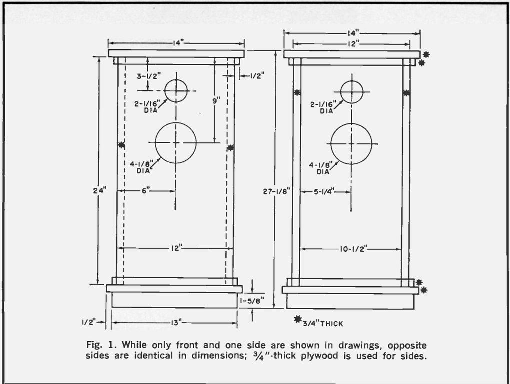
Fig. 1. While only front and one side are shown in drawings, opposite sides are identical in dimensions;  $\frac{3}{4}$ "-thick plywood is used for sides.
