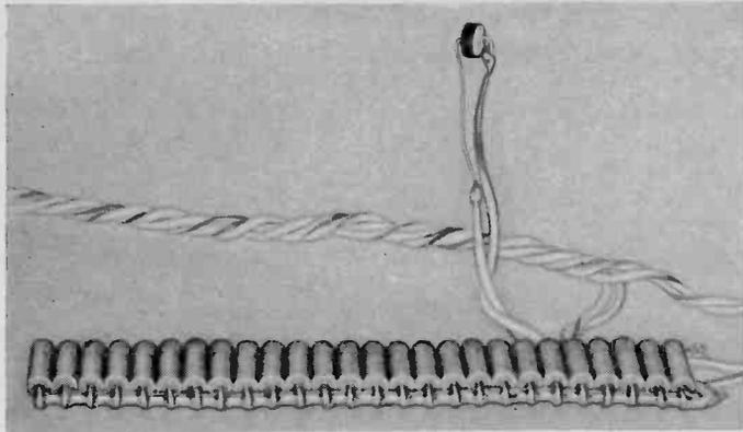
coating too thick, but make certain that the entire assembly and the attached ends of the wires are completely sealed. A water leak from improper sealing will cause the heater to fail, and copper in solution from the wires will harm your fish.
