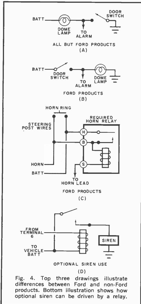
Fig. 4. Top three drawings illustrate differences between Ford and non-Ford products. Bottom illustration shows how optional siren can be driven by a relay.
