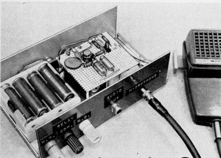
The three relay contacts—normally open, normally closed, and armature are terminated in three binding posts on the rear apron. These are connected as required by the external equipment being controlled, which can be either a tape recorder or transceiver.
