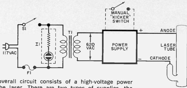
Fig. 2. The overall circuit consists of a high-voltage power supply and the laser. There are two types of supplies, the automatic that comes on a second or so after line power is applied, and the manual start with a "kicker" switch.
