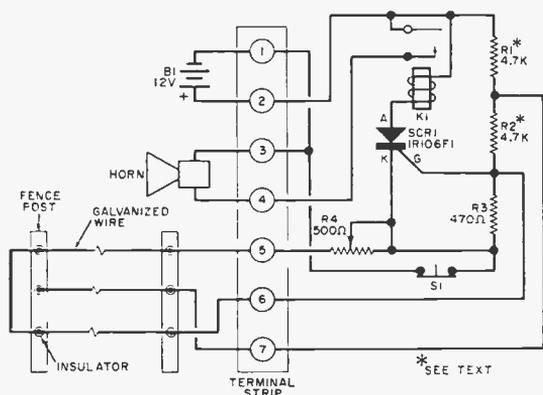
Fig. 1. Fence wires form closed loops and are resistively balanced with system. Imbalance due to short or open circuit will trigger alarm system.
