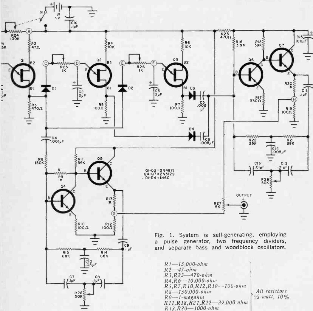
Fig. 1. System is self-generating, employing a pulse generator, two frequency dividers, and separate bass and woodblock oscillators.
