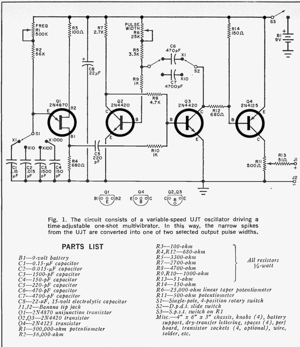
Fig. 1. The circuit consists of a variable-speed UJT oscillator driving a time-adjustable one-shot multivibrator. In this way, the narrow spikes from the UJT are converted into one of two selected output pulse widths.
