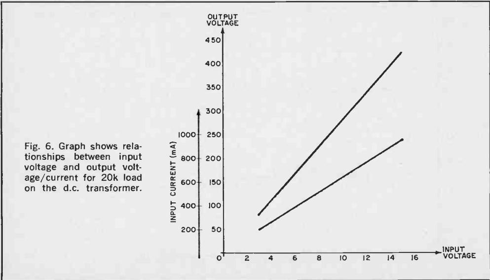
Fig. 6. Graph shows relationships between input voltage and output voltage/current for 20k load on the d.c. transformer.
