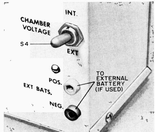
Switch S4 is used if it is desired to use a higher voltage for the ion chamber for more sensitivity.
