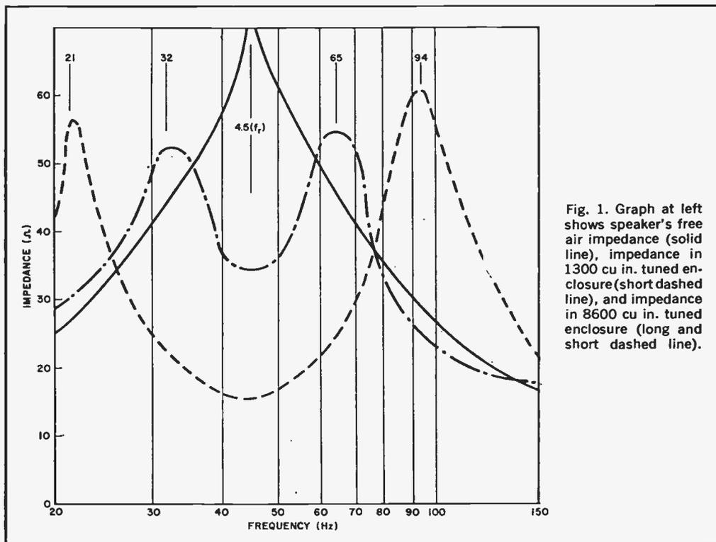
Fig. 1. Graph at left shows speaker's free air impedance (solid line), impedance in 1300 cu in. tuned enclosure (short dashed line), and impedance in 8600 cu in. tuned enclosure (long and short dashed line).
