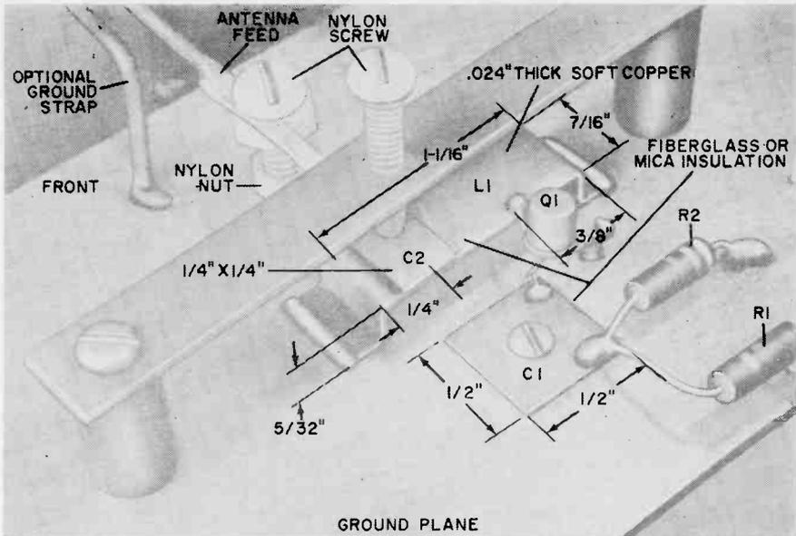
Fig. 3. Mechanical construction of the transmitter. Antenna coupling capacitor  $C2$  has its thin lead wedged between the nylon support screw head and a nylon nut. Use a piece of scrap PC board to make the tuning screw support bridge, using a metal screw to tap the  $C2$  hole.
