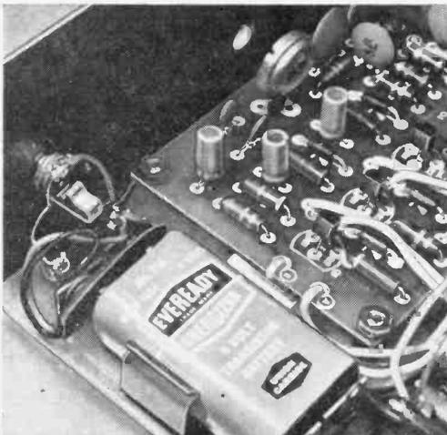
Battery can be conveniently mounted inside chassis with dual AA cell holder; use a conventional snap-on connector. Holes drilled directly in line with R28 and R29 (see top center of photo) provide access for tuning bass and woodblock oscillators. Mount output jack on rear.
