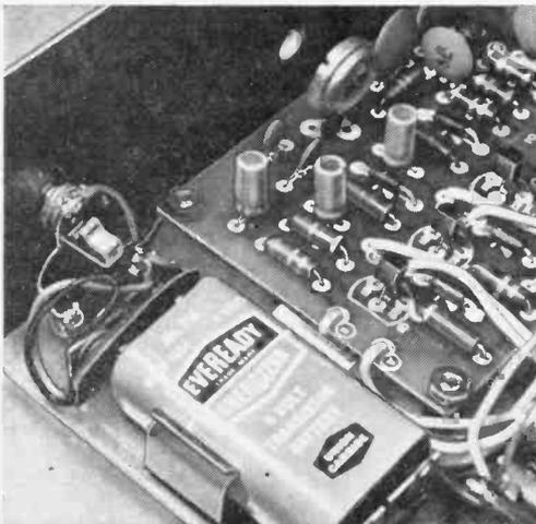
Battery can be conveniently mounted inside chassis with dual AA cell holder; use a conventional snap-on connector. Holes drilled directly in line with R28 and R29 (see top center of photo) provide access for tuning bass and woodblock oscillators. Mount output jack on rear.
