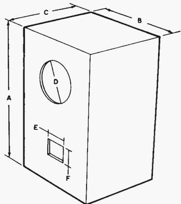
Fig. 3. "Universal" enclosure recommended by T. W. Richardson for "orphan" loudspeakers. Tune enclosure to 40 Hz. Use  $\frac{3}{4}$ " plywood, well braced, and glued and screwed together with glue blocks inside the corners. Volume should be at least 5 cu. ft. Typical values for A, B, and C would be 30", 21", and 14.5" respectively. If tuning equipment is not available, try 4 in. for E and  $3\frac{1}{2}$  in. for F.
