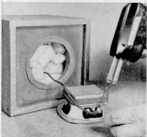
Cut a piece of acoustical fiberglass to  $6'' \times 24''$ . Roll it up and insert it through the speaker cutout into the enclosure. Now carefully unroll it, and press it into place around the interior walls. Then press into place against the rear wall another piece of fiberglass.
