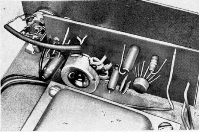
Fig. 3. Circuit board mounts to front of case via long threaded shaft of volume control. Use shielded cable to connect input jack to circuit board as shown.
