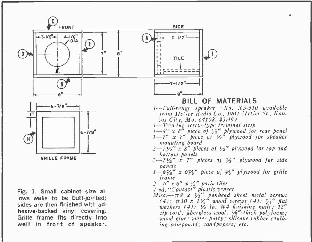
Fig. 1. Small cabinet size allows walls to be butt-jointed; sides are then finished with adhesive-backed vinyl covering. Grille frame fits directly into well in front of speaker.
