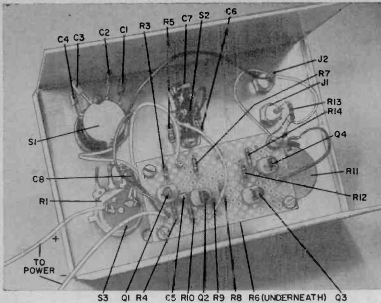
Fig. 2. Underside of chassis shows placement of board components and front-panel mounted controls and terminals.
