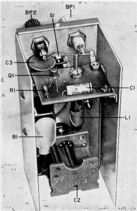
Fig. 4. Mount battery to side of box with length of aluminum stock,  $\frac{1}{2}$ " spacers, and #6 hardware.
