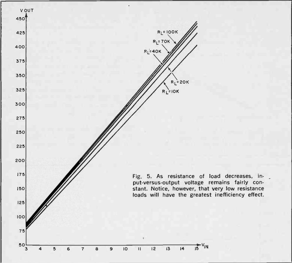
Fig. 5. As resistance of load decreases, input-versus-output voltage remains fairly constant. Notice, however, that very low resistance loads will have the greatest inefficiency effect.
