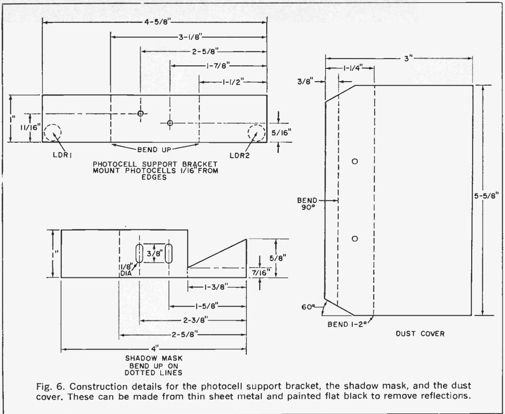
Fig. 6. Construction details for the photocell support bracket, the shadow mask, and the dust cover. These can be made from thin sheet metal and painted flat black to remove reflections.
