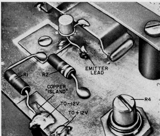
Fig. 2. The emitter of *Q1* couples to *RFC1* via an insulated wire fed through a hole in the PC board. Use a sharp blade to create an insulated "island" for the -12-volt feed. Don't forget the mica insulator underneath bypass capacitor *C1*.
