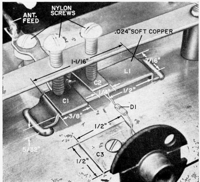
Fig. 7. Construction details of receiver. Strapline *L1* is the same as used in the transmitter. Be sure to install mica insulators under capacitors *C1*, *C2*, and *C3*. Receiver uses the same antenna construction as that used with the transmitter.
