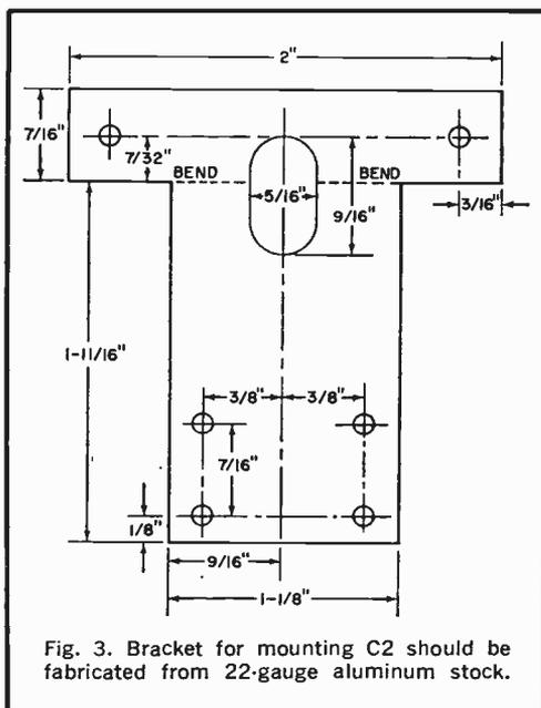
Fig. 3. Bracket for mounting *C2* should be fabricated from 22-gauge aluminum stock.
