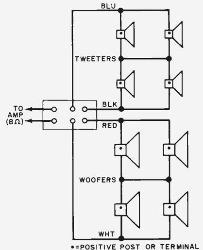
Fig. 5. Tweeters and woofers are wired in series-parallel to present 8-ohm impedance to amplifier.
