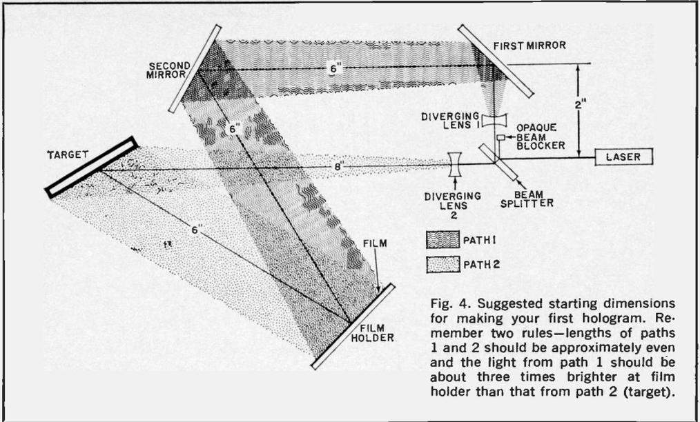
Fig. 4. Suggested starting dimensions for making your first hologram. Remember two rules—lengths of paths 1 and 2 should be approximately even and the light from path 1 should be about three times brighter at film holder than that from path 2 (target).
