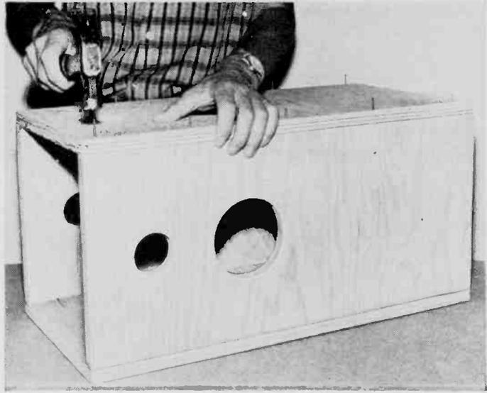
has four woofer-midrange speakers connected through a 3000-Hz crossover to four horn-type tweeters. Thus a woofer-tweeter pair faces each of the four walls or the corners if desired. The use of four small woofers results in an enclosure of modest dimensions that occupies only about  $1\frac{1}{3}$  sq ft of floor space. A control on the bottom-mounted crossover network balances the tweeter output to that of the woofers.
