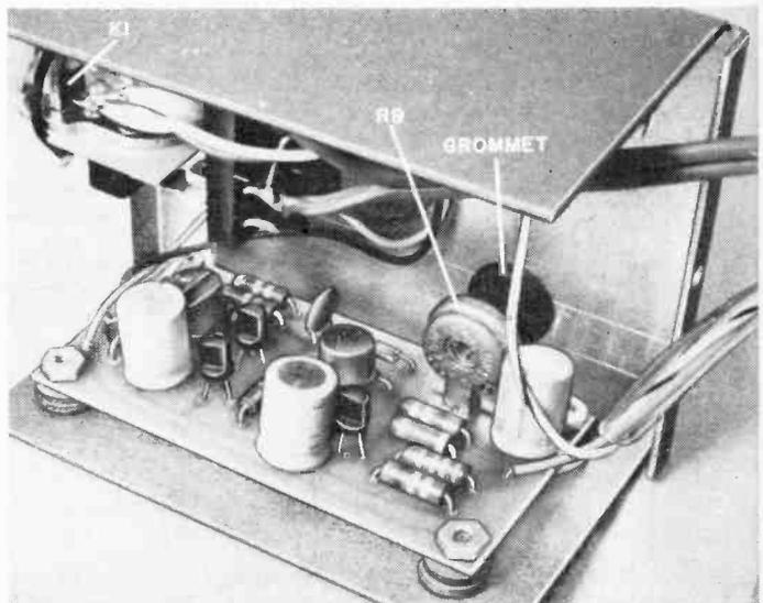
the timer. The wire that goes to the battery should be connected to the BATTERY terminal on the timer. The GROUND terminal of the Time Out is connected to any convenient ground point such as under the head of an existing screw in the
