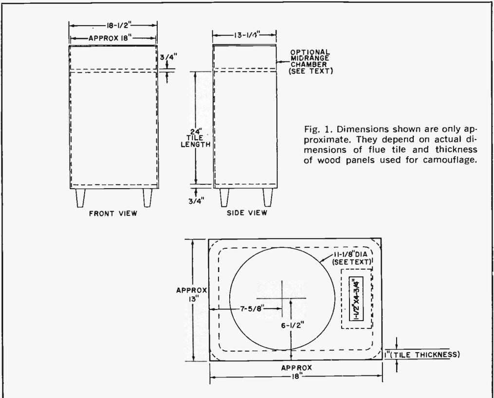
Fig. 1. Dimensions shown are only approximate. They depend on actual dimensions of flue tile and thickness of wood panels used for camouflage.
