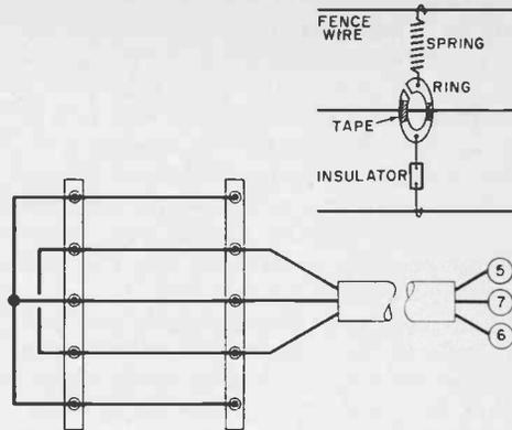
Fig. 2. Jiggle (top) triggers alarm if fence wires are compressed or spread. Numbered wires on 5-wire fence match same numbered lugs on terminal strip.
