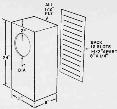
Fig. 4. Compact (1 cu ft) enclosure for 8" speakers has all sides lined with 1" absorbent material. Back is lined with soft cloth. Slots may be made by cutting strips of 1/2" plywood to proper width and mounting them on a frame width 1/2" spacing. Or cut a row of 10 holes 1/2" in diameter to give about the same area as the 8" x 1/4" slot.
