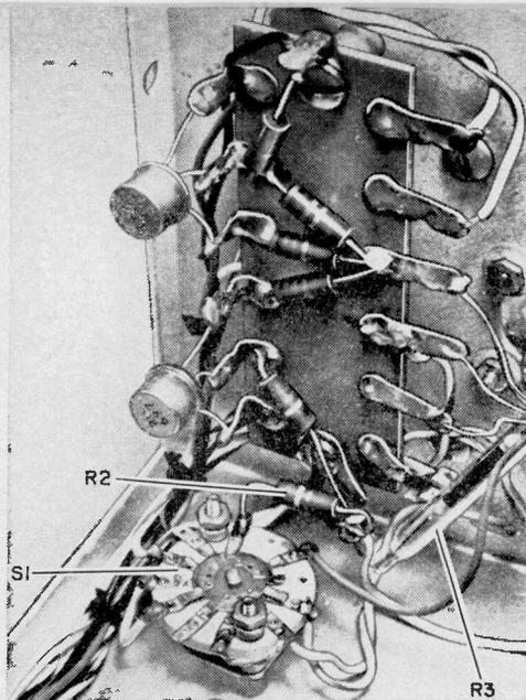
Function switch S1 is located near the electronics board. Use a high-quality ceramic switch to prevent leakage around the very high value of resistor R3.
