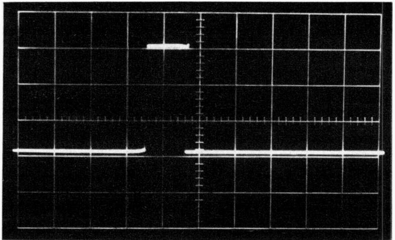
Typical output pulse shows the extremely rapid rise and fall times on this pulse generator. The width of the pulse can be adjusted by the setting of switch S2.
