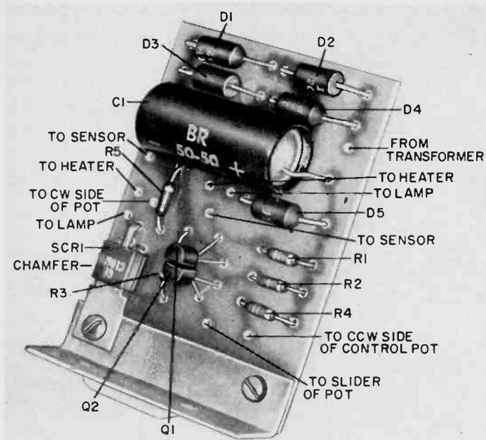
Fig. 4. Actual-size printed circuit board etching guide is given at lower left. Component locations and orientations on circuit board are shown in photo. For proper heat sinking of SCR1, bolt its tab to mounting bracket used for circuit board as shown.
