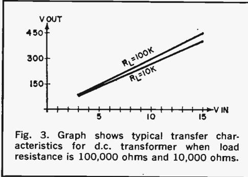
Fig. 3. Graph shows typical transfer characteristics for d.c. transformer when load resistance is 100,000 ohms and 10,000 ohms.
