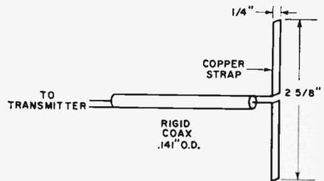
Fig. 9. This simple dipole can be used to perform experiments with various antenna arrays. These can include beams, horns, or parabolic systems. Remove the old antenna and ground plane and install this.
