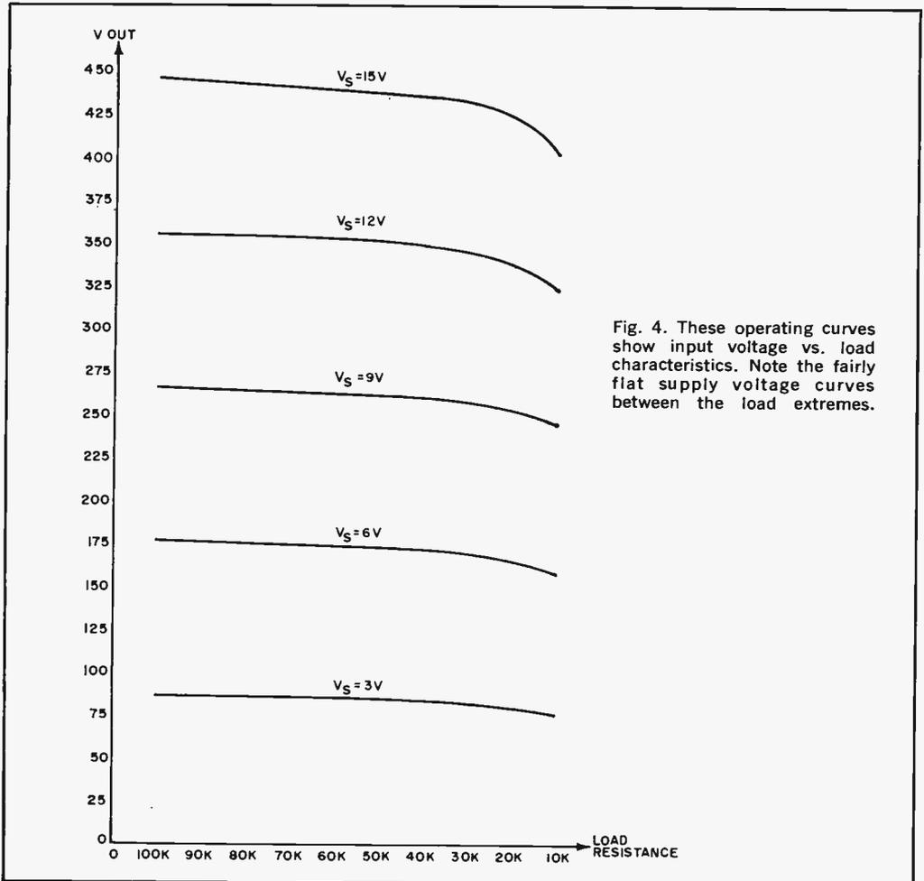
Fig. 4. These operating curves show input voltage vs. load characteristics. Note the fairly flat supply voltage curves between the load extremes.
