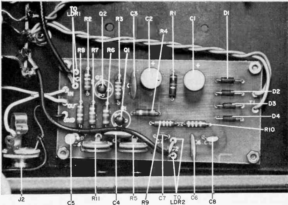
Fig. 3. After installing all components on board, make sure both trimmer potentiometers are accessible through holes drilled in side of chassis. This view also shows connections to other elements.
