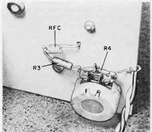
Fig. 4. Underside view of the transmitter showing the location of the RFC and  $R3$ . One end of the RFC feeds through a hole and contacts  $Q1$  emitter.
