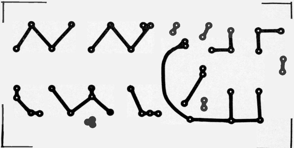
Fig. 3. Actual-size foil pattern for automatic start supply. Drill mounting holes at the four corners.
