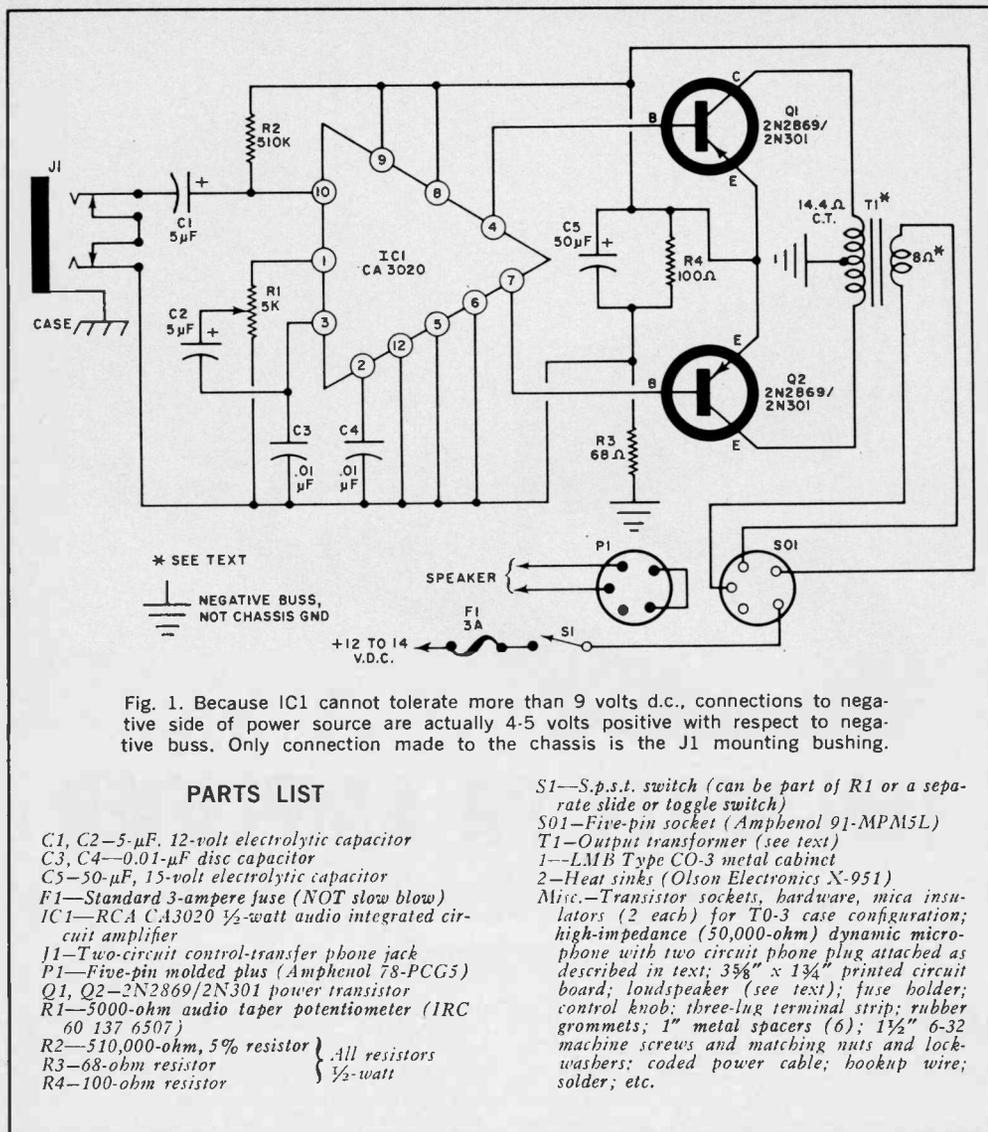
Fig. 1. Because IC1 cannot tolerate more than 9 volts d.c., connections to negative side of power source are actually 4-5 volts positive with respect to negative buss. Only connection made to the chassis is the J1 mounting bushing.
