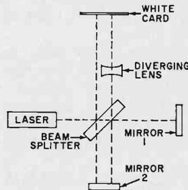
the white card. You can adjust the optics slightly to make both pairs visible. Further adjustment of the optics will cause one pair of dots to be superimposed on the other pair.
