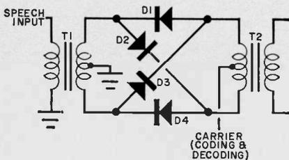
With no speech applied to the primary of *T1*, when the applied encoding carrier is positive going (with respect to ground), the currents in the primary of *T2* and the secondary of *T1* (through diodes *D1* and *D4*) are out of phase so that no carrier signal is developed in the secondary of *T2*. When the encoding carrier is negative going, the same thing happens as the current flows through diodes *D2* and *D3*. Thus none of the encoding carrier gets through output transformer *T2*.
