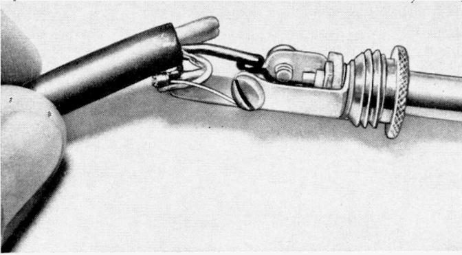
Fig. 5. When connecting plug to microphone cable, use only two shorter contacts. Do NOT allow cables to touch long one.
