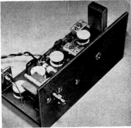
For a front panel for transmitter, prototype had a second sheet of double-faced copper clad board.
