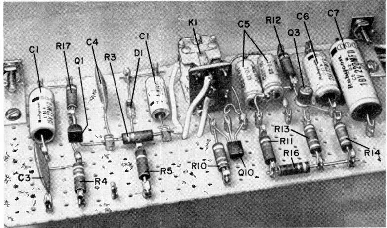
Single piece of perforated board was used in prototype to accommodate all parts (except jacks and controls) in basic circuit and auto/manual add-on.
