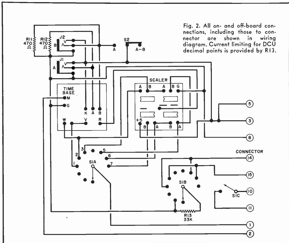
Fig. 2. All on- and off-board connections, including those to connector are shown in wiring diagram. Current limiting for DCU decimal points is provided by *R13*.
