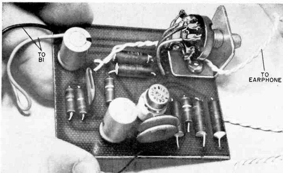
Although presently as small as a cigarette pack, the receiver can be made smaller by tightening up on the foil pattern, eliminating the IC socket, and using smaller physical sizes for C8, C9 and R2. A hearing-aid battery can be substituted for the 9-volt transistor radio battery, and a ferrite loopstick can be tried in place of the coil. Any number of receivers can be used on one loop.
