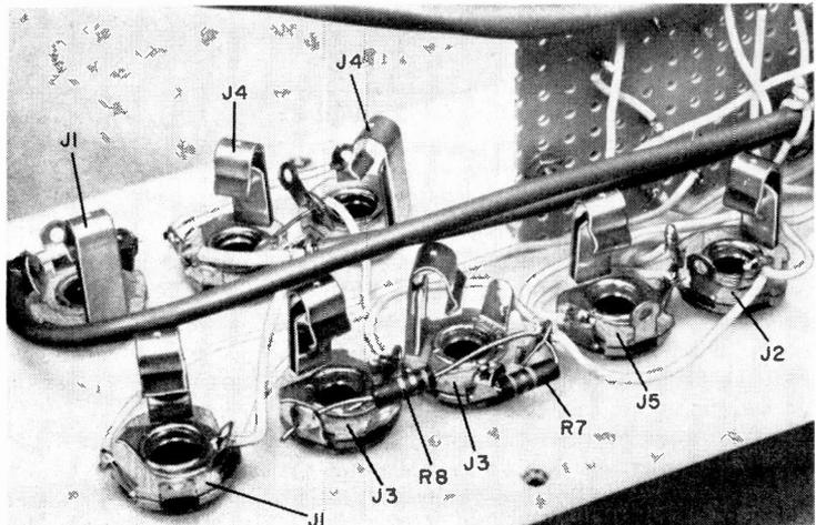
Wired clipper amp board fastens to front panel with 4-40 machine hardware and small L bracket. Wires connecting sub-assembly into system are soldered to terminals on the bottom side of the circuit board.
