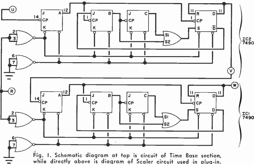
Fig. 1. Schematic diagram at top is circuit of Time Base section, while directly above is diagram of Scaler circuit used in plug-in.
