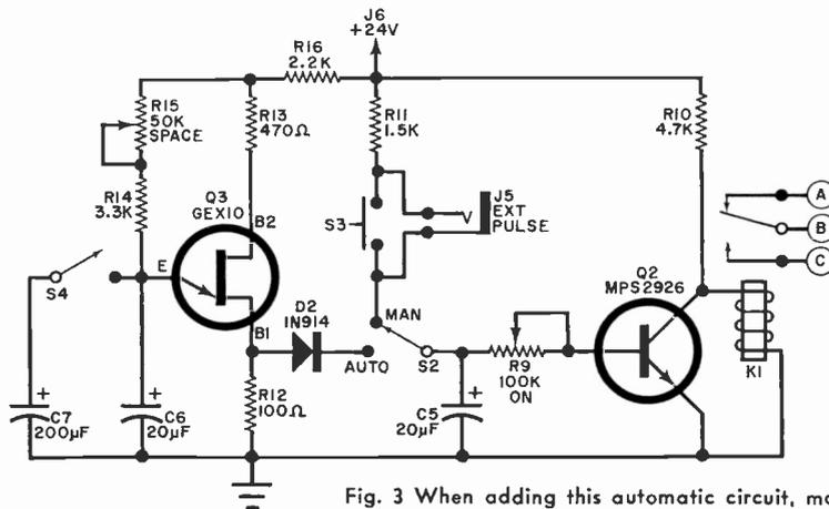
Fig. 3 When adding this automatic circuit, match lettered contacts on K1 to same lettered points in manual circuit and eliminate S1. Use S3 to initiate envelope.
