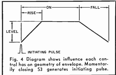
Fig. 4 Diagram shows influence each control has on geometry of envelope. Momentarily closing S3 generates initiating pulse.
