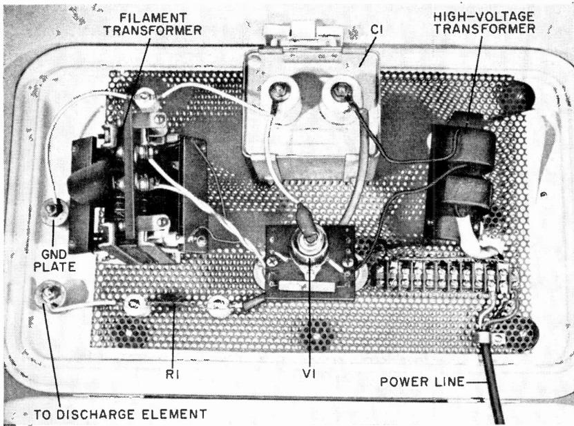
Fig. 4. Because the weak plastic chest cover will not support much weight, a perforated metal base plate is used to mount the heavy components. Feedthroughs are used to couple to the "antenna" and the main ground plate that supports the flower pot.
