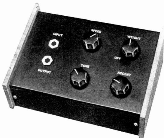
In prototype, top of case slopes downward. Top, front, and rear panels are painted flat black to contrast with rich tones of walnut side panels. Controls and jacks are lettered in white, using dry-transfer lettering kit.
