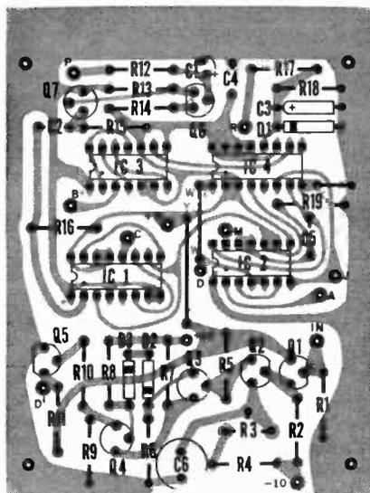
sistors, diodes, and electrolytic capacitors. When you finish soldering, examine the foil sides of the boards, comparing them against the guides in Fig. 7, to determine if any solder bridges exist between the closely spaced foil conductors. If you locate a solder bridge, reheat the connection adjacent to it and remove the excess solder.
