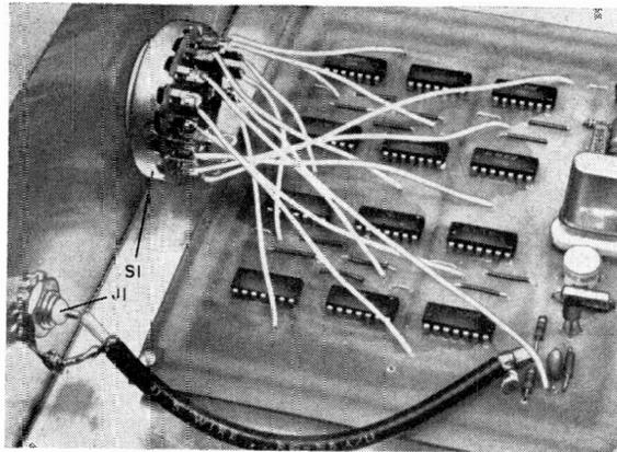
The connections from the PC board to the selector switch should be made as short as possible. A short length of coaxial cable serves as the output lead.
