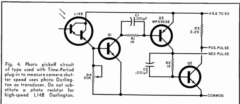
Fig. 4. Photo pickoff circuit of type used with Time-Period plug-in to measure camera shutter speed uses photo Darlington as transducer. Do not substitute a photo resistor for high-speed L14B Darlington.
