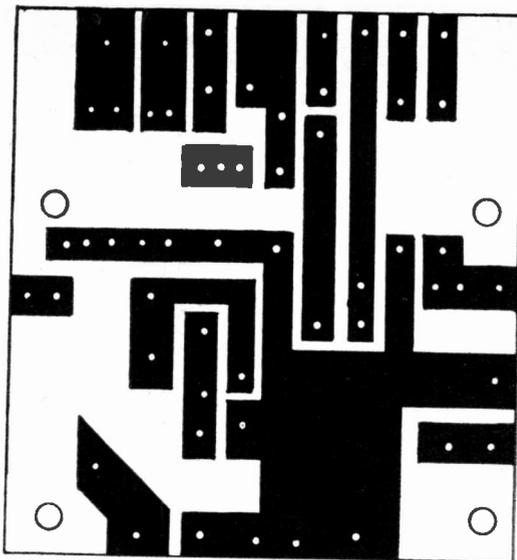
This figure also shows the component installation and the external connections. Transistor sockets should be used to prevent thermal damage to the semiconductors during soldering.
