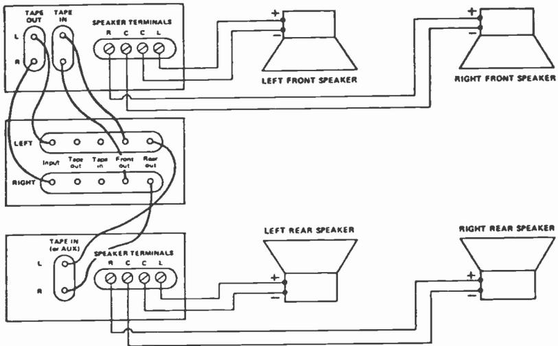
Rear panel connections for both inputs and outputs.
