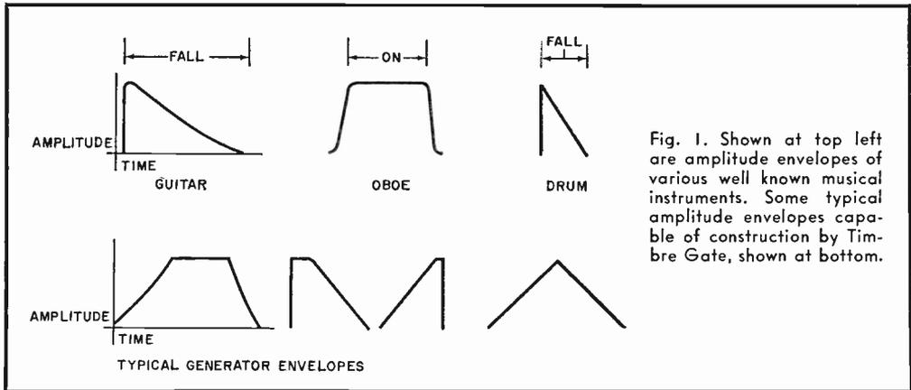
Fig. 1. Shown at top left are amplitude envelopes of various well known musical instruments. Some typical amplitude envelopes capable of construction by Timbre Gate, shown at bottom.
