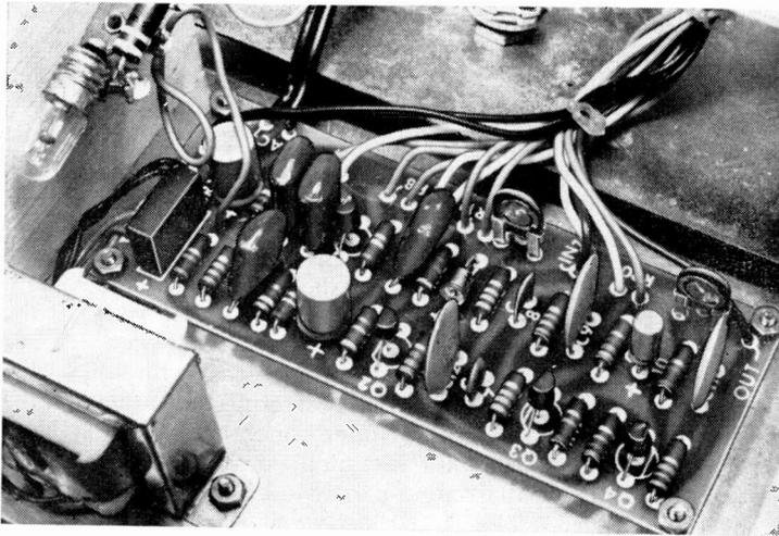
Neatly dress control and jack wiring to one side of circuit board and lace together with cable ties or lacing cord. Secure power transformer to chassis with 4-40 machine hardware; add  $\frac{1}{4}$ " spacers when mounting board in place.
