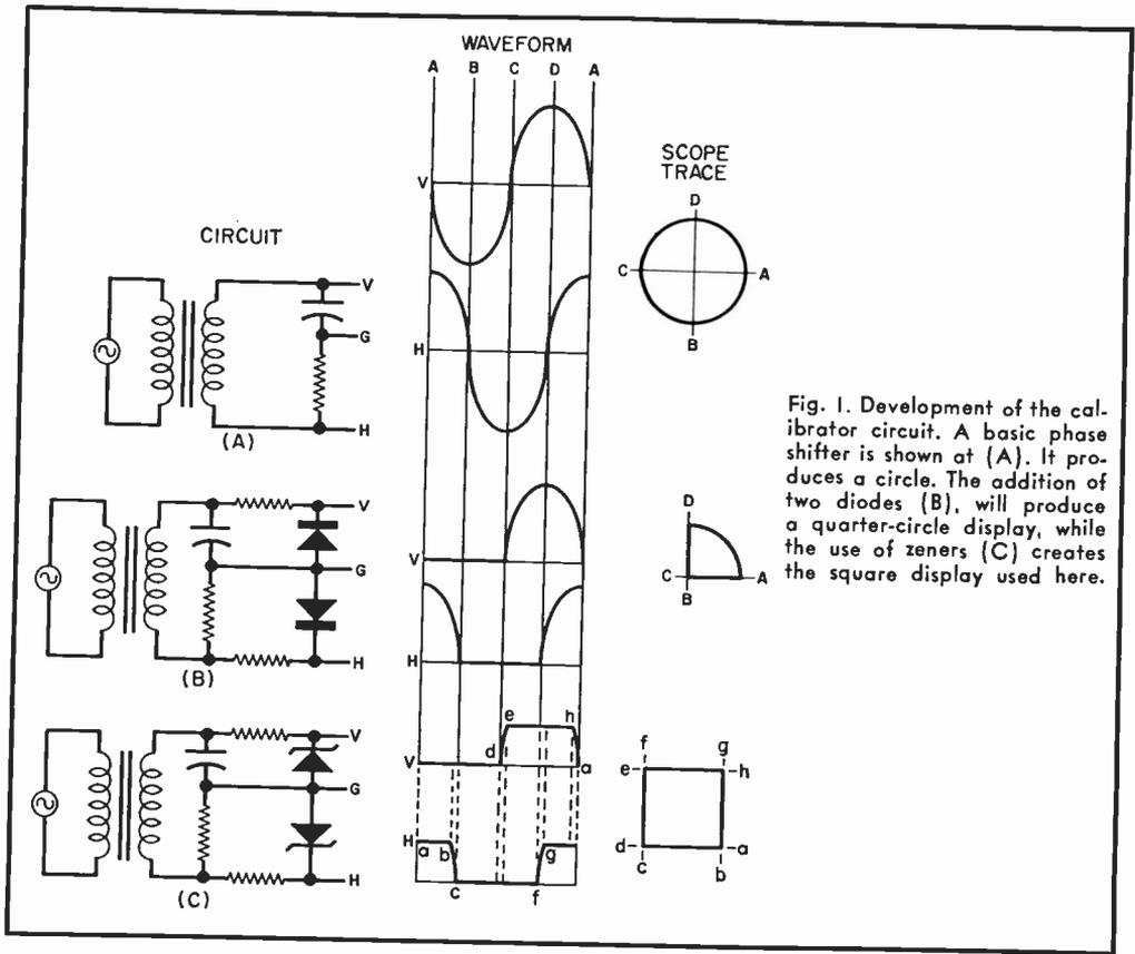
the voltage can be preset from zero to the maximum determined by the zener diodes.
