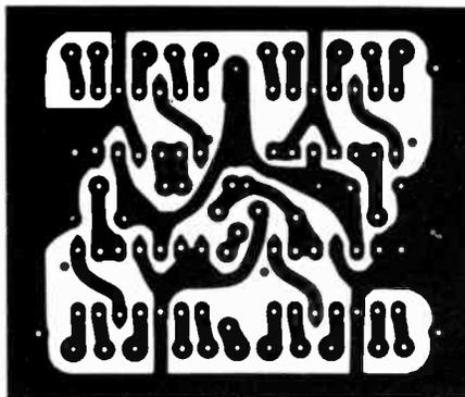
Fig. 7. Actual size etching guides for Time Base and Scaler circuit boards are shown at left and above, respectively. Use etching guides to check for solder bridges between closely spaced conductors after all components are soldered to circuit boards.
