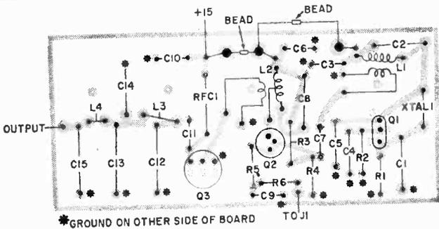
Fig. 4. Above is printed circuit foil pattern for underside of the double-faced board. Parts placement is shown at left. Note that this is a view looking up through both copper foils. Terminations that are not marked with an asterisk go through the top side of the board and are soldered to remaining etched foil pattern.
