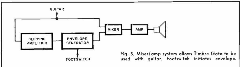
Fig. 5. Mixer/amp system allows Timbre Gate to be used with guitar. Footswitch initiates envelope.
