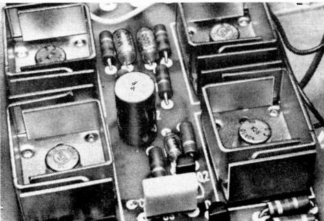
size wire. The circuits to which these wires connect carry as much as 10 amperes when the amplifier is driven to full power. If too small a wire size is used, power will be sacrificed and damping will suffer.)
