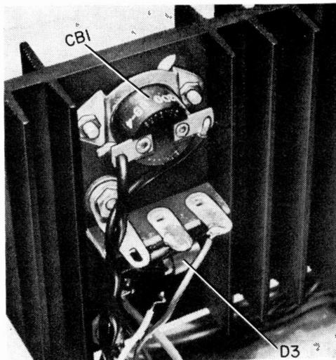
For proper operation, sensing element of thermal circuit breaker *CBI* must contact *Q7*'s heat sink.
