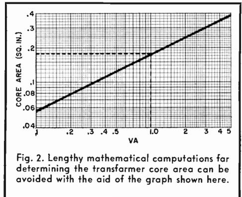
Fig. 2. Lengthy mathematical computations for determining the transformer core area can be avoided with the aid of the graph shown here.
