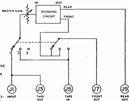
The Master volume control provides control of all four channels when decoding. To start, turn this control fully clockwise. Then advance the volume controls of the front and rear amplifiers to the loudest level you expect to use. The decoder's Master volume
