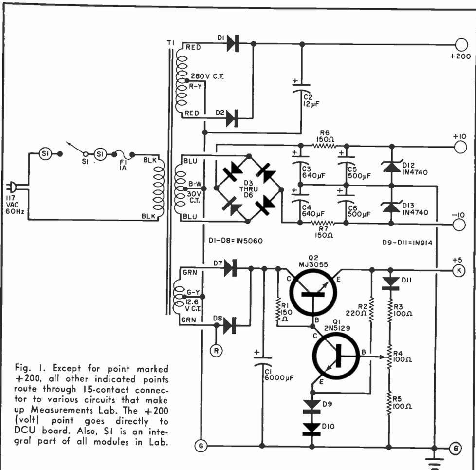
Fig. 1. Except for point marked +200, all other indicated points route through 15-contact connector to various circuits that make up Measurements Lab. The +200 (volt) point goes directly to DCU board. Also, S1 is an integral part of all modules in Lab.
