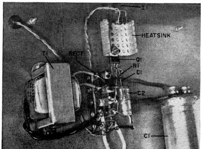
Use a 2-square-inch piece of scrap aluminum as the heat sink for Q1. Isolate the heat sink from the chassis using an insulated spacer.
