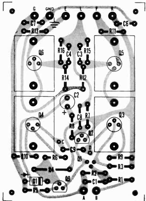
Fig. 2. Actual size etching guide is shown at left. In component layout and orientation diagram (above), boxes around Q3-Q6 represent outlines of heat sinks on these transistors. Note: connect the minus side of C2 to R8.
