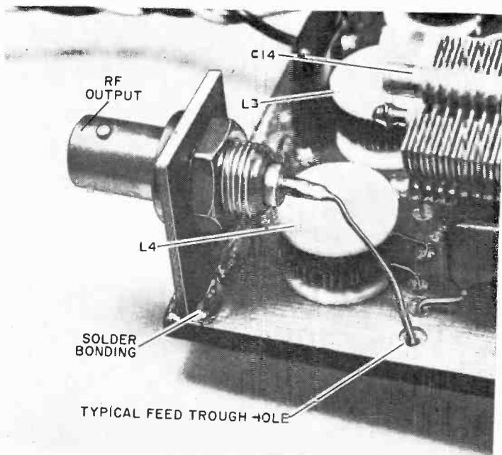
The author used a BNC output connector, though any coax connector could be substituted. Capacitor *C14* is adjusted by screwdriver from the front panel for operation on QRP frequency most used in your locality.
