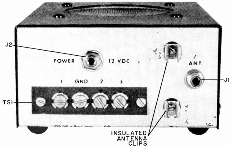
**Power Supply and S-Meter.** Any type of 12-volt dc power supply may be used with the receiver. One suitable circuit is shown in Fig. 4. Note that no filtering is shown since there are filters on the receiver PC board.
