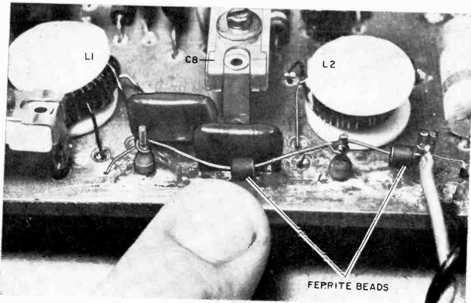
Ferrite beads are used in the plus 15-volt line to be sure harmonic radiation is kept down. The beads are slipped over the wires between the feedthru capacitors which are soldered on the board.
