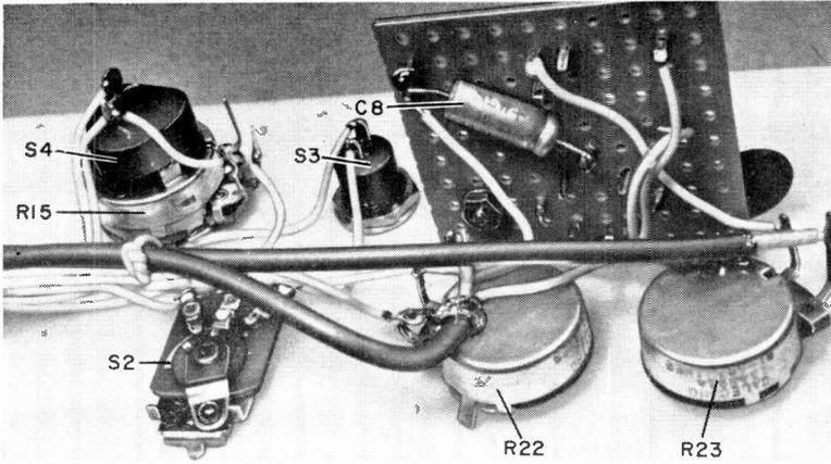
Solder shields of audio cables to the housings of potentiometers R22 and R23. Also note that capacitor C8 mounts on the bottom of clipper amp circuit board.
