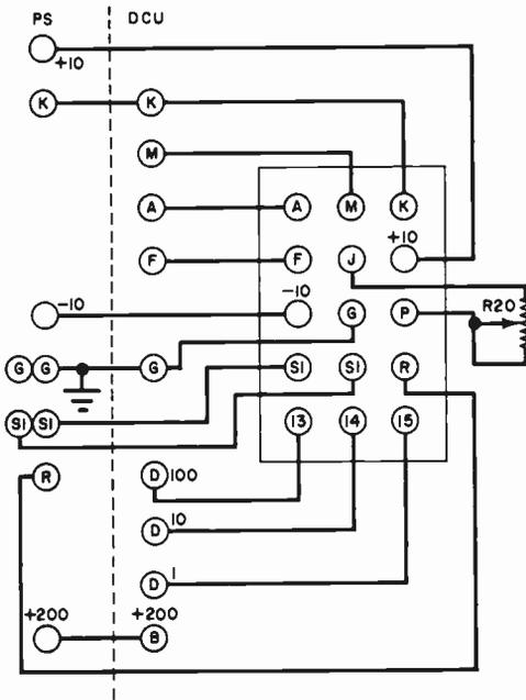
Fig. 3. Power supply (PS) and readout (DCU) boards and 15-contact connector are wired together as shown. Potentiometer R20 is display time control.
