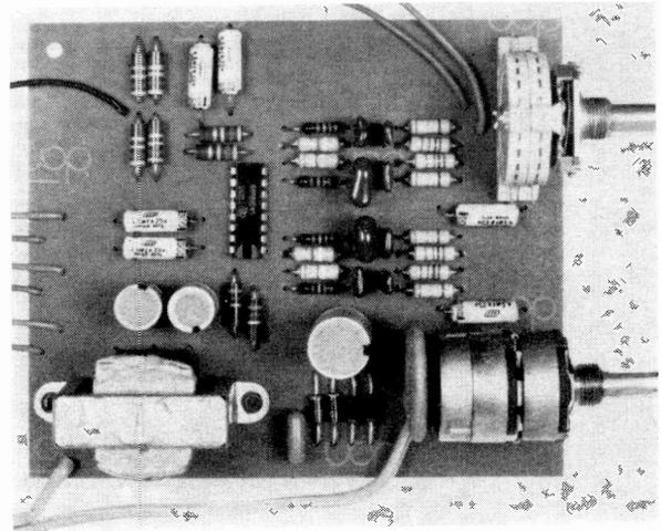
Top view of the decoder PC board.
