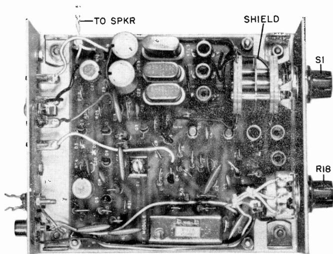
It is recommended that a shield be located between the two segments of S1 to avoid coupling. The collapsible antenna is attached to a pair of insulated fuse clips mounted on the rear apron. The speaker is fixed to the upper part of the chassis, while the four angle brackets secure the two chassis sections.
