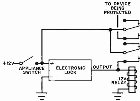
are turned off. This occurs when any pushbutton is depressed. However, when the correct pushbutton is depressed Q1 is inhibited by the charging of one of the capacitors through an SCR. Thus, "good" numbers do not cause cancellation, but any false number cancels everything. Also, if only four numbers are being used, and a fifth number is selected, the register is cancelled.
