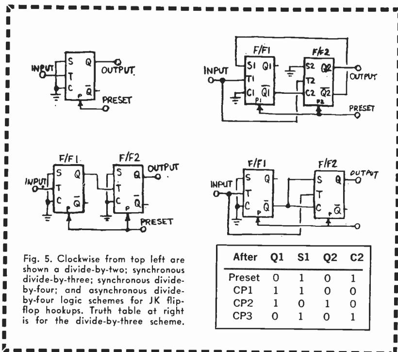
equal to about twice the propagation delay, or 60 nanoseconds, should be sufficient for the average medium-power JK flip-flop.
