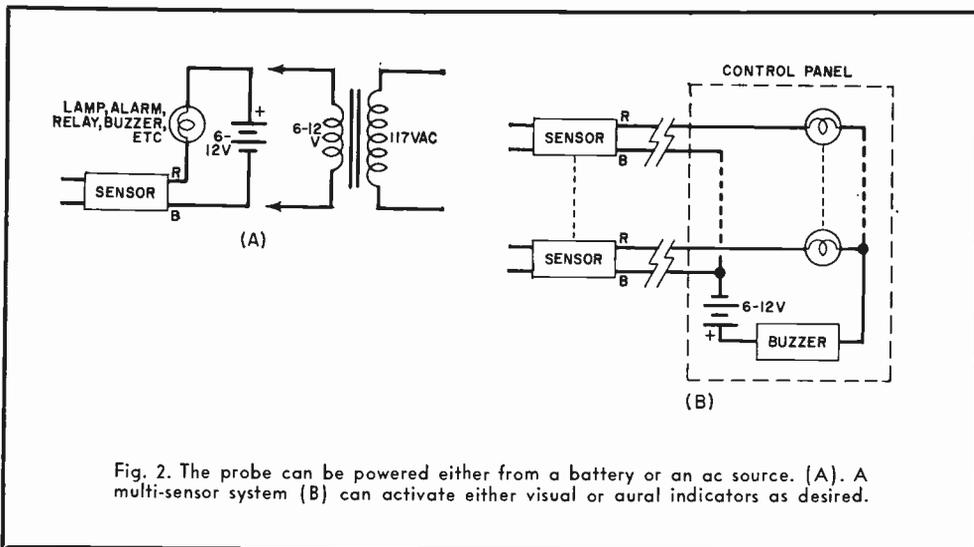
necter can be used to join the sensor to a longer set of leads to run back to the power supply and control panel.
