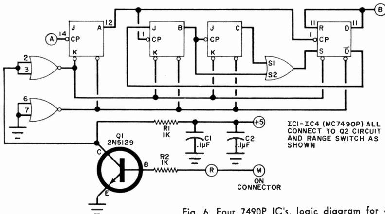
Fig. 6. Four 7490P IC's, logic diagram for only one of which is shown in Scaler circuit, connect to Q1 stage.
