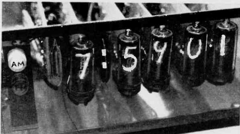
The colon is made by painting black bands on a neon lamp. If desired, another colon may be used between the seconds (the two readouts on the right) and the adjacent unit minutes indicator. In this time example, the tens hours neon is not lit. To reduce glare and to increase the readout contrast, mount a length of polarized material so as to completely cover the entire readout. Place the polarized material on a shiny metal surface and determine which side reduces the glare most. This will be the side that should be facing the viewer. Use adhesive to fix it in place.
