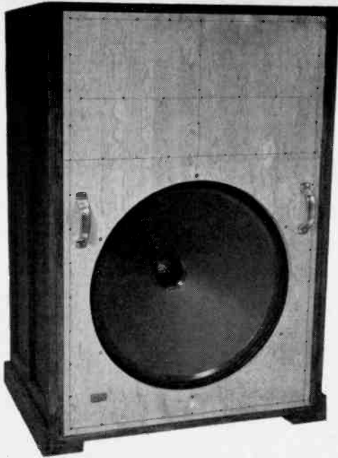
Woofer cone faces rear of enclosure. Grille cloth is used solely to protect cone from dust and dirt.
