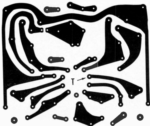
Fig. 3. Actual size foil pattern and component installation for the 540 amplifier.
