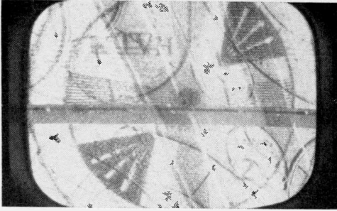
Actual reception (left) of KTVH, channel 12, Hutchinson, Kan. (155 miles) using only an outdoor antenna cut for that channel. Note severe adjacent channel interference from channel 13 (2.1 miles). Right is reception of channel 12 using the All American unit.
