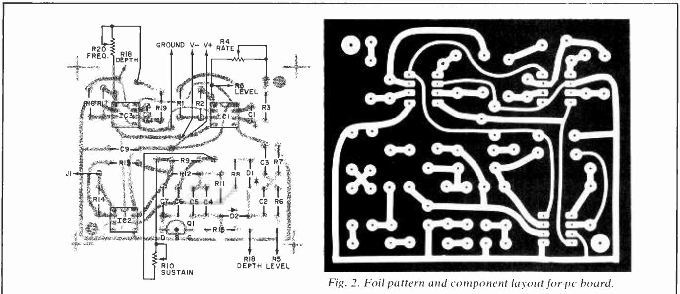
Fig. 2. Foil pattern and component layout for pc board.
