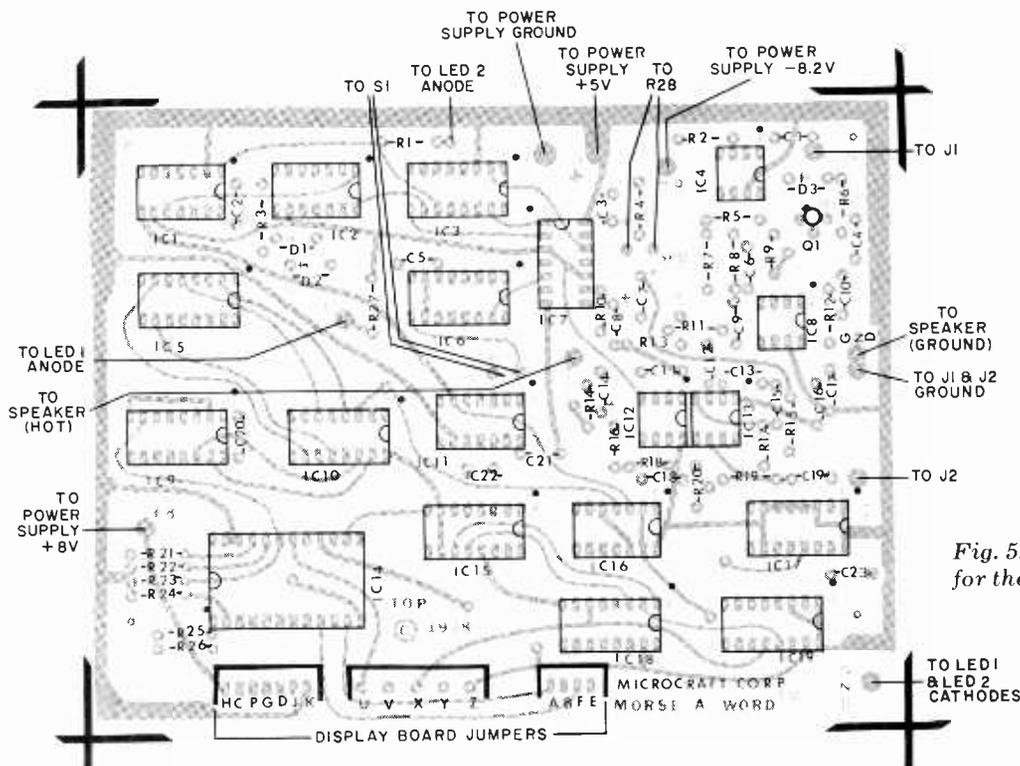
Fig. 5. Parts placement guide for the main circuit board.
