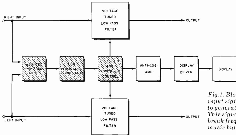
Fig. 1. Block diagram shows how input signals are processed to generate a control signal. This signal governs filter's break frequencies to pass music but attenuate noise.
