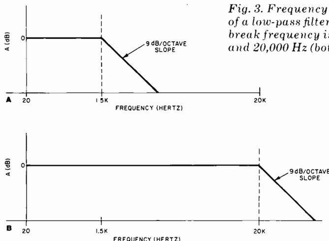
Fig. 3. Frequency response of a low-pass filter when its break frequency is 1500 Hz (top) and 20,000 Hz (bottom).
