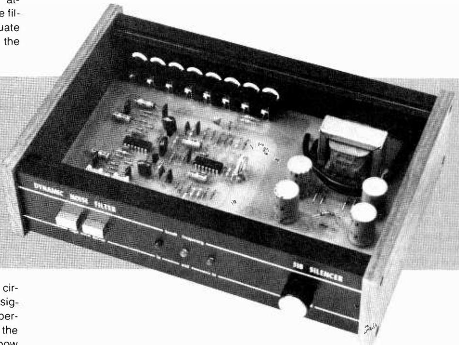
**About The Circuit.** The silencer circuit constantly analyzes incoming signals for amplitude, frequency, and persistence. These factors determine the bandwidth at any instant, as well as how quickly the variable low-pass filter changes. Attack and release times vary with the music, thus eliminating a "pump and wheeze" effect of noise modulation.
