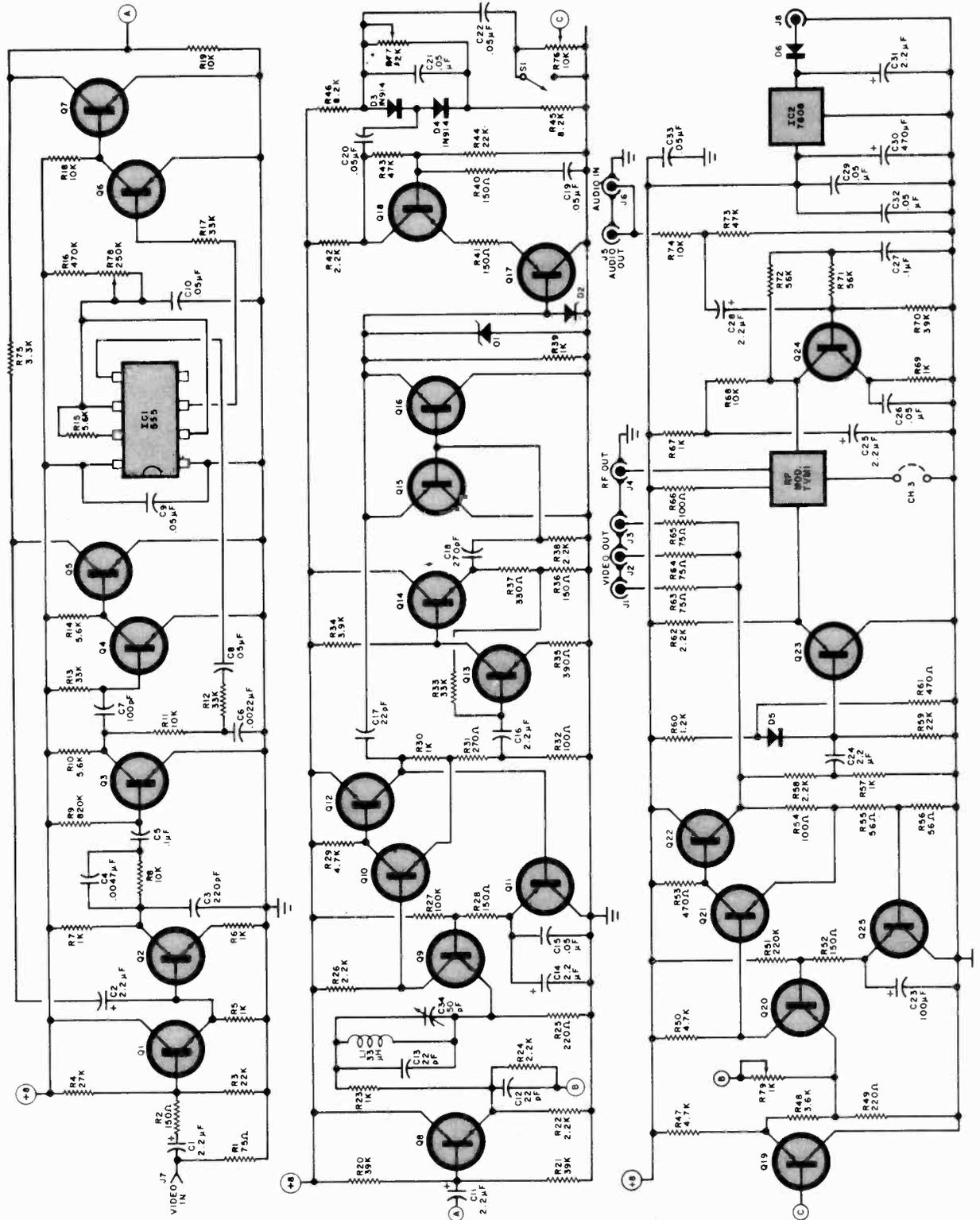
Fig 6. Schematic diagram of Video Enhancer
