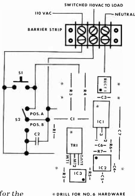
Fig. 3. Parts placement guide for the printed circuit board is shown at right.
