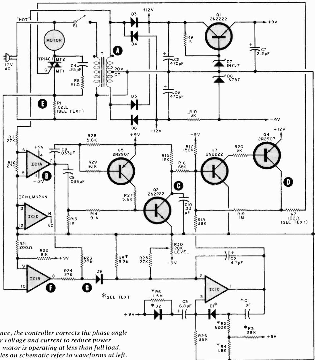
Fig. 2. In essence, the controller corrects the phase angle between motor voltage and current to reduce power required when motor is operating at less than full load. Letters in circles on schematic refer to waveforms at left.
