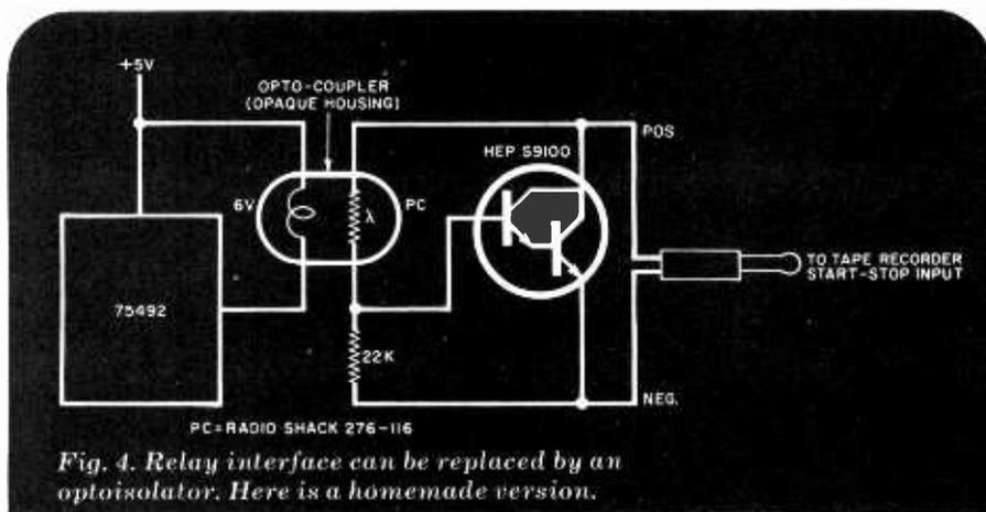
Fig. 4. Relay interface can be replaced by an optoisolator. Here is a homemade version.
