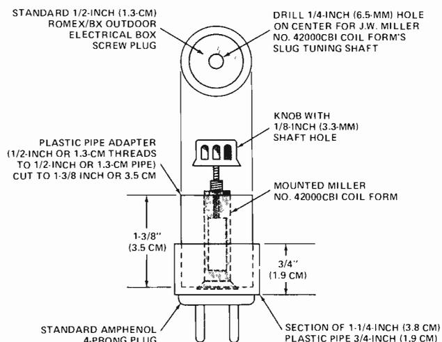
*Fig. 5. Assembly details for each plug-in coil ( $L2$ ).*
