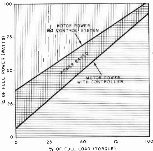
Fig. 1. These curves are the results of tests made by NASA on a  $\frac{1}{3}$ -hp split-phase and  $\frac{1}{4}$ - and  $\frac{3}{4}$ -hp capacitor-start motors. Note that the power-factor controller reduced the no-load power demand by a factor of 6. Motor slowdown was less than 2%.
