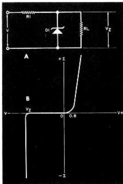
*Fig. 1. Zener-diode reference supply. The circuit is shown at A, while the characteristic curve is below at B. The fact that the zener voltage is dependent on temperature must be kept in mind in circuit design.*
