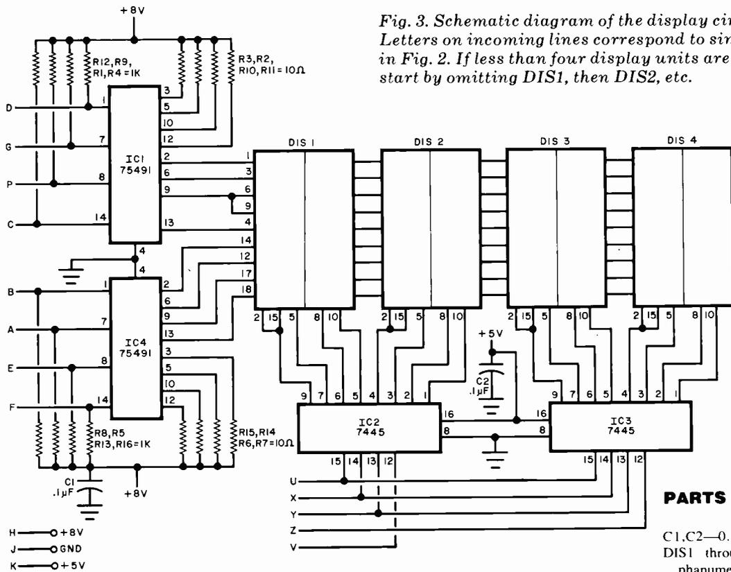
Fig. 3. Schematic diagram of the display circuit. Letters on incoming lines correspond to similar points in Fig. 2. If less than four display units are used, start by omitting DIS1, then DIS2, etc.
