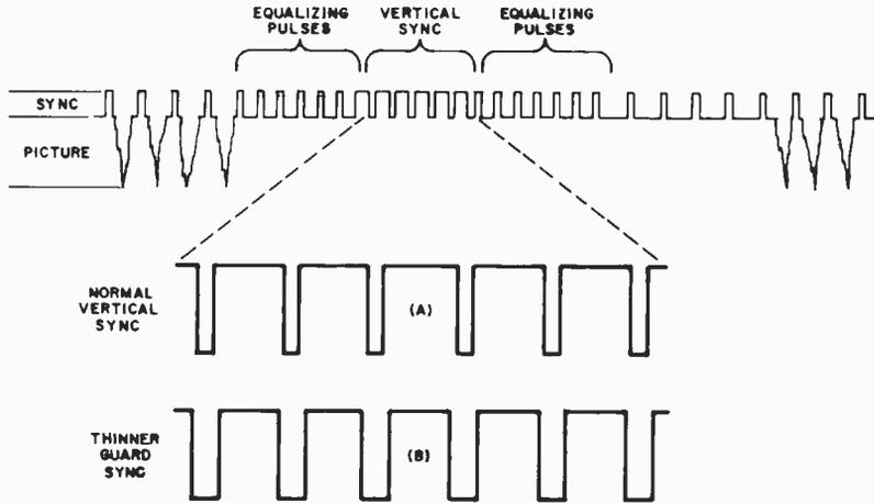
Fig. 2. Top trace shows standard sync pulses and picture signals. Contrast between normal vertical sync and thinner guard sync are illustrated in (A) and (B).
