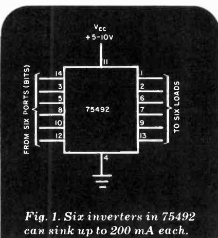
**Fig. 1.** Six inverters in 75492 can sink up to 200 mA each.
