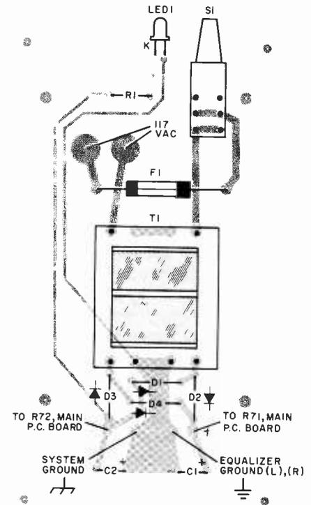
Fig. 9. Component placement for the ac power supply.
