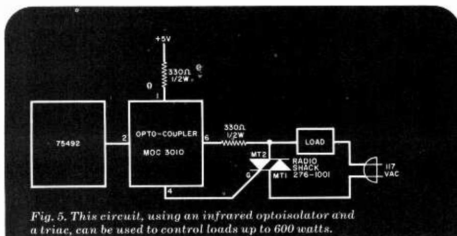
Fig. 5. This circuit, using an infrared optoisolator and a triac, can be used to control loads up to 600 watts.
