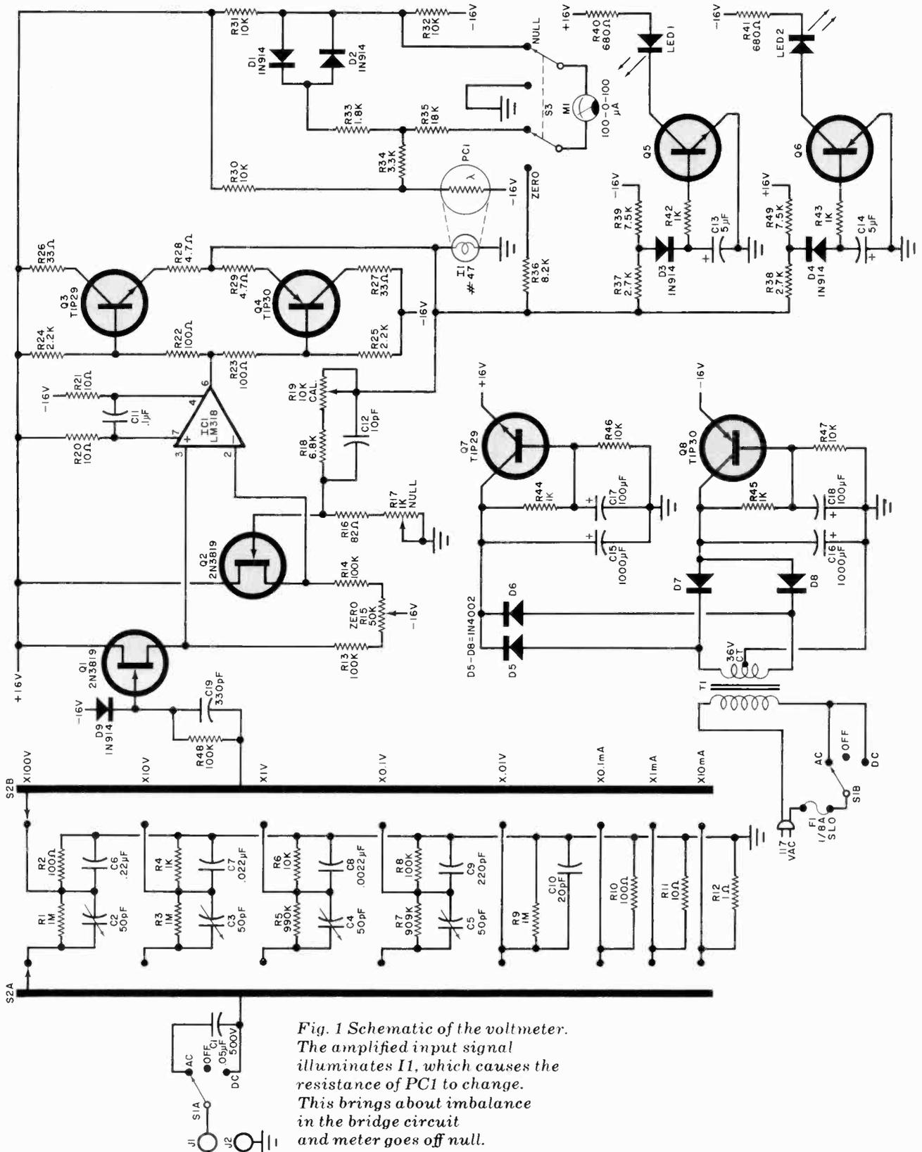
*Fig. 1 Schematic of the voltmeter. The amplified input signal illuminates I1, which causes the resistance of PC1 to change. This brings about imbalance in the bridge circuit and meter goes off null.*
