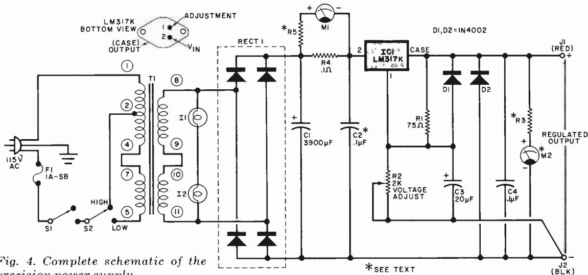
Fig. 4. Complete schematic of the precision power supply.
