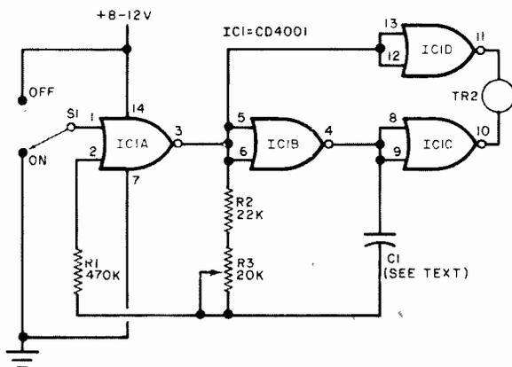
Fig. 2. This ultrasonic transmitter employs four NOR gates.
