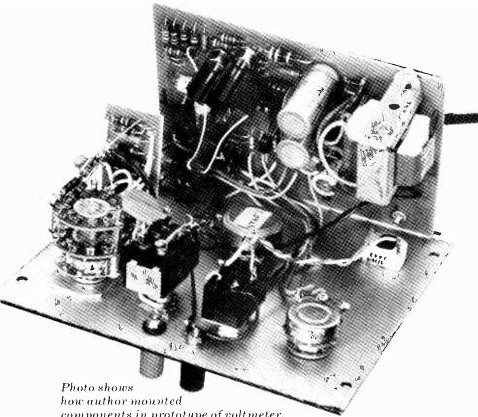
Photo shows how author mounted components in prototype of volt meter.
