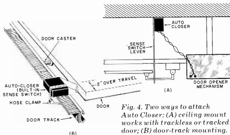
Fig. 4. Two ways to attach Auto Closer: (A) ceiling mount works with trackless or tracked door; (B) door-track mounting.
