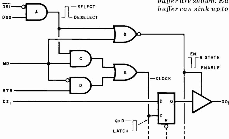
through buffer, to name just a few of its applications. This high-speed Schottky TTL device includes eight data latches and output buffers that can be tri-stated (switched to high impedance). Each buffer can sink up to 15 mA.
