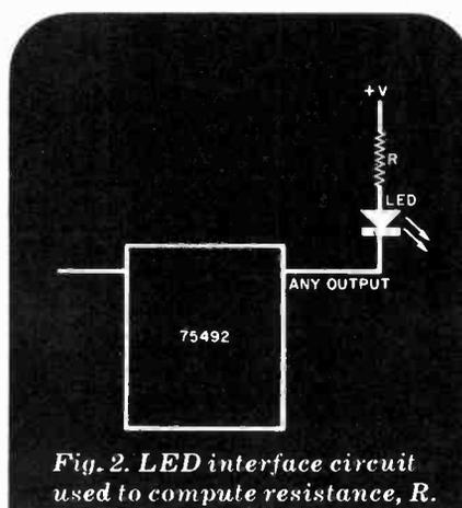
**Fig. 2.** LED interface circuit used to compute resistance, R.
