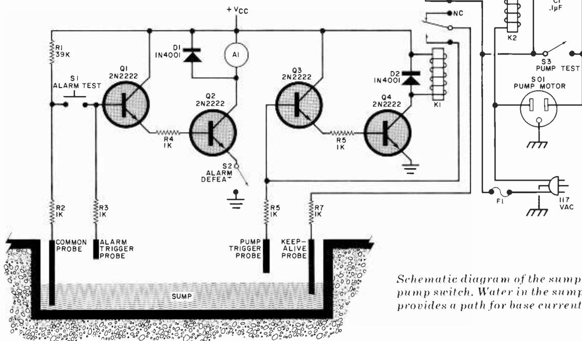
Schematic diagram of the sump pump switch. Water in the sump provides a path for base current.
