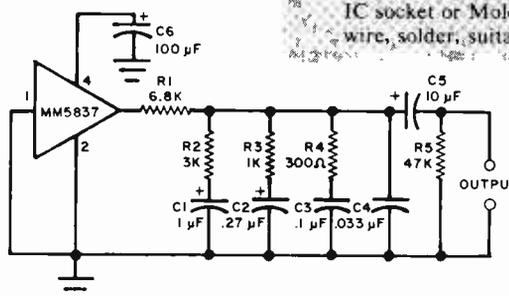
Fig. 2. Schematic diagram of the pink noise generator.
