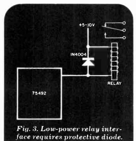
**Fig. 3.** Low-power relay interface requires protective diode.
