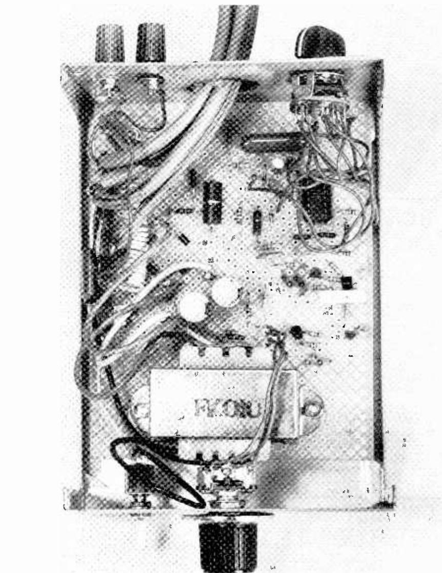
*Photograph of the author's prototype which was built on perf board, though a printed circuit board is recommended. The binding posts and switch on the rear were used for testing during design.*
