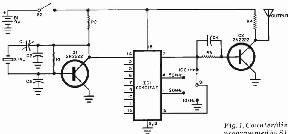
*Fig. 1. Counter/divider IC1 can be programmed by S1 to provide marker frequencies at selected intervals.*
