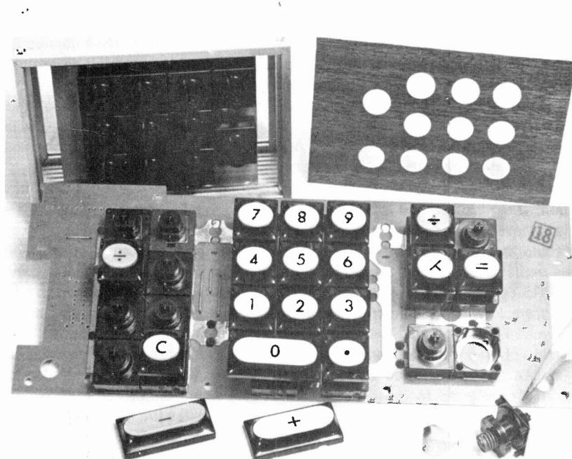
*Desktop calculator keyboard can be cut apart to make smaller keypads. The pencil at right points to removed top part of keyswitch. Topside brass stampings form part of switch and key strings.*
