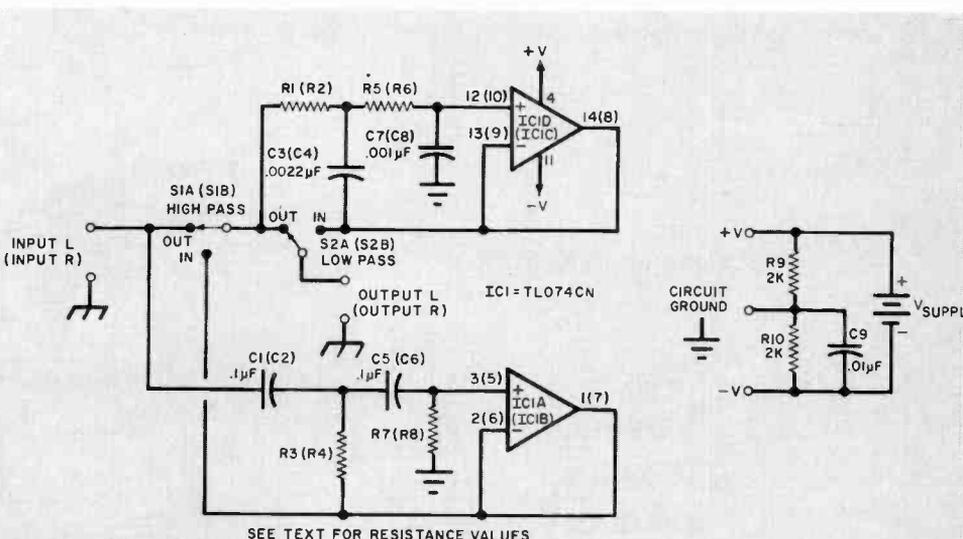
Fig. 2. Schematic diagram of the complete project.
