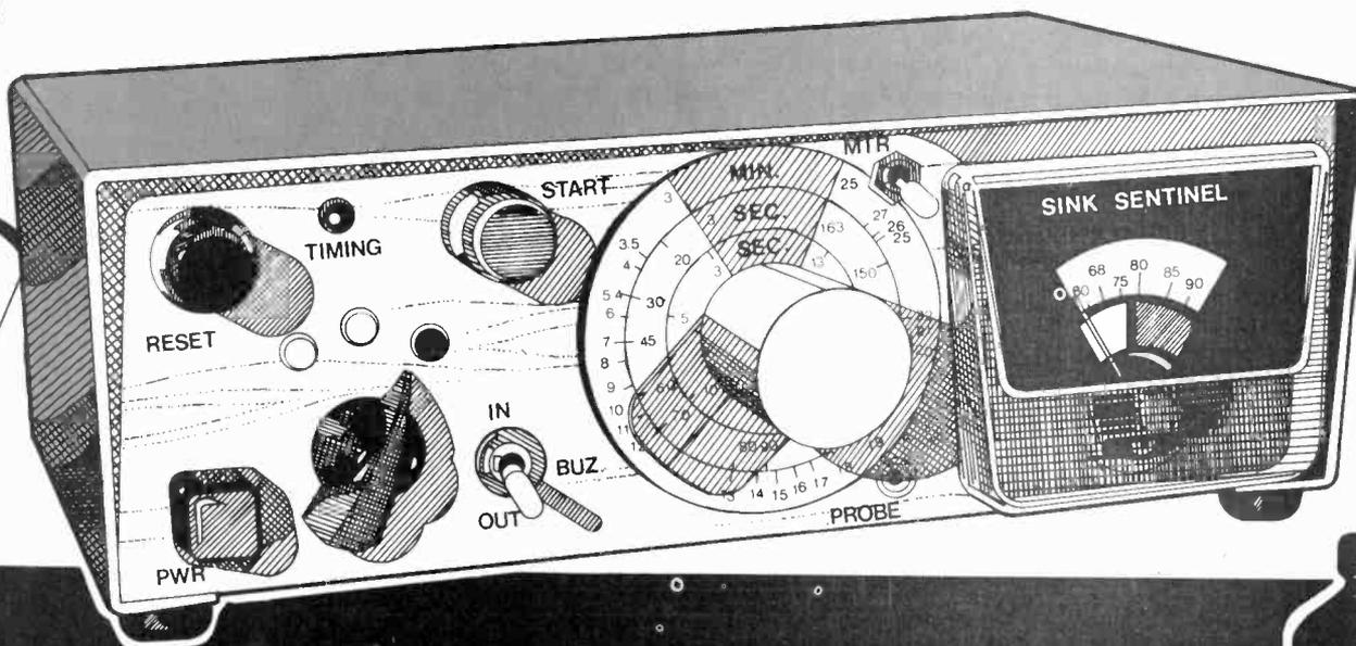
and C values shown in Fig. 1 were set in three ranges. The first and most commonly used for photographic printing and enlarging is from about 3 to 23 seconds; the second from 20 seconds to nearly 3 minutes; and the last from 3 to almost 30 minutes. If desired, the R and C values can be changed to produce any desired timing interval.
