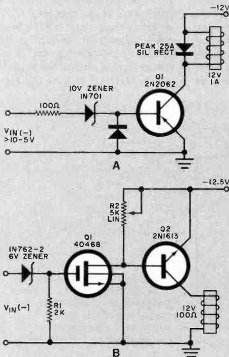
Fig. 5. Driver circuits with close differential operation:
