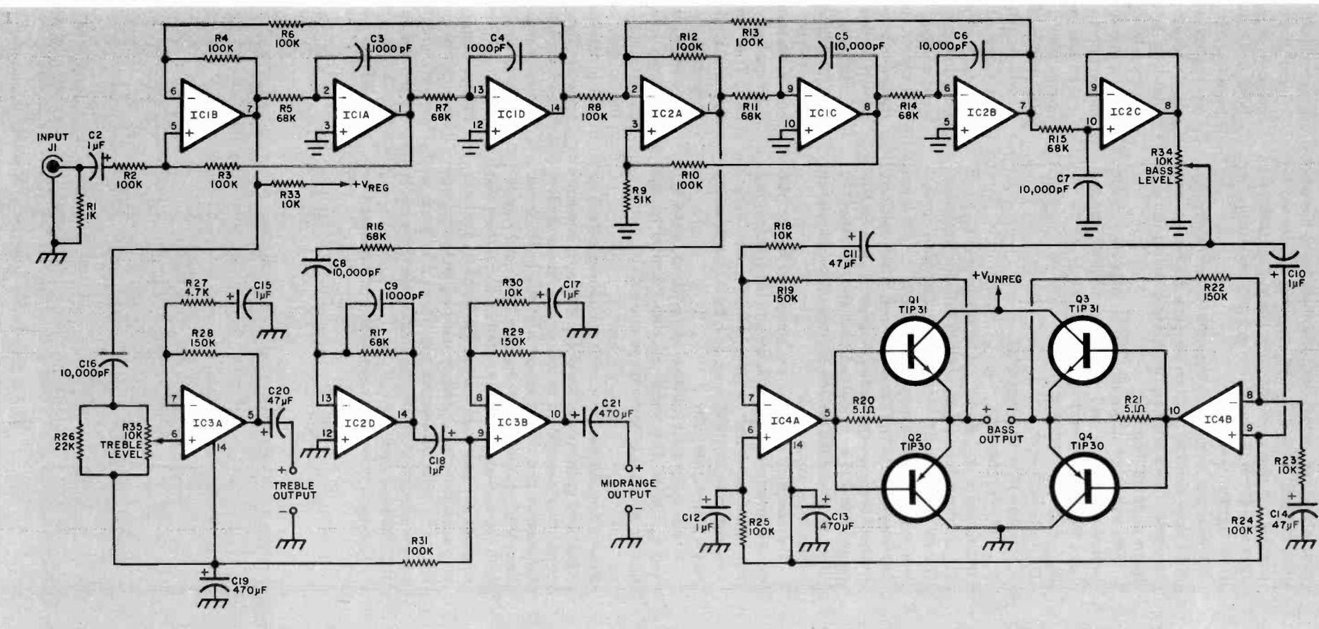
then divides the low and middle frequencies. The high, middle, and low frequencies, which appear at the outputs of IC1B, IC2A, and IC2B, respectively, are fed to passive high-pass and low-pass filters C16, R26, and R35 and C7, R15 and to active band-pass filter C8, R16, C9, R17, and IC2D.
