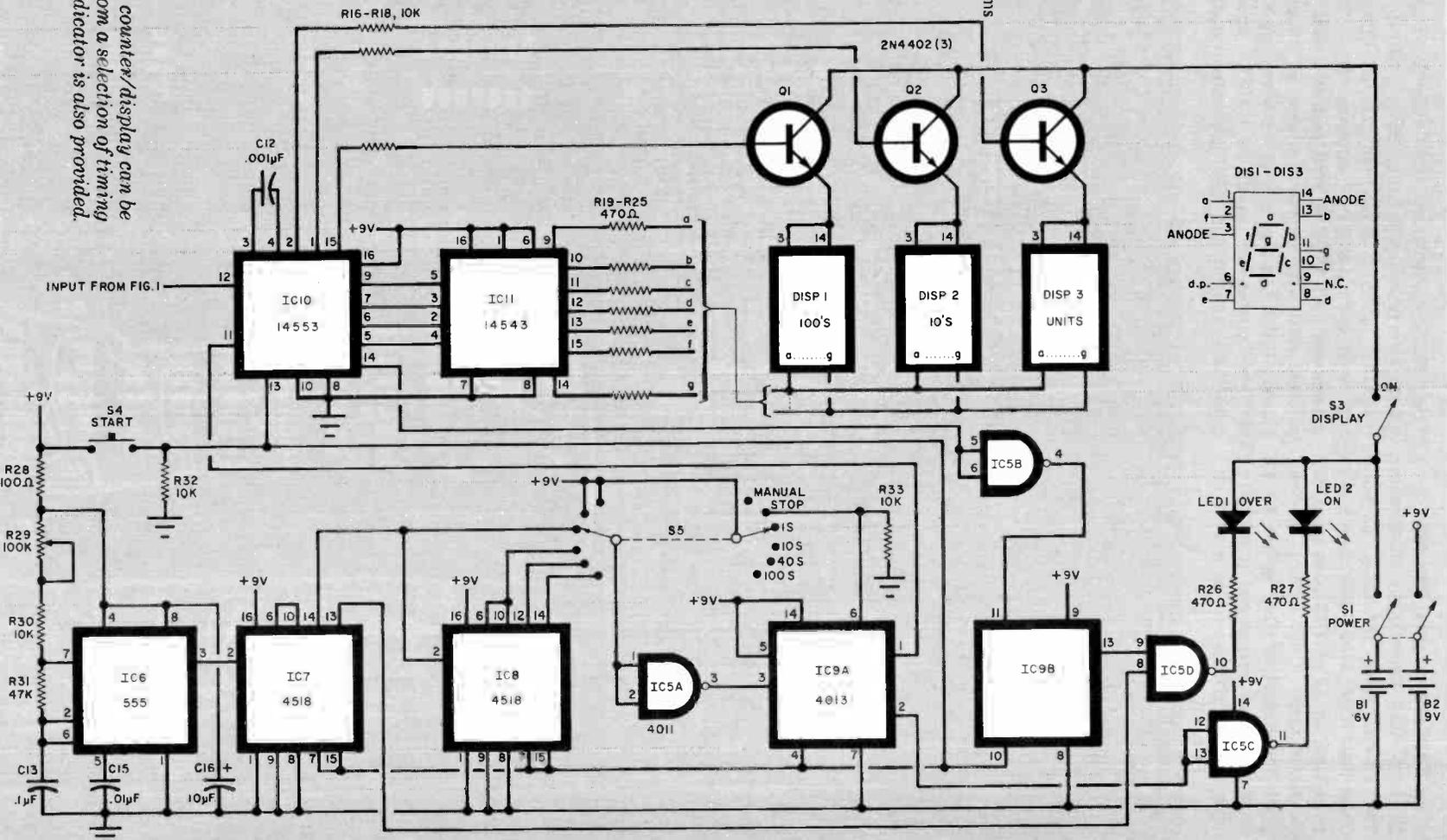
*Fig. 2. The conventional 3-digit counter/display can be enabled either manually or from a selection of timing signals. A blinking overrange indicator is also provided.*
