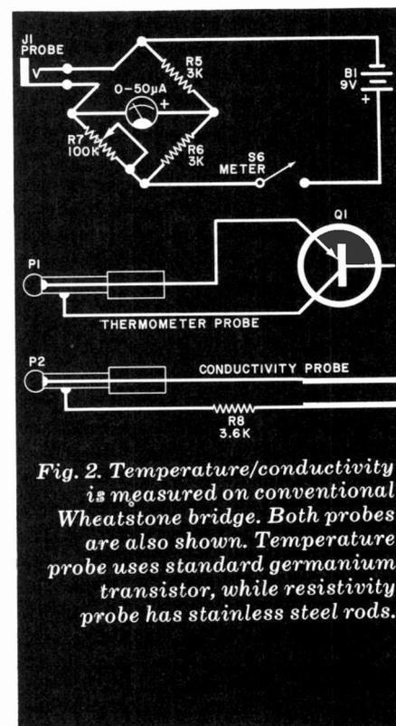
*Fig. 2. Temperature/conductivity is measured on conventional Wheatstone bridge. Both probes are also shown. Temperature probe uses standard germanium transistor, while resistivity probe has stainless steel rods.*
