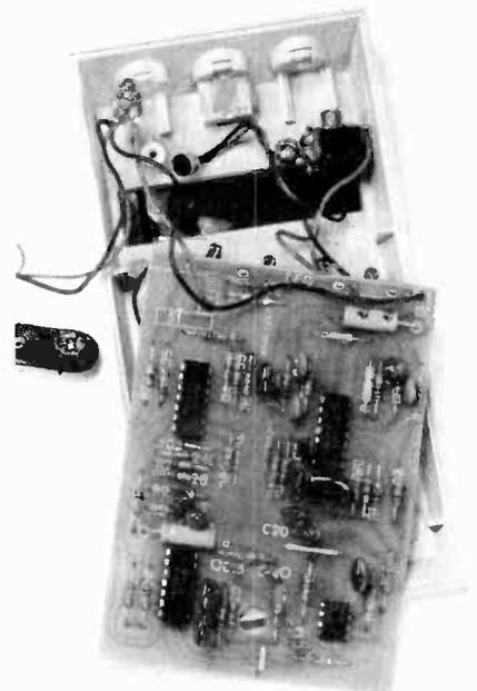
*LEDs are positioned in window area, miniature microphone is put in center cutout at top of case.*
