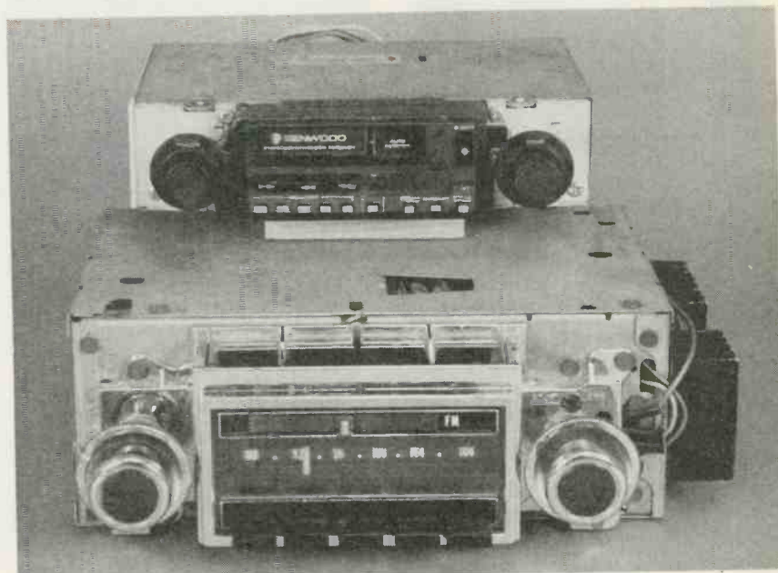
FIG. 5—CONTRAST IN CASE SIZE. A modern automotive AM/FM stereo case with an audio tape deck atop a 23-year old AM/FM radio.
