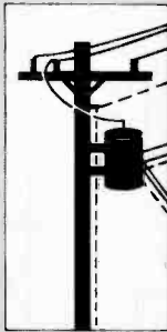
DISTRIBUTION STEP-DOWN TRANSFORMER 0.1-1μT, WITH A FAST MAGNETIC FIELD DROP-OFF AT 1/r^3
