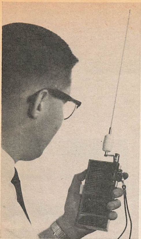
Walkie-talkies may be incorporated in your CB system if they can meet certain FCC specifications. Note in this photo that the old sixty-inch antenna has been replaced with a Hy-Gain loaded whip.
