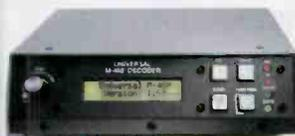
The **Universal M-450v1.5** reader copies: **Baudot, SITOR, FEC-A, ASCII, SWED-ARQ** and **Weather FAX** (to printer port) plus the **ACARS** aviation teletype mode. Features a big two-line, 20 character LCD and bidirectional parallel port. Operates from 12 VDC or supplied AC adapter. U.S.A. #0450 \$399.95 (+\$8)
