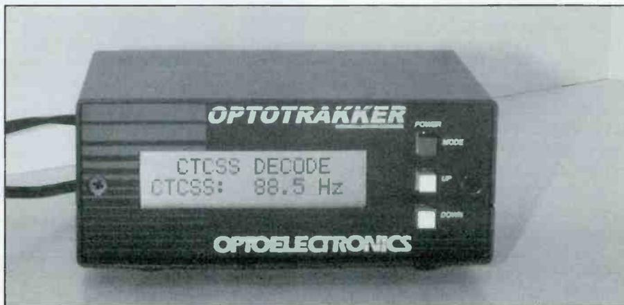
The Optotrakker makes a great add-on decoder to almost any radio. It also works with computer-controlled systems to add tone capabilities and trunking functions.
