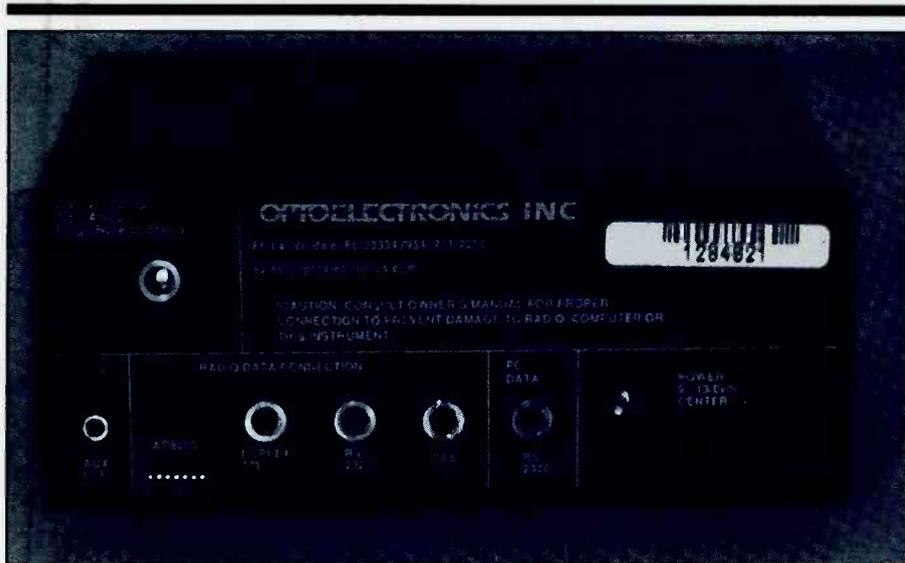
A myriad of connections is available on the rear panel, but unless you're using the unit under computer control, you'll only need power and audio at the upper left. Note the AR-8000 ribbon connector at the bottom left.
