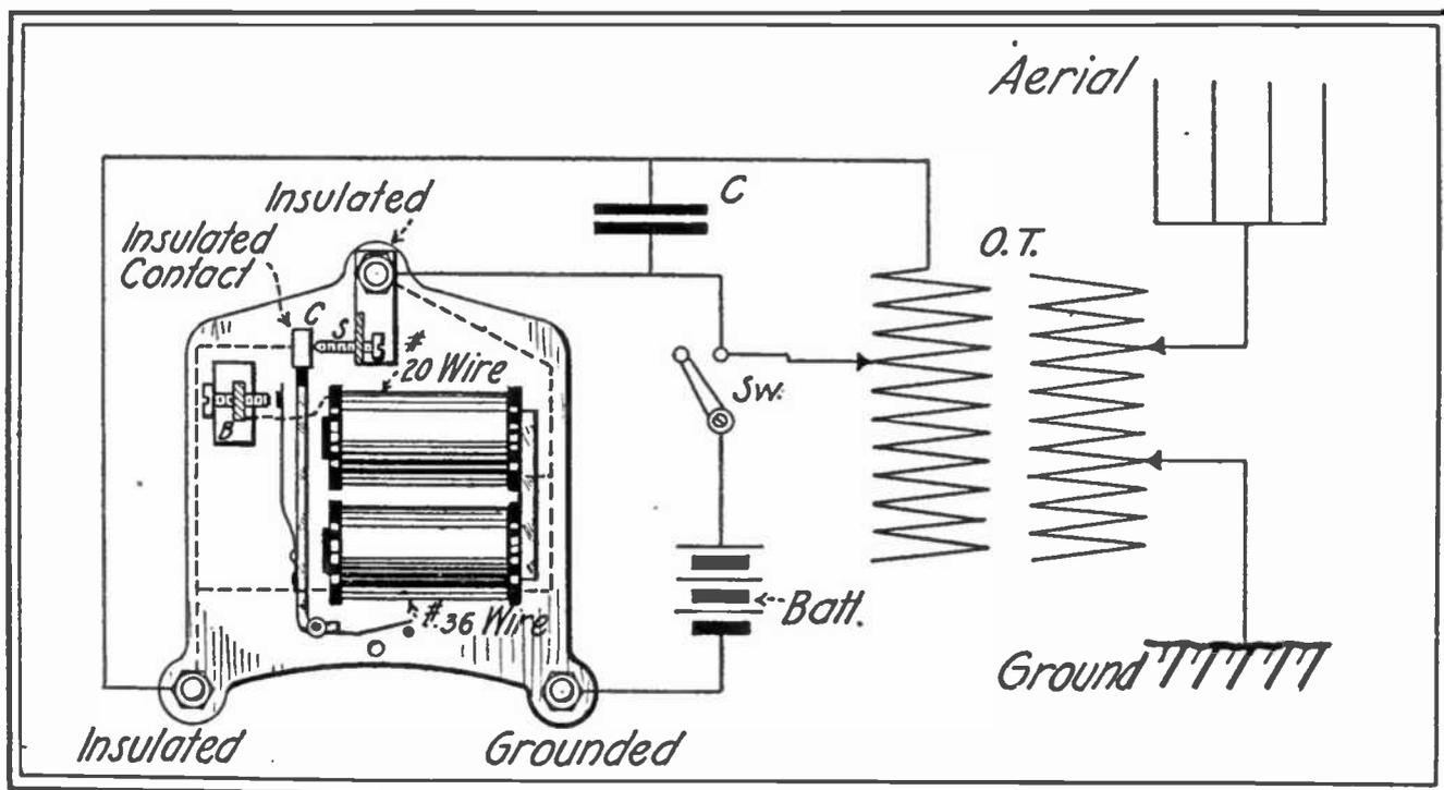
Hook-up for Buzzer Transmitting Set of Original Design. Such a Transmitter Will Emit Waves in Keeping with the Wireless Law Restrictions.
