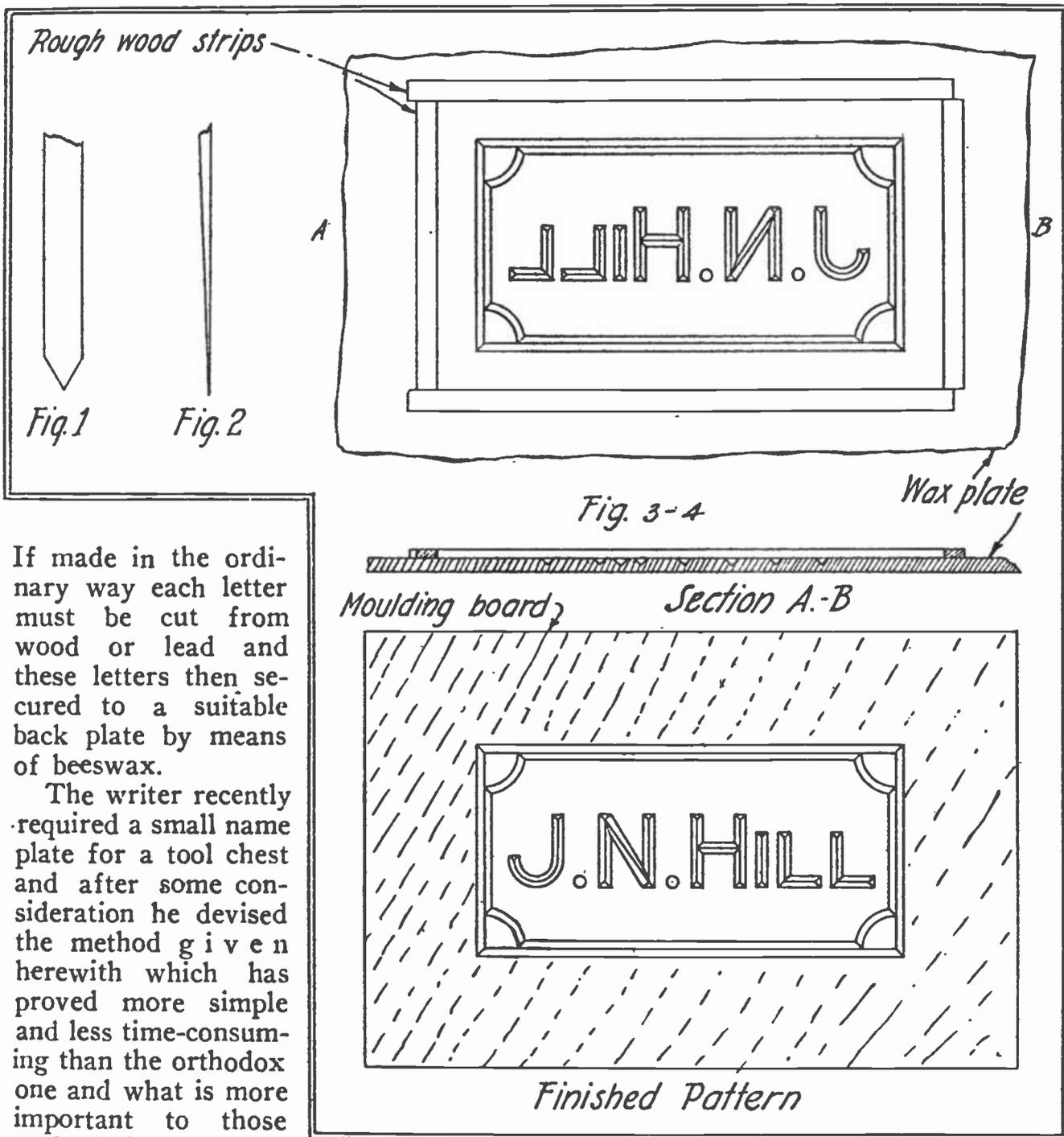
If made in the ordinary way each letter must be cut from wood or lead and these letters then secured to a suitable back plate by means of beeswax.
