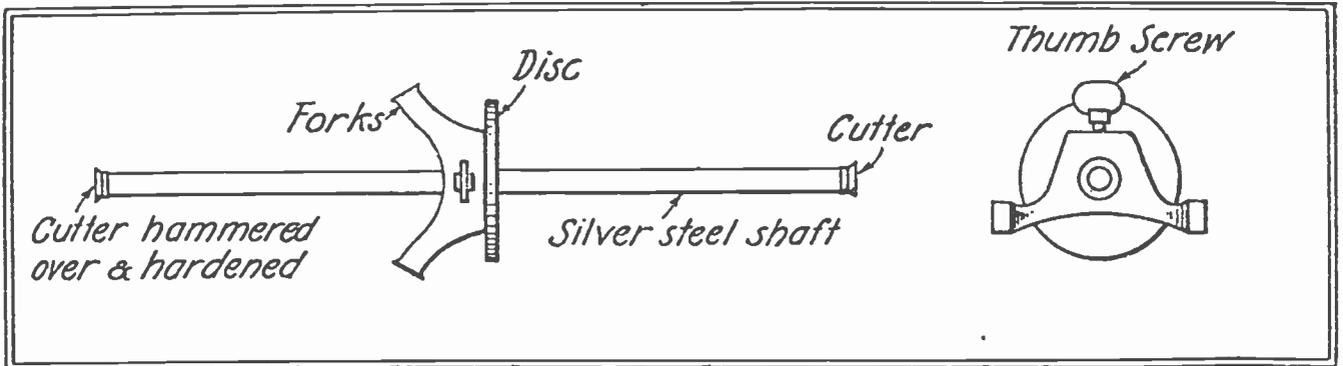
ters being also provided on the shaft. A pattern is required for the head—a useful lesson in small pattern making—and if the cutters are properly hardened the gauge may be used for marking metal as well as wood.
