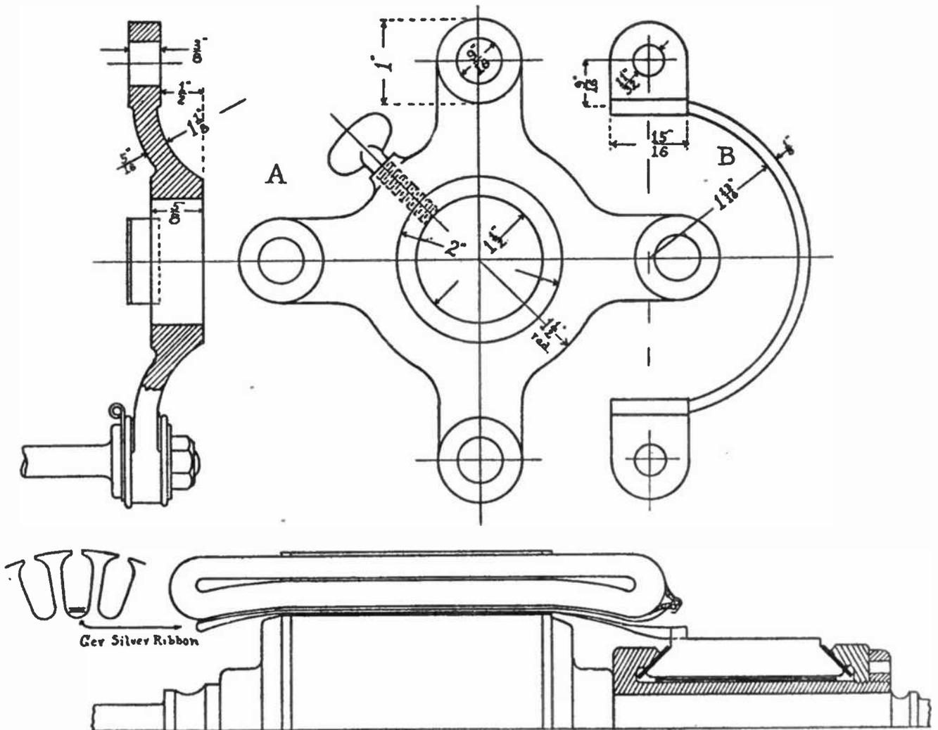
Fig. 47.—Details of Brush-holder Yoke, Cross Connector and Commutator Resistance Leads.
