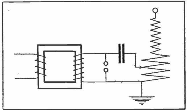
Fig. 15.—Diagram of an Oscillatory Circuit.
