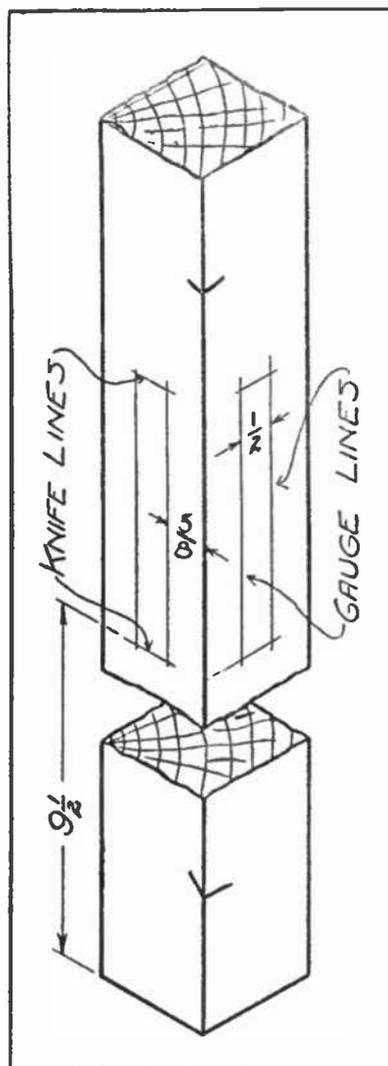
Fig. 5.—Layout for the Mortises.
