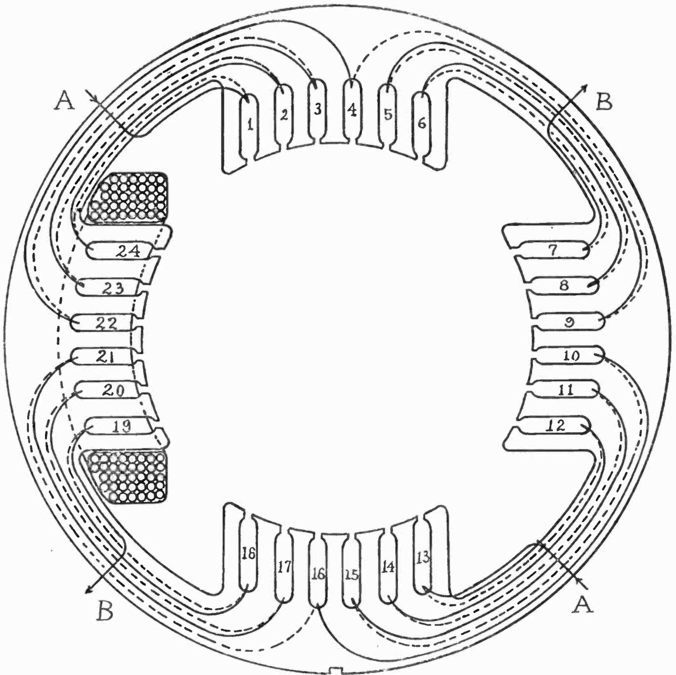
Fig. 46.—Diagram of Compensated Winding for Series Motor, showing also One of the Regular Field Spools in Position.
