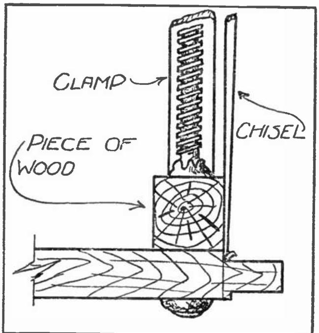
Fig. 3.—Suggestion for Chiseling Sharp Corner on Shoulder.
