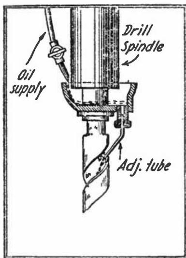
found around the shop. The main part is the oil cup. In this case the steam chamber from an old 1 1/4-inch steam whistle was employed. The threads were bored out and the hole tapered to slide
