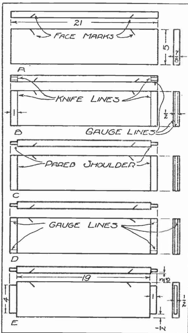
Fig. 1.—Methods of Cutting the Tenons on Chair Rails.
