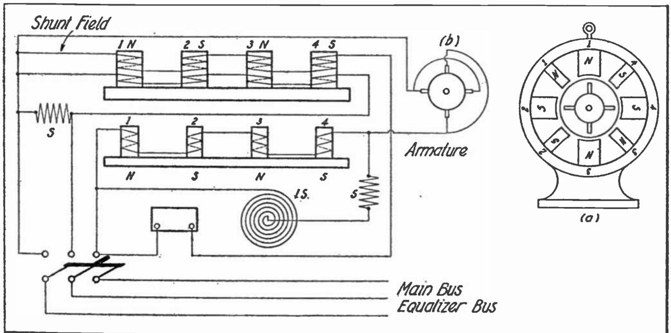
Wiring Scheme for an Interpole Dynamo.
