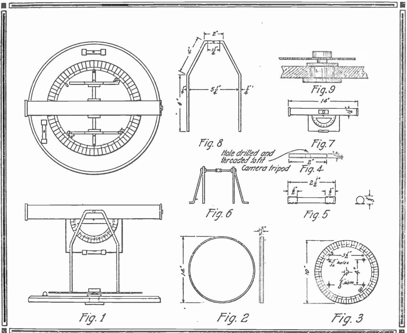
The oak disc should be turned true on a lathe and centered. With reference to Fig. 3 in the drawing the holes may be drilled in the piece of sheet brass as indicated and the brass disc fastened to the wood with small screws, making sure that the centers of the two discs coincide. The next opera-
