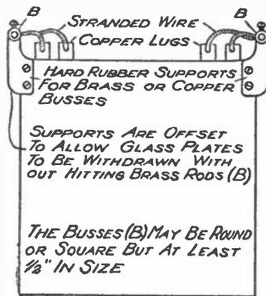
Fig. 8.—Method of Making Connections with Lugs.
