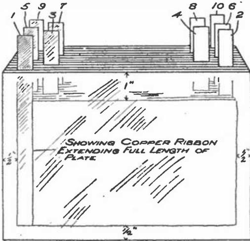
Fig. 1.—View of Glass Condenser Plates Assembled.
