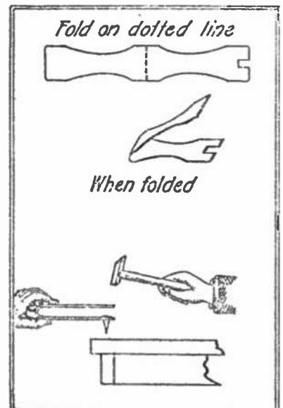
a bit of tin or cardboard. The nail or tack is inserted in the slot and the overlapping piece of metal serves to hold it by its head. This gives a sort of handle by means of which the tack can be held just where it is wanted and in a perfectly upright position, ready to be started with the first blow of the hammer. The holder can then be withdrawn and the tack driven home.
