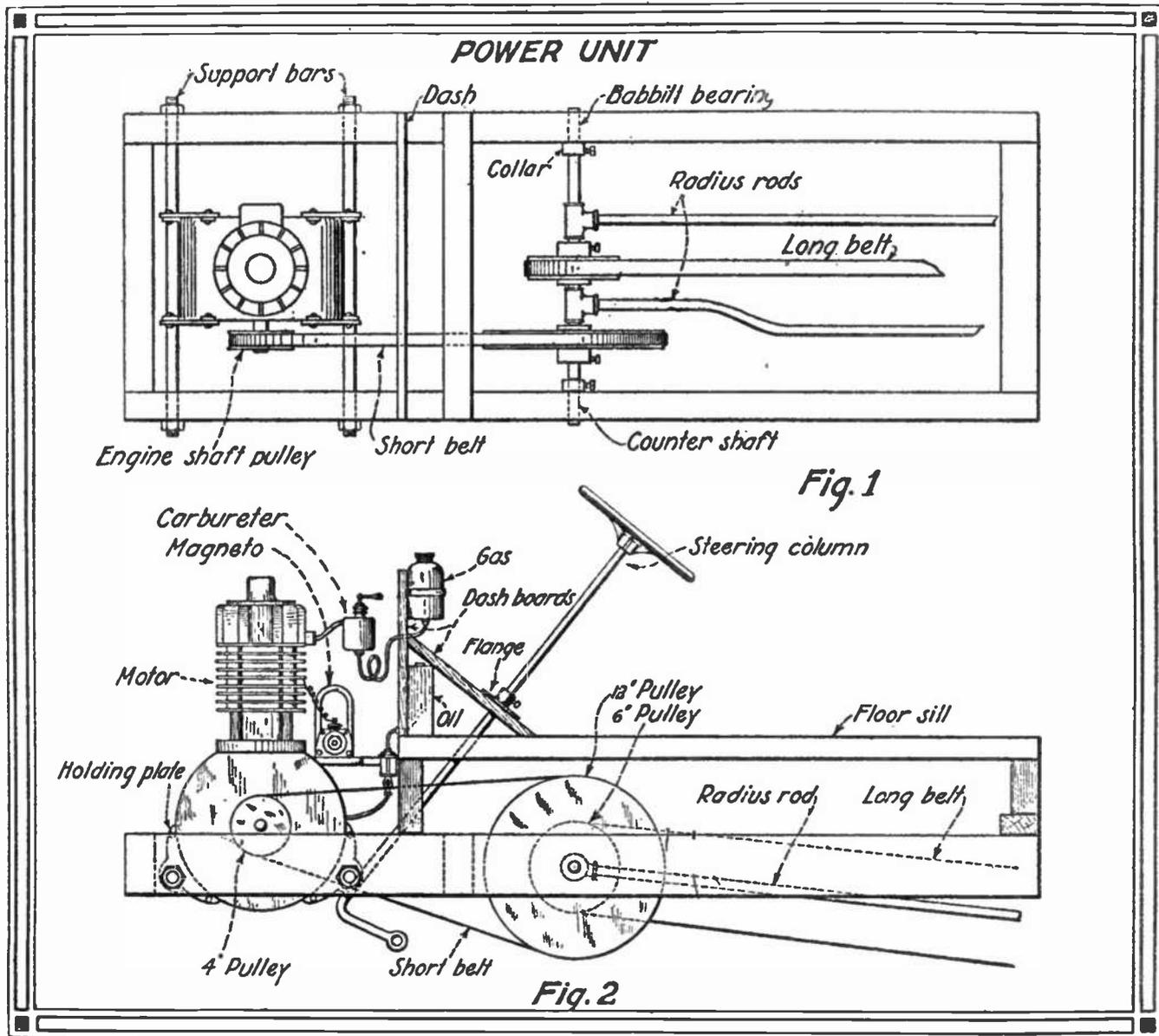
eters are based upon the assumption that the motor is capable of developing between four and five horsepower, which is the average performance of motors of this type. The belt pulley on the engine crankshaft is four inches in diameter and it drives to a pulley 12 inches in diameter; the ratio is obviously 3 to
