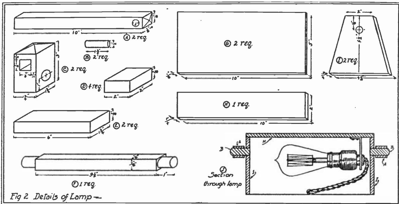
Details of Parts of Piano Lamp.
