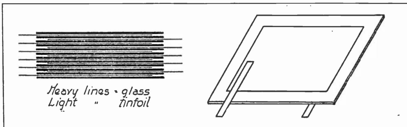
Showing Method of Assembling Plates of Condenser with Lugs Projecting. Also View of Single Plate of Glass with Tinfoil in Position.
