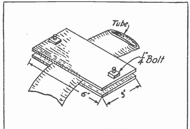
3 by 6 inch pieces of iron as shown in the accompanying sketch. The holes in the under piece should be a snug fit for the shoulder of the bolts, while those in the upper piece should be an easy clearance fit. It is preferable to employ wing nuts on the ends of the bolts in order that no wrench may be necessary for tightening.
