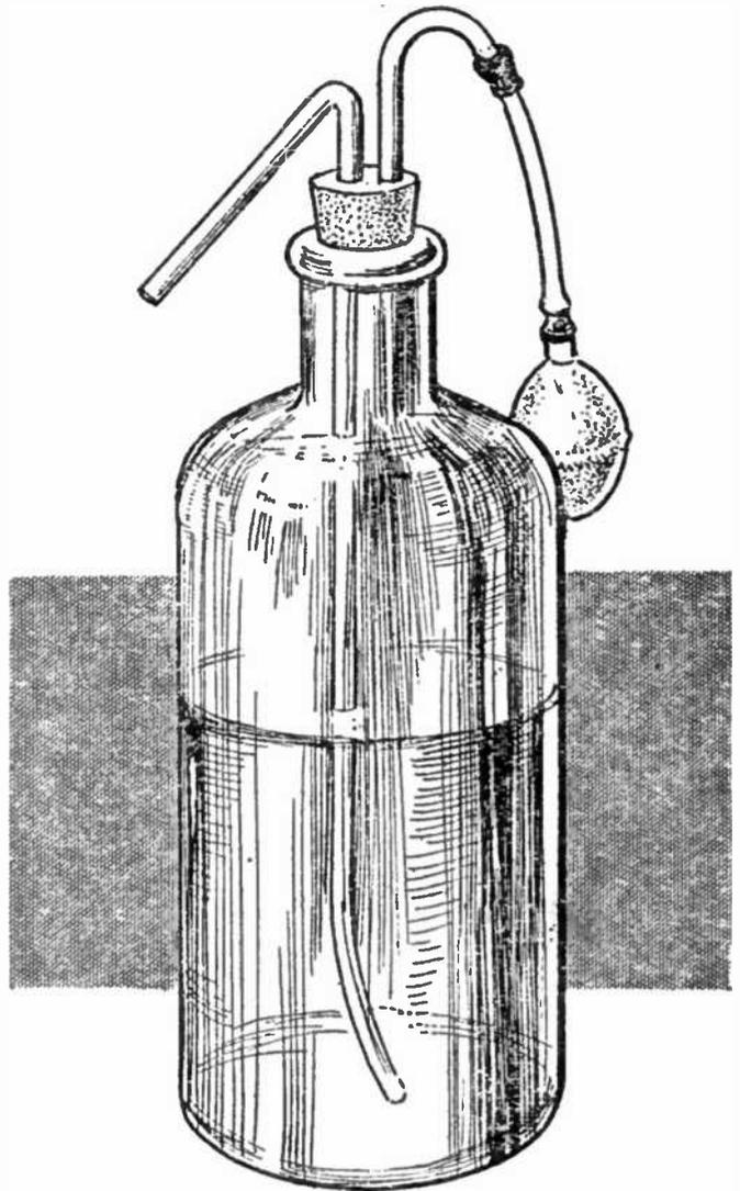
and an atomizer bulb. When the bulb is pressed air is forced into the bottle causing the water to flow into the prescription bottle held under outlet tube.
