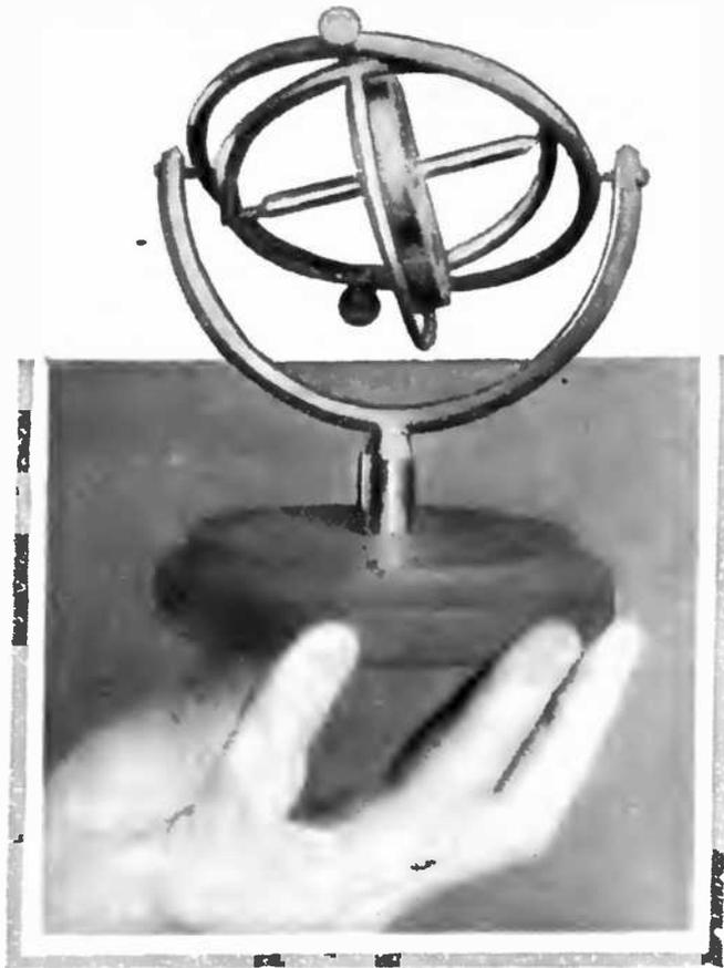
The Simple Toy Gyroscope—the Principle of which is Applied for Opening Ice-bound Waters to Navigation.
