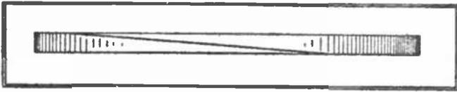
ting the joint as long and slim as possible as indicated in the sketch. The longer the cut, the narrower the crack after the cylinder wears a trifle.
