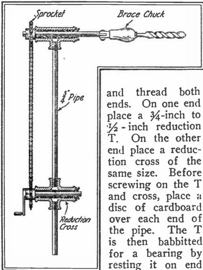
and thread both ends. On one end place a 3/4-inch to 1/2-inch reduction T. On the other end place a reduction cross of the same size. Before screwing on the T and cross, place a disc of cardboard over each end of the pipe. The T is then babbitted for a bearing by resting it on end on a paper pad and
