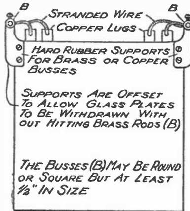
Fig. 8.—Method of Making Connections with Lugs.
