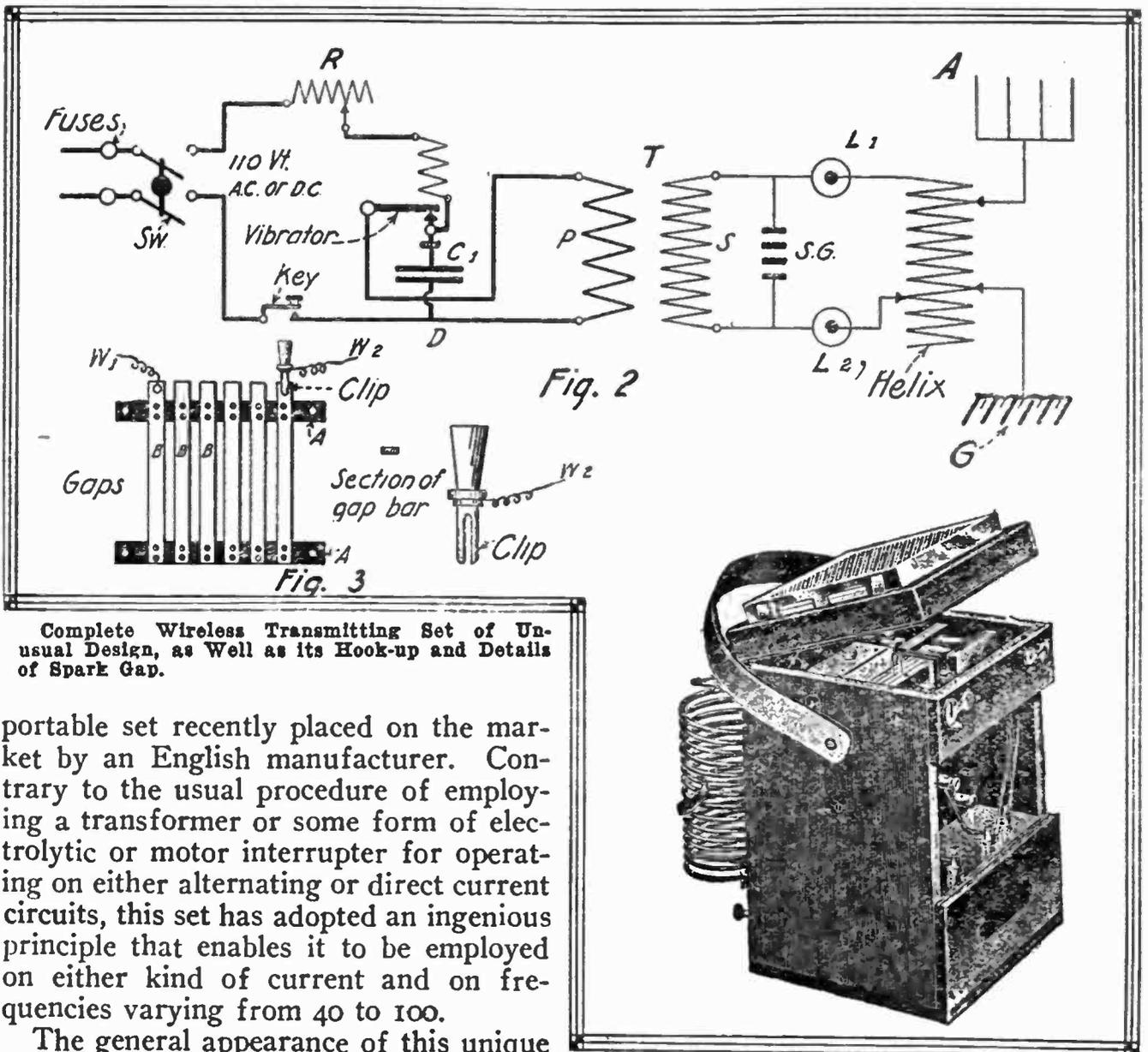
Complete Wireless Transmitting Set of Unusual Design, as Well as its Hook-up and Details of Spark Gap.
