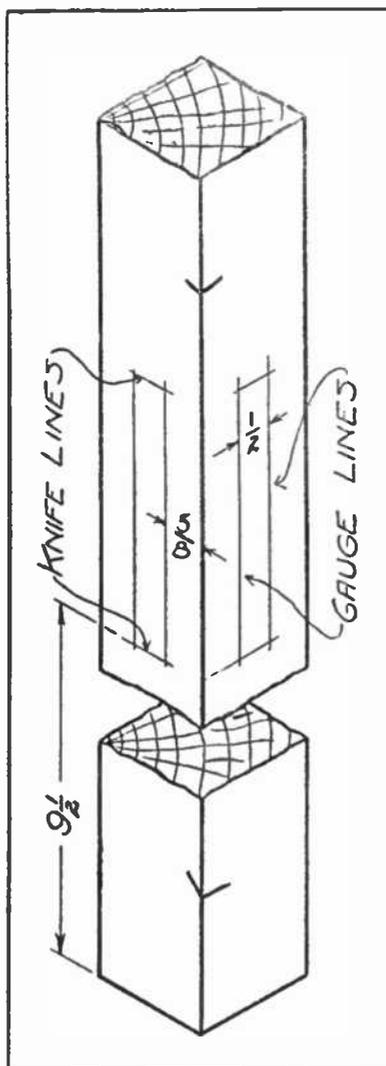
Fig. 5.—Layout for the Mortises.
