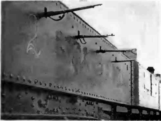
Armored train at Ypres with rifles projecting through the loop holes in its sides. The Belgian army has employed a large number of these armored trains with telling results. The rifemen are secure from hostile rifle fire yet capable of meting out severe punishment to their opponents.
