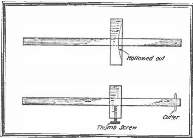
ture of a little time and trouble. The improvement consists simply in cutting a hollow out of the face of the head as shown in the drawing. The gauge may
