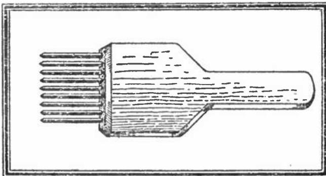
corners with a knife or file. Drive a row of ten penny finishing nails into the end of the broad part near enough together to let the shank of a six or eight penny nail enter, but not far enough apart to permit the heads to pass
