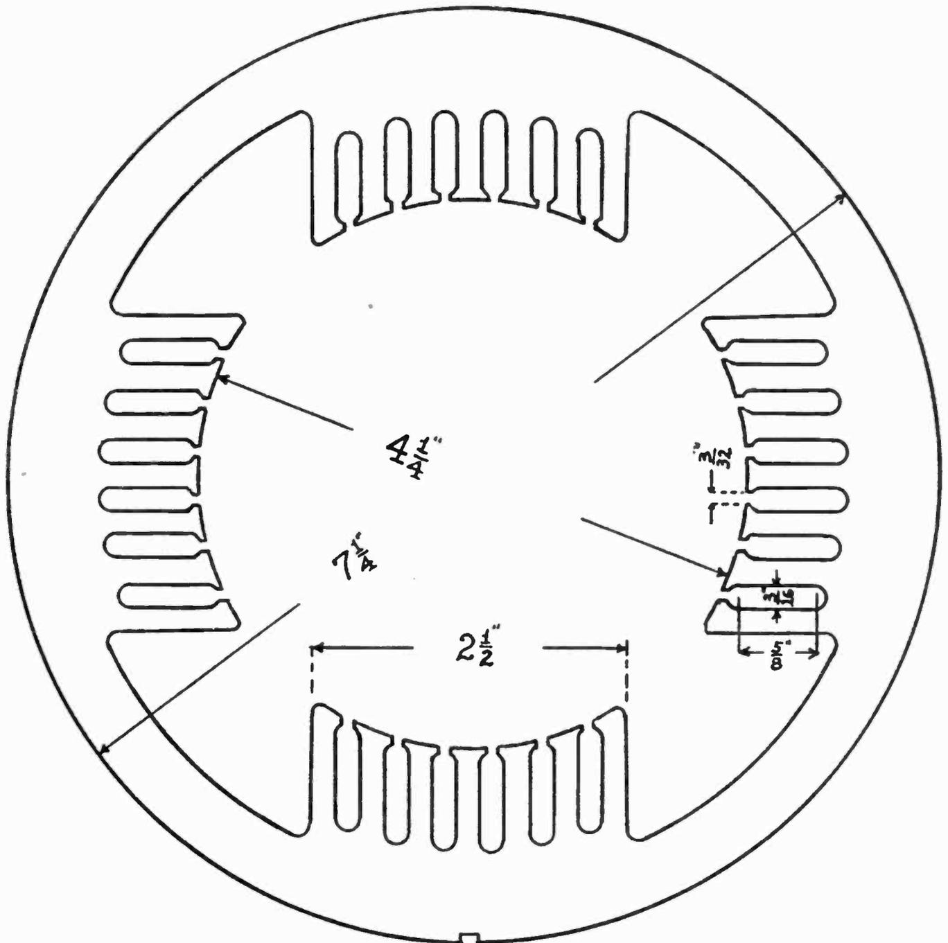
Fig. 45.—Field Punching for Compensated Series Motor.
