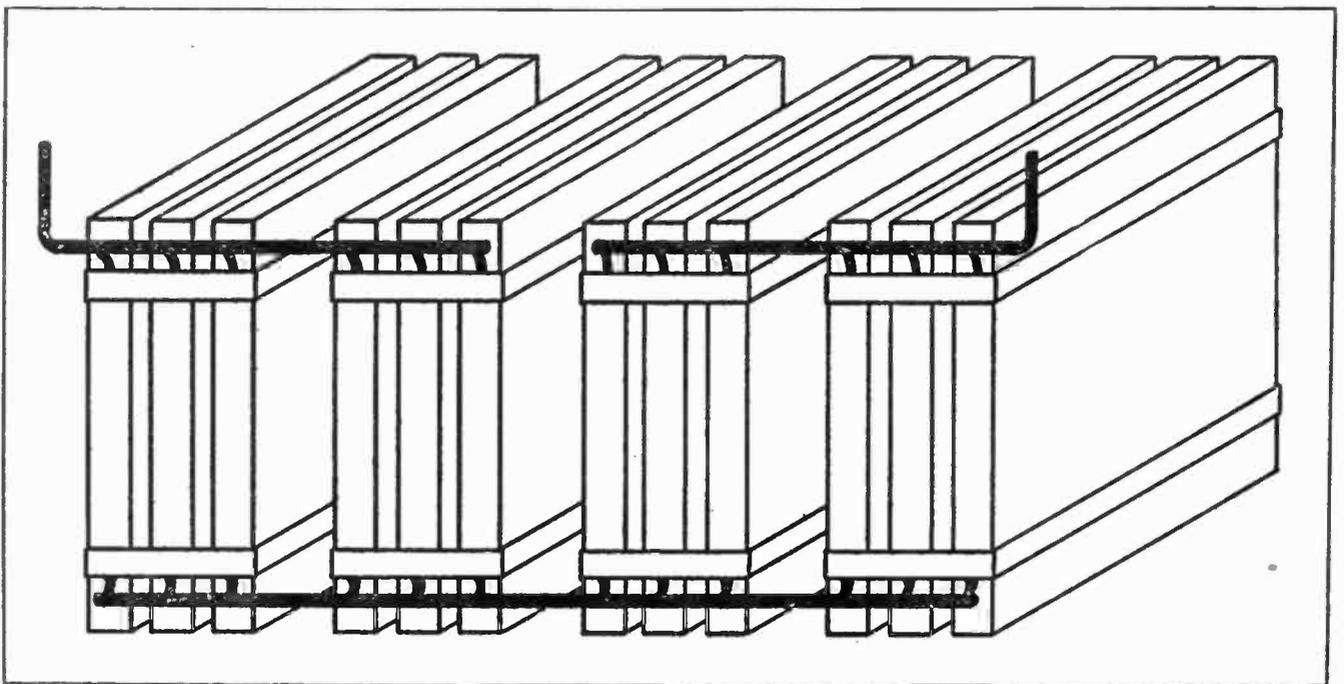
Complete Condenser, Showing Method of Connecting.
