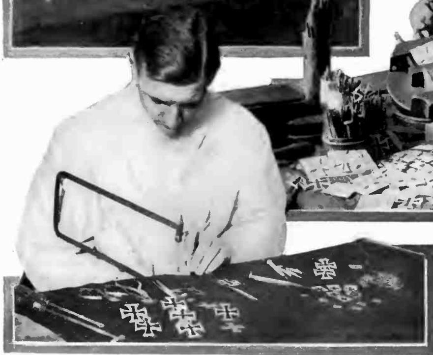
Using a scroll saw in order to cut out from a silver sheet the silver edge of the Iron Cross. Previously, the silver squares have been punched to shape.
