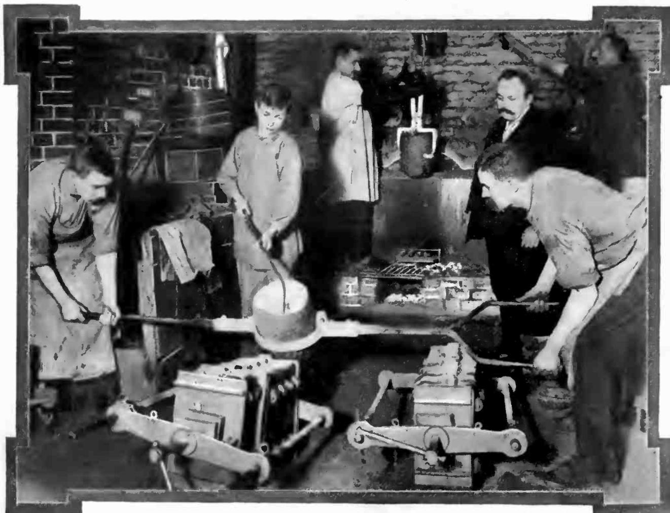
Pouring the Molten Iron Into Molds for Casting the Center Portion of the Iron Cross.
