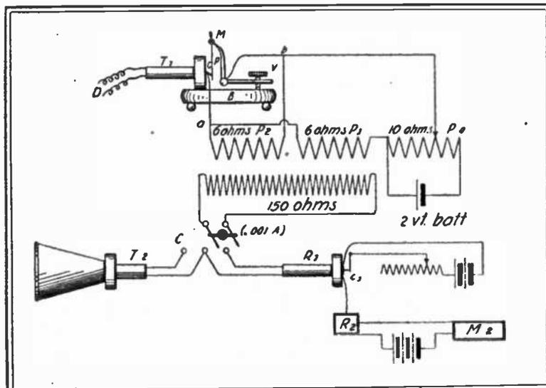
Wiring Diagram of New Wireless Recording Apparatus.
