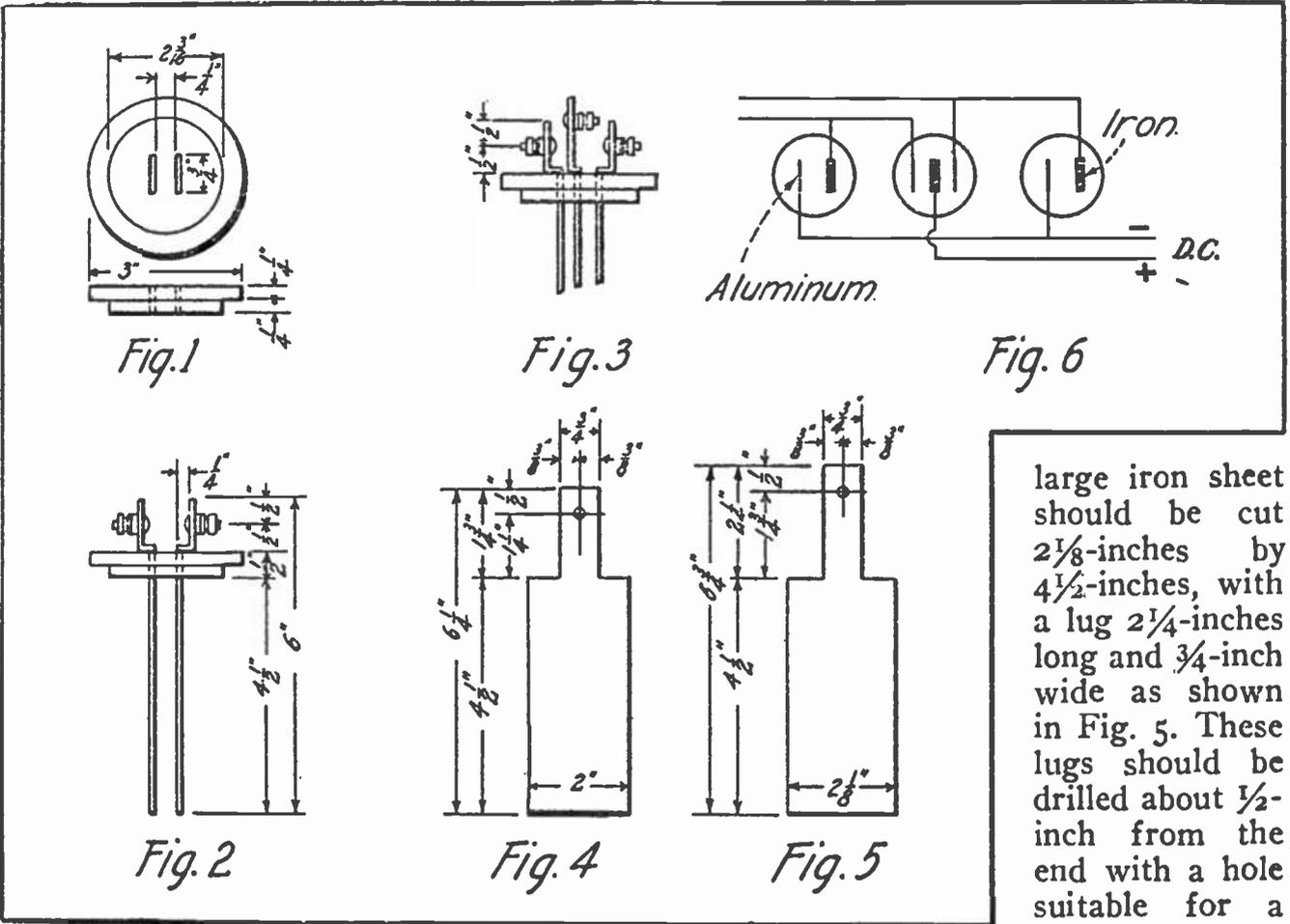
large iron sheet should be cut  $2\frac{1}{8}$ -inches by  $4\frac{1}{2}$ -inches, with a lug  $2\frac{1}{4}$ -inches long and  $\frac{3}{4}$ -inch wide as shown in Fig. 5. These lugs should be drilled about  $\frac{1}{2}$ -inch from the end with a hole suitable for a binding post.
