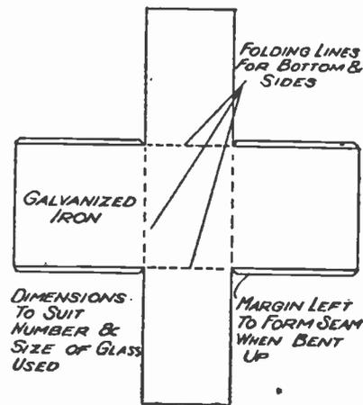
Fig. 2.—Pattern for Condenser Tank.
