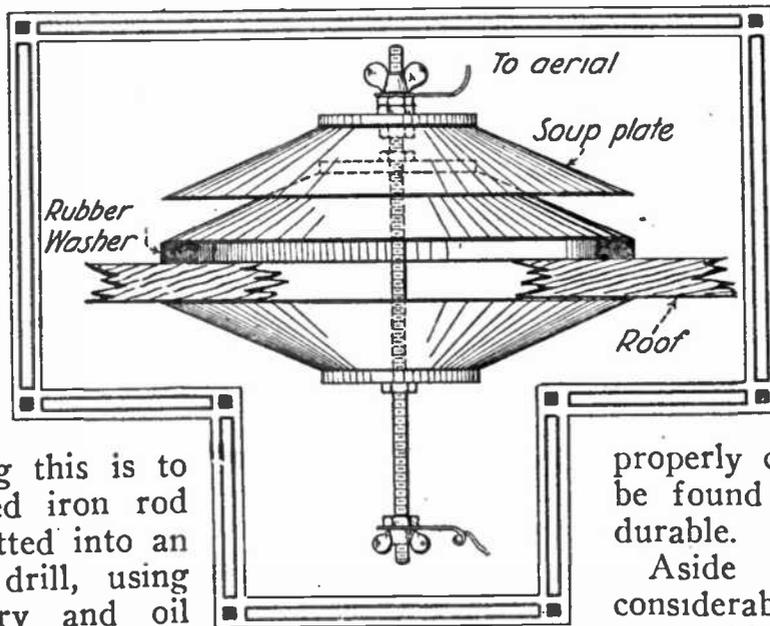
Diagram of Inexpensive Roof Insulator.
