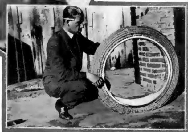
A View of the new steel tire, as well as a single section of interlocking pieces.
