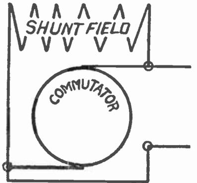
Fig. 16.—Connections for the Generator.
