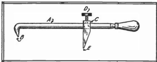
steel  $\frac{1}{4}$  inch thick,  $\frac{3}{8}$  inch wide and one inch long, sharpened to a cutting edge at *E*. A hole is drilled to pass the  $\frac{1}{4}$  inch rod and in the top of the cutter another hole is drilled and tapped for the set screw *D*. A handle fitted to
