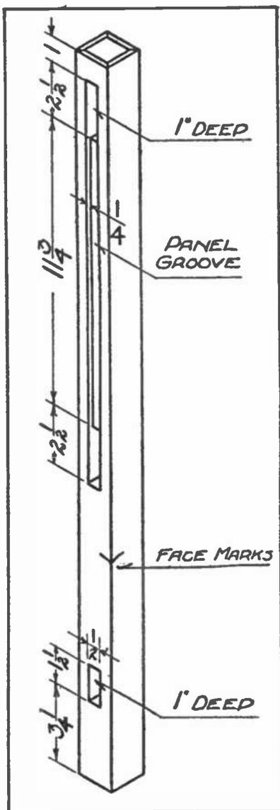
Fig. 1.—Detail of Inside Corner of Leg.
