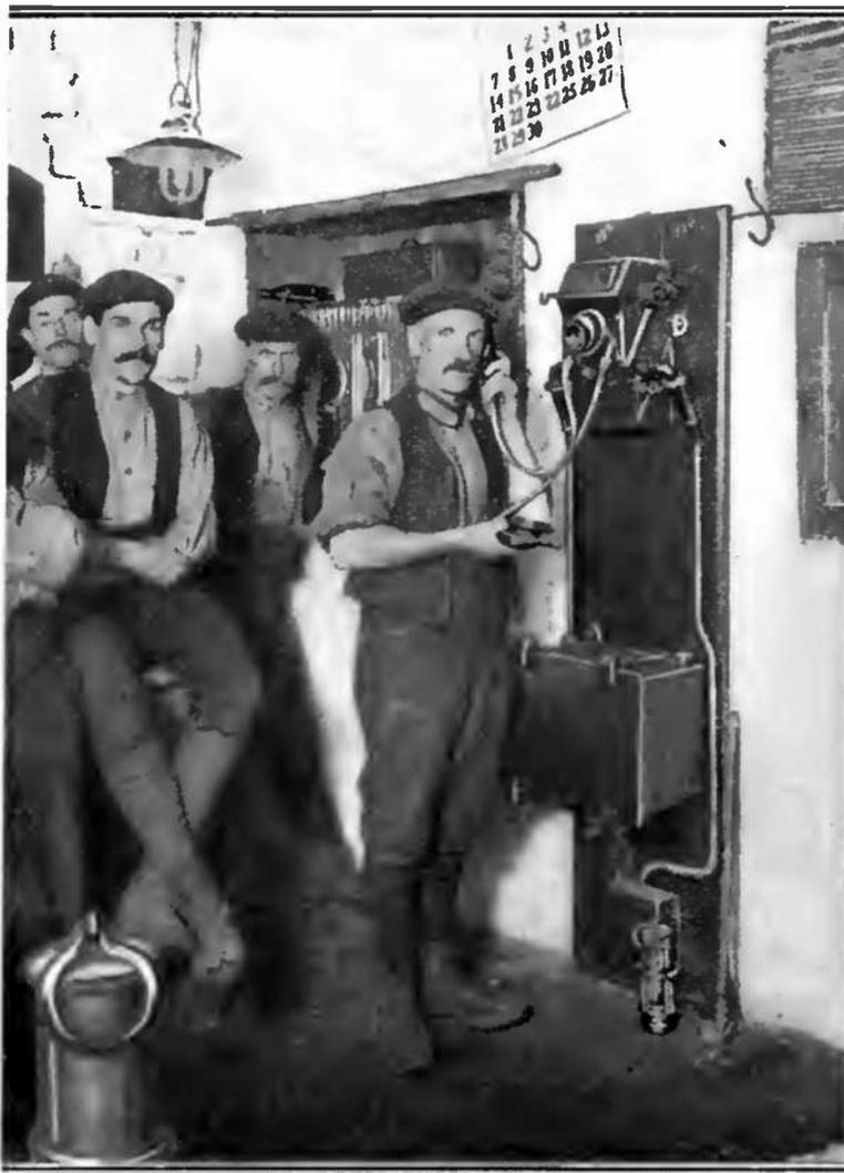
In Many German Mines a System of Wireless Telephony is Employed; the Rails and Pipes through the Mine Conveying the Current Between the Instruments.
