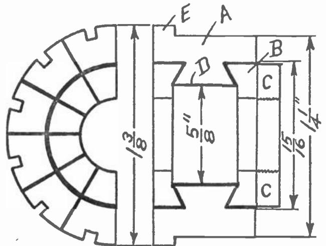
Fig. 10.—A Cross Section of the Commutator and One of its Segments.
