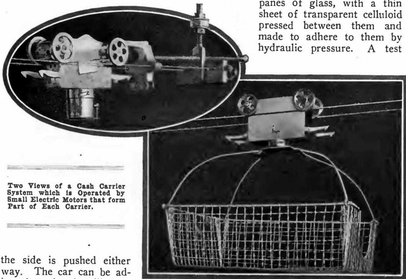
Two Views of a Cash Carrier System which is Operated by Small Electric Motors that form Part of Each Carrier.
