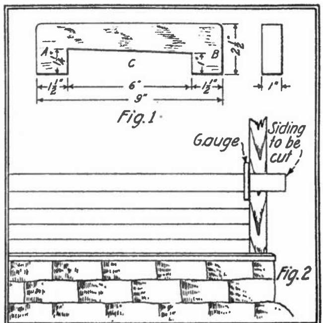
siding on a house, is readily made by the carpenter. A piece of wood is cut as shown in Fig. 1, which shows the utter simplicity of the device. In use, the parts marked *A* and *B* rest against the upright corner board of the house, allowing the piece of siding to be cut to pass through the open part *C*, as in Fig. 2. The piece is then marked with pencil or knife.
