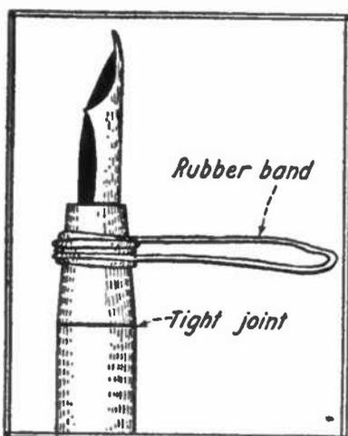
become firmly stuck together, wind a rubber band around the neck several times, keeping it tightly stretched while winding. The rubber will provide a grip that enables the user
