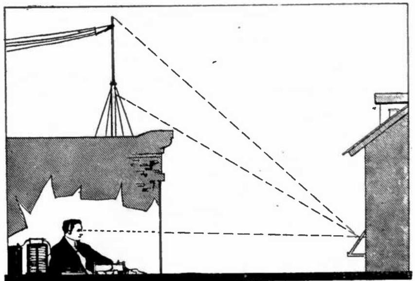
Without Leaving His Seat, an Amateur Operator Can See His Aerial by Means of a Simple Mirror Device.
