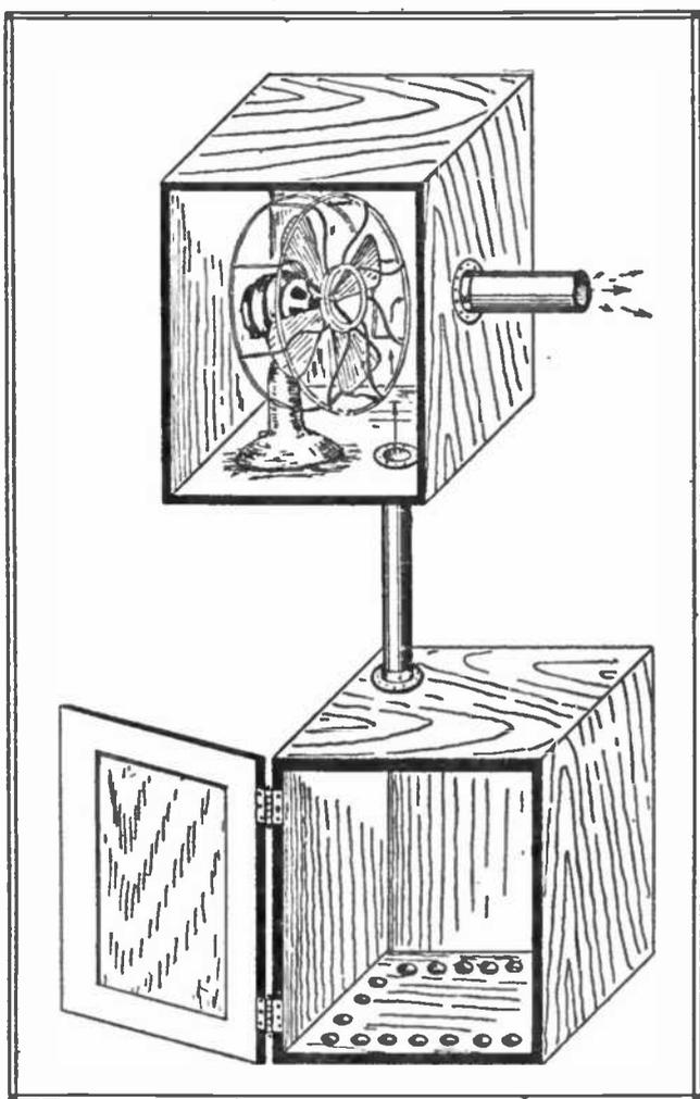
A Fume Hood fitted with Piping and Fan Blower for Carrying away Gases.
