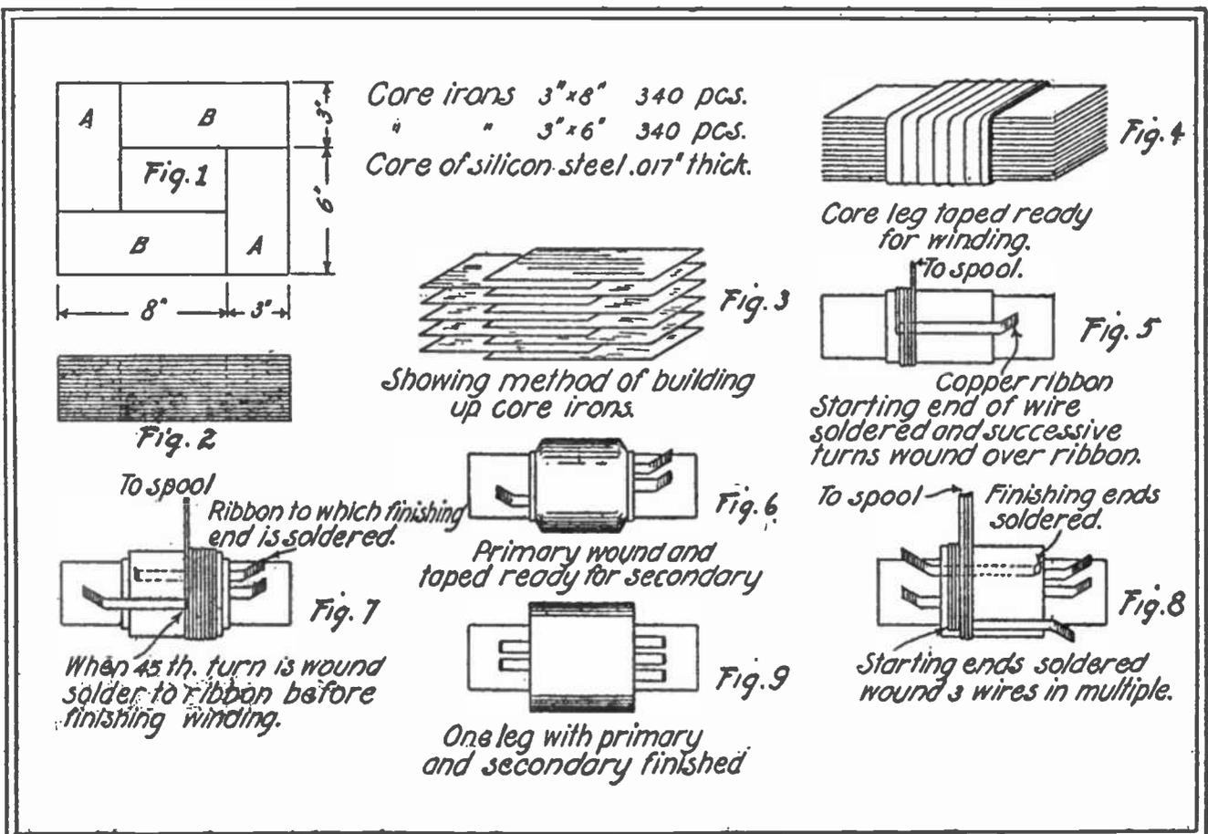
Constructional Details of the Welding Transformer.
