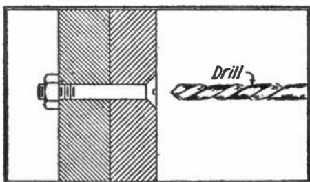
head until the shank is reached, after which the bolt can be driven
