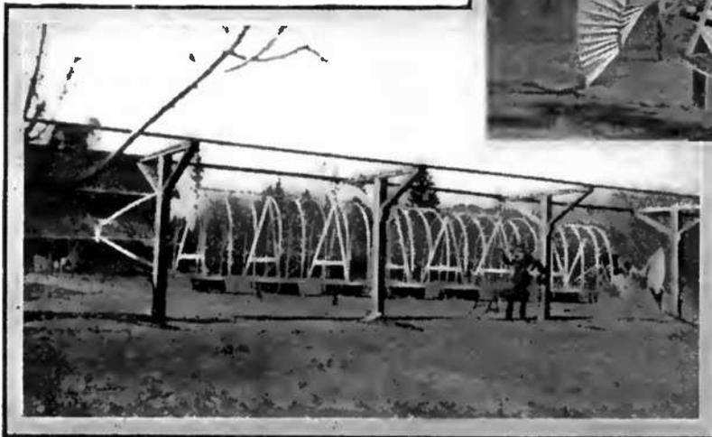
Two views of the aerial trolley car designed and constructed by a Californian inventor. The suspended vehicle is driven by a gasoline engine connected to an aerial propeller.
