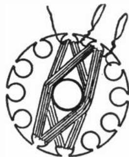
Fig. 14.—Winding of the Armature.
