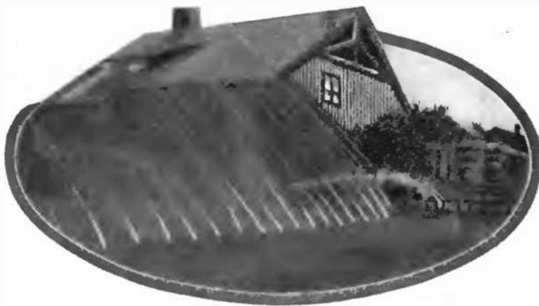
A Pipe With a Row of Holes being Employed to Good Advantage as a Lawn Sprinkler.
