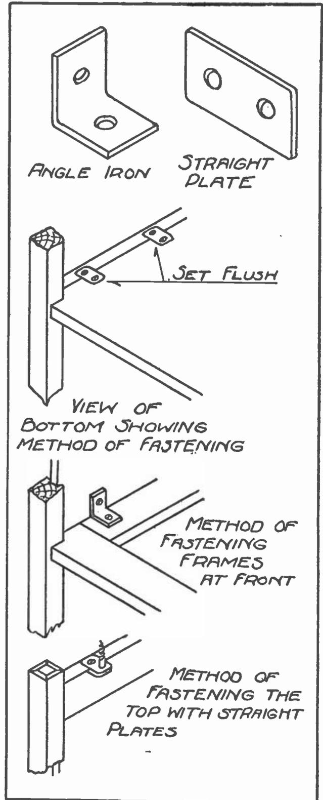
Fig. 3.—Methods of Fastening the Different Members.
