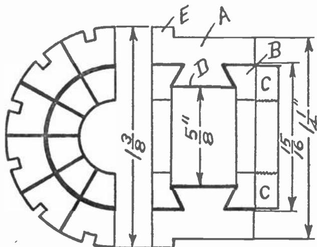
Fig. 10.—A Cross Section of the Commutator and One of its Segments.
