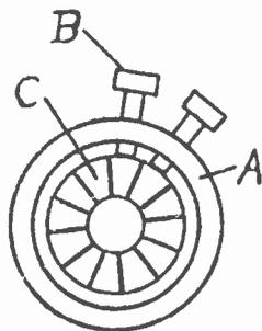
Fig. 12.—Ring for Holding Commutator.
