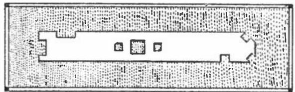
angle to facilitate reaching the tool. The space between is sharpened to a screw-driver wedge. The three openings in the center of the tool are for different sizes of taps and reamers, while the remaining slots are to fit the dogs used on the lathe.
