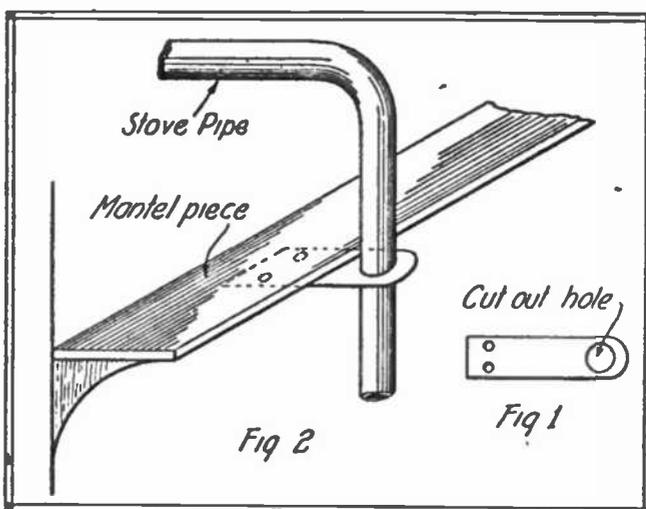
its place a holder that is neater and stronger. The holder is merely a piece of stove pipe iron cut to the shape indicated in Fig. 1 and having the holes as
