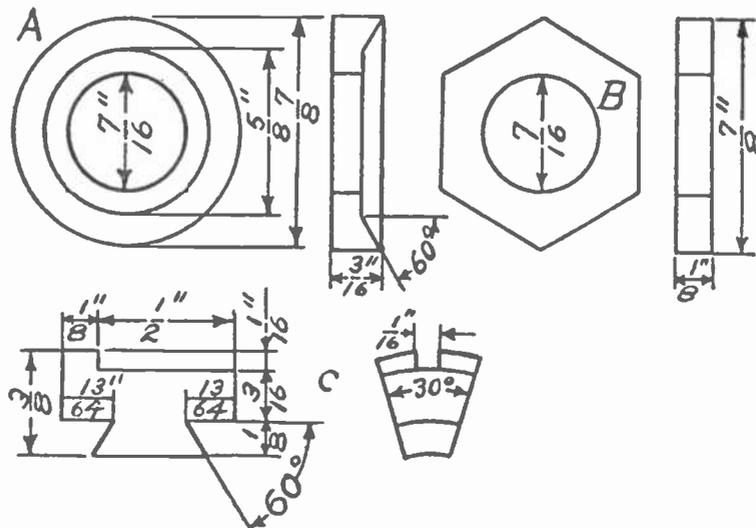
Fig. 11.—Parts of the Commutator.
