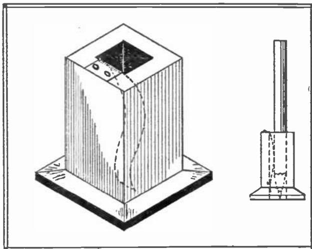
piece of spring steel inserted as shown in the illustration. If the workman is more ambitious, he can make the holder out of a piece of square wooden stock, as shown in the larger drawing. The holder is to be nailed to the wall above the bench.
