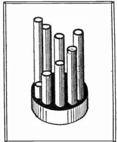
Place a rubber band around the disc and then drill a row of 3/8 inch holes around the edge as shown in the illustration. In each hole insert a piece of brass tubing, starting with a piece one inch long and making each succeeding piece 1/2 inch longer until five pieces are in place. Then start with another one inch piece in the opposite half of the disc and continue as before. When finished, the device is pushed down inside the horn, the rubber band on the edge of the disc holding it in place.
