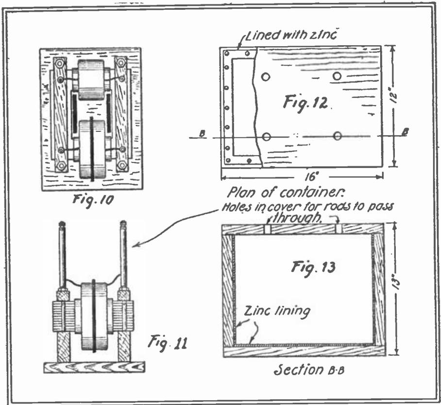
The Transformer with its Container, Complete.
