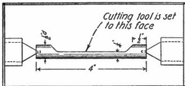
either end and milled down to exactly half its diameter as shown in the drawing. The rod is placed between lathe centers and the tool set to the height of the milled portion.
