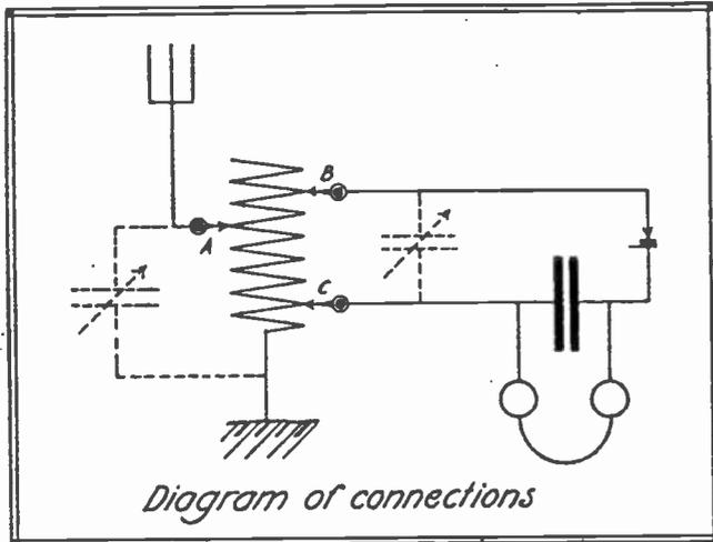
Wiring Diagram for the Tapped Three-Slide Tuner.
