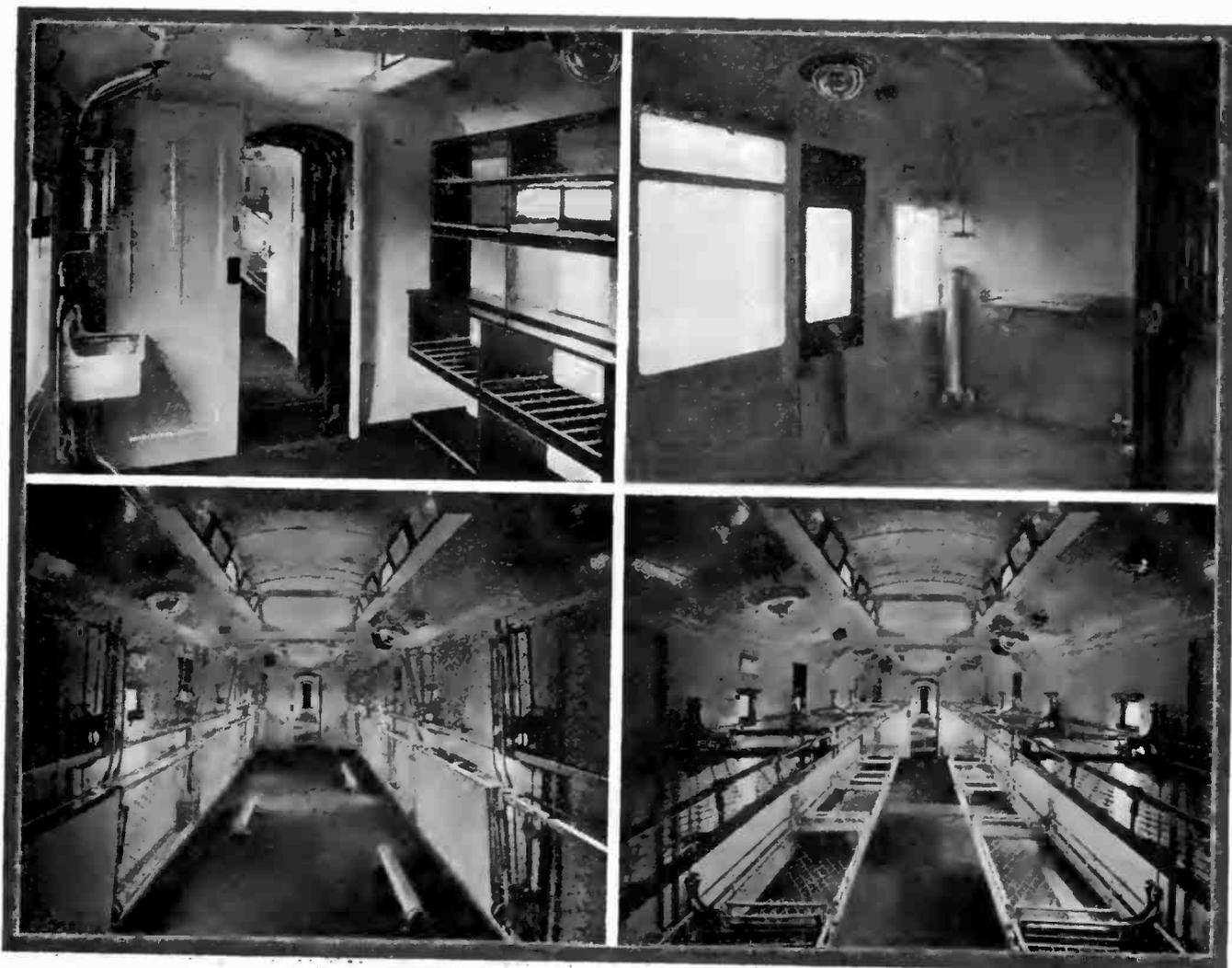
The above views in the order shown are: -Pharmacy compartment, the treatment room, and a sleeping compartment with the cots folded and the same view with the cots in position for use.
