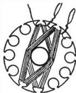
Fig. 14.—Winding of the Armature.
