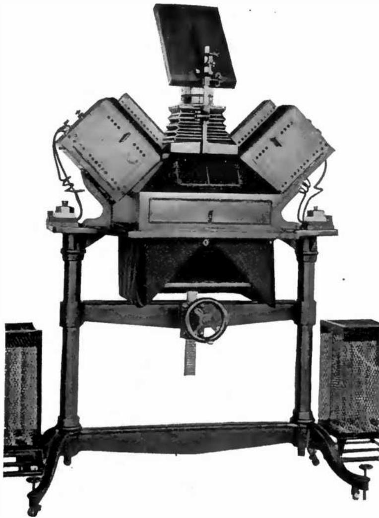
Large objects may be shown with this Arc Light Projector, which was originally intended to project on the screen a view of the entire mechanism of a cash register.
