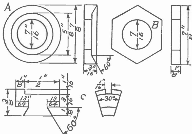
Fig. 11.—Parts of the Commutator.
