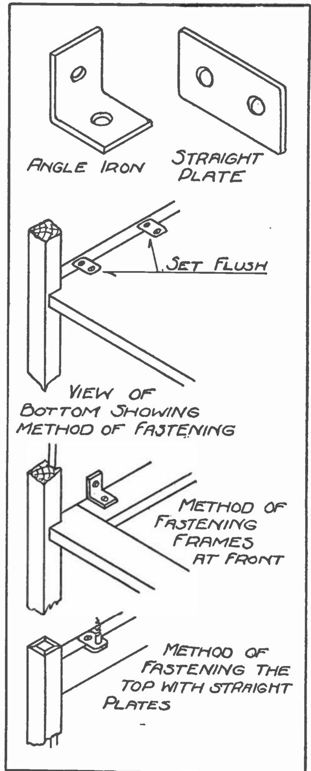
Fig. 3.—Methods of Fastening the Different Members.
