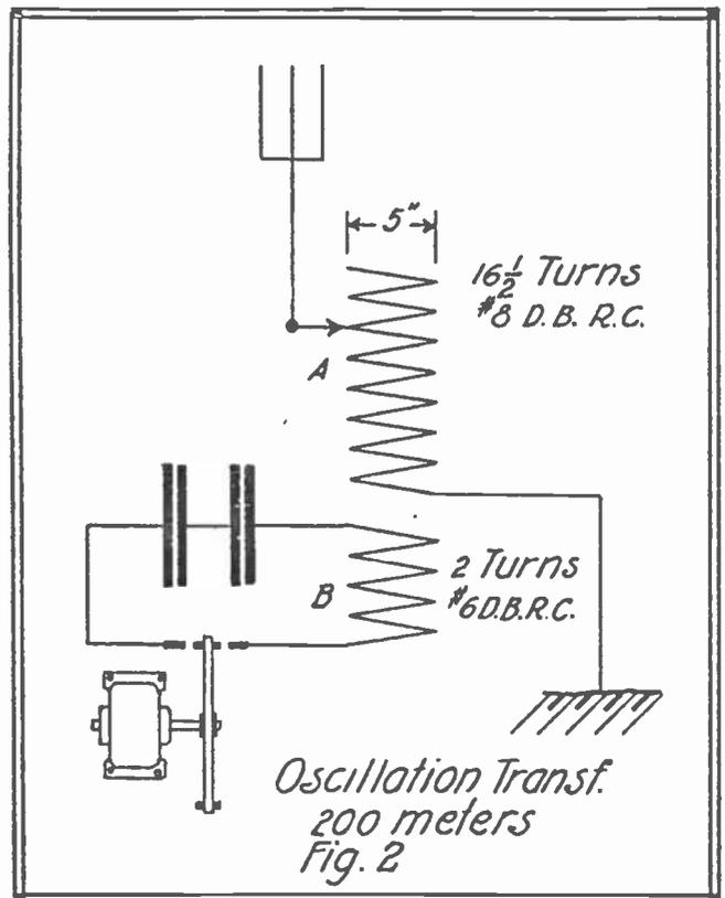
Connections for an Oscillation Transformer, Condenser and Rotary Gap.
