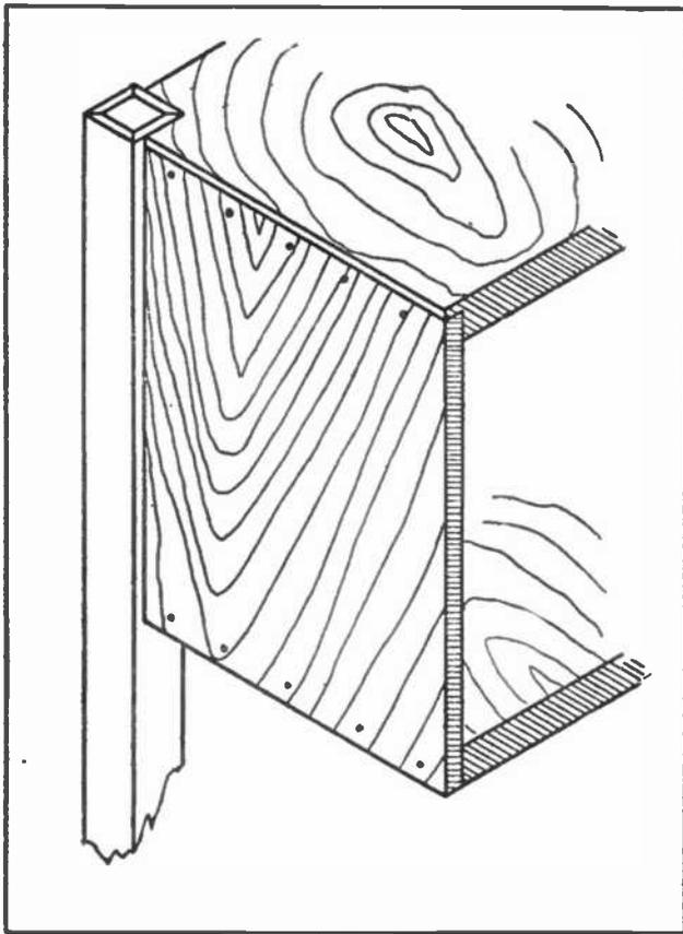
Fig. 2.—Section Through Back, Showing How it is Fastened to Top and Bottom of Cabinet.
