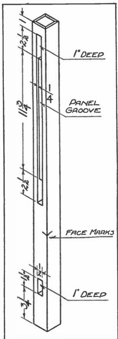
Fig. 1.—Detail of Inside Corner of Leg.
