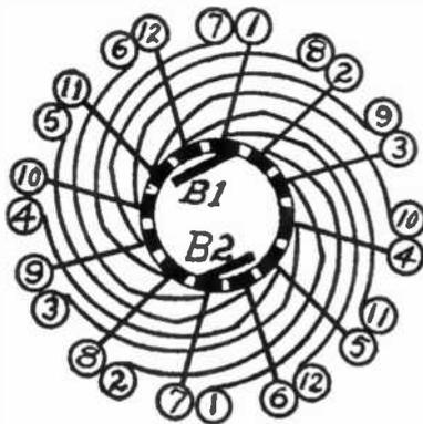
Fig. 15.—Scheme for Connecting Armature Windings to Commutator.
