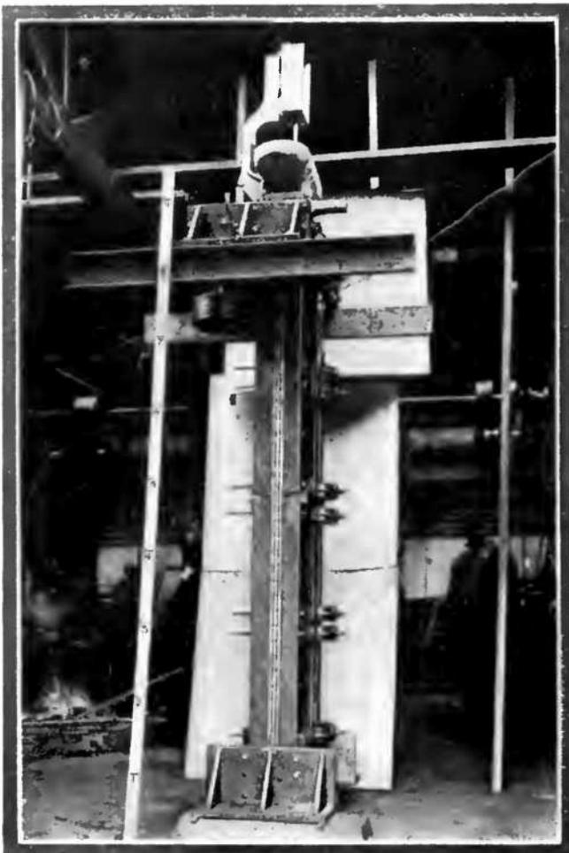
By Means of this Machine, Continuous Brass Tubing can be Made with No Other Attention than to Furnish the Metal.
