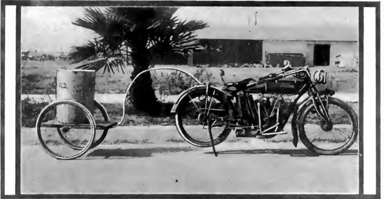
By means of a light, two-wheeled cart, the motorcycle may be employed to good advantage for the delivery of merchandise.
