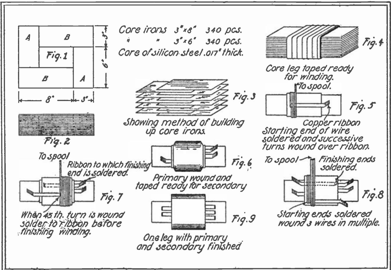
Constructional Details of the Welding Transformer.
