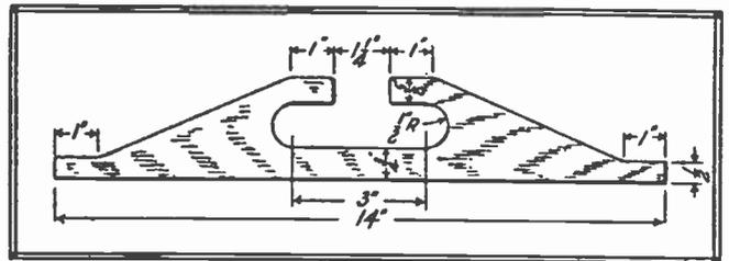
where it can be found when wanted. The illustration shows the construction clearly and no further explanation is necessary.
