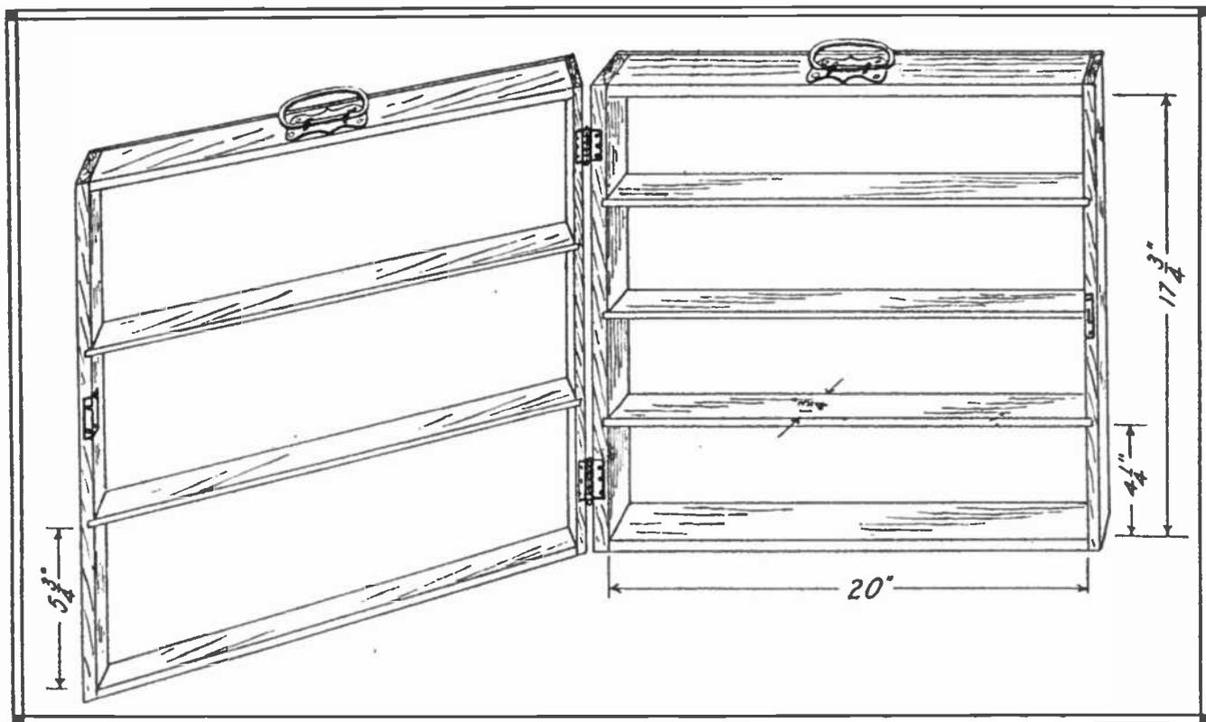
Dimensioned Sketch of a Case for Holding the Bottles of Chemicals. Shelves Built in this Manner Facilitate the Transportation of the Outfit.
