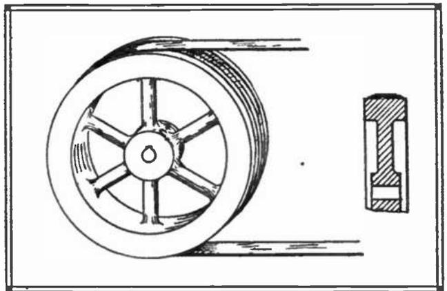
oughly shellacked and when the varnish had dried, the wheel was given a test which quickly proved the scheme to be practicable. At the end of the season the tape was found to be but slightly worn. During the entire run the belt did not once leave the fly wheel.
