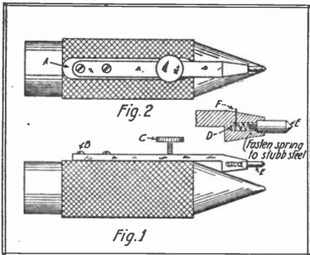
ing been made or bought, is placed in the milling machine and a cut taken at *A*, Fig. 2. This forms a seat for the spacing arm *B*, which is filed up from a piece of Stubb steel. In the end of *B* is a hole to take the coiled spring which forms a cushion for the pointed plunger *E*. The spring is retained in the hole by means of the pin, *F*. The spacing arm, *B*, is to be hardened and then drawn to a spring temper after all the operations have been completed.
