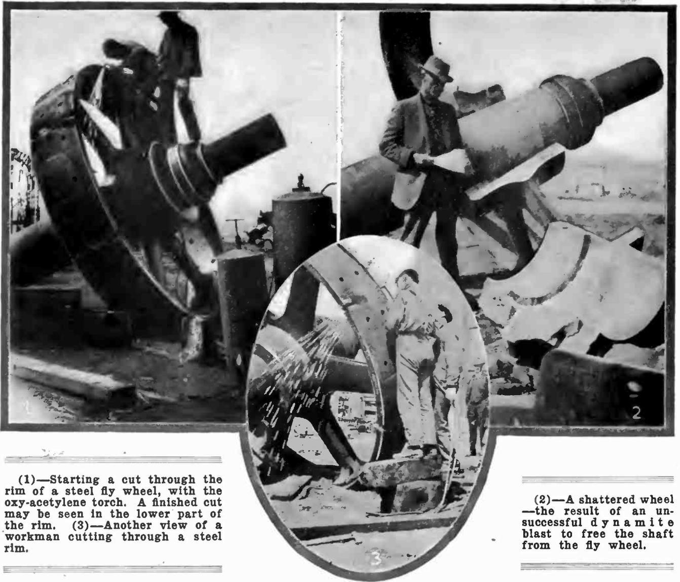
(1)—Starting a cut through the rim of a steel fly wheel, with the oxy-acetylene torch. A finished cut may be seen in the lower part of the rim. (3)—Another view of a workman cutting through a steel rim.
