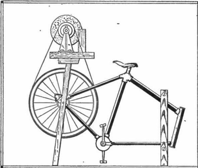
To build the grinder a chainless bicycle without a coaster brake is preferable, although a chain bicycle could be used with a guard over the chain and sprockets. The front forks and handle bars and the rear tire are removed and the seat post turned backward. Wooden legs are carefully fitted and bolted to the frame. The tall (now front) legs are fitted with horizontal supports and the table screwed or nailed on.
