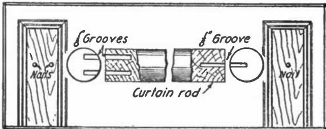
grooves cut into the end grain, as shown. The rod is prepared by cutting it to a length that will make it a snug fit between the door jambs. The slots are then cut, two being placed in one end and one in the other end of the rod. Headless nails are driven in the door jamb on either side to take the slots and the support is finished.
