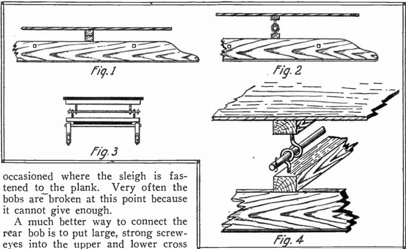
occasioned where the sleigh is fastened to the plank. Very often the bobs are broken at this point because it cannot give enough.
