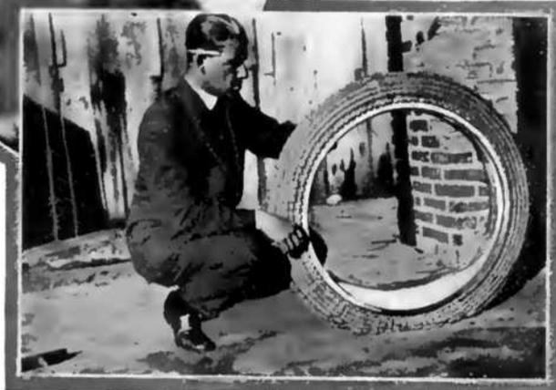
A View of the new steel tire, as well as a single section of interlocking pieces. The usual inner tube is employed, the steel pieces forming an outer covering.
