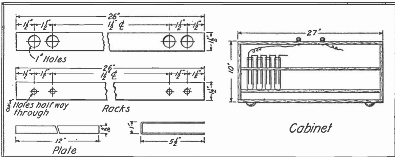
A containing cabinet is now constructed from  $\frac{1}{2}$  inch oak measuring overall 27 inches in length, 10 inches in height and  $9\frac{1}{2}$  inches in width. Brass screws should be used throughout the work to avoid the corrosive effect of the battery solution. The interior of the cabinet should be coated with lampblack or a similar acid resistant.
