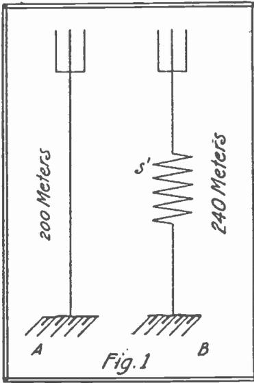
Wave Length of an Aerial With and Without Oscillation Transformer.
