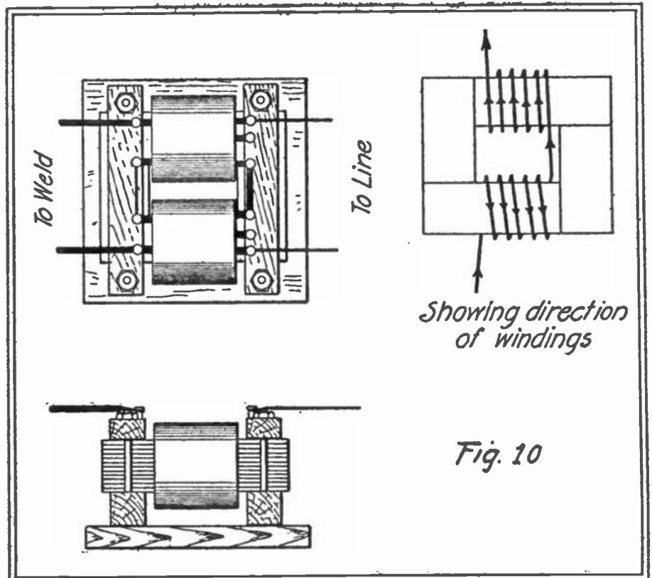
View of the Welding Transformer as it Appears when Completed.
