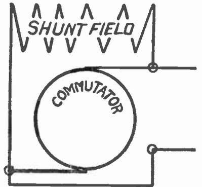
Fig. 16.—Connections for the Generator.
