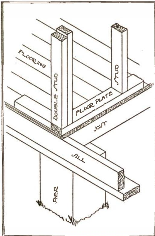
Fig. 12—Showing the Construction of the Framing at Floor.
