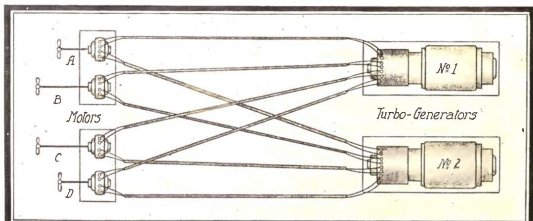
Two turbo-generators, operating either independently or in tandem, supply the current which operates the electric motors that drive the propellers.
