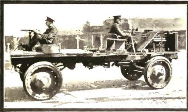
To Allow Greater Flexibility of Action, Recent Canadian Armored Automobiles are being Fitted with a Double Set of Controls.
