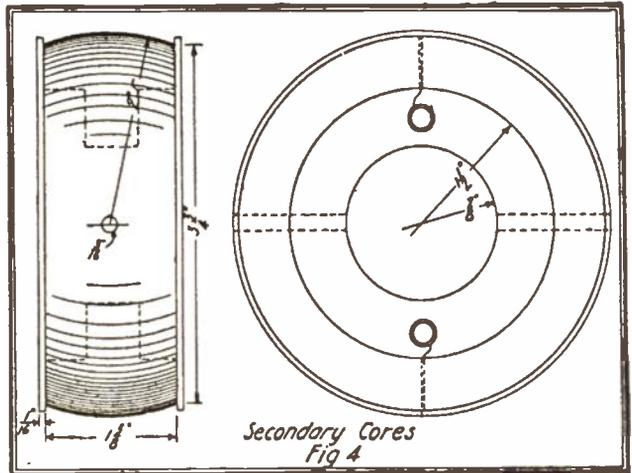
Wooden Spools Which Are Used for Holding the Secondary Windings of the Coupler.
