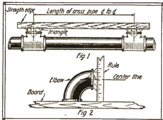
found by using two of these triangles and measuring the distance between their center points.
