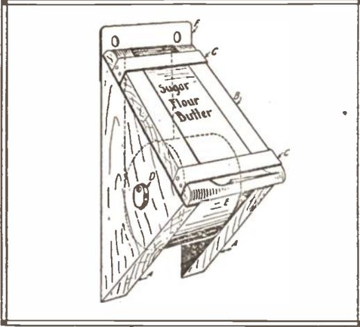
wooden or metal rod to hold a roll of paper, such as is used in adding machines, or any other roll of paper that may be obtainable—the roll determining the size of the parts for the holder.
