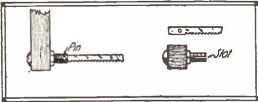
to admit stove bolts. The threaded portions of the bolts should be slotted with a hack saw and drilled with small holes at right angles to the slot. A pin should be inserted through these holes and through the holes in the ends of the saw blade.
