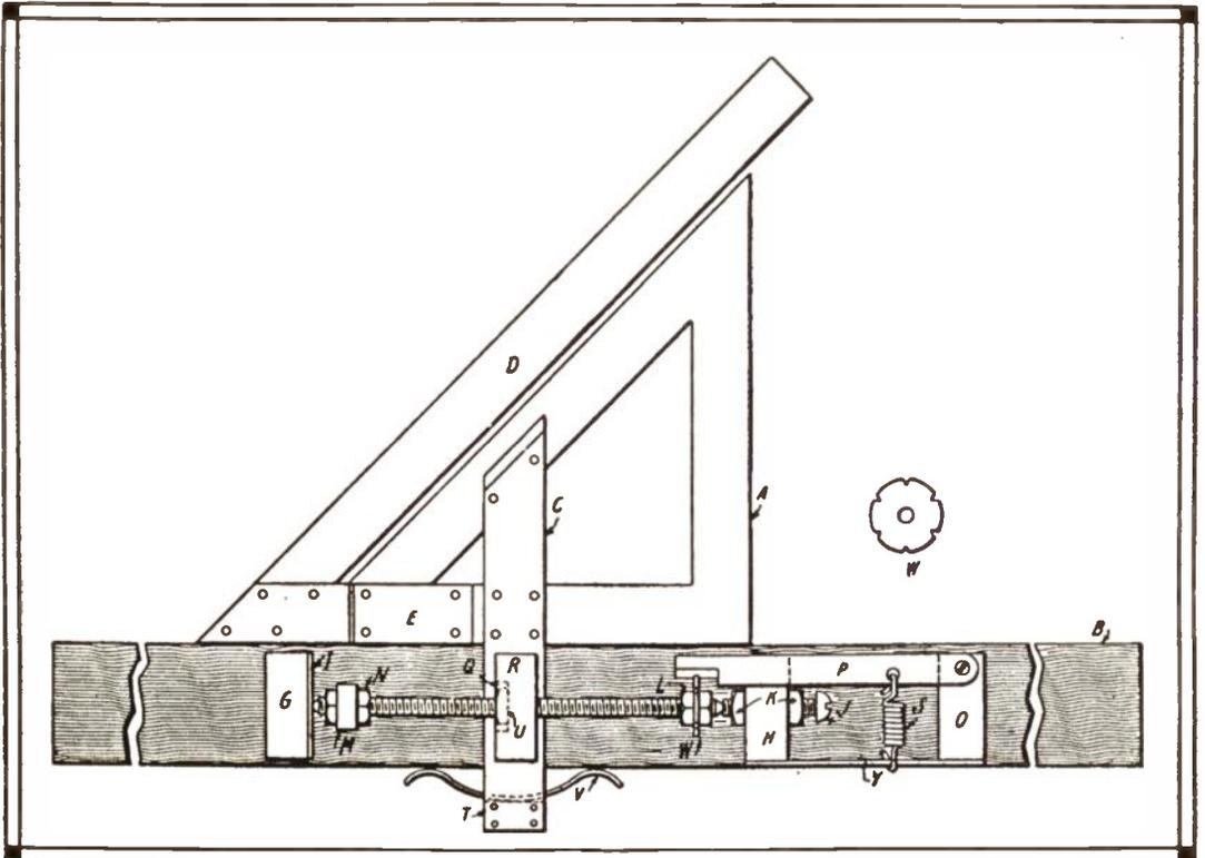
screw, *J*, which passes through the block *H*, and is held in position by the nuts, *K*. The ratchet, *W*, is held in place by the hexagonal nuts, *L*.
