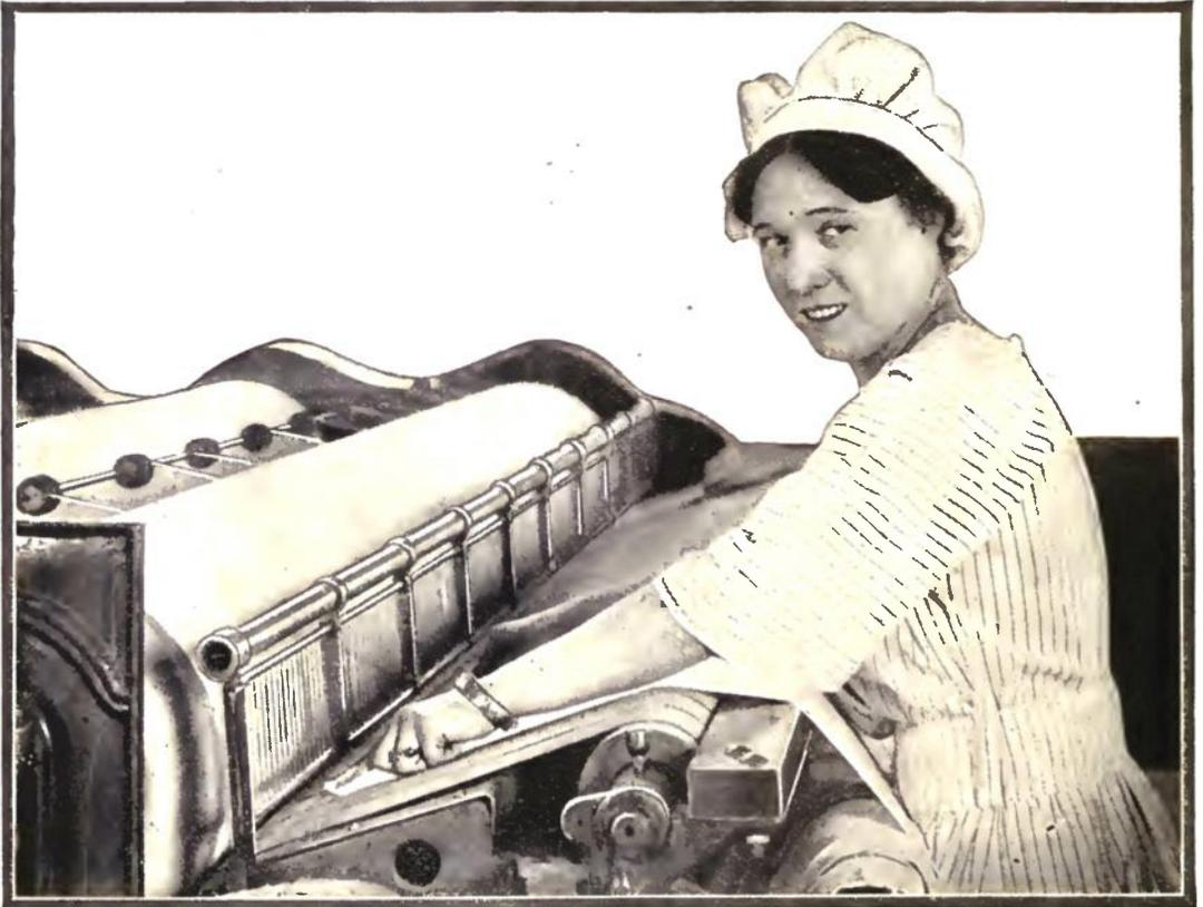
A Little Steel Fence Along the Entire Length of the Roller Prevents the Worker's Fingers from Being Caught in the Mangle or Ironing Machine.
