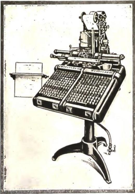
A Monotype Keyboard which Perforates a Paper Ribbon that is Afterwards Placed on the Casting Machine.
