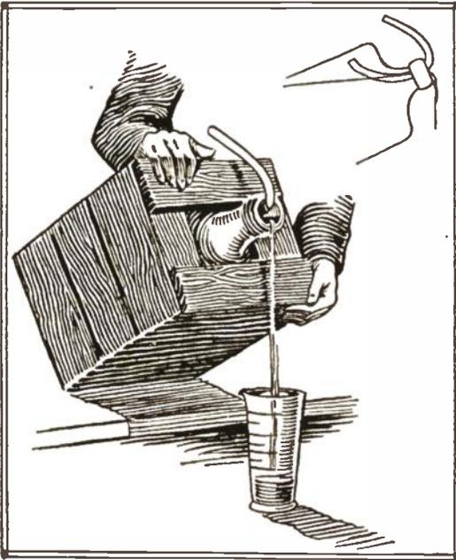
phuric acid from a carboy can be avoided if a bent glass tube is inserted into the neck of the bottle so that the partial vacuum caused by the liquid gushing out is equalized.
