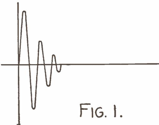
Highly Damped Oscillations Produced by a Parallel Plate Quenched Gap.
