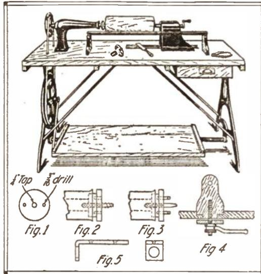
sort at the head. The cross sectional view, Fig. 4, shows the tail stock, the groove in the bed and the method of locking.
