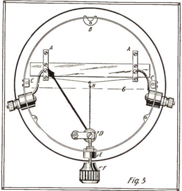
Front View of the Working Parts of the Hot Wire Meter as It Appears When Finished.
