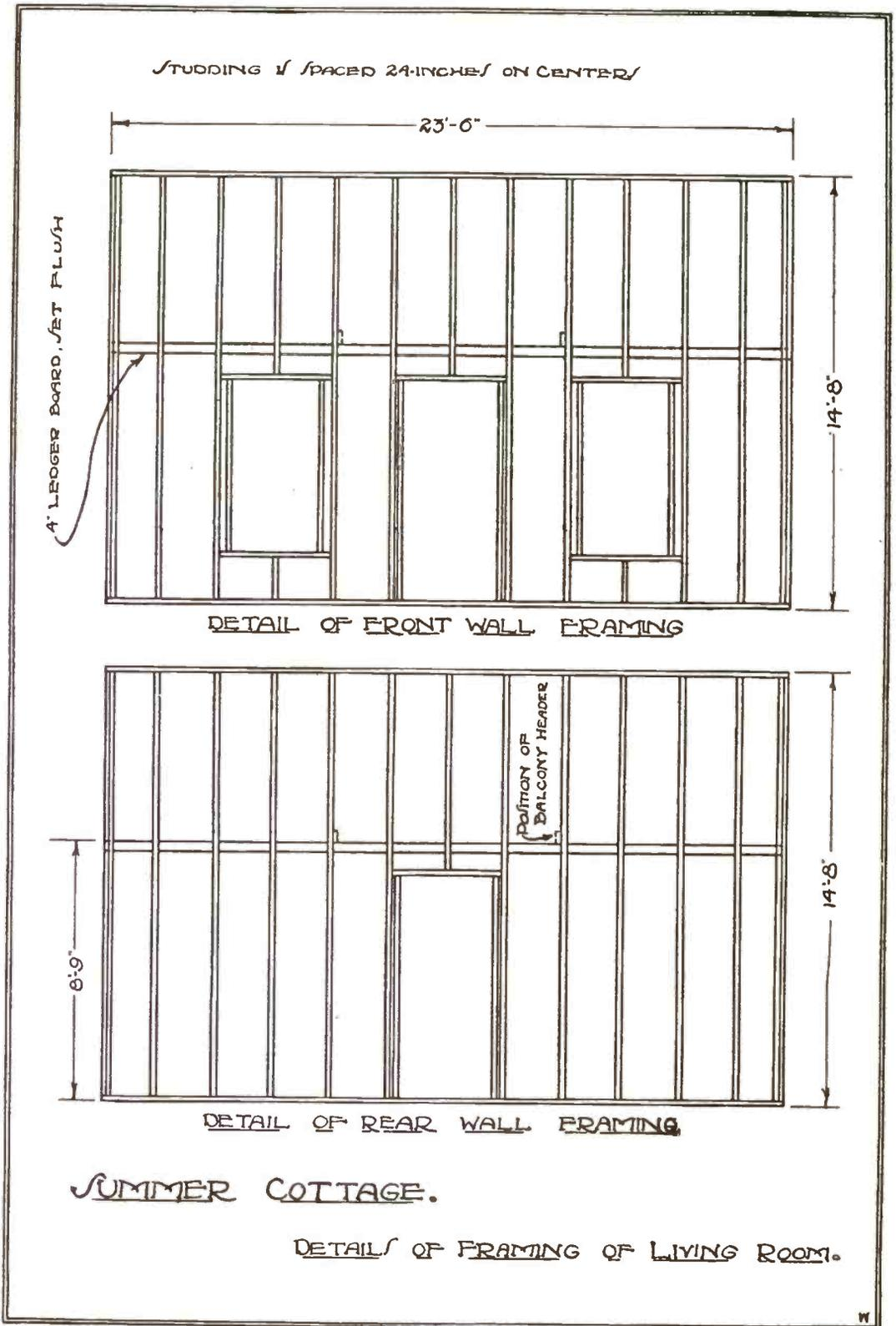
Fig. 13—Details of the Front and Rear Wall Frames of the Living Room.
