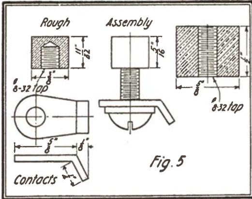
Details of Switch Points and Connecting Lugs.
