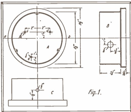
The Details of the Case for the Hot Wire Meter.
