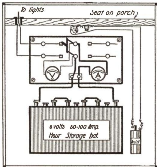
Arrangement of Storage Battery and Switchboard Under Porch Seat.
