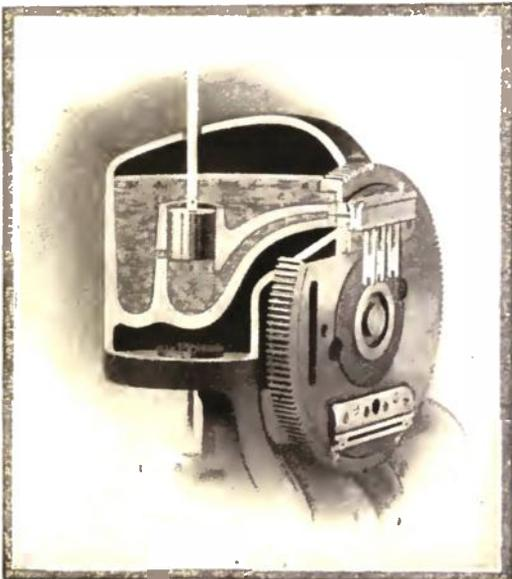
The Casting Mechanism of the Linotype, Showing the Melting Pot, Plunger, Mouth of Mould and the Assembled Line of Matrices.
