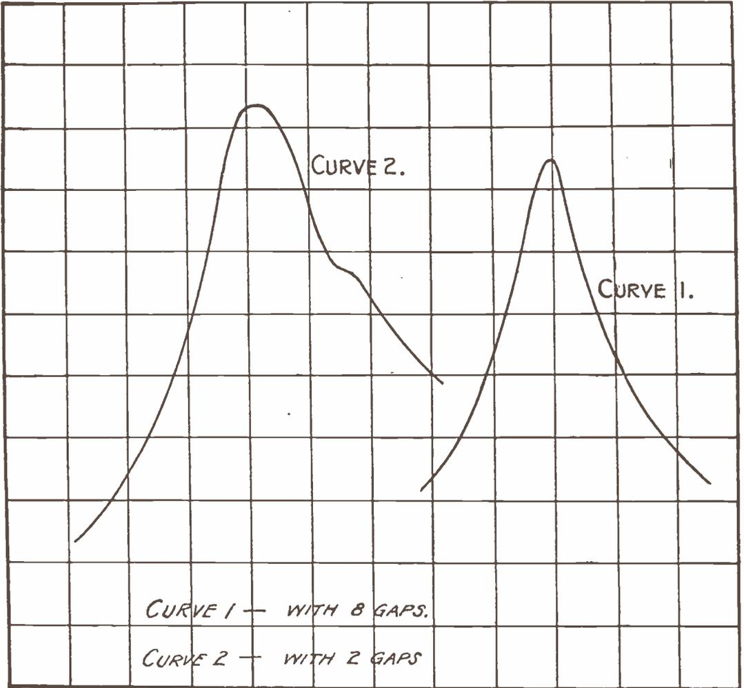
Fig. 6.—Diagrammatic Representation of the Characteristics of the New Spark Gap.
