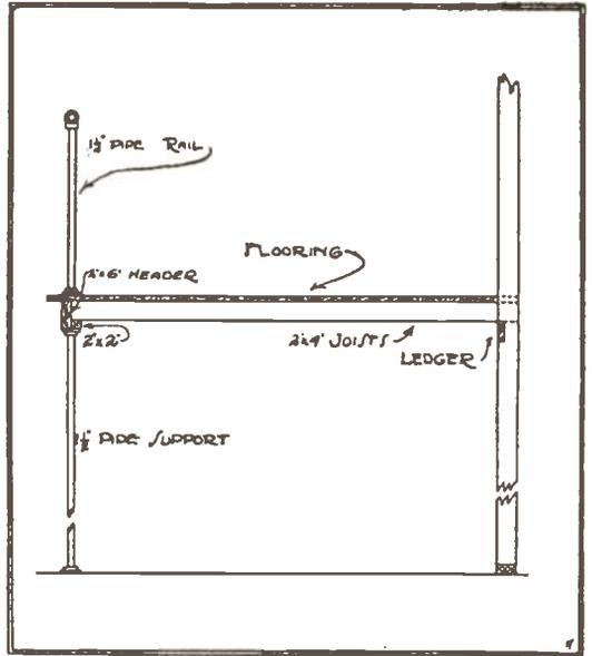
Fig. 19—Detail of Balcony Construction.
