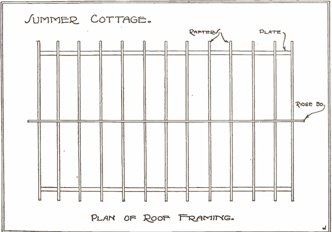
Fig. 17—Plan of the Rafters as they Should Appear After Being Nailed in Place.
