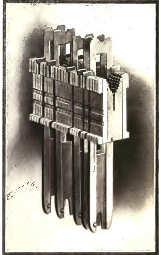
A Line of Matrices and Space Bands as they Appear When Assembled, Ready for Casting.
