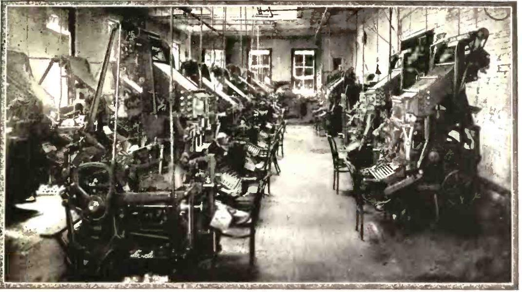
A Typical Newspaper Composing Room, in which a Number of Linotype Machines are being Used to Set up the Reading Matter. Many Linotypes are required by Every Daily Newspaper, Because of the Vast Amount of Type Matter that Must be set up within a Limited Time.
