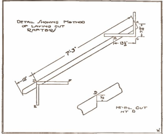
Fig. 16—Showing the Method of Laying Out the Rafters.
