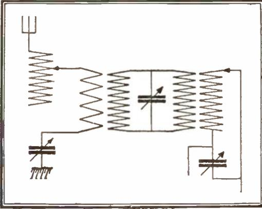
Wiring Diagram of a Simple Marconi Multiple Tuner, Showing Relation of Different Windings and Condensers.
