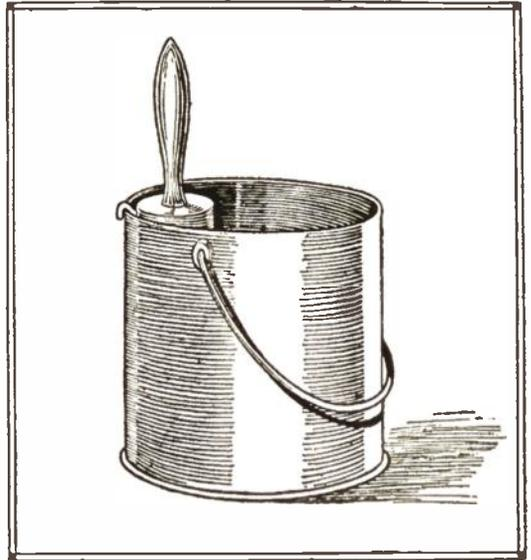
handle of a brush, as shown in the sketch. Thus, when the brush is not required for the moment, it may be placed in the can without danger of its becoming entirely covered with paint.
