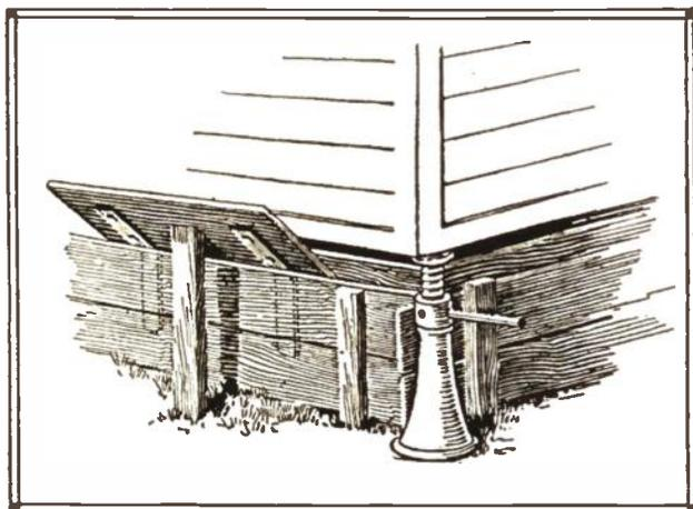
wards at an angle of about 45 degrees. A piece of wood or other material fastened to the middle of the board on the outside has its free end on the ground, thus holding the board in the proper position.
