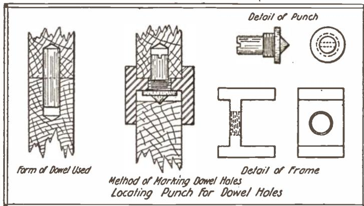
The device is invaluable for marking off dowel holes in the edges of boards used for table tops and in other places where it is essential that accurate
