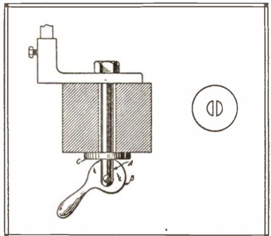
have a slot at one end to admit the cam, *B*. The washer, *C*, should be cut at the center to fit loosely over the slotted bolt.
