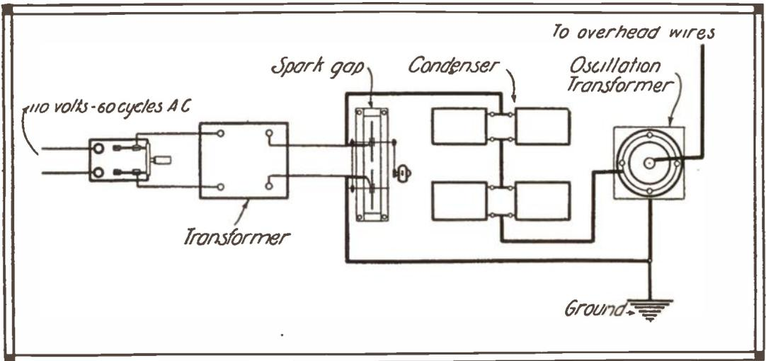
Wiring Diagram for the Connecting of the Various Pieces of Apparatus to be Used in Electrical Plant Culture.
