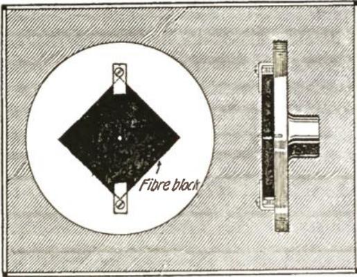
**To Cut Large Holes in Fibre**
