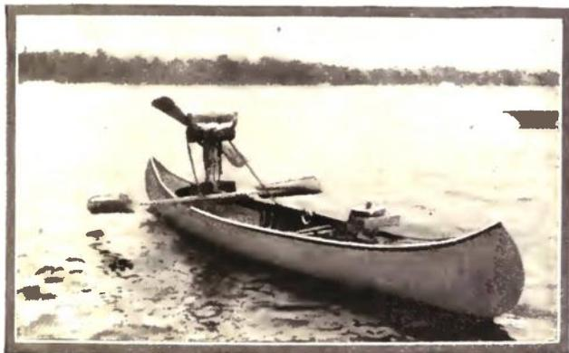
Propelled by Both a Marine and Aerial Propeller, This Canoe is Claimed to be Safer Than the Ordinary Craft of That Class—and Far Speedier.
