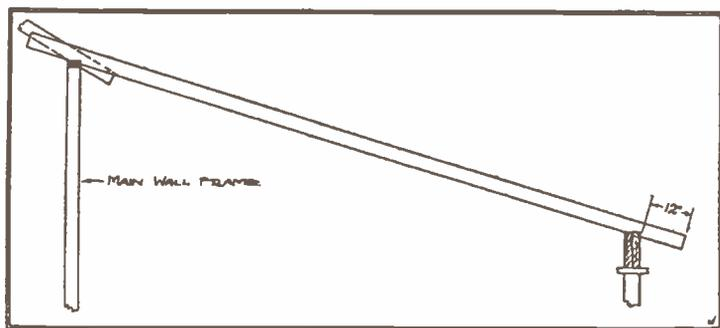
Fig. 23.—Detail of Porch Rafter Framing.
