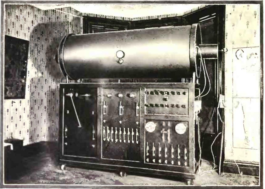
The Stanley X-Ray Apparatus: High Tension Transformer and Switchboard Producing and Controlling the Current for the X-Ray Tube.
