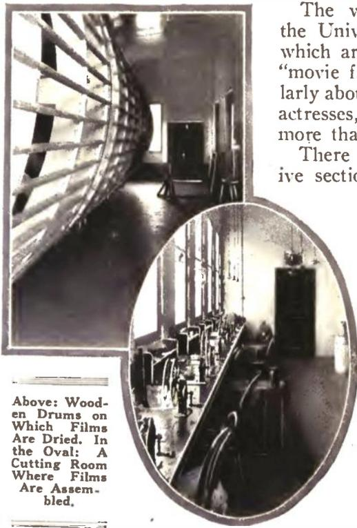
Above: Wooden Drums on Which Films Are Dried. In the Oval: A Cutting Room Where Films Are Assembled.
