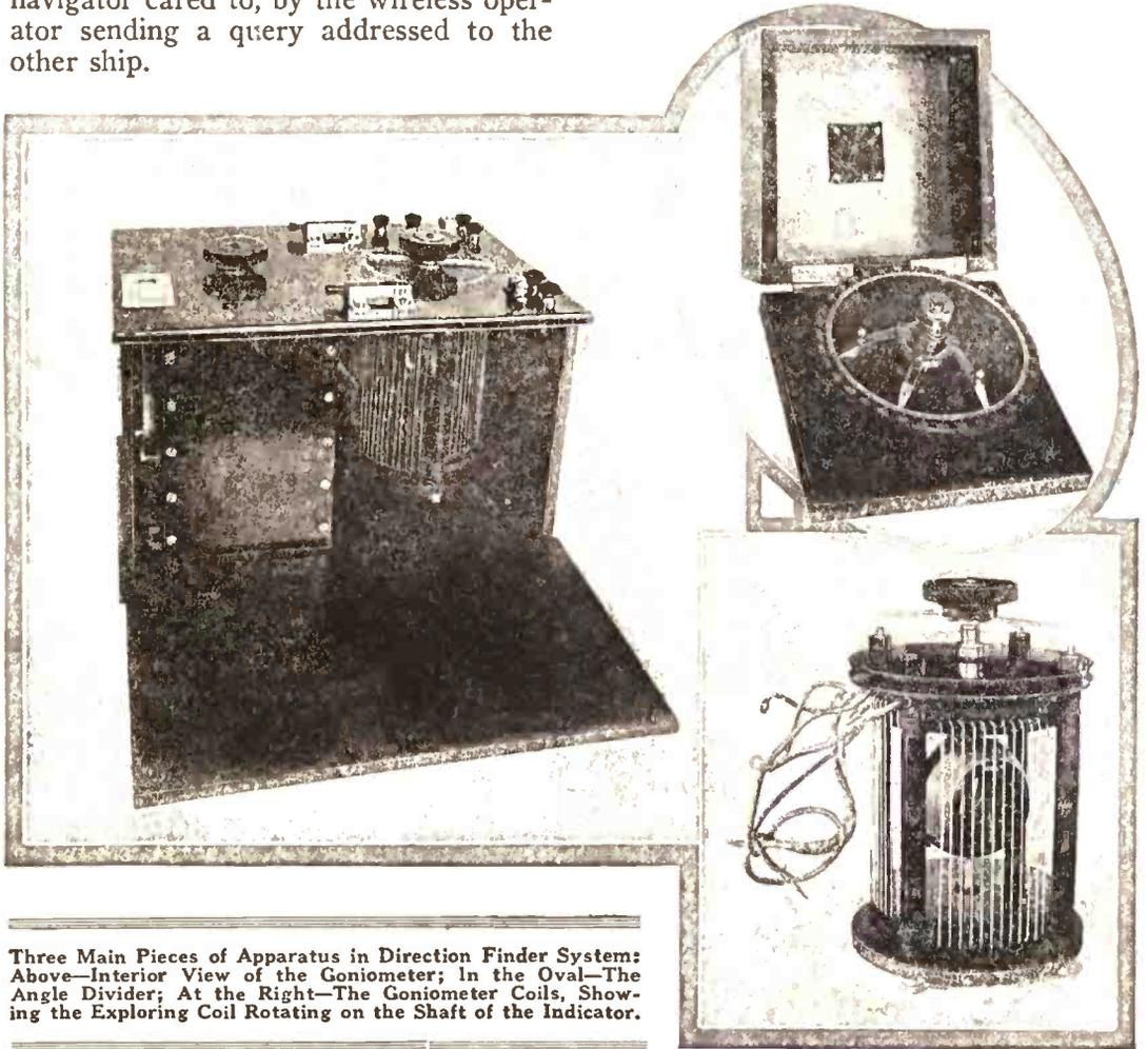
Three Main Pieces of Apparatus in Direction Finder System: Above—Interior View of the Goniometer; In the Oval—The Angle Divider; At the Right—The Goniometer Coils, Showing the Exploring Coil Rotating on the Shaft of the Indicator.
