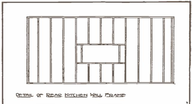
Fig. 25.—Arrangement of Framing for Rear Kitchen Wall.
