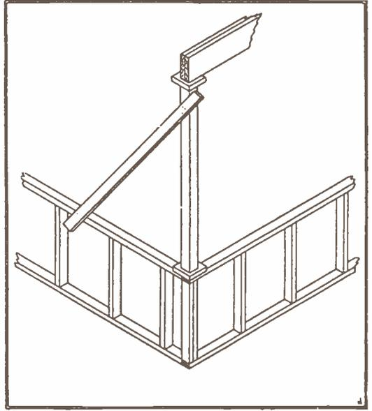
Fig. 22.—Porch Framing Detail.
