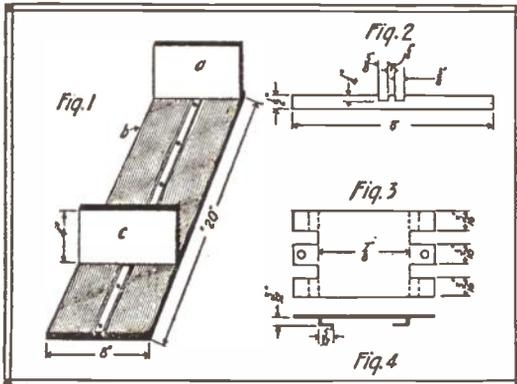
Two parallel grooves should be cut along the centre and a brass strip mounted along the track between them. One end rest, *a*, should be secured to the base with wood screws, while the other, *c*, slides along the track by means of the brass slider shown in Fig. 4. The end elevation of the base is shown in Fig. 2. Fig. 3 shows the slider before it is bent to the proper shape.
