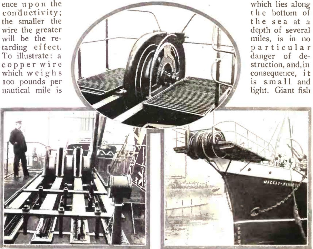
The Sheaves of the Cable Steamer "Mackay-Bennett." At the Left: The Bow Cable Sheaves as Viewed from Inboard. At the Right: Another View of the Bow Sheaves that are Used for Paying Out and Picking Up Submarine Cables. In the Oval: The Stern Sheaves that are Used for the Same Purpose as Those at the Bow.
