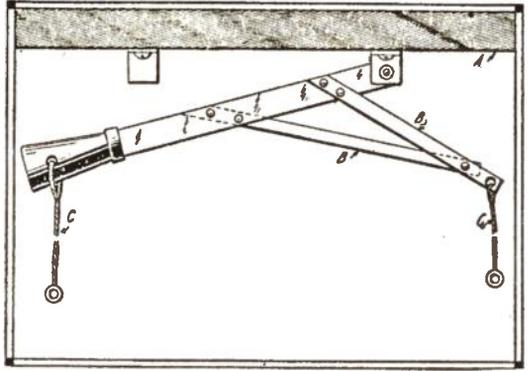
bored in the handle. Pulling on cord G closes the circuit; pulling on cord C opens it. The metal strips are indicated as BB in the drawing.
