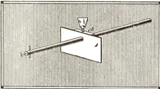
be bored at one end with two holes, one for a marking point and the other for a set screw to hold the marking point, or scribe, in place. Referring to the drawing, B is a block of hard wood bored with a hole which should be threaded to accommodate a wing clamp screw. A is a larger wood board of thinner material along which the object to be marked slides.
