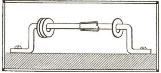
dle, fastened to the back of the delivery wagon and containing a number of washers. When one delivery is made a number of washers to correspond with the number of units of whatever sort are delivered are moved from one side of the handle to the other. To prevent them sliding back and becoming mixed when the wagon is under way, a small wire clip, inserted through a hole drilled in the handle and bent at the ends as shown should be added.
