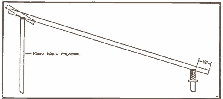
Fig. 23.—Detail of Porch Rafter Framing.
