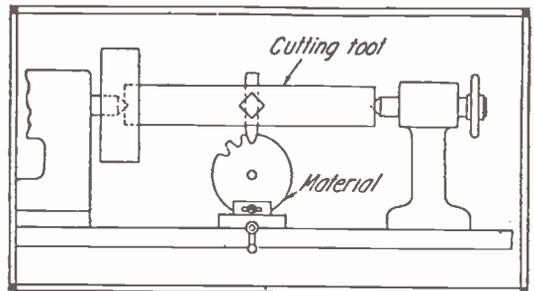
sists of a  $1\frac{1}{2}$ " steel rod about 15" in length. This rod should be centered at both ends in the lathe. At the centre of the rod, two small holes should be drilled. One of these should be filed out square to accommodate the cutting tool and the other threaded for a lock bolt. The material for the cog is a disc of metal of the desired diameter. It should be clamped in a slide rest and turned as the succeeding teeth are cut.
