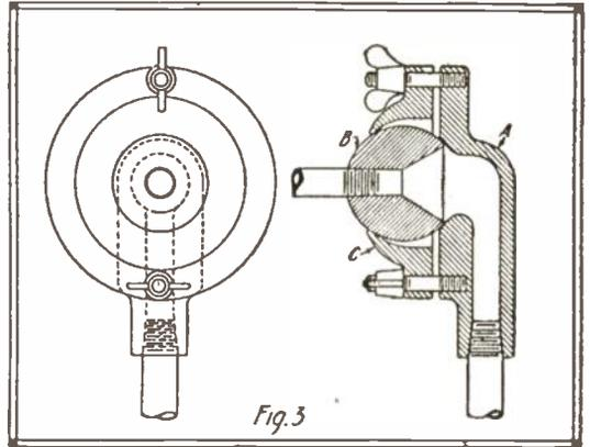
base to the adjusting clamp and socket. This pipe should, of course, be hollow to admit the passage of lamp cord. Referring to Fig. 3, the tube from the base is screwed into a small culvert running through a round casting and terminating in a flaring opening. The socket, rounded as shown, fits into this opening. A smaller tube connects the socket to the lamp socket.
