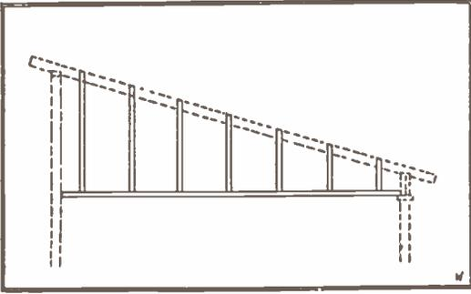
Fig. 24.—Detail of Framing of Upper Porch Section.
