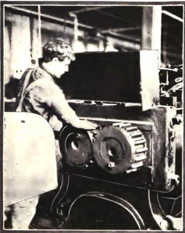
Gears are Recognized as a Constant Source of Danger to the Operatives. A Simple Metal Cover Does Much to Reduce—if Not Entirely Eliminate—the Danger.
