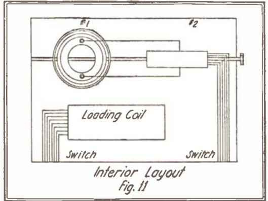
Arrangement of Loose Couplers and Loading Coil.
