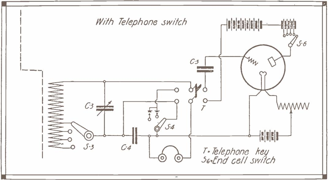
Wiring Diagram of Complete Receiving Set, with Telephone Switch.
