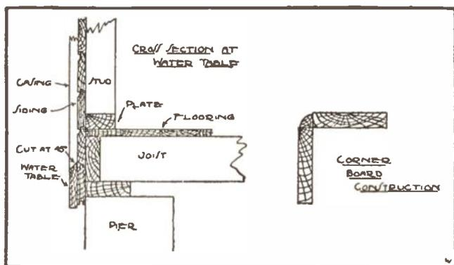
Fig. 27.—Details of Exterior Finish.
