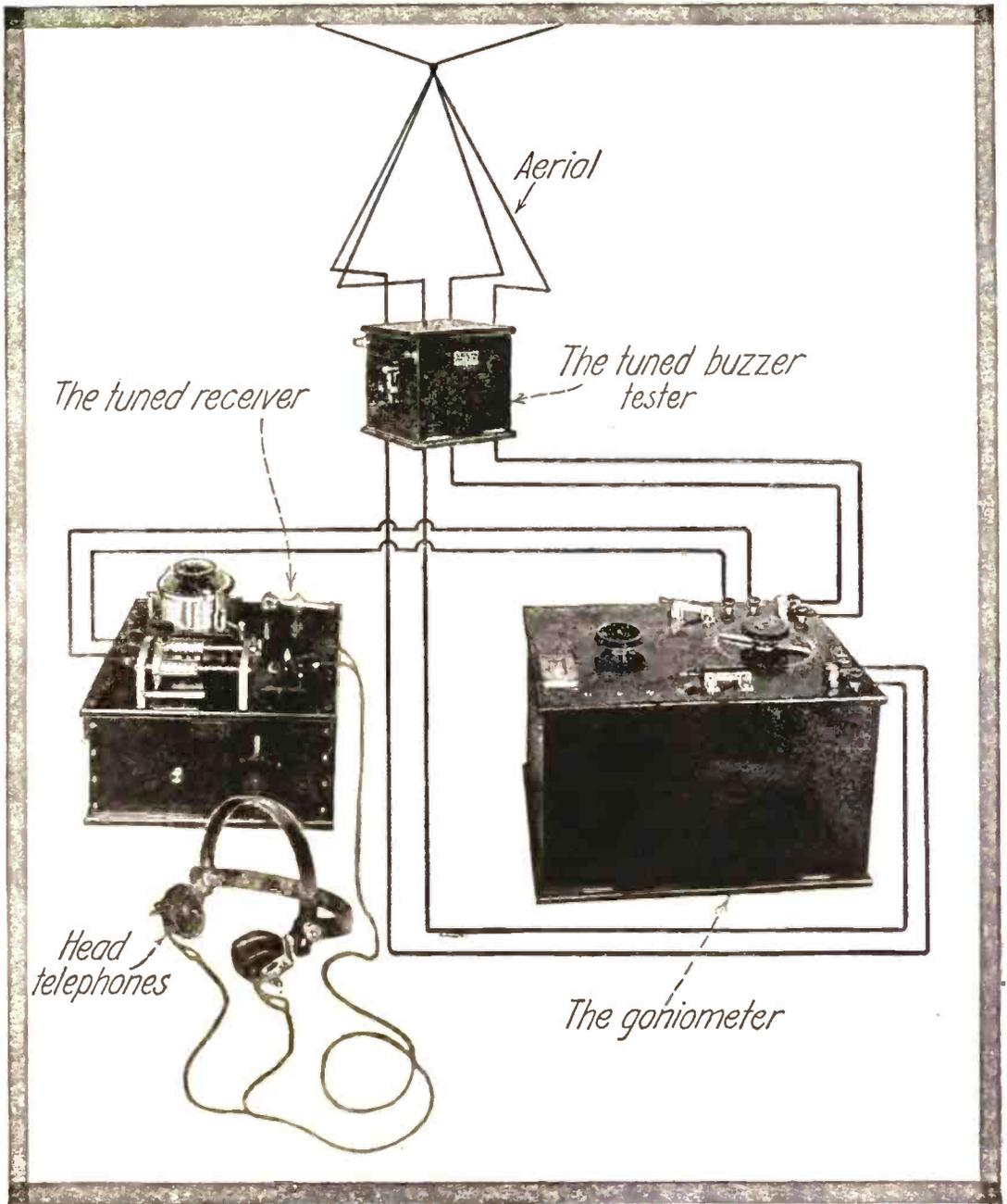
Arrangement of the Different Pieces of Apparatus, as Well as the Wiring Scheme for a Direction Finder Receiving Set.
