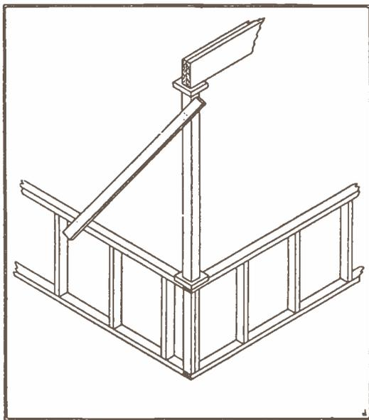
Fig. 22.—Porch Framing Detail.
