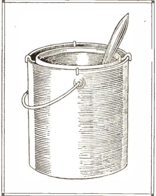
ing illustration. It consists of a strip of metal bent in the form of a circle of such size as to be slightly smaller than the bucket into which it fits. The circle is held in place by small hooks which fit over the top edge of the can.
