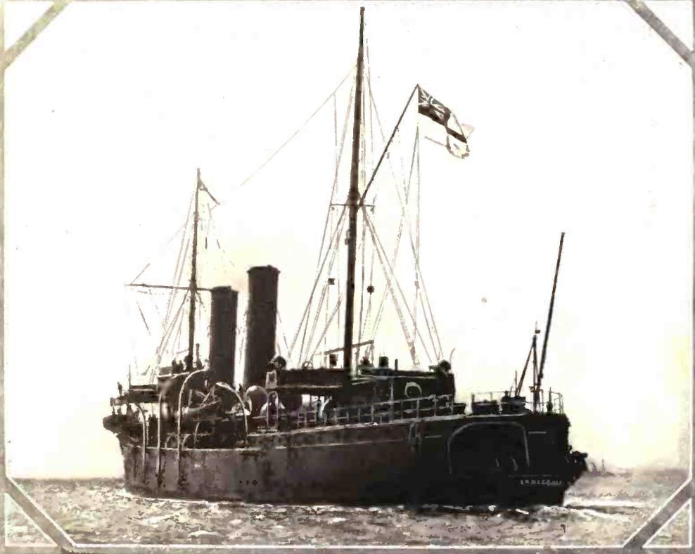
**T**HE "Iphigenia," one of Great Britain's many mine layers. The mines are cast into the water from the stern of the vessel by means of two adjustable gangways.
