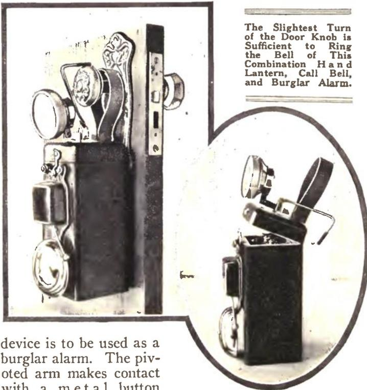
device is to be used as a burglar alarm. The pivoted arm makes contact with a metal button when the outfit is suspended from the strap, and this contact serves to light the lamp and ring the bell. The reader will note that when the device
