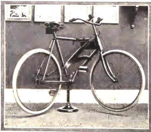
One of the Folding Bicycles used in the Swedish Army, which can be Folded and Carried on the Soldier's Back by Means of a Strap.
