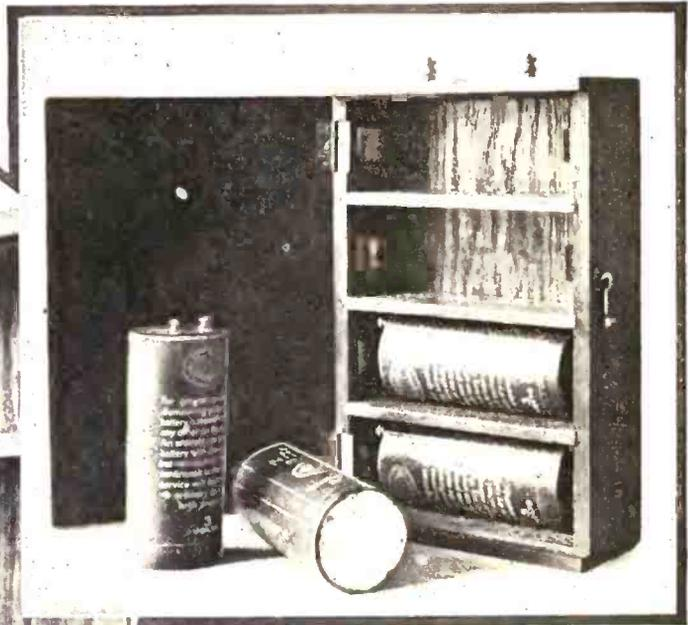
Two Views of a Battery Container of New Design. Contact with the Battery Terminals is Made Through a Pair of Phosphor Bronze Strips. The Contacts Can Be Arranged for Series or Multiple Connection or a Combination of Both.
