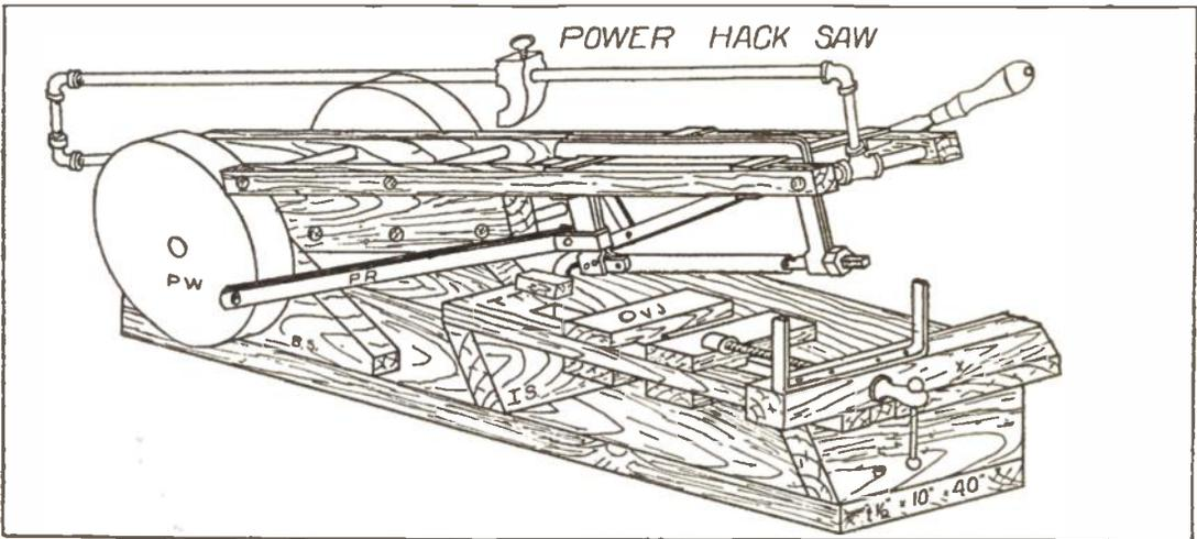
maple or other hard wood. The metal parts are mostly of mild steel, excepting, of course, the cold rolled shaft and the vise screw. Inasmuch as there are no hard joints to make, the wood parts may be very quickly gotten out and fastened together.
