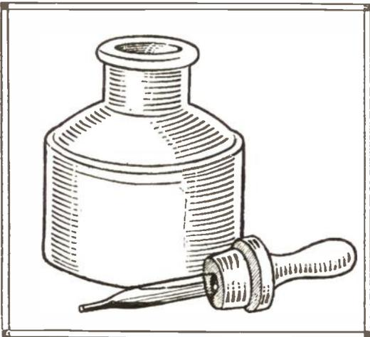
mis-laid at that. A convenient way of keeping a filler is to bore a hole through an ink bottle stopper and push the filler through it. The filler will then be always handy when wanted and perfectly clean.
