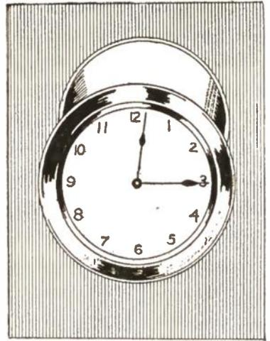
By the Ingenious Combining of an Alarm Clock and Steam Gauge Case, A Ship's Clock is Obtained.
