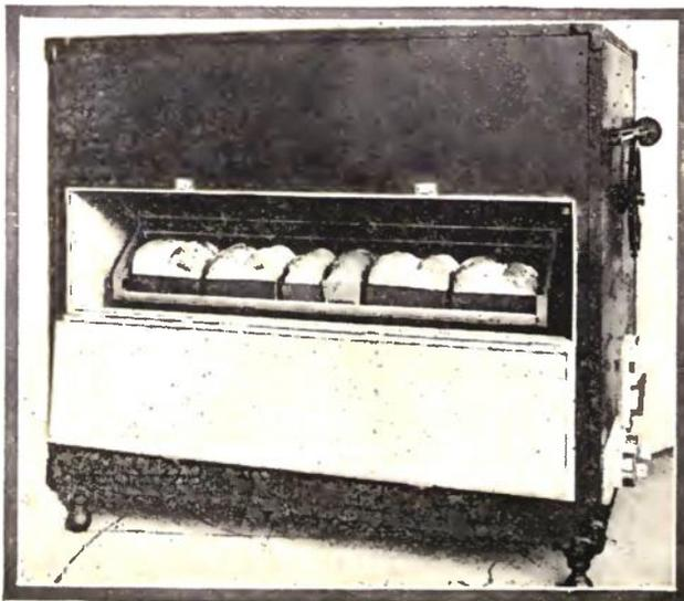
An Electric Oven Designed by a Minneapolis Baker for Baking Bread, Biscuits and Cake.
