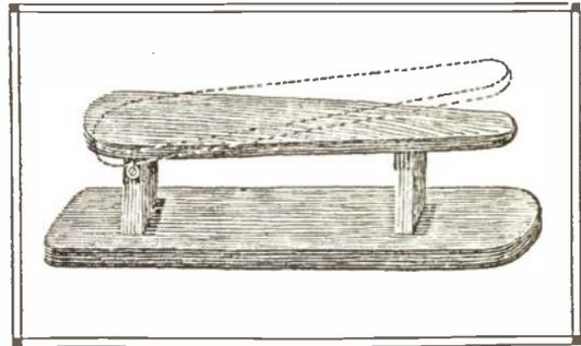
moved, the standards strengthened and the broad end of the board hinged by means of screw-eyes to one of the standards. The top of the upright upon which the board hinges should be planed round.
