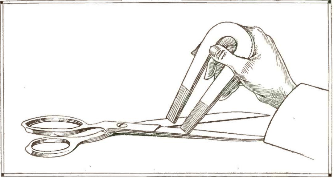
shoe magnet can be employed for magnetizing any pair of scissors. To magnetize the scissors the two poles of the magnet are placed in contact with the scissors near the pivot, and drawn to the end of the blades. This operation is repeated several times, care being exercised that the same poles of the magnet touch the same blades of the scissors.
