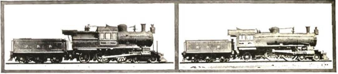
Two of the Earlier Atlantic Type Locomotives Used on the Pennsylvania Railroad. At the Left is the First Locomotive of That Design, Which Was Later Replaced by the One at the Right for the Reason That the Arrangement of Separate Cabs for Engineer and Fireman Was Found Impracticable.
