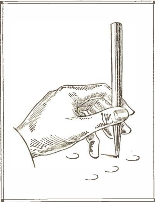
the centering of flange or shear lines which are usually centered with two marks close together for the purpose of distinguishing between the center marks for holes and those of the shear or flange lines. The idea is made clear by the illustration.
