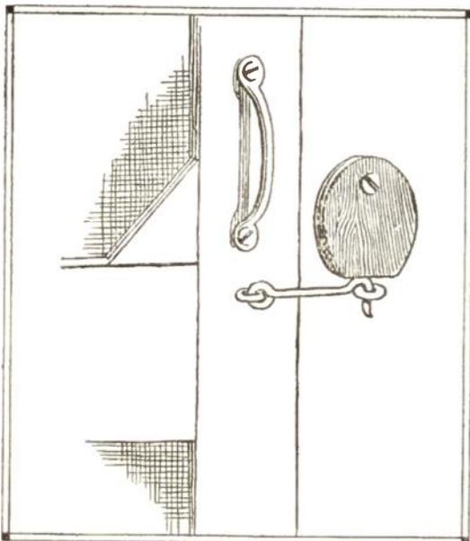
two inches high and one inch wide. The corners are cut off so as to give it the shape shown in the illustration. A hole is then bored in one end so that it may be fastened in place. The other end is cut off in order that it will cover the hole of the eye.
