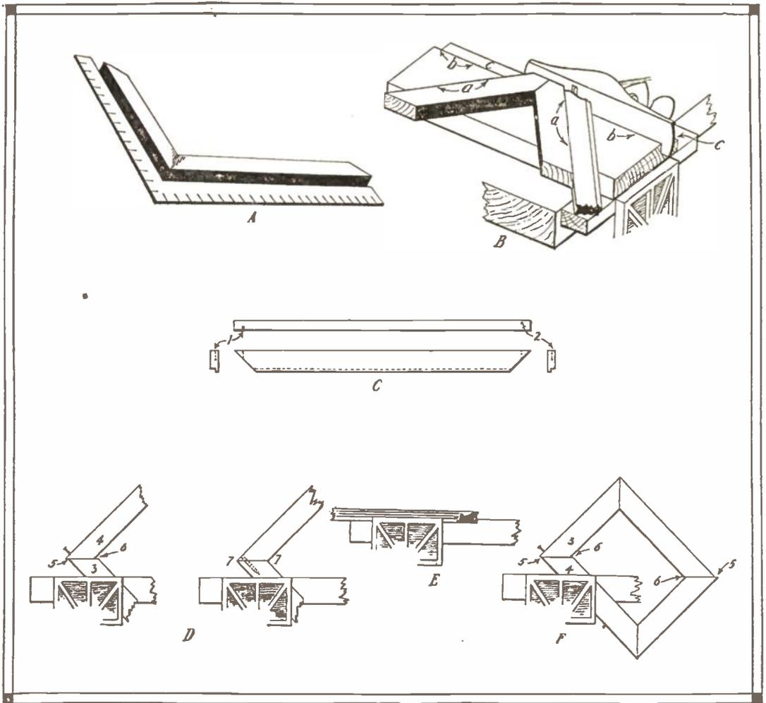
The Tools Required for the Making of Frames, as well as Details of the Work in the Various Stages.
