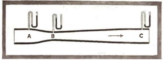
A Simple Diagram to Indicate the Action of the Water Meters Used in the Catskill Aqueduct.
