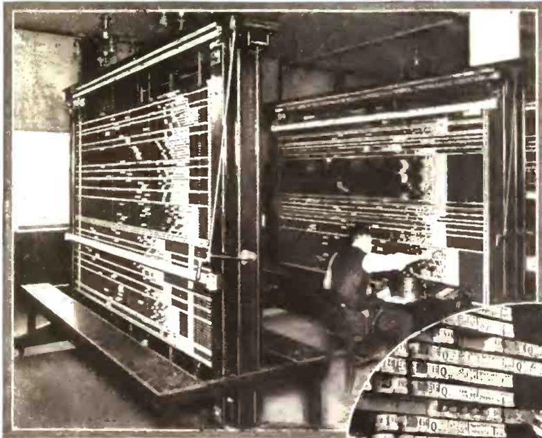
Above: Two of the Control Boards used in an Automobile Factory, Enabling an Accurate Record to be Kept of the Numerous Parts being Manufactured and Those in Stock. At the Right: A Close View of a Control Board, Showing the Method of Inserting the Lettered Blocks.
