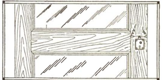
can be made "tamper-proof" by screwing two springs above the bolt, so that when the bolt is withdrawn from them they are separated. If the springs are placed in an electric circuit composed of dry cells and a doorbell, when the lock is tampered with, the bell will sound an alarm.
