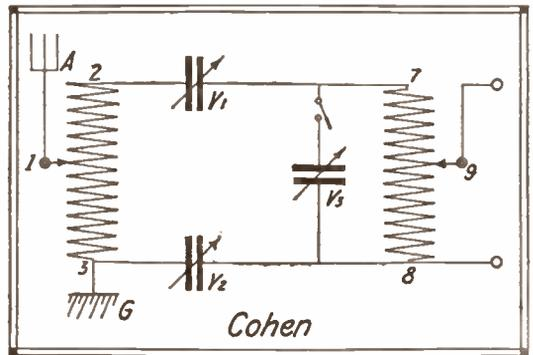
Wiring Plan of the Cohen Circuit for a Multiple Tuner.
