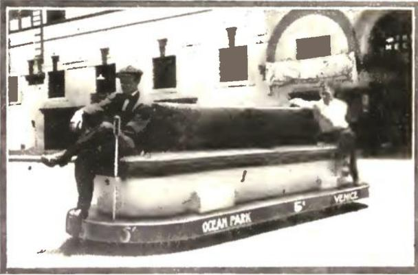
An Electrically Operated Rolling Chair Which is Being Operated at a Californian Seaside Resort.
