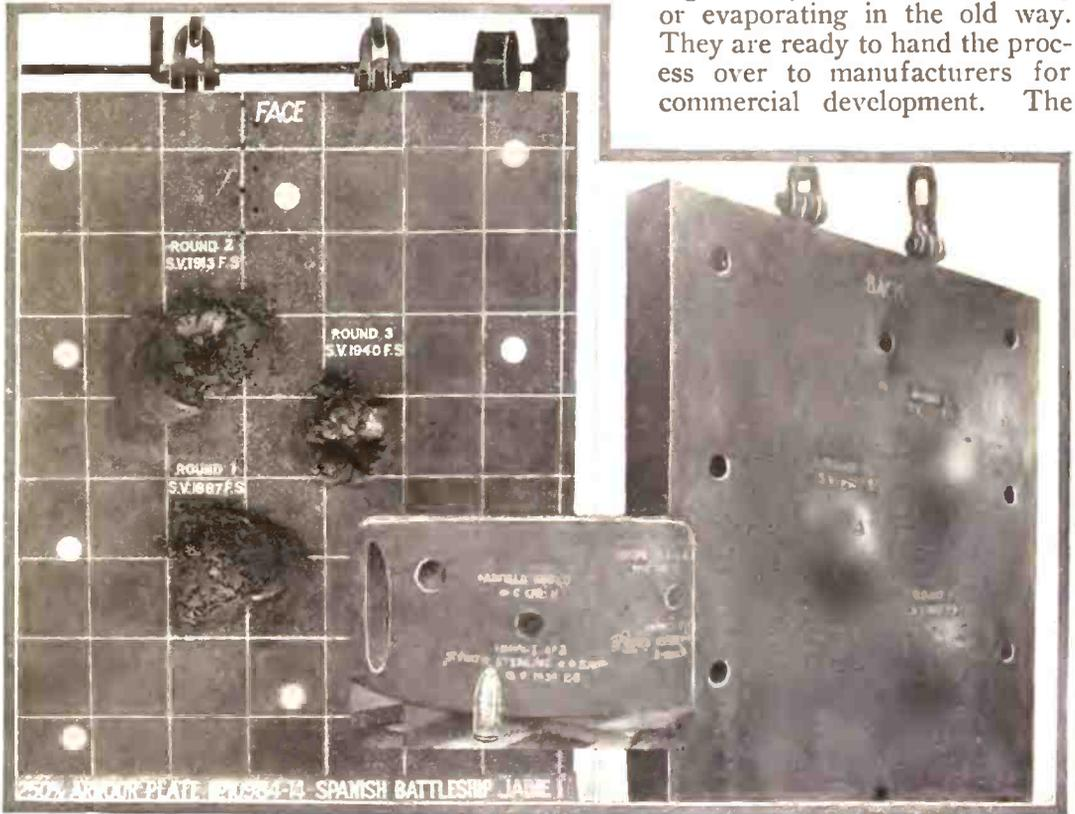
The Effect of Modern Shells on Steel Armor Plates: At the Left is an Armor Plate of the Spanish Battleship "Jaime I," Which Was Damaged by Fourteen-Inch Shells.
