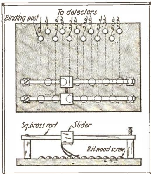
Any One of Several Detectors May be Cut In by Means of This Simple Detector Switch.
