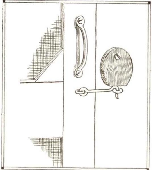
two inches high and one inch wide. The corners are cut off so as to give it the shape shown in the illustration. A hole is then bored in one end so that it may be fastened in place. The other end is cut off in order that it will cover the hole of the eye.
