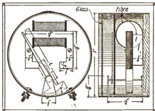
coil in the right hand, so that the fingers encircle it in the direction of the north pole. The dial may be divided in any way, to indicate the direction of the current.
