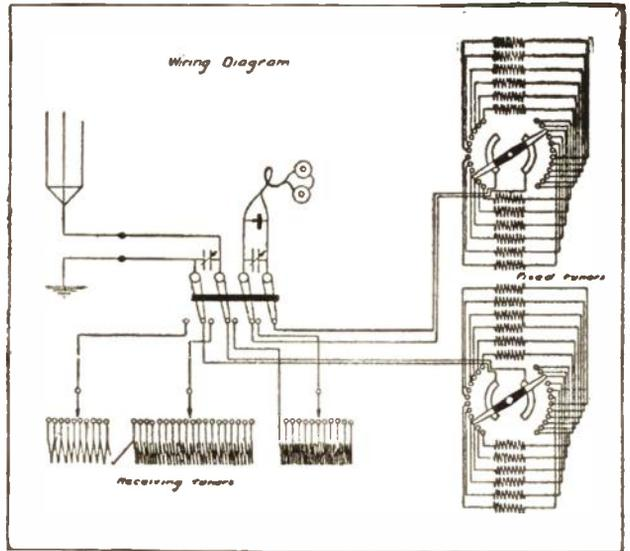
Wiring Diagram for the Inductive Tuner.
