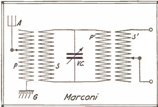
A Diagram of the Marconi Scheme for a Multiple Tuner.
