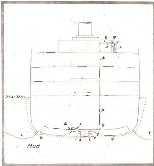
Diagram of the "Zeeland's" Position on the Mudbank, as Well as the Method of Installing the Piping Through Which the Compressed Air Was Forced for Blowing Out the Mud Beneath the Vessel.
