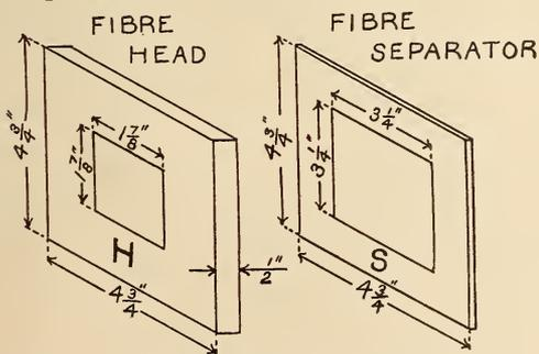
FIG. 2. CONSTRUCTION OF FIBRE HEADS
