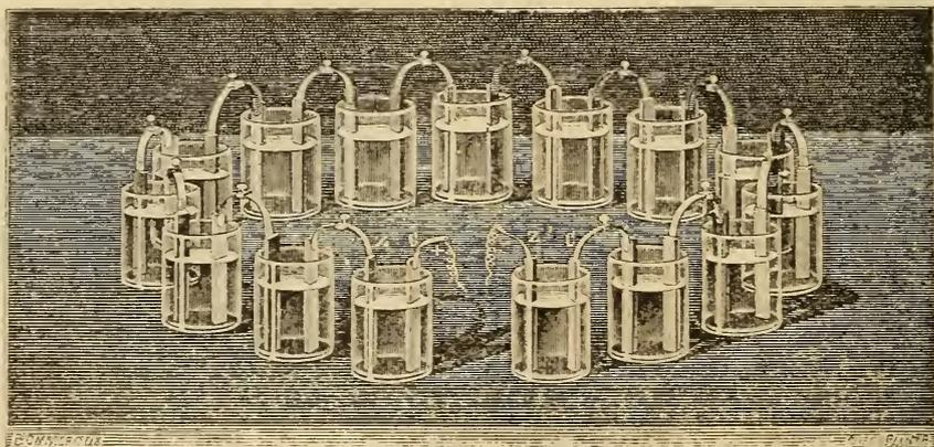
FIG. 115. FIFTEEN VOLTAIC CELLS CONNECTED IN SERIES
