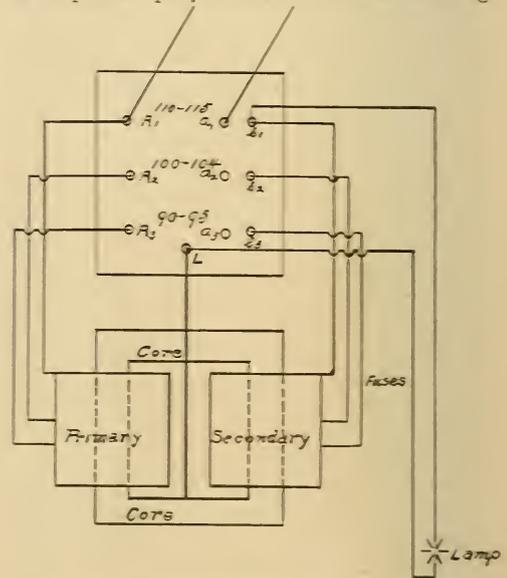
FIG. 4. CONNECTIONS OF BELL AUTO-TRANSFORMER
