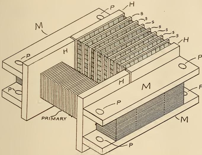
FIG. 6. PERSPECTIVE VIEW OF TRANSFORMER PARTS
