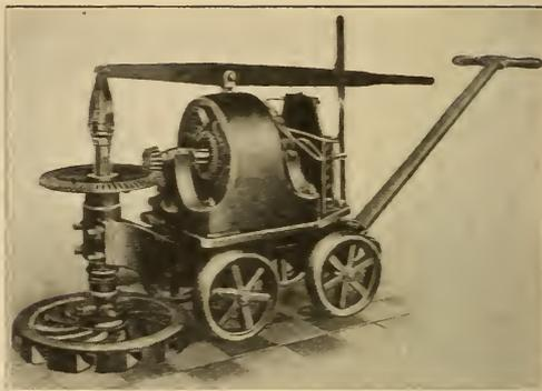
FIG. 1. SURFACING MACHINE
