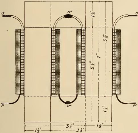
FIG. 3. STEPS IN CONSTRUCTION OF A CORE TYPE TRANSFORMER
