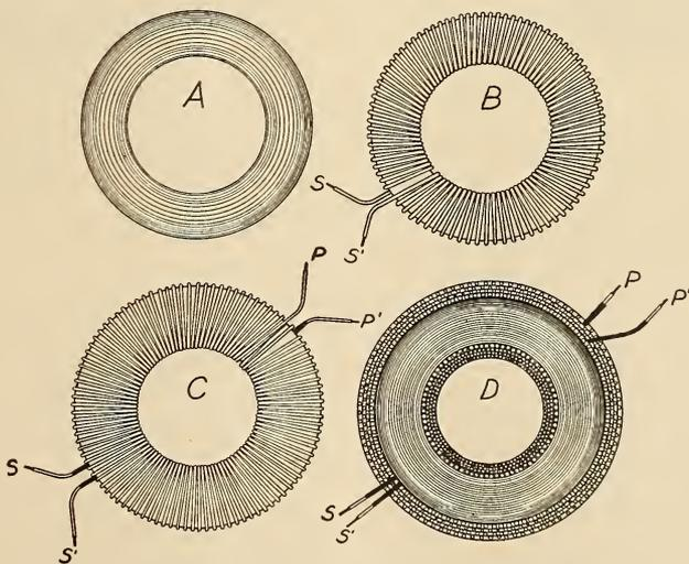
FIG. 1. STEPS IN CONSTRUCTION OF RING TRANSFORMER
