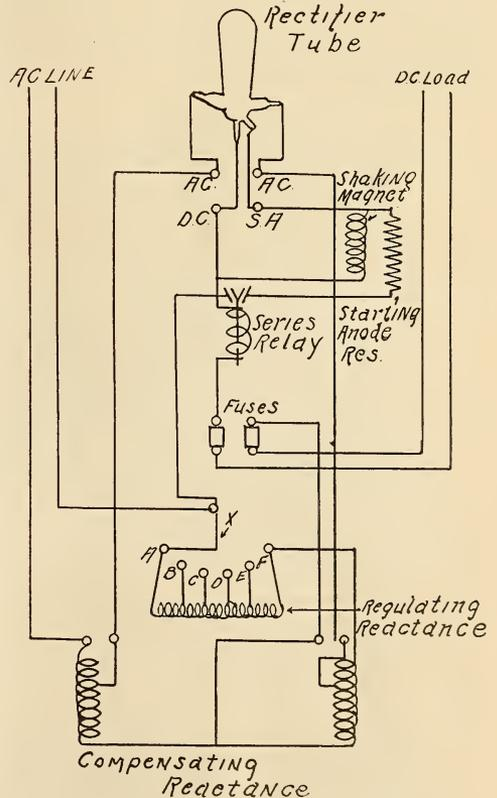
FIG. 13. CONNECTIONS OF MERCURY ARC RECTIFIER
