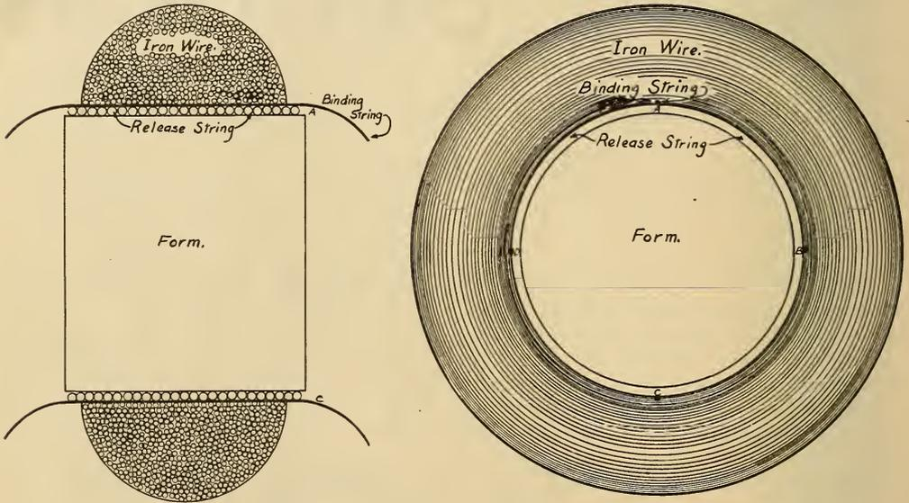
FIG. 2. WINDING OF THE CORE
