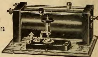
Double slide tuning coil—Wave length 100 to 300 meters—Latest type detector condenser—Mounted on mahogany base.
