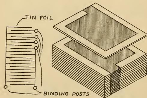
FIG. 8. METHOD OF ASSEMBLING CONDENSER
