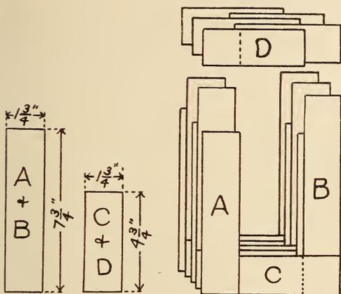
FIG. 1. THE DIMENSIONS OF CORE
