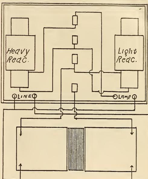
FIG. 6. CONNECTIONS OF COMPENSARC
