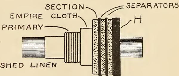
FIG. 3. ASSEMBLY OF PRIMARY AND SECONDARY
