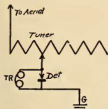
FIG. 25. CONNECTIONS OF SINGLE SLIDE TUNING COIL
