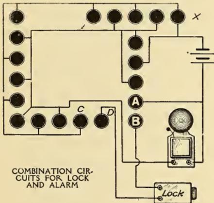
serves as a lock. With this device, when bought from the dealer, is also furnished a stiff spring, designed to fit into the jamb of the door. This does the duty of forcing the door open when the electric lock, or door opener, is operated. In the present case the spring is attached to the chest and exerts an upward pressure against the lid.
