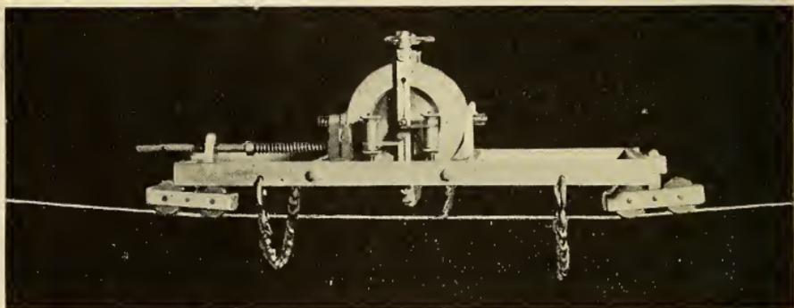
A GYROSCOPE CAR: IT CANNOT BE DISLODGED EVEN BY SWINGING THE CABLE
