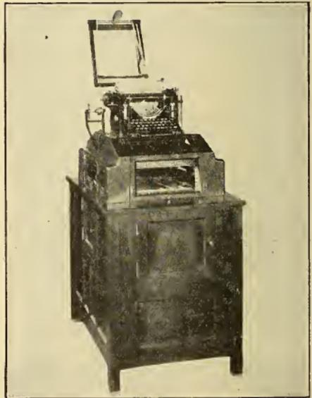
THE OPERATOR, SHOWING THE LETTER HEAD FEED MECHANISM
