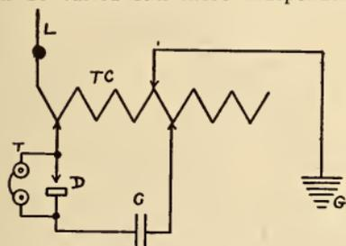
FIG. 27. CONNECTIONS OF THREE SLIDE TUNER
