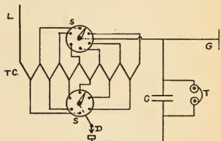
FIG. 28. CONNECTIONS OF DOUBLE POINT TUNER
