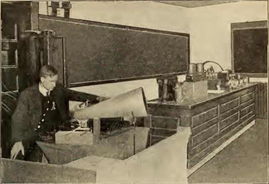
A VOICE IN A DISTANT ROOM, SPEAKING OR SINGING INTO AN ARC LAMP CIRCUIT, IS REPRODUCED AT THE FUNNEL—AN EXPERIMENT UNUSUALLY FASCINATING
