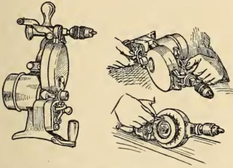
A PORTABLE DRILL WITH GRINDER ATTACHMENT
