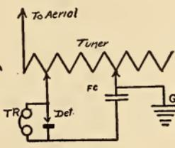
FIG. 26. CONNECTIONS OF DOUBLE SLIDE TUNING COIL
