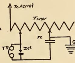
FIG. 26. CONNECTIONS OF DOUBLE SLIDE TUNING COIL
