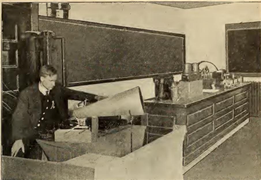
A VOICE IN A DISTANT ROOM, SPEAKING OR SINGING INTO AN ARC LAMP CIRCUIT, IS REPRODUCED AT THE FUNNEL—AN EXPERIMENT UNUSUALLY FASCINATING
