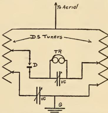
FIG. 31. CONNECTIONS OF INTERFERENCE PREVENTER.
