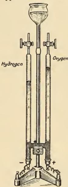
APPARATUS FOR WATER ELECTROLYSIS
