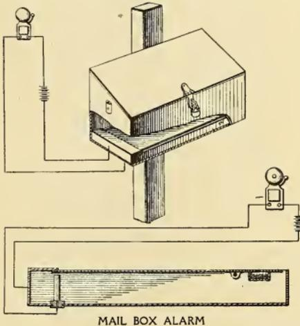
sists of a tilting bottom in the box in the form of a lever slightly weighted at one end and provided with an electric contact under the other. A postal card dropped into the box will cause the tilting bottom to swing down and close the bell circuit.
