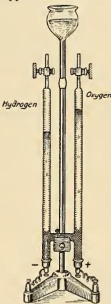
APPARATUS FOR WATER ELECTROLYSIS
