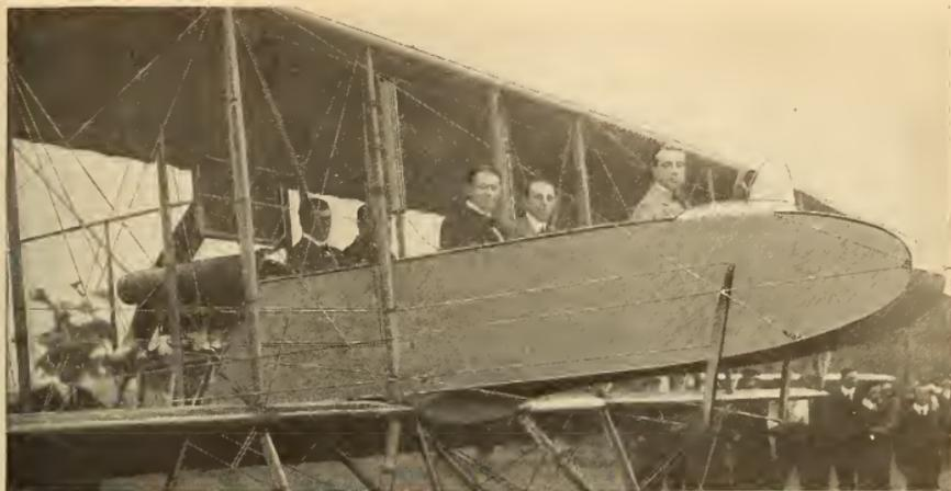
A successful trial flight with a new type of passenger carrying biplane was undertaken recently in England. The machine has a span of 75 feet. Four passengers were piloted by Mr. Grahame-White over several circuits at an altitude of about 300 feet.
