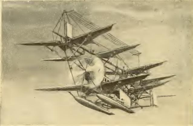
The Batson Aero-Yacht, a Great Machine, with Multiple Wings Designed for Great Stability and Carrying Power Sufficient, it is Hoped, for Trans-Oceanic Flight
