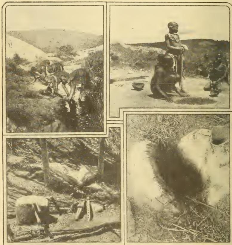
Washing the Iron Bearing Sand at the Side of a Stream Interior of a Native Blacksmith's Shop where Ore Smelting and Sword Making are Performed
