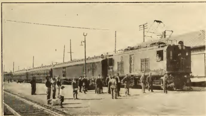
First Electric Motor Passenger Train on the Butte, Anaconda & Pacific Railroad—the Only Railroad, by the Way, which is Operated Entirely by Electricity
