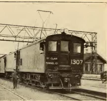
Electric Locomotive of the St. Clair Tunnel at Port Huron, Mich. It is capable of Hauling the Heaviest Freight and Passenger Trains through the Great Bore
