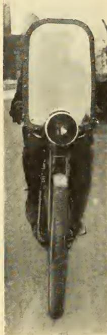
One of the principal objections to motorcycling on cold and windy days has been overcome by the introduction of a motorcycle wind shield. As seen in the illustration it can be attached to the handle-bars of any motorcycle in two minutes' time by means of adjustable clamps and consists simply of a metal frame one foot wide and two feet high. The frame is glazed with a sheet of celluloid such as is used in automobile curtains and weighs five pounds complete.
