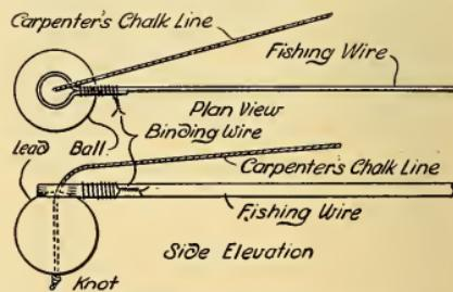
Fig. 2. Method of Making Ball and Loop
