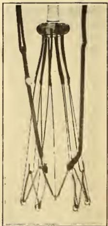
Showing the Spiral Form of the Nitrogen Lamp Filament
