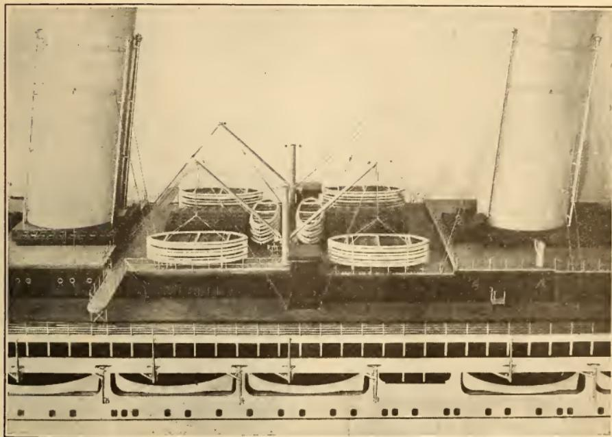
**Collapsible Boats Nested Between the Funnels of the S. S. Imperator, Arranged to Economize Space**
