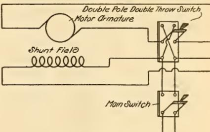
Diagram of Reversing Connections
