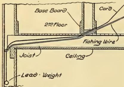
Fig. 1. How Ball and Loop Are Used
