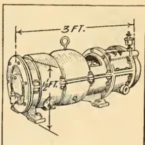
Turbo-Generator that Develops One Kilowatt on 90 Pounds Steam Pressure
