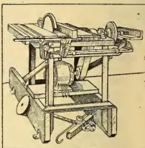
Circular Saw With a Boring Attachment
