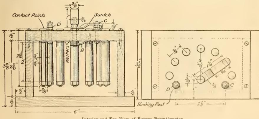
Interior and Top View of Rotary Potentiometer
