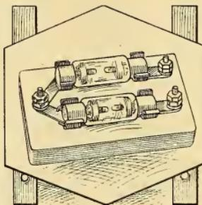
Arrester Mounted in Cartridge Fuse Manner
