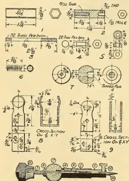
tubing and rod such as may be purchased at any experimenters supply house. The work to be done on these parts is shown in the detail drawings. It is necessary to use care to get them dressed down so that they will fit and work together smoothly.
