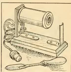
Soldering Iron Furnace in Either Round or Oval Form
