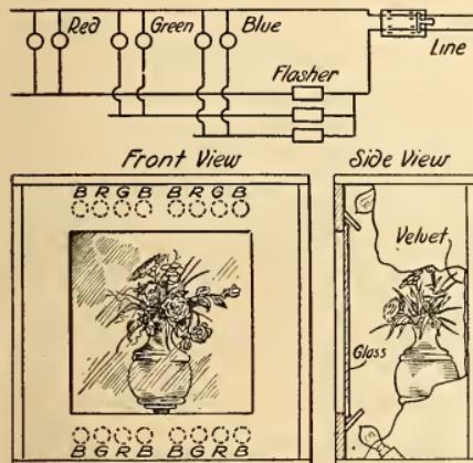
Circuit and Arrangement of Lamps
