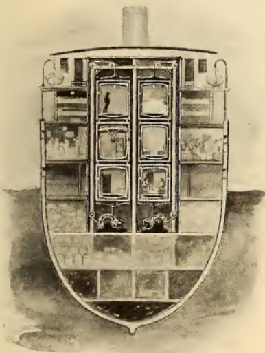
Novel Plan to Hang a Ship's Cabins in an Elevator and Control Their Action Electrically
