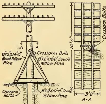
Fig. 1. Platform to Steady Pole
