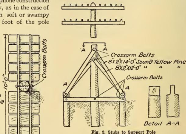
Fig. 2. Stubs to Support Pole
